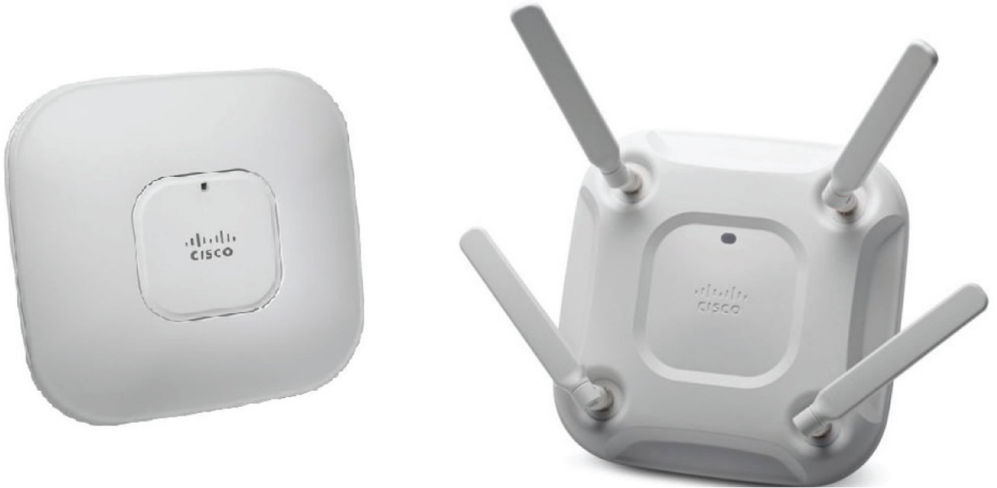
FIGURE 2.8 WAPs with internal and external antennas
