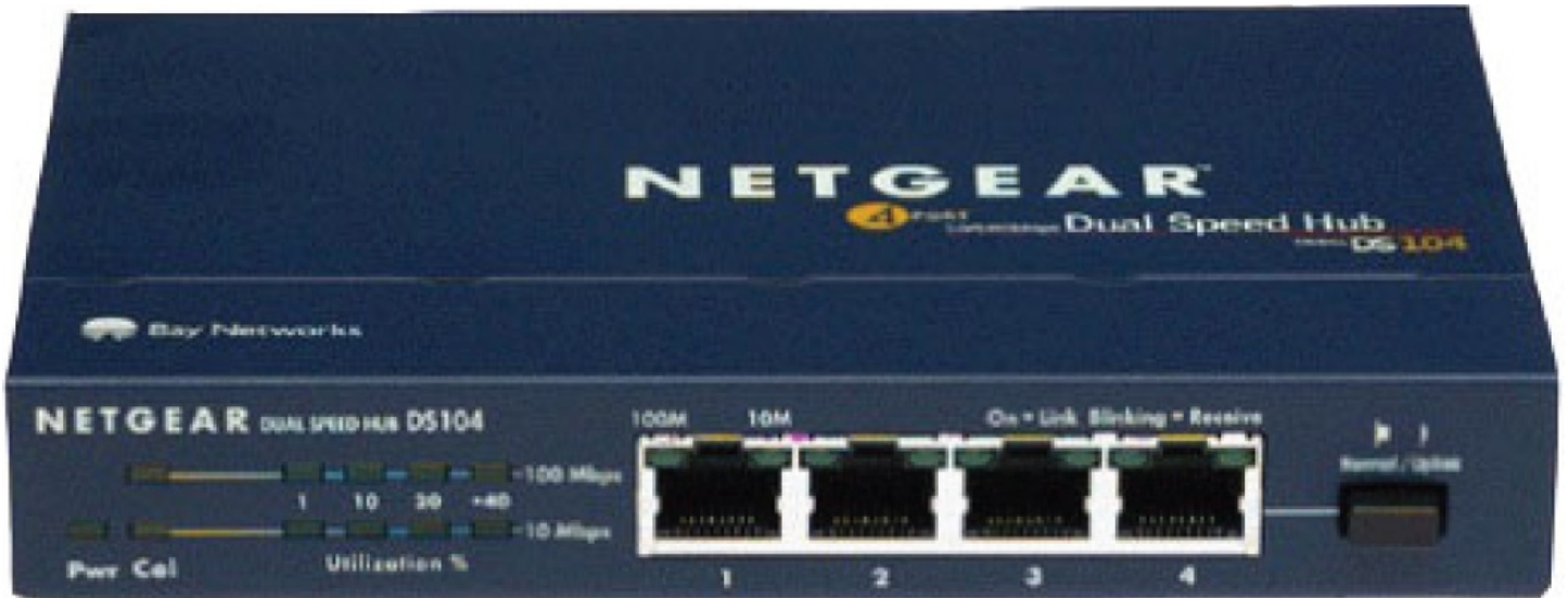
FIGURE 2.1 Four-port active hub
