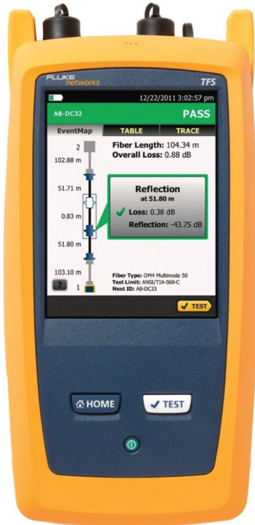
FIGURE 5.10 An optical time-domain reflectometer
