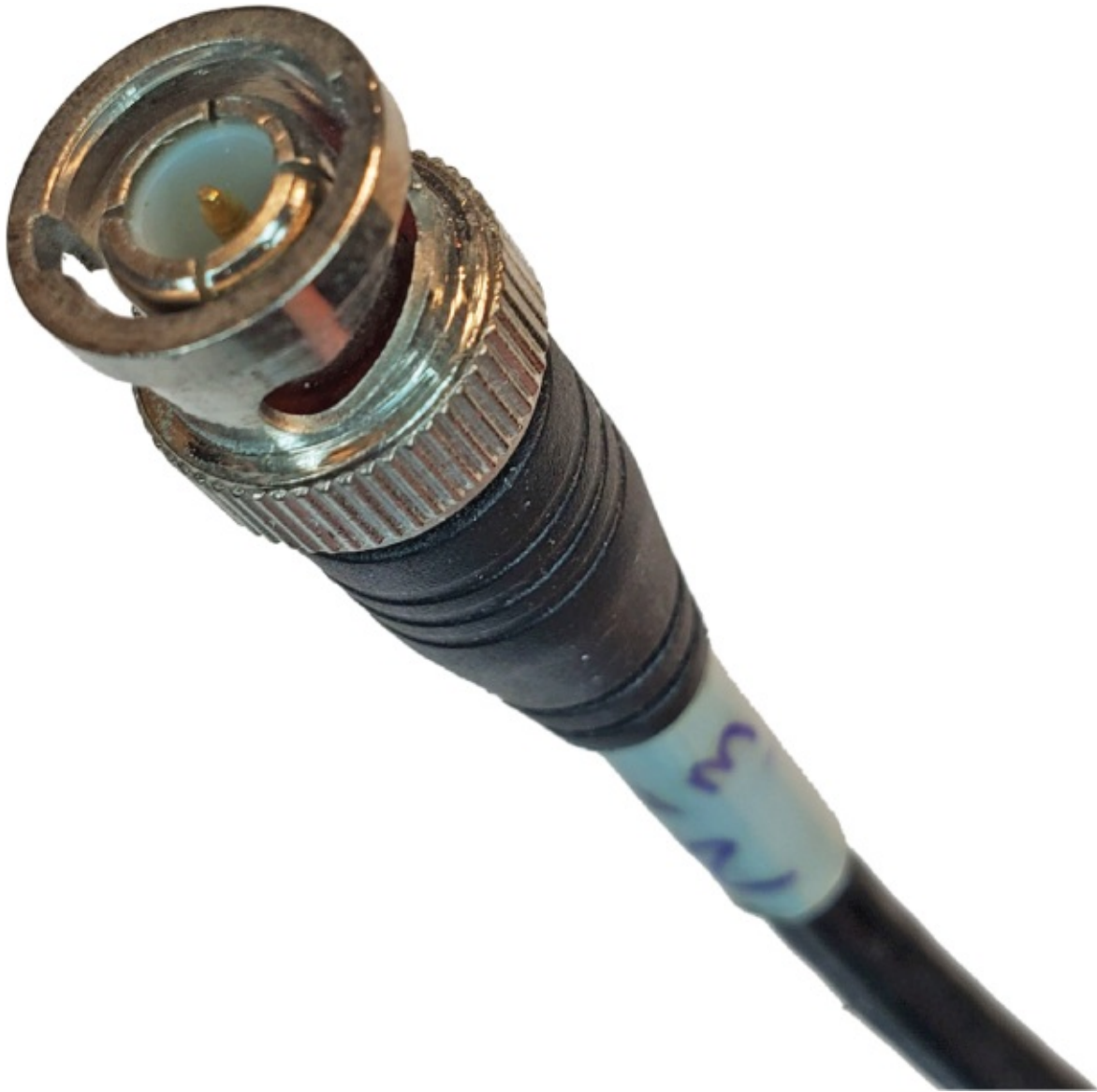
FIGURE 1.38 A BNC connector
