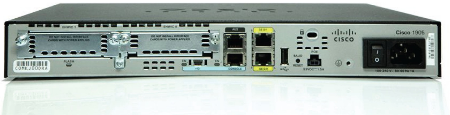
FIGURE 2.5 Typical edge router
