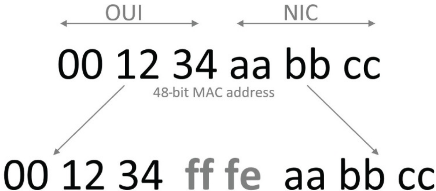
FIGURE 1.71 Padding process of EUI-64 addresses
