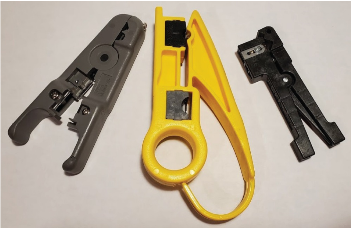
FIGURE 5.18 Typical cable strippers
