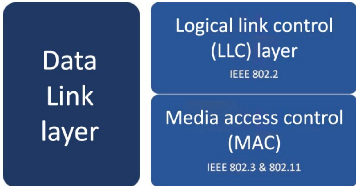
FIGURE 1.6 The Data Link layer and the sublayers within
