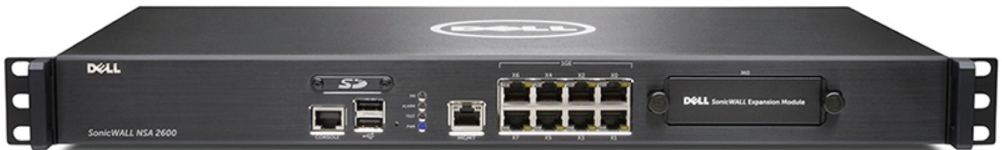
FIGURE 2.16 A typical hardware firewall appliance
