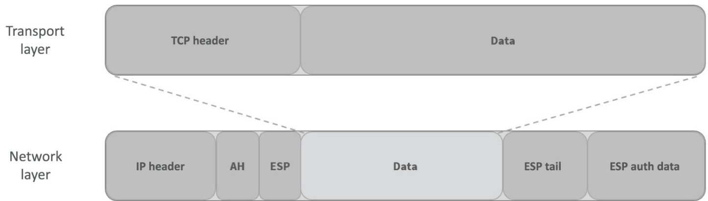
FIGURE 1.92 AH and ESP
