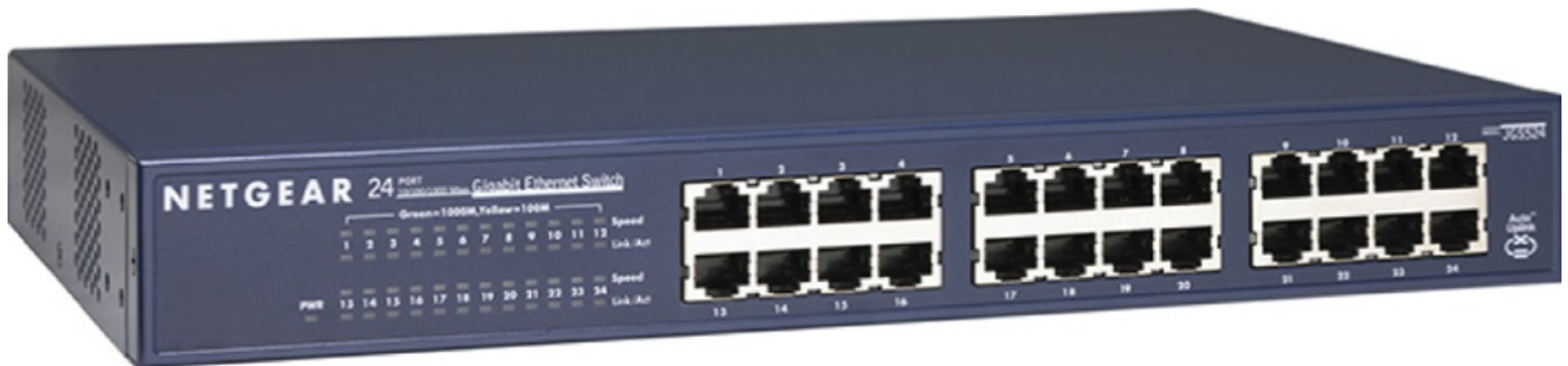
FIGURE 5.3 A typical Ethernet switch
