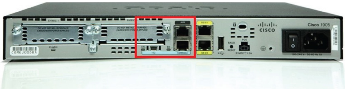
FIGURE 5.1 A router console connection
