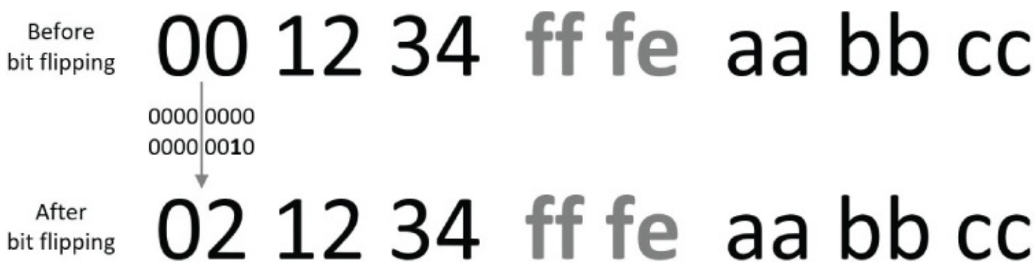
FIGURE 1.72 Bit flipping for EUI-64 addresses
