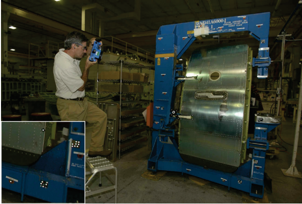
Fig. 6.35: Object recording using a photogrammetric offline system (GSI) (lower left: detail enlargement showing coded targets).
