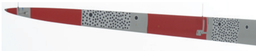
Fig. 8.51: Photogrammetric measurement of rotor blades using textured adhesive film (ForWind, Uni Hannover).
