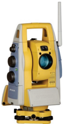
Fig. 6.14: Total station with integrated camera (Topcon GPT-7000i).
