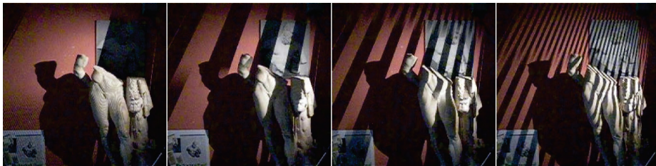
Fig. 8.13: Projected pattern and image sequence in a fringe projection system (AICON/Breuckmann).
