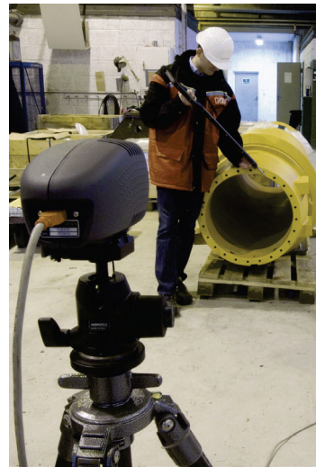
Fig. 6.29: Example of a single-camera system with 3D touch probe (Metronor).
