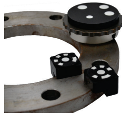
b) Targeting with flange adapters
