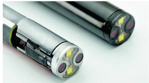
b) Stereo endoscope with two miniature cameras in the tip of the endoscope
