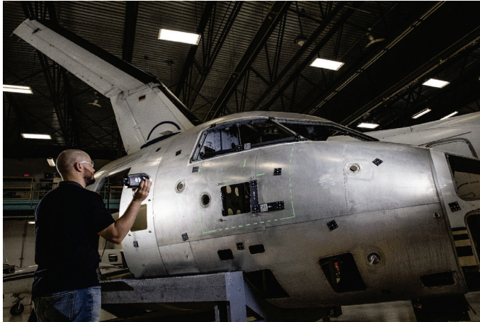
Fig. 6.36: Object measurement using an offline photogrammetry system with active projection of the field-of-view (Creaform).
