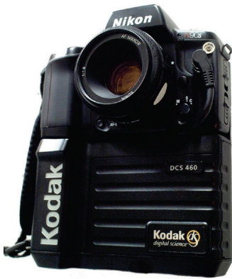
Fig. 1.44: Still-video camera Kodak DCS 460 (ca. 1996).
