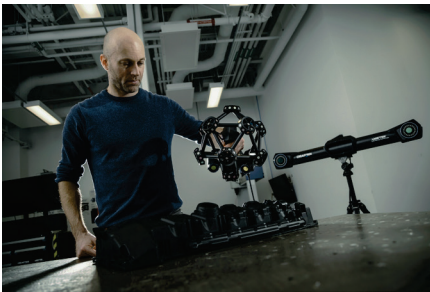
Fig. 6.85: Surface-scanning sensor located by an external stereo camera (Creaform).
