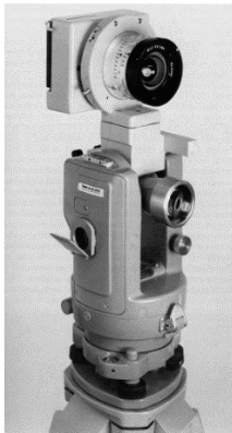
Fig. 1.31: Wild P32 metric camera mounted on a theodolite.
