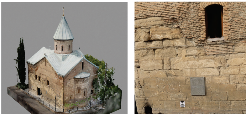
Fig. 4.30: 3D model with rectified image areas and superimposed textures (Lurdji monastery, Tbilisi, Georgia, see also Figs. 6.111 and 6.112).
