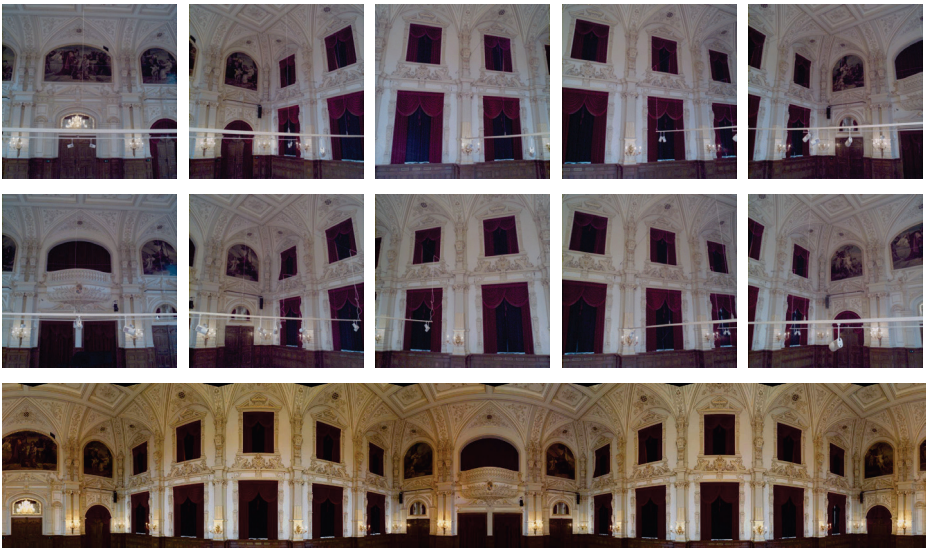
Fig. 3.138: A digital cylindrical panorama created by stitching together overlapping camera images.
