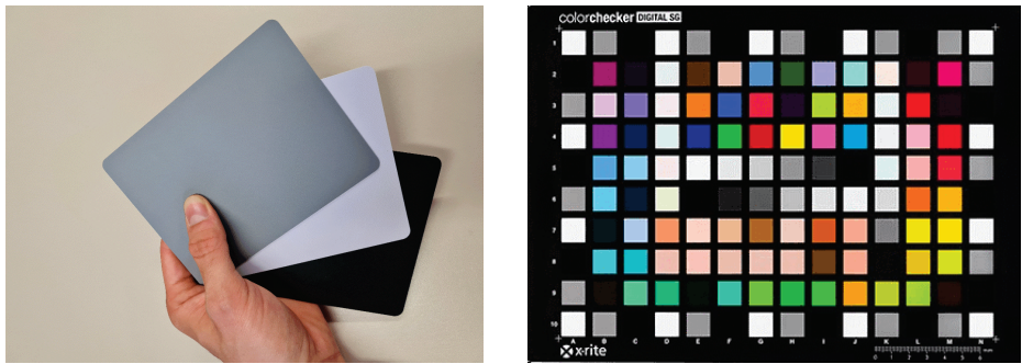
Fig. 5.28: Left: grey charts; right: colour calibration chart (X-Rite ColorChecker).
