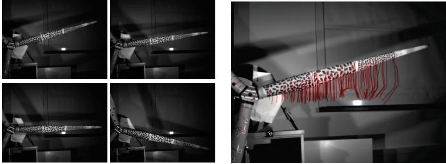
Fig. 5.109: Image sequence (left) and calculated optical flow (right).
