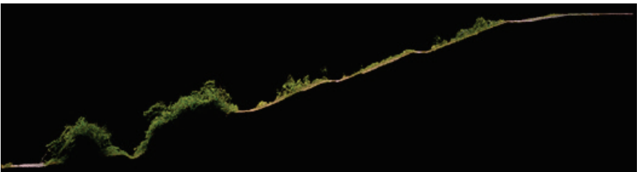
Fig. 8.38: Profile section through a DTM including vegetation (Frankfurt UAS).
