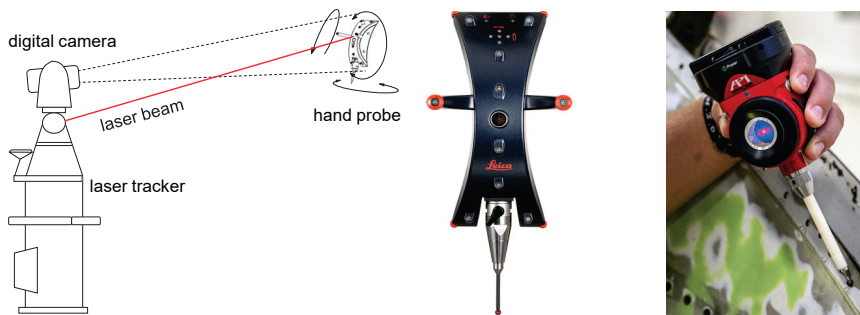
Fig. 6.19: Left: Laser tracker combined with a digital camera for measurement of position and orientation of a hand-held probe (Leica T-Probe); right: hand-held probe with internal orientation sensors (API vProbe).
