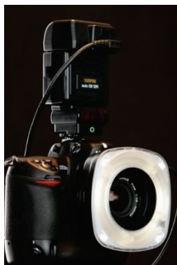
Fig. 3.155: Digital SLR camera with ring flash.
