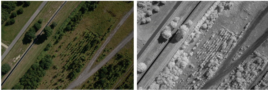
Fig. 8.39: RGB and NIR image from a drone (Frankfurt UAS).
