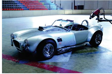
b) Surface scan by fringe projection
