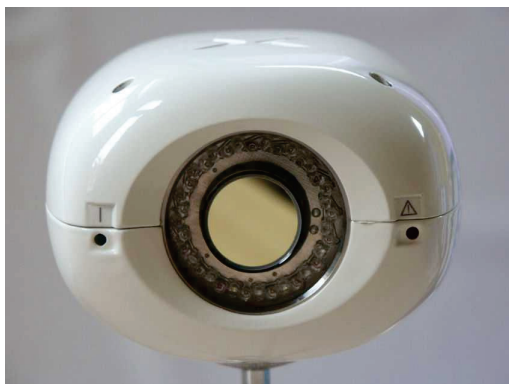
Fig. 3.156: Digital metric camera with integrated LED ring flash (AXIOS 3D).
