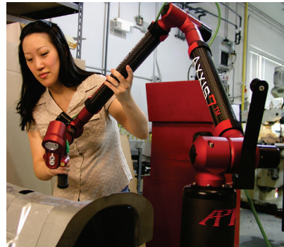
b) Line scanner attached to CMM arm (API)
