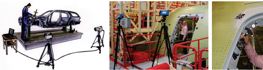
Fig. 6.34: Online metrology system with manual tactile probing (GSI).
