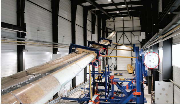
Fig. 8.60: Rotor blade during a load test (red: photogrammetric targets) (Fraunhofer IWES).
