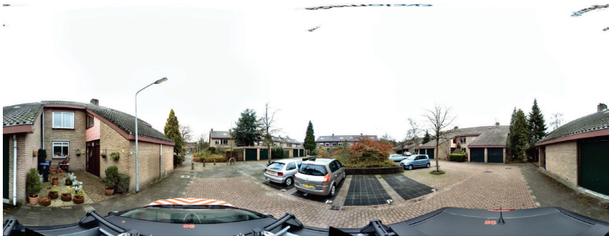
Fig. 3.140: Digital panorama created from the images in Fig. 3.139 (Cyclomedia).
