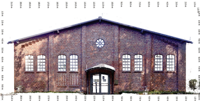
b) Orthophoto generated from a 3D point cloud and additional RGB images
