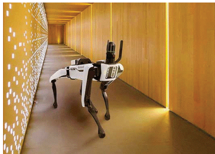
d) Autonomous robot platform with laser scanner (Boston Dynamics, Leica)
