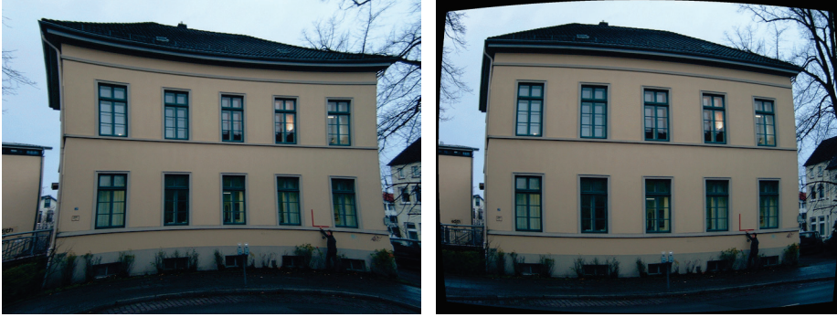
Fig. 3.18: Pincushion (left) and barrel distortion (right) in an actual image.
