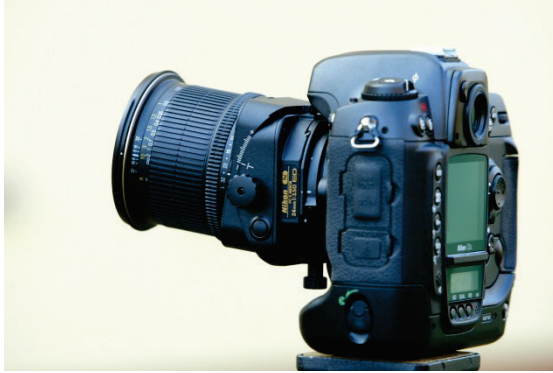
Fig. 3.105: A digital SLR camera fitted with a tilt-shift lens.
