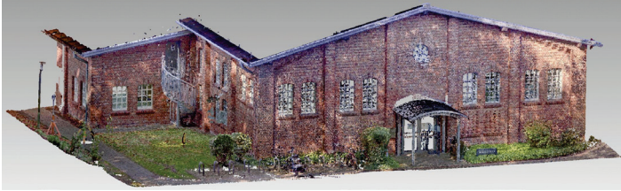
a) Complete registered point cloud generated using individual scans from a laser scanner
