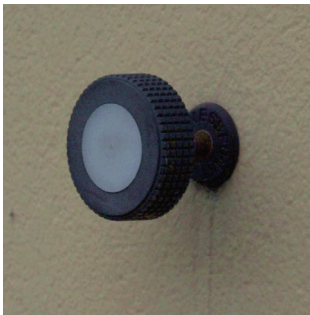
a) Target with a bright plastic centre ( \varnothing = 50 mm)
