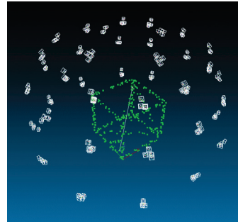
Fig. 7.17: Imaging configuration for assessment of length measurement error.
