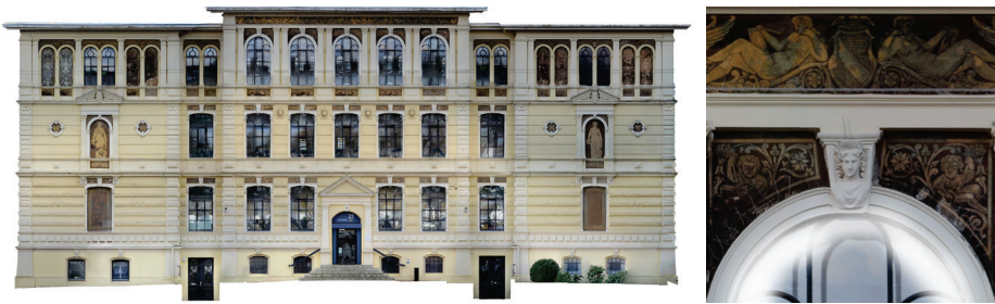
Fig. 8.4: True orthophoto of a façade with close-up detail (SPM3D).
