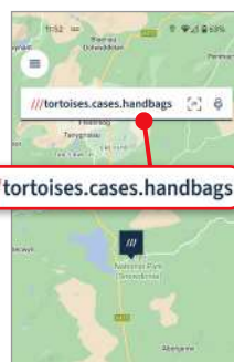
What3words divides the world into 57 trillion squares and gives each a unique three-word code
