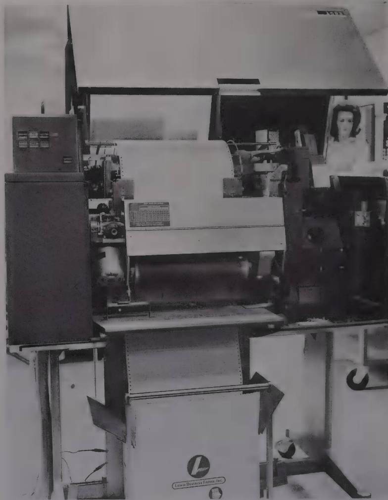
Figure 1-15. High-speed printer capable of 800 lines/minute (Photo courtesy of J. R. Langley.)
