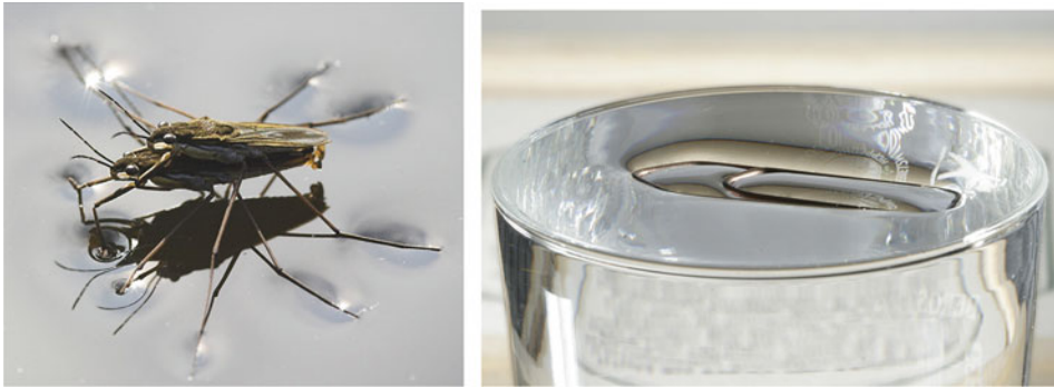
Fig. 3.7 Experimental observations as an evidence for surface tension. The surface tension of water carries water striders and a paper clip. The picture of the water striders was taken by Markus Gayda, see https://de.wikipedia.org/wiki/Datei:Wasserl%C3%A4ufer_bei_der_Paarung_crop.jpg for details. For the paper clip see https://www.wikiwand.com/de/Oberfl%C3%A4chenspannung#/Media/Datei:Surface_Tension_01.jpg
