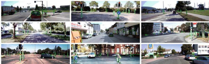
**Fig. 3.8** The calibration results on several scenarios. Green points represent the projected LiDAR line points
