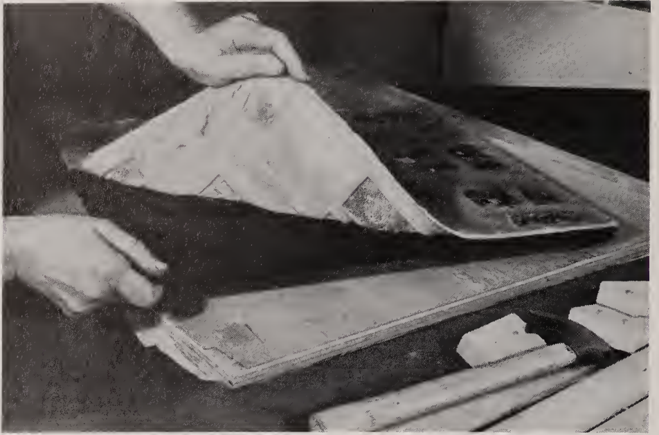
The latex release sheet is stripped easily from the panel.
