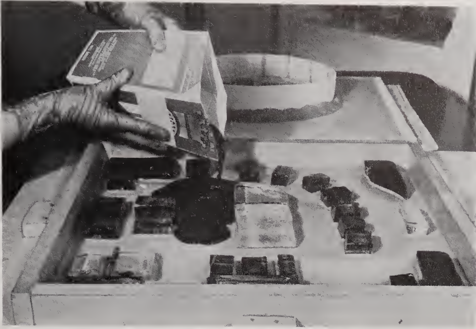
A half-gallon milk carton makes an excellent pouring vessel for the heavy dark epoxy that is poured over the dry latex. Notice the linoleum frame in the background into which excess epoxy will be poured for a smaller panel.
