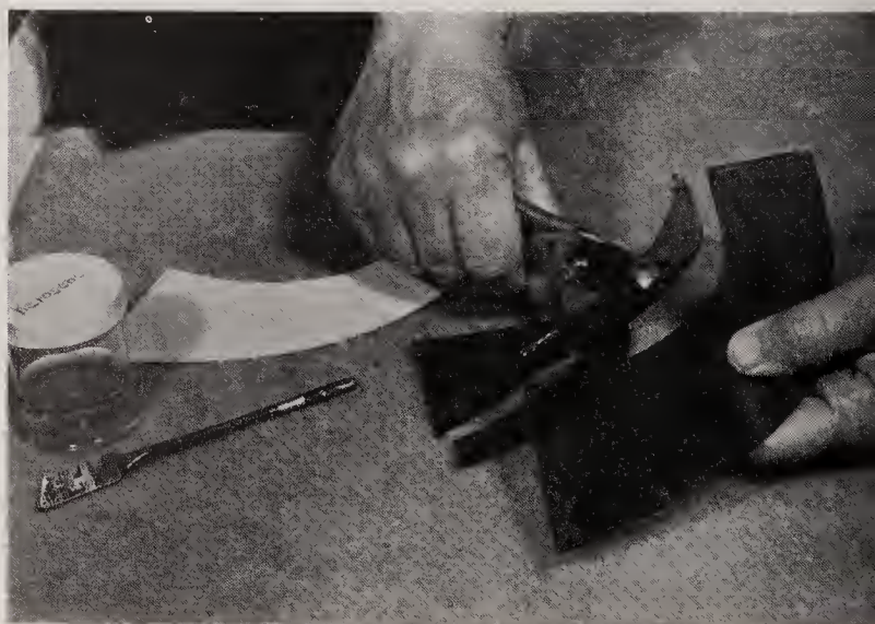
The narrow piece of glass is separated with pliers while one hand bends the larger section outward.
