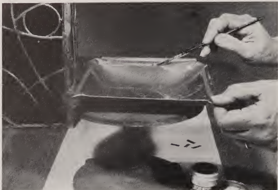
Brush low fusing 40/60 paste solder along each section of the copper top where the lantern will be positioned. Notice the small lead pieces that will be soldered into the juncture between the lantern and its top.
