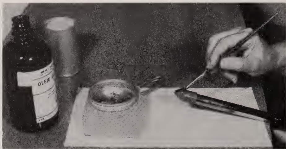
Flux the tip of the iron with oleic acid.
