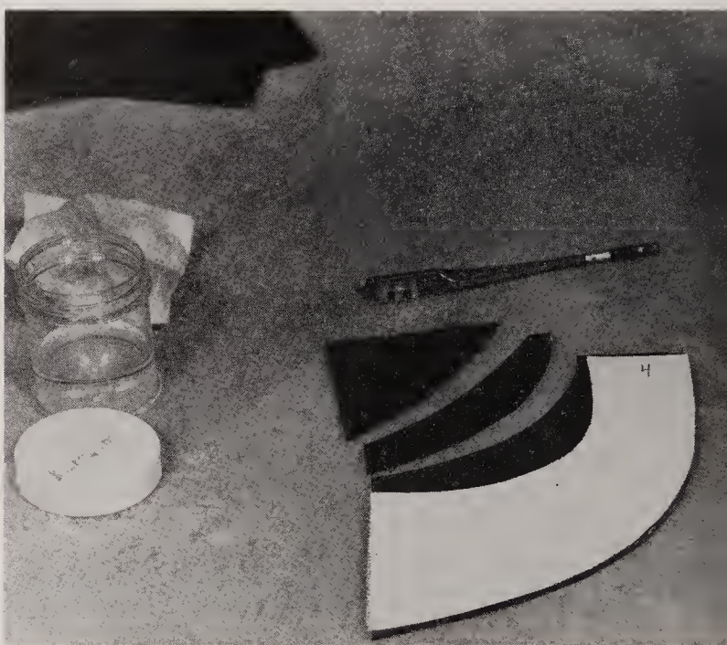
Deep curves are cut in shallow sections, one at a time.
