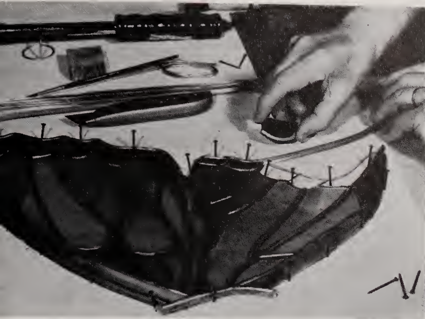
One piece of lead is bent around two sides of each border scalloped piece before it is inserted into the border leading.
