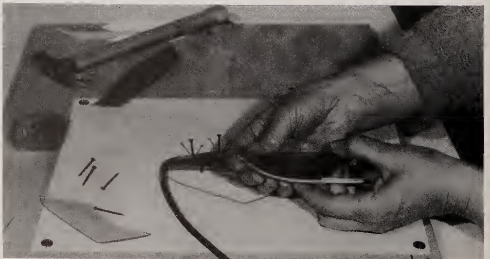
Fit lead along a curved edge by holding the glass piece and pressing the lead firmly around the curve.
