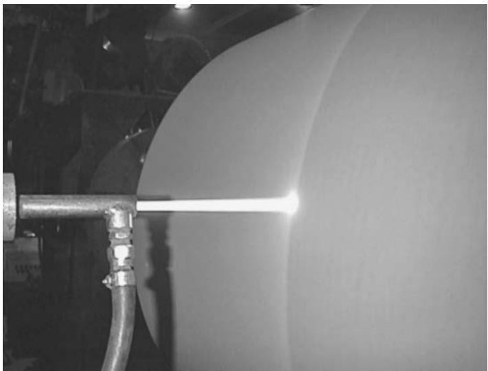
FIGURE 14.13 High-velocity oxygen fuel thermal spray process. (Courtesy of M. Gariepy, WEIR Engineering Services, Montreal, Canada)
