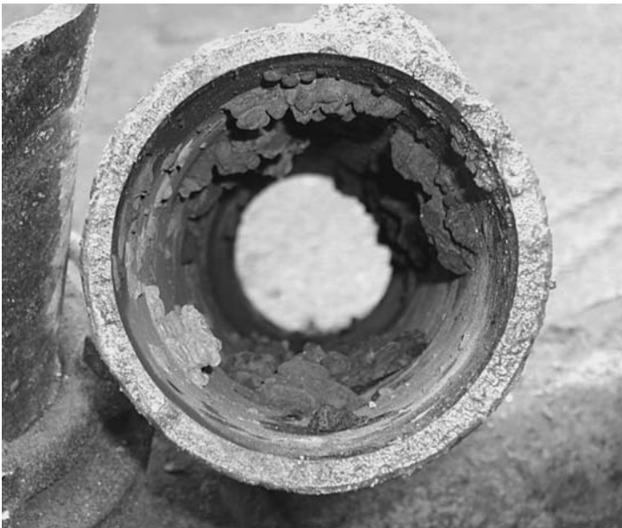
FIGURE 8.1 Tubercles in a small diameter water pipe. (Courtesy of Public Works and Services, City of Ottawa)
