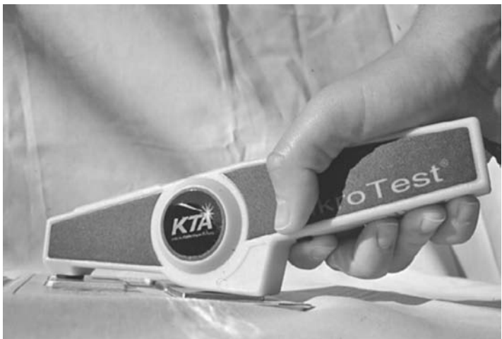
FIGURE 14.26 Magnetic pull-off dry film thickness measurement gauge. (Courtesy of KTA-Tator, Inc.)
