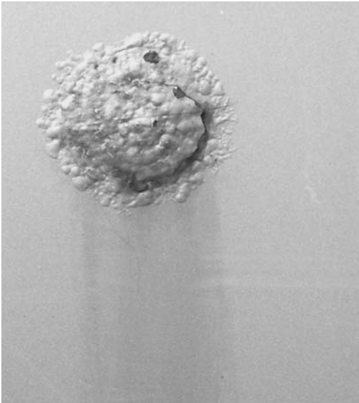
FIGURE 9.17 Filiform corrosion and paint blistering accelerated by deicing salt.
