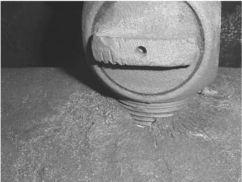
FIGURE 7.21 Corrosion of a water main ductile iron adjacent to a copper fitting. (Courtesy of Drinking Water Services, City of Ottawa)
