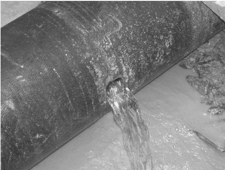
FIGURE 10.5 A corrosion pit that led to the perforation and leak of a water main. (Courtesy of Drinking Water Services, City of Ottawa)
