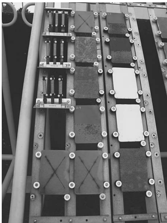
FIGURE 9.43 Coated panels exposed on an atmospheric test rack in a marine environment with CLIMAT coupons for corrosivity calibration. (Courtesy of Defence R&D Canada-Atlantic)
