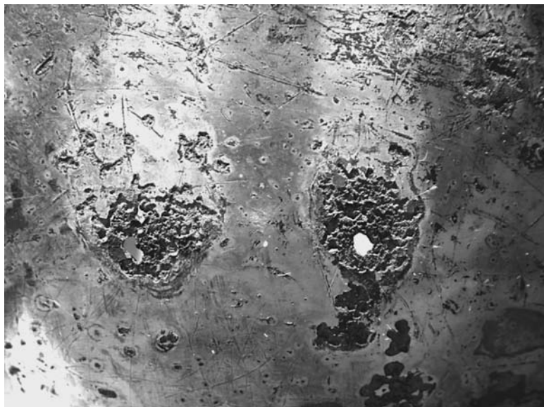
FIGURE 9.50 Close-up of corrosion pits in a water jug (Fig. 6.8) made of a silver-plated zinc casting.
