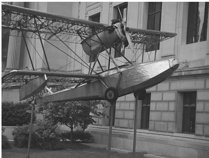
FIGURE 9.48 The Budd BB-1 Pioneer built in 1931 and mounted on a pylon outside the Franklin Institute Science Museum in Philadelphia. The lower wing and empennage fabric has been lost to the weather.
