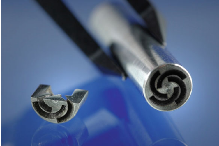
Fig. 31.16 Nozzle for water jet deburring. Source ILT
