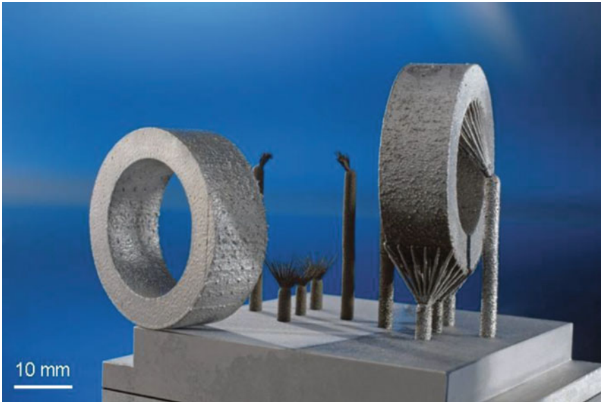
Fig. 7.67 Left: etched and ultrasonically cleaned test geometry, right: untreated test geometry (ring profile), reprinted from Schmithüsen et al. (2017)
