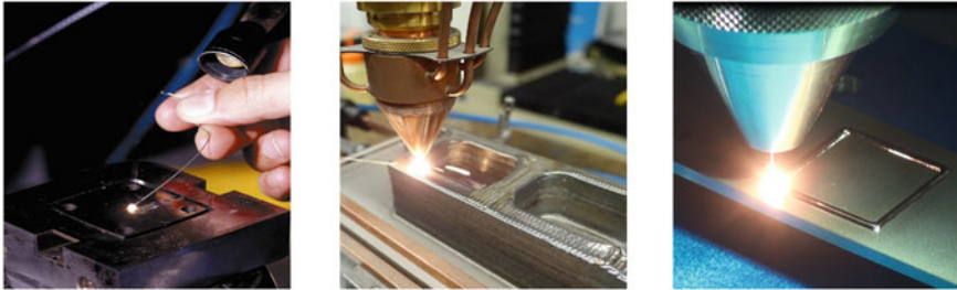
Fig. 8.2 Pulsed laser LMD process with manual wire feeding (left) and automated LMD processes with cw laser radiation and continuous powder feeding (middle) and coaxial wire feeding (right)
