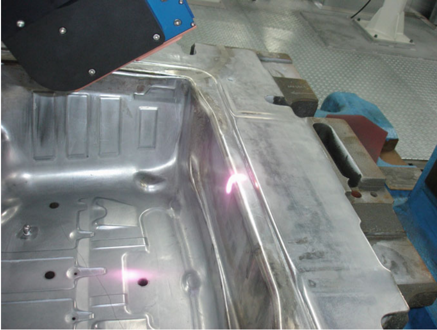
Fig. 6.20 Laser hardening of a tool using the system technology depicted in Fig. 6.19
