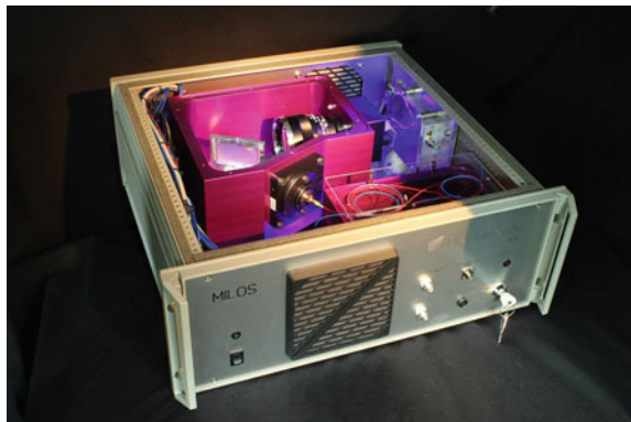
Fig. 39.9 Control unit (19-inch rack), fiber optics (yellow cables) and measuring head (black cylindric housing) of a »bd-2« sensor. Photo Fraunhofer ILT
