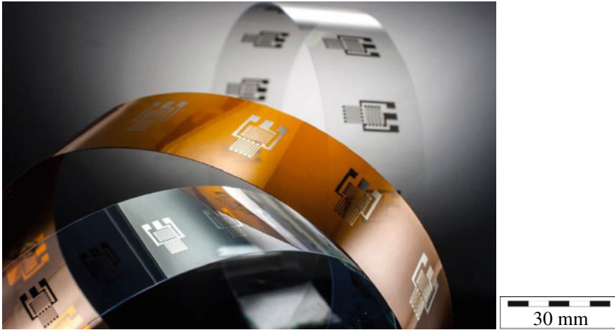
Fig. 16.1 Printed and laser sintered strain gauge on various temperature-sensitive polymers (Fraunhofer ILT 2020)
