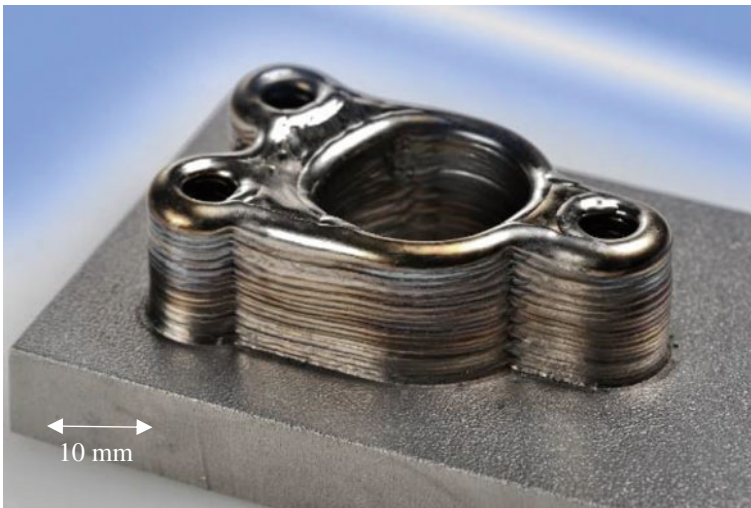
Fig. 12.6 Part out of Inconel 718 built with the coaxial wire LMD process
