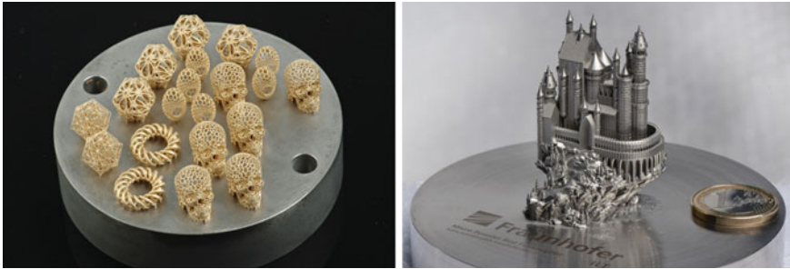
Fig. 7.43 Left: jewelry parts made of gold after micro bead blasting, right: castle made of stainless steel 316L in the “as built” state
