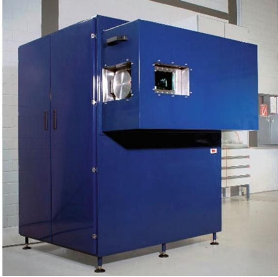
Fig. 40.8 High-speed scanning LIBS microanalysis system SML to measure steel samples for the analysis of segregations, inclusions, and decarburization zones
