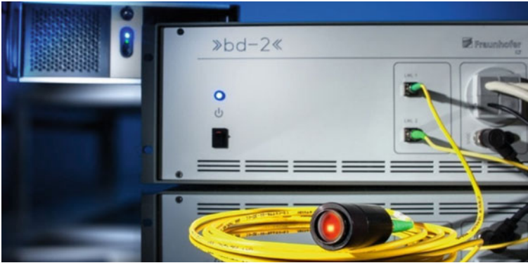
Fig. 39.9 Control unit (19-inch rack), fiber optics (yellow cables) and measuring head (black cylindric housing) of a »bd-2« sensor. Photo Fraunhofer ILT
