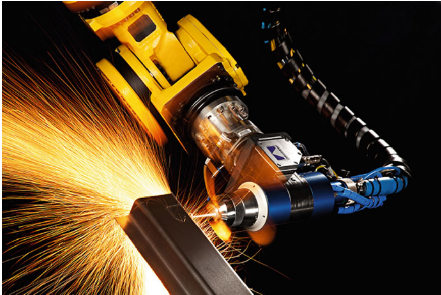
Fig. 38.10. 3D laser cutting by use of solidcutter; Source of image Precitec GmbH and Co. KG, Gaggenau-Bad Rotenfels, Germany
