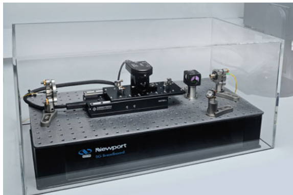
Fig. 39.11 Calibration setup for »bd-x« sensors with ultra-precision linear stages
