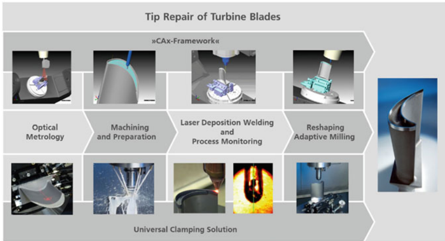
Fig. 13.2 Exemplary process chain for automated adaptive turbine blade repair (TurPro 2013)
