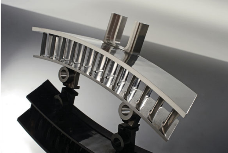
Fig. 7.57 12-Row guide vane cluster manufactured with LPBF and post-processed with MMP
