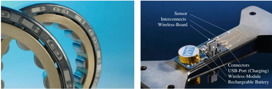
Fig. 16.12 Additively manufactured thick film strain and body sound sensors on roller bearings (varying production steps) through print and laser process (left) (Vedder et al. 2017), Additively manufactured thin film strain gauge (full bridge) with wireless telemetry on metal component (right) (Vedder 2021)
