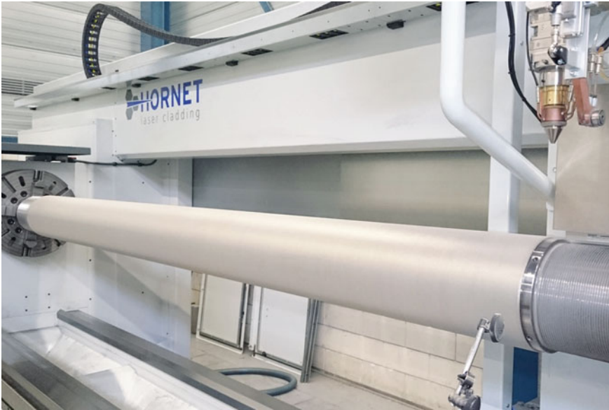
Fig. 14.9 Hydraulic cylinder coated with the EHLA process (Inconel 625). Source IHC VREMAC Cylinders
