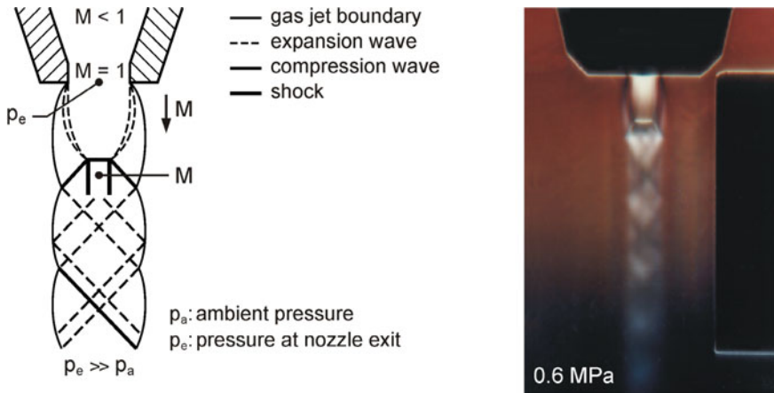
Fig. 32.3 Schematic and Schlieren optical representation of the free jet under a cutting nozzle
