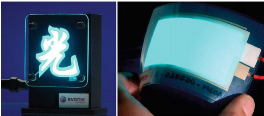
Fig. 19.15 Electroluminescence lamps with printed and laser-treated ITO layers on glass and polymer substrates (Vedder 2013)
