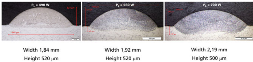
Fig. 12.4 Cross sections of single tracks out of Inconel 718 produced with different laser power P_L
