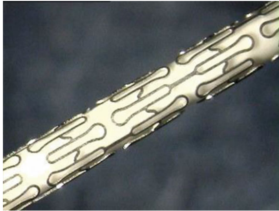
Fig. 36.6 Laser cut stent (diameter 1.6 mm) after polishing (© Fraunhofer ILT)
