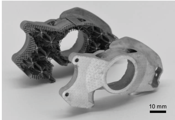
Fig. 7.69 Parts before and after wet-chemical etching
