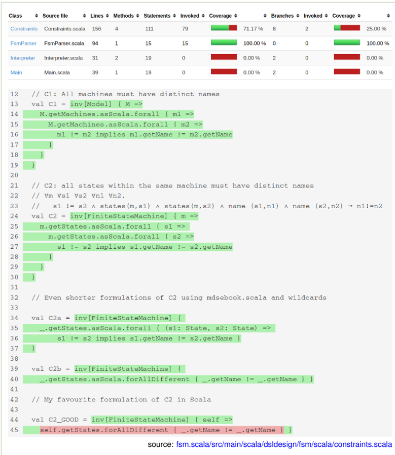
Figure 5.21: A fragment of a test-coverage report for tests of constraints for the fsm example; Top : a summary of the statistics, Bottom : detailed coloring of covered and not covered code
