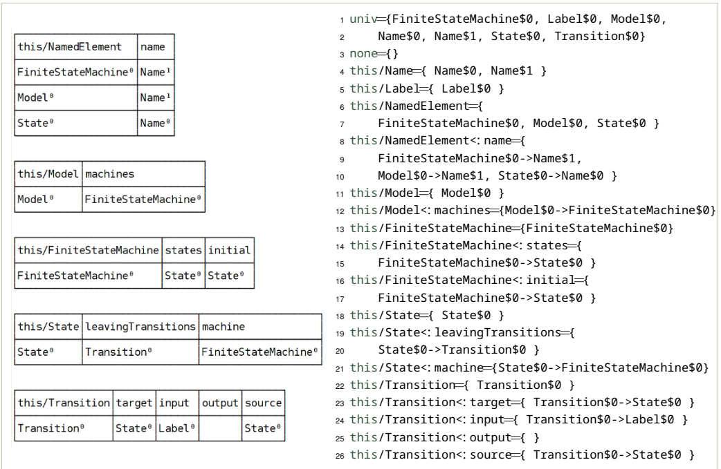
Figure 5.14: An example instance generated by Alloy tools for the model in Fig. 5.12. Presented as relations in the left column, and using Alloy's textual instance syntax in the right column
