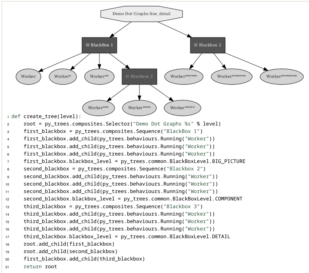
Figure 10.17: Bottom: an internal DSL model of a behavior tree in py_trees syntax. Top: a visualization of the same model generated using py_trees tools. Source: https://github.com/splintered-reality/py_trees , BSD Licensed code
