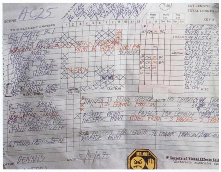
A line-up sheet. This is used to plot the way in which elements of a composite shot are combined in an optical print.
