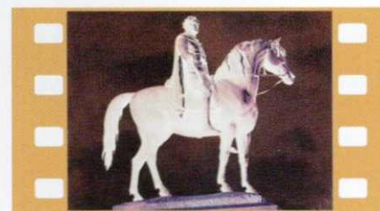
3 Internegative . Made from copying the master negative on to reversal film to produce another negative, or by copying the master positive on to negative film. Many additional positives can be struck from this film – edited release prints, for example. Also called an interdupe or colour reversal intermediate .
