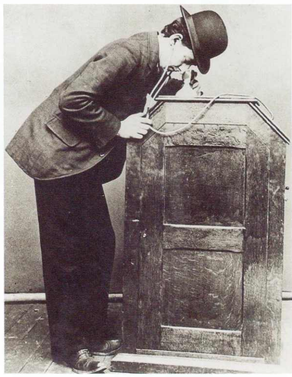
Edison's 1894 Kinetophone improved on the Kinetoscope, combining moving images with a soundtrack provided by the Phonograph.
