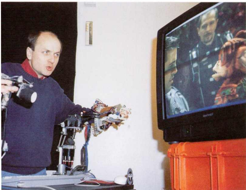
The Henson Performance Control System allows puppeteers to engineer the actions of their characters by remote control. The performer places their hands in a pair of mechanical gloves; a video camera and monitor are used to view the puppet's actions when it is some distance away.
