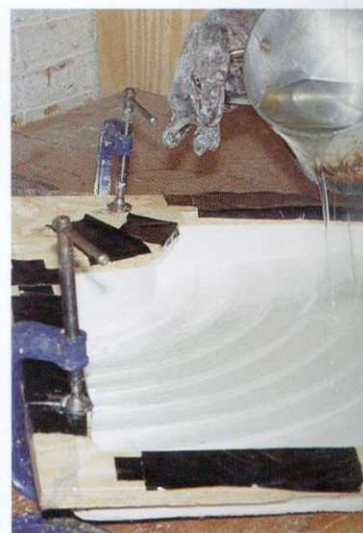
Making breakaway glass. Far left: Pieces of solid resin are melted over a stove. Below: The liquid resin is poured into rubber, plastic or fibreglass moulds. Right: As the resin sets, its surface is warmed to prevent bubbles and ripples. Far right: The set resin is carefully removed from its mould, ready for use. This shape is one quarter of a lighthouse lens for the film The Lighthouse (2000).
