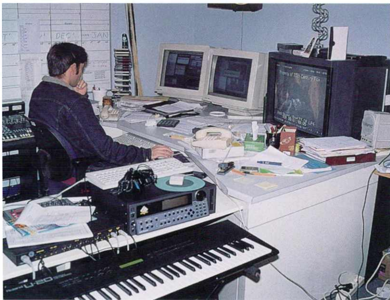
A typical modern sound-mixing suite. Digitized sounds are mixed in a computer and can even be played like music on a keyboard. There is a library of compact discs to hand, containing a huge range of pre-recorded sound effects.
