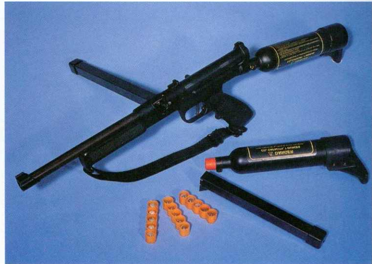
A gun using compressed air to fire capsules containing blood, silver paint or zirconium can be used to create a number of bullet-hit effects.
