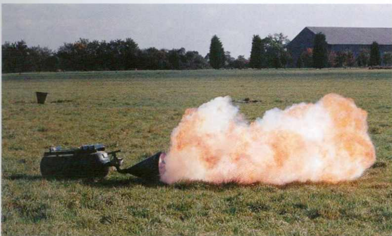
Compressed propane gas is expelled and ignited by a gas mortar.
