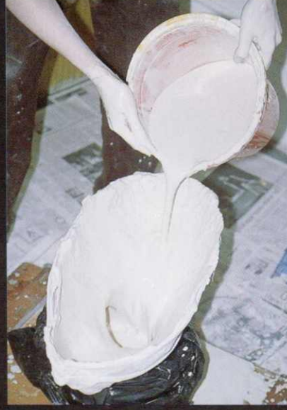
The empty mould is then turned upside down and filled with liquid casting plaster
