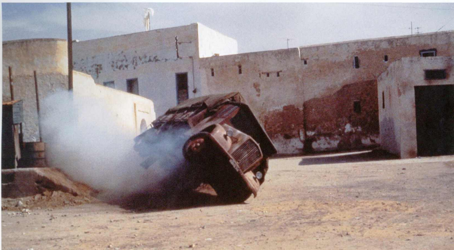
A pyrotechnic cannon fitted to the underside of a truck was used to tip the vehicle over in this scene from Raiders of the Lost Ark (1981).
