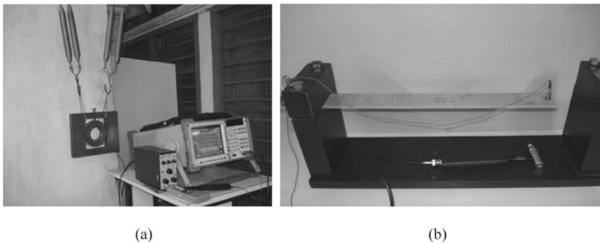
Fig. 9.1 Boundary conditions in modal testing: a free, b fixed
