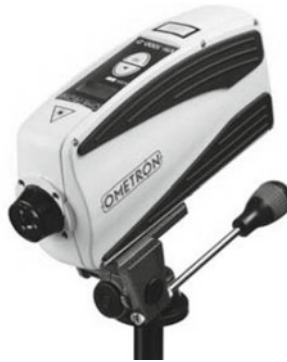
Fig. 3.18 Laser Doppler vibrometer (Courtesy of Brüel & Kjær, Denmark)
