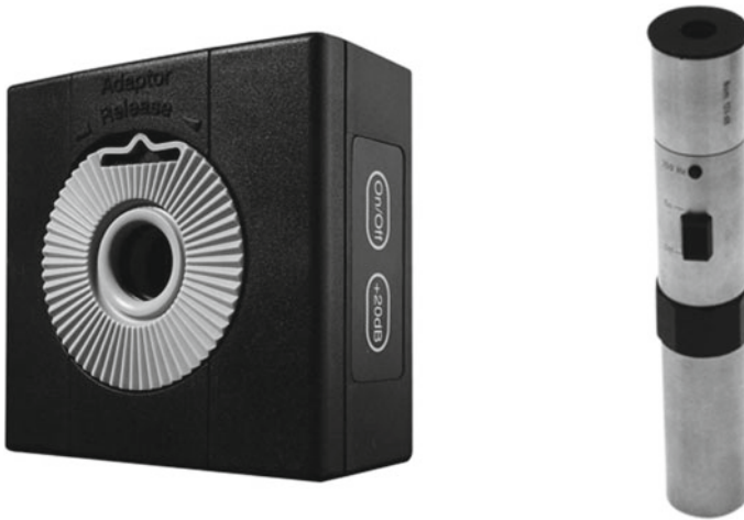
Fig. 5.19 Photographs of calibrators (Courtesy of Brüel & Kjær, Denmark)
