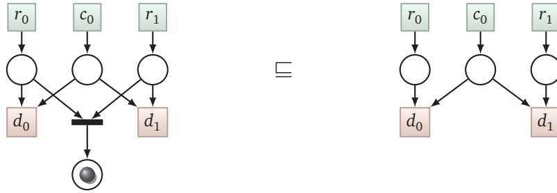
Figure 16.4: Deleting terminal places refines the specification.
