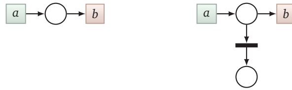
Figure 3.6: Petri nets clearly distinguish between two processes with similar interfaces but different progress obligations. The left Petri net always acknowledges an input on a with an output on b , which the right one need not.
