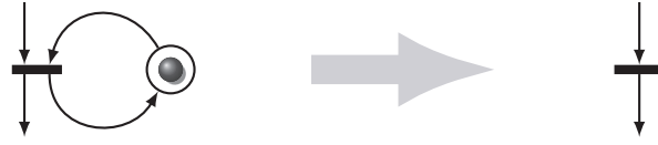
Figure 9.4: A marked place whose preset coincides with its postset and contains only one transition may be deleted.
