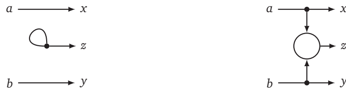
Figure 15.3: a correct but suboptimal implementation (left) and an irredeemably wrong implementation (right) of the process in Figure 7.8
