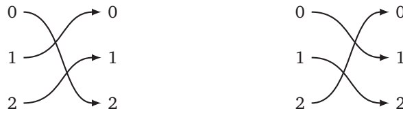
Figure 8.10: Left, the permutation network described by \langle 2, 0, 1 \rangle acknowledges input 0 with output 2, input 1 with output 0, and input 2 with output 1, contrary to that of \langle 2, 0, 1 \rangle^{-1} , right.
