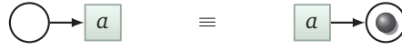
Figure 5.1: A permanently disabled/unsafe input transition a is expressible as such in an open Petri net by an unmarked preset place disable it (left) or by a marked postset place to make it unsafe (right), with either alternative being semantically equivalent to the other.
