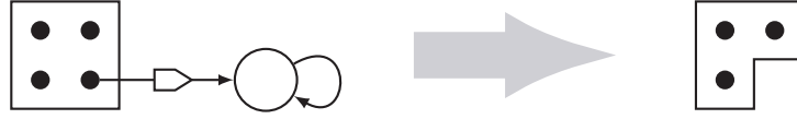
Figure 11.2: If there were no better way to implement an LJOIN, it could be made from a dense decision wait of similar dimensions with the outputs due to invalid input combinations suppressed.
