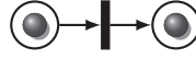
Figure 7.13: Empty transducers map to this Petri net instead of one like Figure 7.10.
