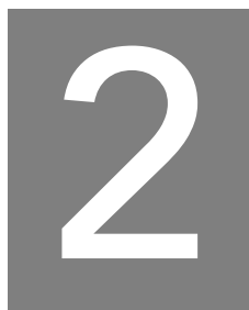
Figure 6.5. An illustration of a filter in a dense layer to detect letter “2.” The filter size is the same as that of the input. Consequently, the parameter space is significantly large. This is also referred to as a strong filter because it can alone detect the letter “2.” Although the filter is strong, the excess amount of parameters in it make a dense layer statistically inefficient. Due to statistical inefficiency, a dense layer would require a large number of samples to automatically learn a filter.
