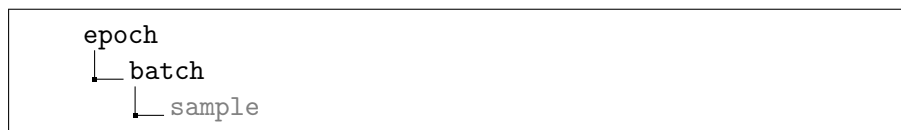
Figure 4.14. Levels of iteration in MLP training. The iterations are interpreted up to the sample level. However, computationally all samples in a batch are processed together using tensor operations. Hence, the sample is grayed here to indicate it is only a logical iteration level.
