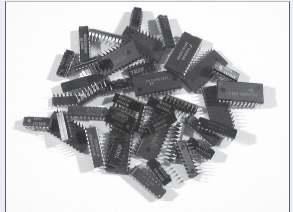
Photo of a group of classic TTL unit logic. Courtesy of Richard Jaeger
