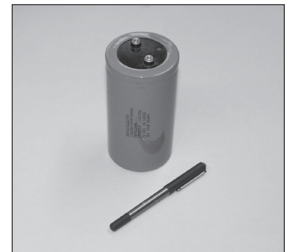
Figure 3.51 (a) Half-wave rectifier circuit with filter capacitor; (b) a-175,000- \mu\text{F} , 15-V filter capacitor. Capacitance tolerance is -10 percent, +75 percent.
