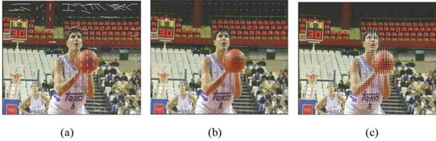
Fig. 5.9 Comparison of calculation results of block matching method and improved dense optical flow iterative algorithm
