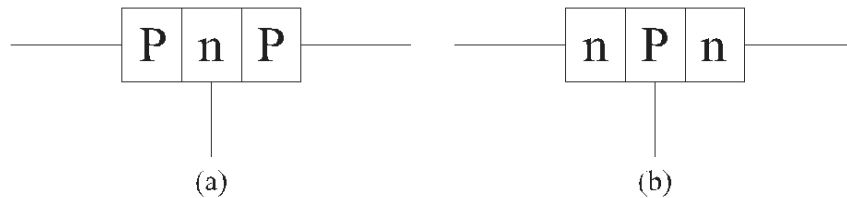
Figure 4-1. Composition of a (a) pnp and (b) npn transistor.
