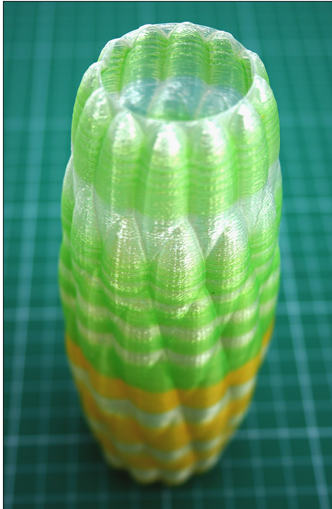
FIGURE 15-29: The hollow-pot 3D model printed as a Spiral Vase. The vertical Z axis never stops being raised slowly, resulting in a seamless print.
