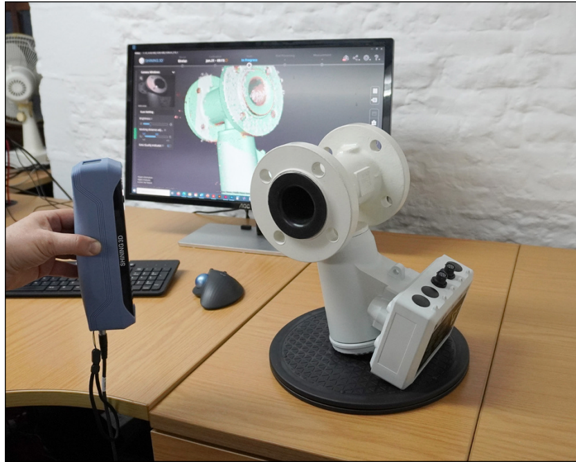
FIGURE 5-7: A handheld EinStar structured-light scanner being used to capture a water meter manifold to be used as a model for 3D printing.
