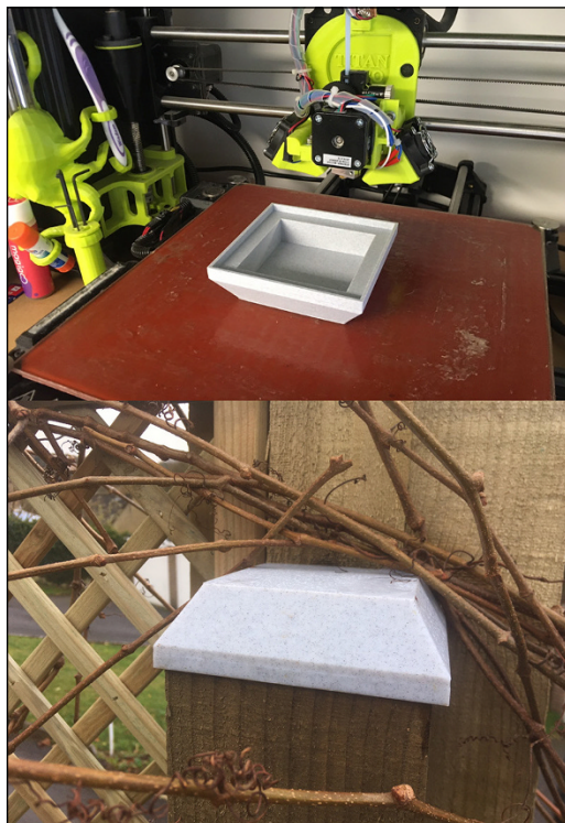
FIGURE 16-8: Custom size and shape end post caps printed in marble PLA will last for years.
