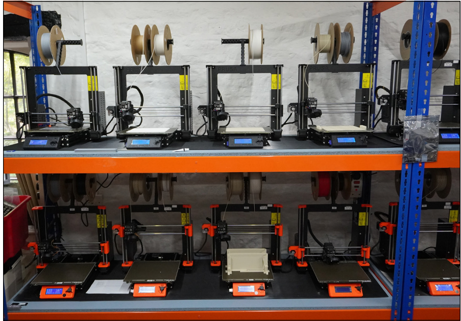
FIGURE 11-1: A simple small 3D print farm using many identical Prusa i3 MK3S+ machines that can share the same production files and produce identical parts.
