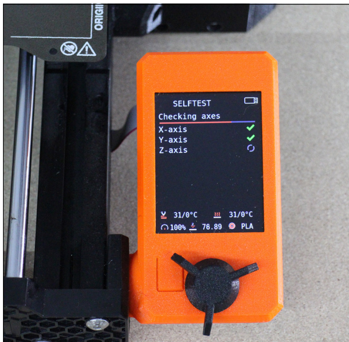
FIGURE 13-21: The firmware wizard will check axes movement including the end-stop position sensing.
