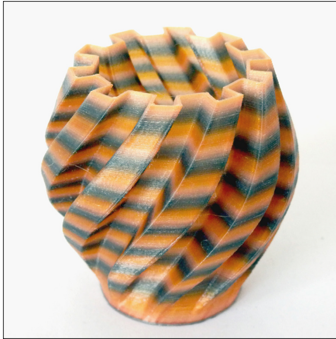
FIGURE 4-3: A dyed nylon 3D-printed object from Richard's experimentation with off-the-shelf clothing dyes.
