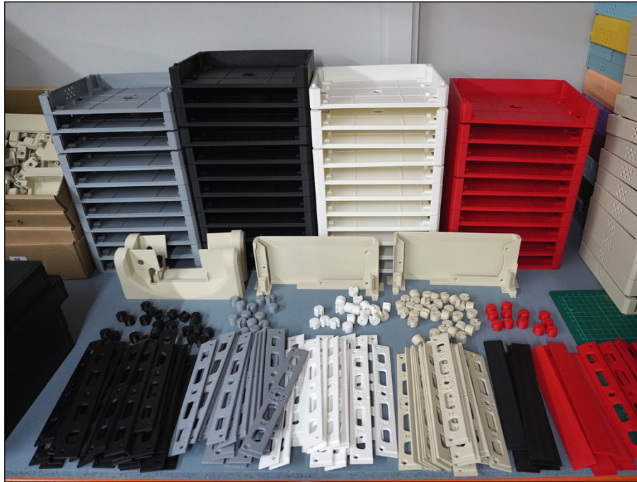
FIGURE 11-3: Range of 3D printer electronic enclosures consisting of multiple parts.
