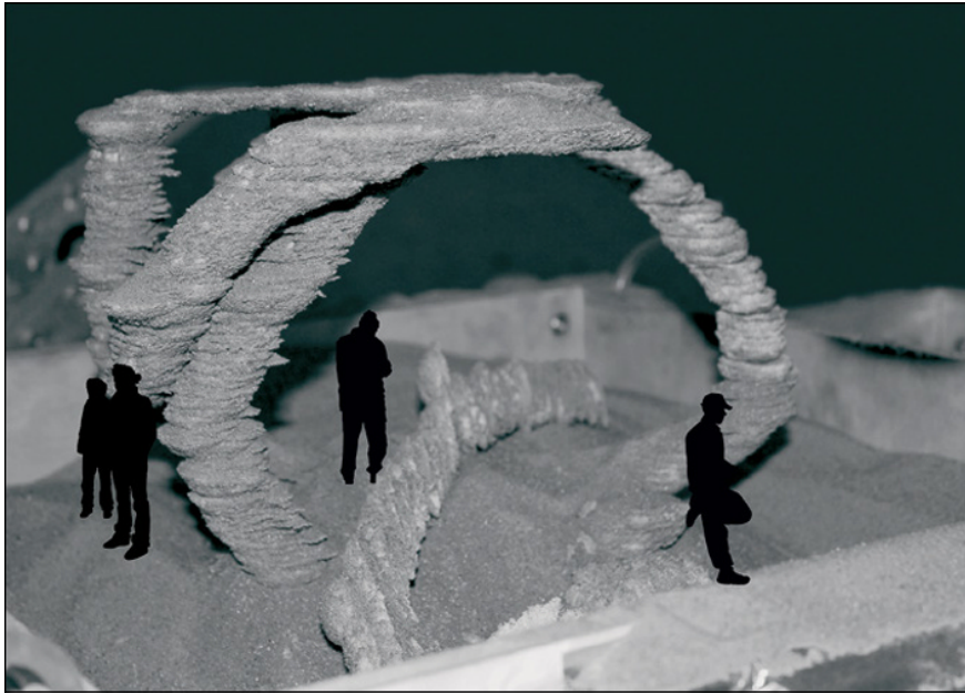
FIGURE 3-6: A structure created by using sunlight to fuse sand.
