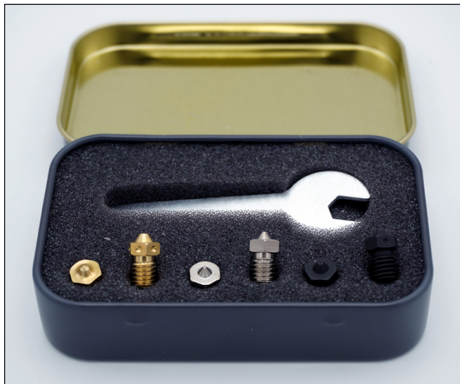
FIGURE 11-19: A range of V6 nozzles in different diameters from 0.2mm to 1.0mm and in brass, stainless steel, and hardened steel.
