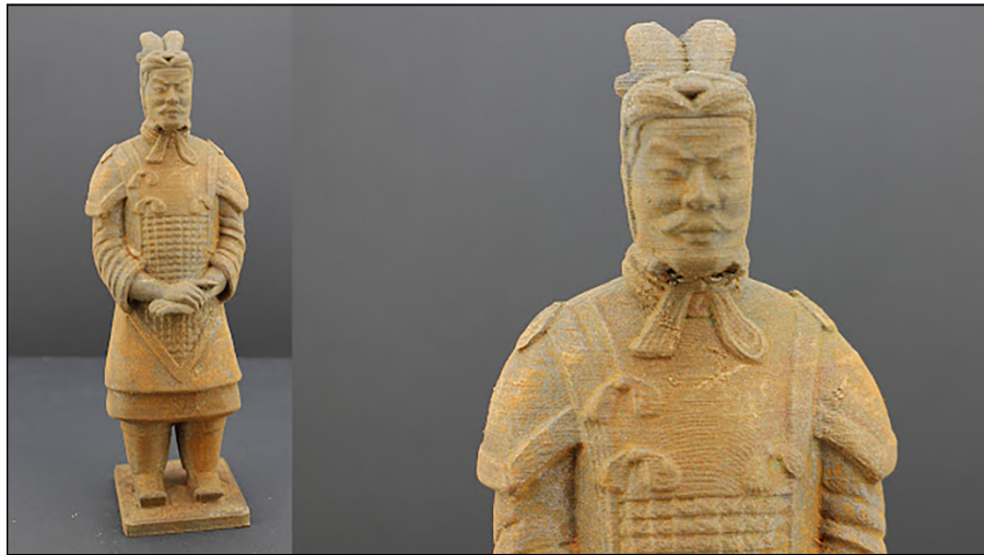
FIGURE 16-15: 3D print of a terracotta warrior in ProtoPasta magnetic iron being rusted.
