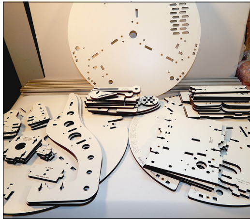
FIGURE 12-10: A highly precise jigsaw puzzle of wooden laser-cut sections forms the frame of the RostockMax 3D printer.
