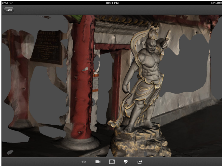
FIGURE 5-13: The full 3D model of the warrior statue before being cleaned up and made ready for 3D printing.
