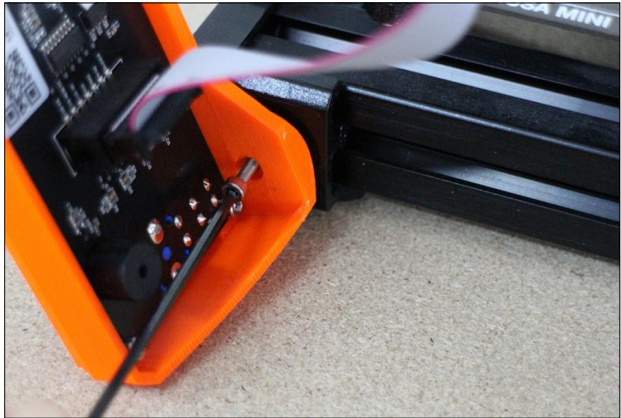
FIGURE 12-17: Fit the LCD screen and controls module using a single bolt; the screen can then be angled as required.
