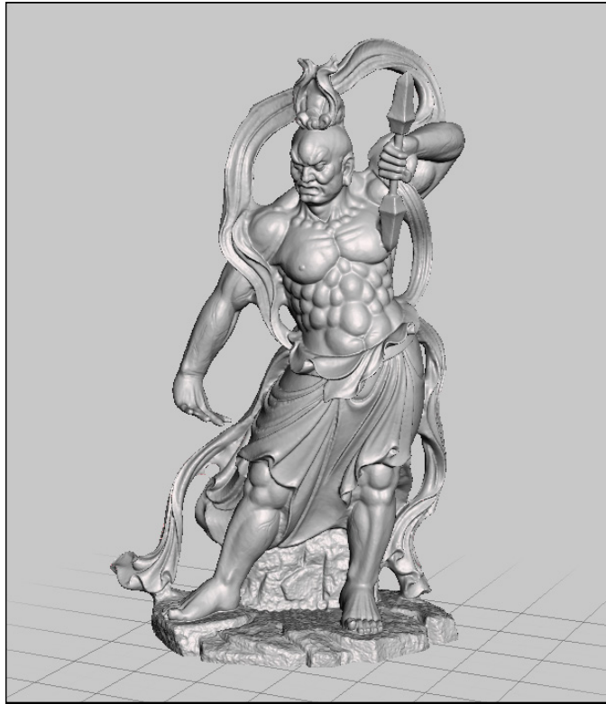
FIGURE 5-12: A 3D model created with photogrammetry and a series of photographs.
