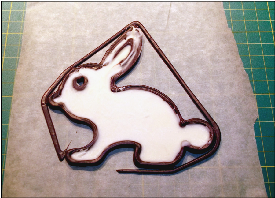
FIGURE 4-5: 3D-printed white-and-dark chocolate bunny, created with a RepRap 3D printer and Richard's Universal Paste Extruder.
