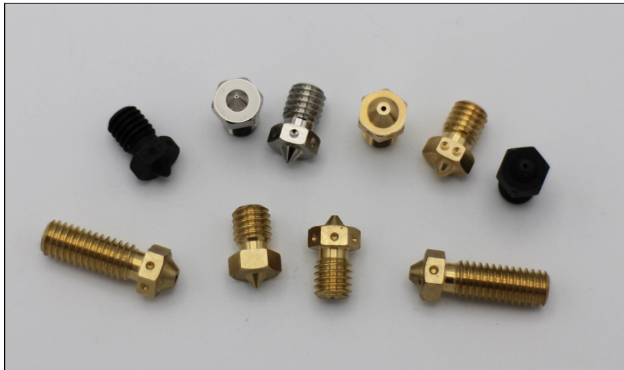
FIGURE 14-20: A selection of compatible E3D V6 and Volcano nozzles that can be fitted into the Prusa MINI or i3 MK2/3/4 3D printers.
