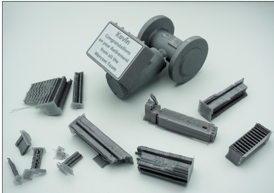
FIGURE 5-16: After printing, it's often necessary to remove support material from a model.
