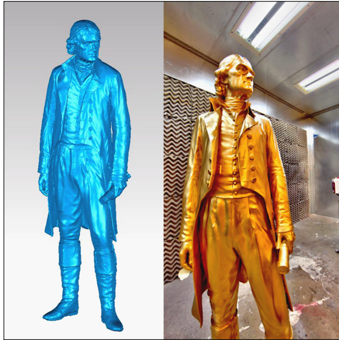
FIGURE 6-1: Digitization of a bronze statue of Thomas Jefferson and its full-scale reproduction.
