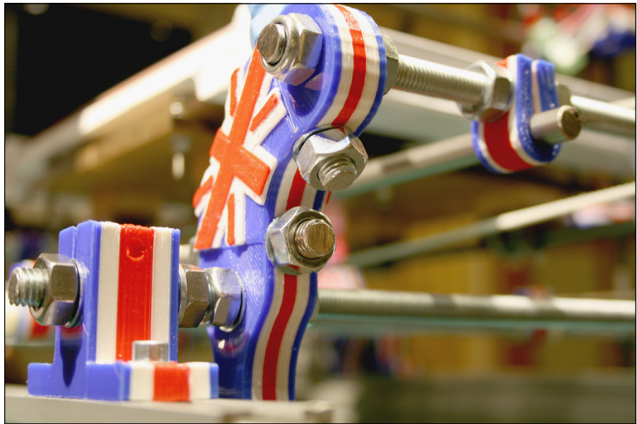
FIGURE 14-29: Layer-selective color printing with a single extruder involves using different layer heights.
