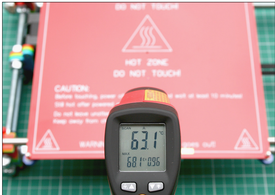
FIGURE 14-33: Use a noncontact laser temperature sensor to make sure that the parts of your 3D printer are running at the correct temperatures.
