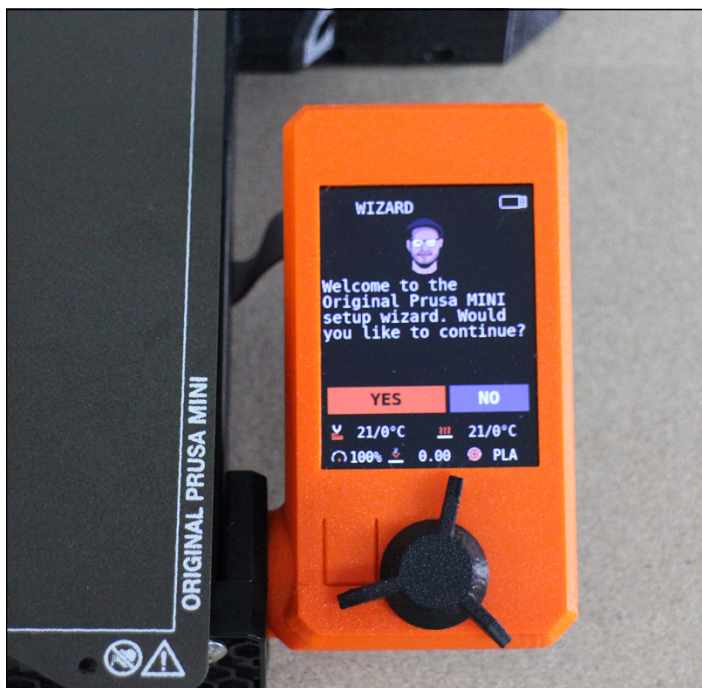
FIGURE 13-20: The first power on will guide you through a few setup options, and then the wizard will check whether the construction has been completed correctly.
