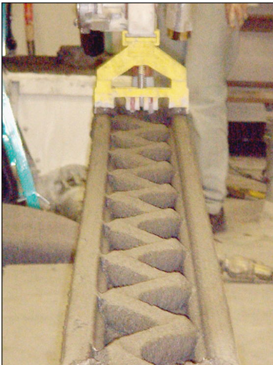
FIGURE 3-7: Corrugated wall made of 3D extruded concrete.
