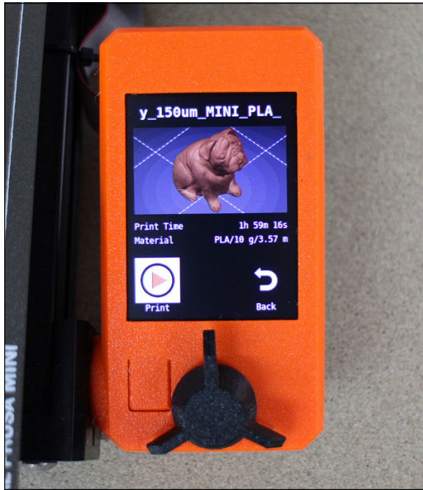
FIGURE 13-9: The Prusa MINI uses a 32-bit ARM Buddy board integrated motherboard and color LCD screen.
