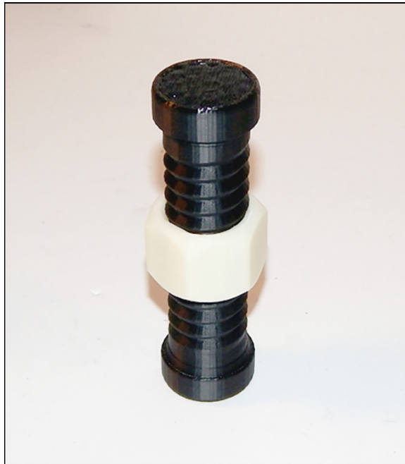
FIGURE 4-2: A 3D-printed puzzle for children includes a printed nut added to a dual-ended bolt paused during fabrication and then completed.
