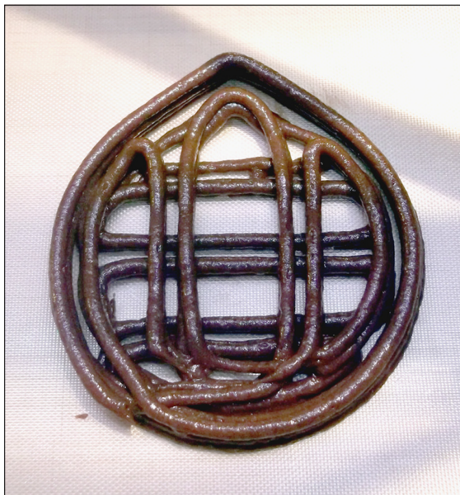
FIGURE 14-25: Printing chocolate muffin mix requires a basic syringe without a needle, which provides a 3mm bead of extrusion.
