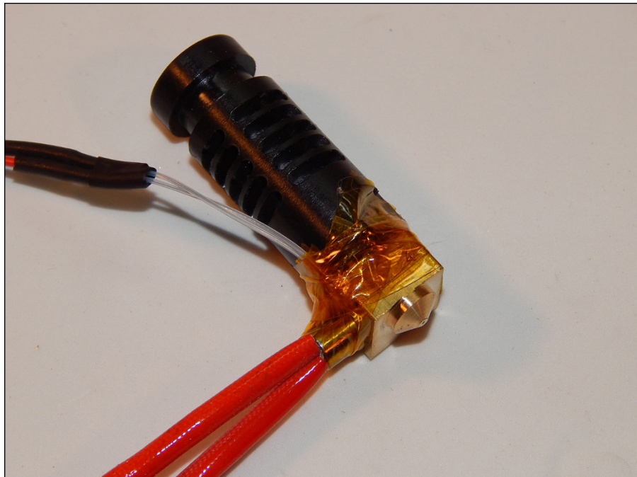
FIGURE 10-8: A standard J-head-style FFF/ FDM extruder hot-end.
