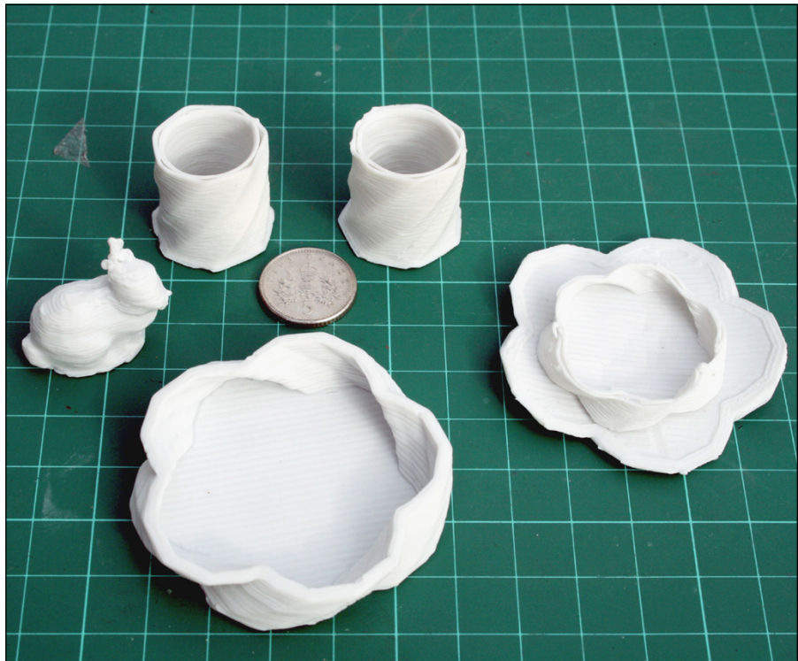
FIGURE 11-14: Fine porcelain clay can be printed with a paste extruder and then fired in a normal kiln to produce ceramic.
