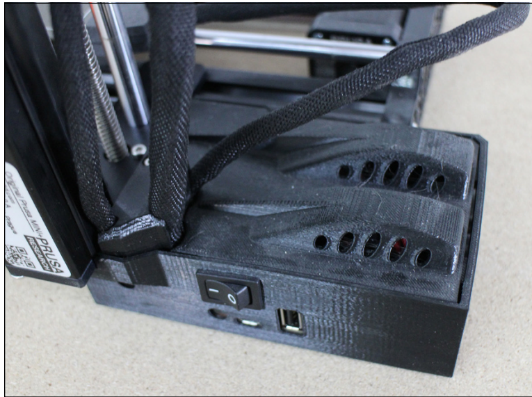
FIGURE 13-19: Fit the cover over the electronics, and you are ready to power on for the first time.
