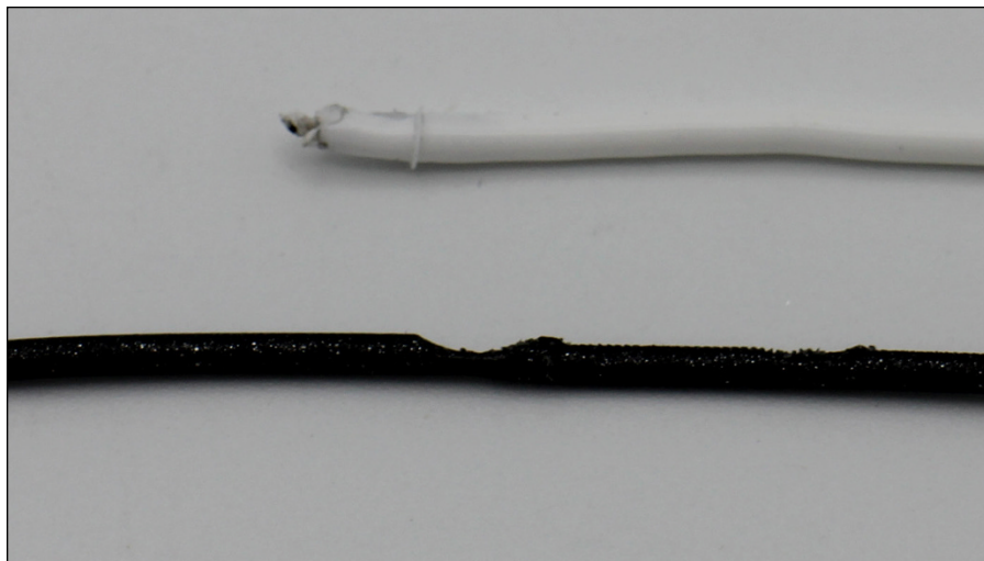
FIGURE 14-13: An extrusion system jam leaves your filaments damaged.
