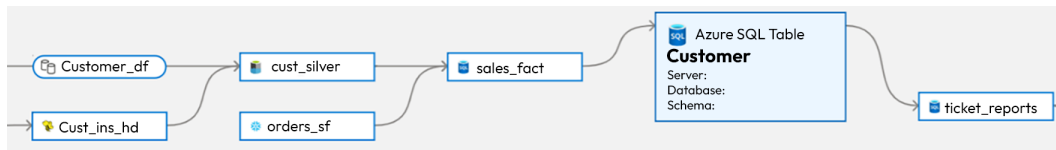
Figure 10.4 – An example of a data lineage in Microsoft Purview. We get a view of the upstream sources and downstream usage of data in the chosen data asset (in this case, a SQL table)
