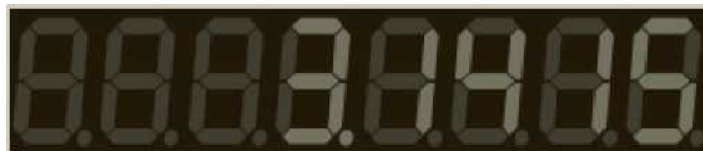
FIGURE 9.1 An eight-digit 7-segment display showing the number 3.1415.
