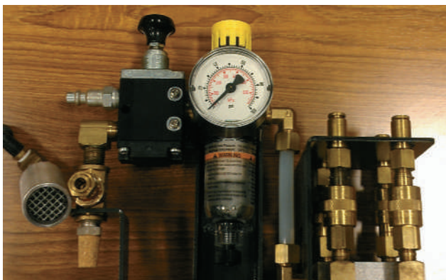
FIGURE 11-5 This pneumatic regulator does not have a lubricator, but it does have a filter bowl that needs to be drained and cleaned from time to time as well as a muffler that needs attention.
