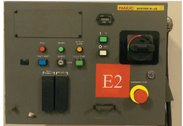
FIGURE 1-14 This FANUC control panel includes a big red E-stop on the lower-right side. It also has an on, off, cycle start, and fault reset button.
