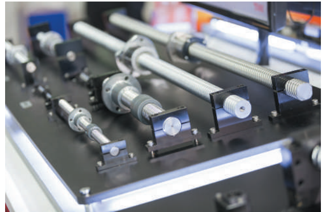
FIGURE 4-19 Some of the various sizes of ball screws that you might encounter in robotic applications.
