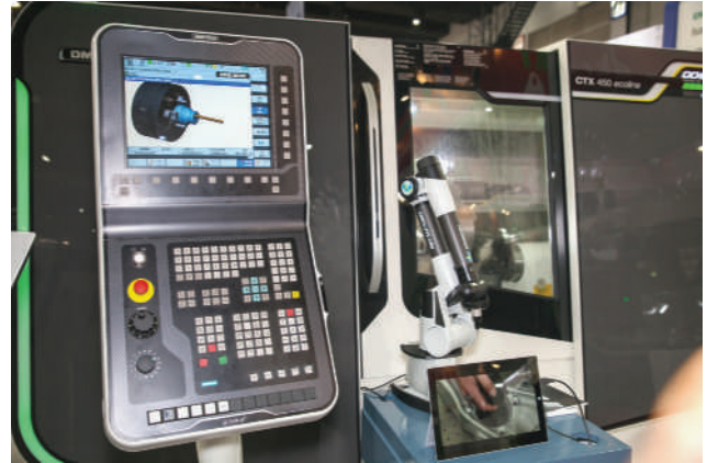
FIGURE 10-11 A CNC machine, being tended by a robot, and the controller for the system. A graphical representation of the machine appears on the screen, and the various buttons used for operator input appear below it. The buttons along the edge and bottom of the display screen are typically used to navigate to various menus and pages in the system.
