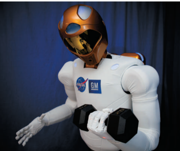
FIGURE 7-8 These two pictures demonstrate the principle behind tactile or force sensing. The astronaut shaking the Robonaut's hand would likely not have enjoyed the experience if the Robonaut had used the same amount of force as it did lifting the 20-lb dumbbell.
