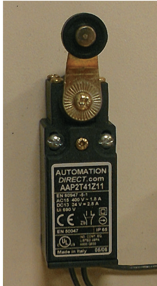
FIGURE 7-2 An Automation Direct limit switch with a much smaller arm and a wheel on the arm to help reduce the connection impact. This type of switch would work well with a door or other movable guarding.
