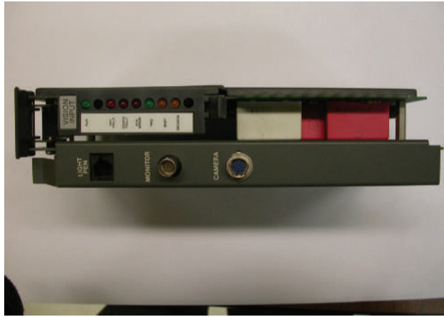
FIGURE 8-1 An example of a machine vision process board—one of the great advancements of the 1980s.
