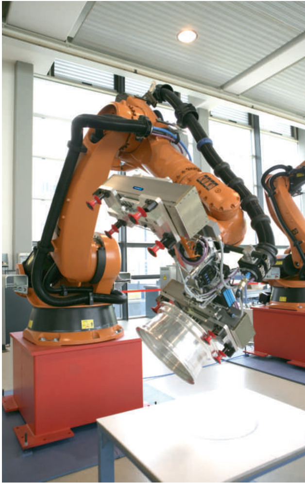
FIGURE 5-6 A four-finger system centering a tire rim.
