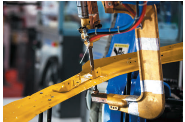
FIGURE 5-17 A spot-welding process welding the frame of a vehicle together.
