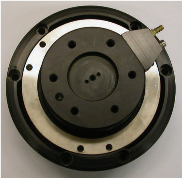
FIGURE 5-30 This active compliance device is mounted between the tooling and the robot to detect issues. Inside there are strain gauges or other such sensors that detect when something is amiss.
