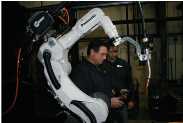
FIGURE 1-4 Here you can see a couple of operators in the danger zone working on the program with teach pendant in hand.
