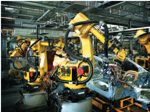
FIGURE 5-19 The X-type spot-welding gun. The primary difference between it and the C style is that both jaws move on the X type.
