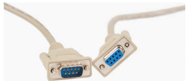
FIGURE 9-9 A male and female DB9, which is a common RS232 cable.
