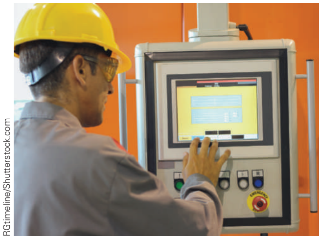
FIGURE 10-15 An operator interacting with a touch screen. Notice that there are only a few buttons and an E-stop under the screen.
