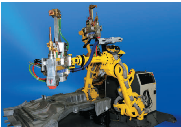
FIGURE 11-10 While this robot is not small by any means, take a moment to look at the tooling it uses during operation. Now imagine trying to hold on to this tooling while simultaneously removing the bolts holding it in place. In situations like this, you definitely need help from your coworkers.
