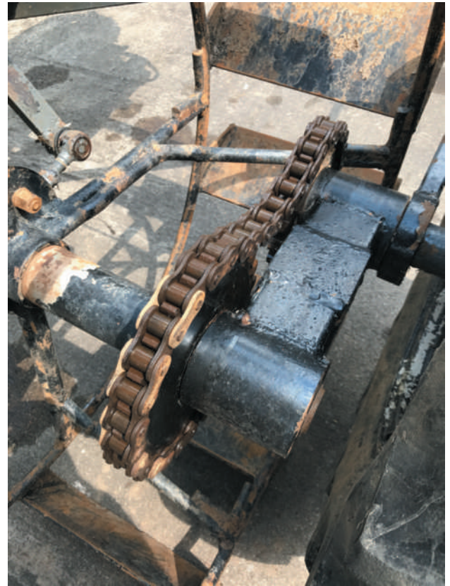
FIGURE 4-14 While this system is not from a robot, it does show the components of a chain system as well as the slack that develops over time.
