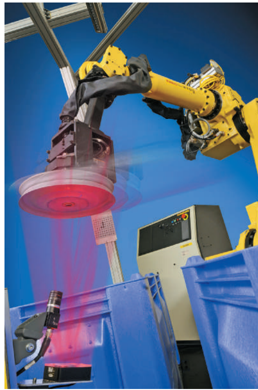
FIGURE 5-24 A robotic system using special lighting and a camera to check the quality and features of a part.
