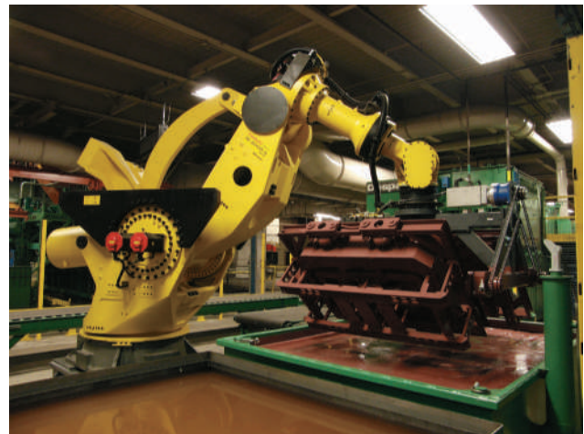
FIGURE 3-10 A FANUC electrical robot moving a large assembly, a job that in years past was reserved for hydraulically powered robots.
