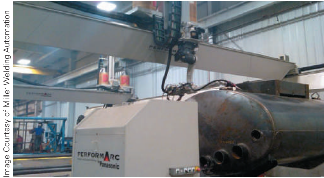
FIGURE 3-19 Panasonic has mounted one of its welding robot arms to a gantry base, combining the large area of the gantry style with the flexibility of a six-axis arm. This creates a “best of both worlds” kind of system.
