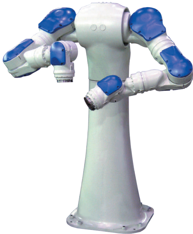
FIGURE 2-12 This photo depicts one of Yaskawa Motoman’s dual-arm robotic systems. Some companies place something on top of the central torso to make the robot look more like a person and usually add camera vision, but either way they get the job done.
