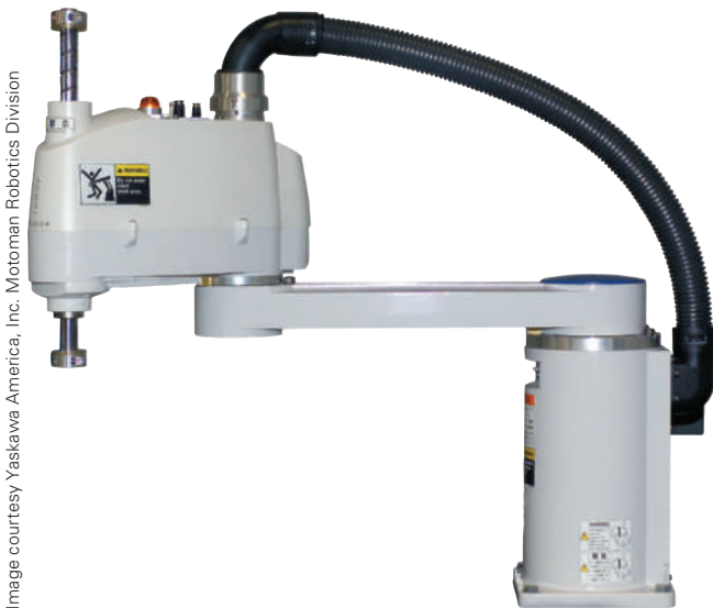
FIGURE 2-6 This photo depicts one of Motoman's SCARA-type robots. The popularity of this design led several robotics companies to invest in and create this type of robot.
