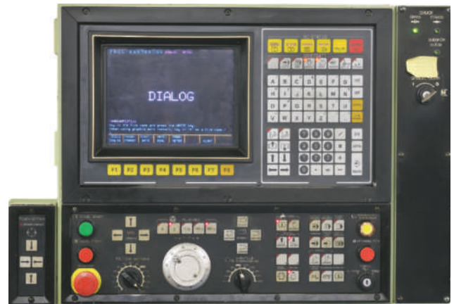
FIGURE 10-12 An older-style CNC controller. Older CRT technology is used for the display, and fewer input buttons are available for this system.
