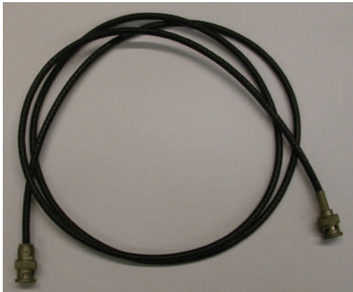
FIGURE 9-7 A coaxial cable. You may have a similar cable bringing satellite or cable TV services into your TV.
