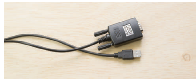
FIGURE 9-12 A USB to DB9 adaptor that you may find in industry. Most of the time this type of adaptor comes with an install disk that has the needed software on it.
