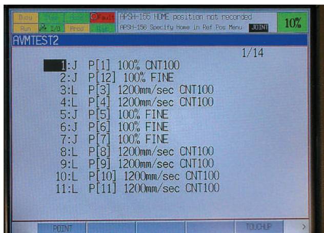
FIGURE 6-3 A level 4 program on the FANUC controller written in my robotics class. In this program, linear and joint movements are used between the various points.
