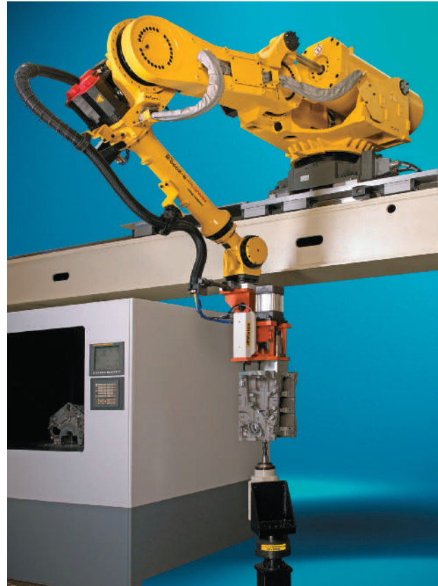
FIGURE 2-18 A FANUC robot bores out an engine body it pulled from the machine with a stand-alone tooling base. Often this type of tooling is tied to the robot controller and controlled in the robot program, along with all the positioning necessary.
