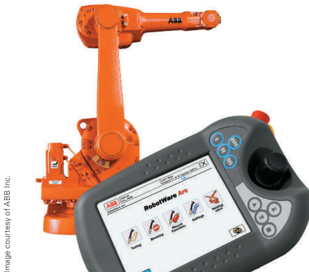
FIGURE 3-14 The teach pendant for an ABB robot. Notice the red E-stop on the upper-right corner.
