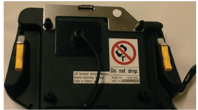
FIGURE 3-15 The two yellow switches pictured here are the dead man's switches for a Panasonic robot's teach pendant. It does not matter which one is depressed, but at least one has to be depressed at all times to allow manual movement of the robot.
