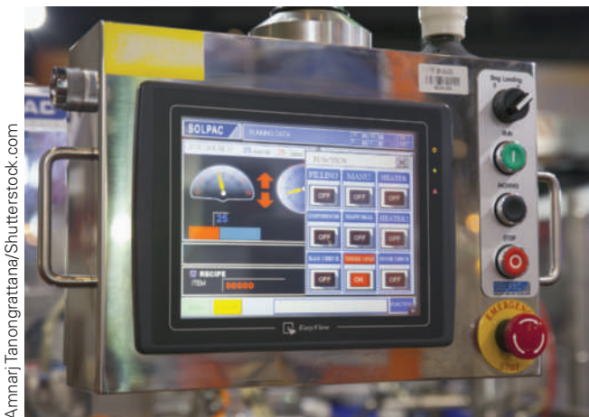
FIGURE 10-14 A few buttons are found on this control, but most of the operations are controlled by the HMI in the middle. Notice the gauges and on/off buttons on the screen.
