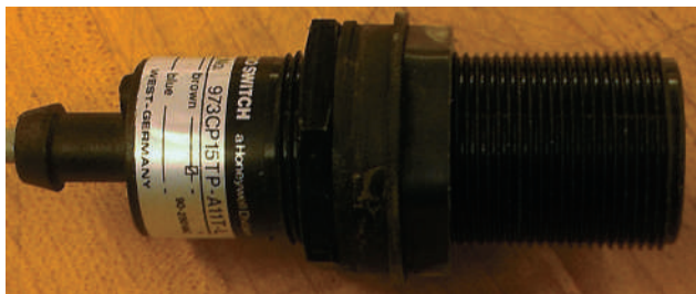
FIGURE 7-6 A capacitive prox switch. Notice how the body is plastic, rather than metal. It is common to find inductive prox switches with metal bodies and capacitive prox switches with plastic bodies, but do not assume that all metal prox switches are inductive or that all plastic prox switches are capacitive.
