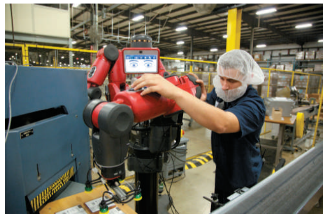
FIGURE 2-7 Rethink Robotics led the collaborative robots charge in 2012 with the release of the Baxter robot. Here you can see Baxter working to help someone in industry.
