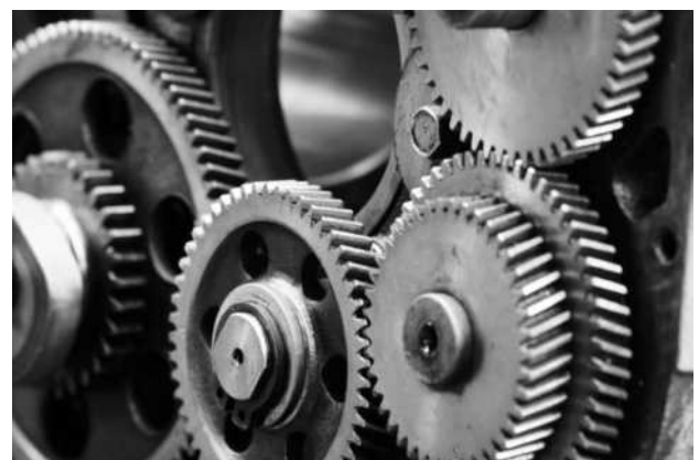
FIGURE 4-17 Part of a gear transmission system, which includes compound gears.
