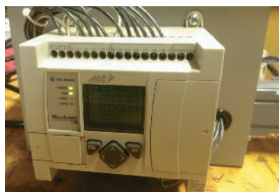
FIGURE 10-4 (left) A MicroLogix 1100. (middle) An SLC system. (right) A ControlLogix system.
