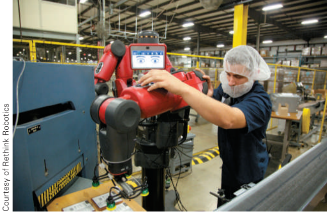
FIGURE 1-8 Baxter operates in an industrial setting without any cage around it. This kind of machine is leading the charge to free the industrial robot from confinement.
