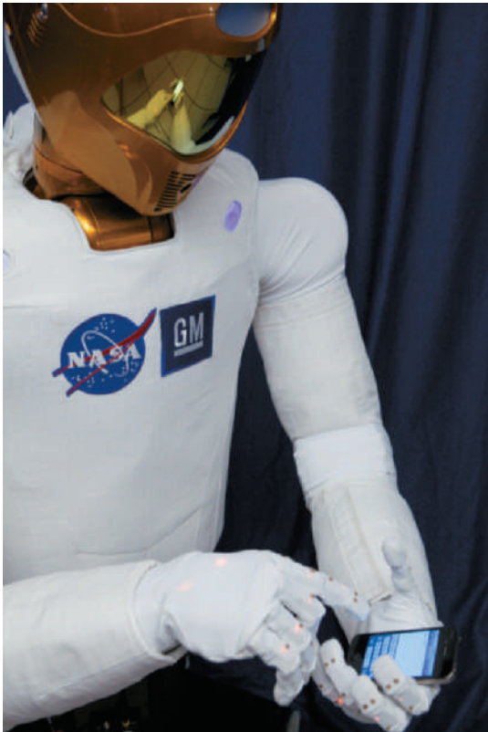
FIGURE 5-1 The Robonaut, created through a partnership between NASA and GM, utilizes an advanced hand-style gripper that allows the robot to perform tasks in a very human manner.
