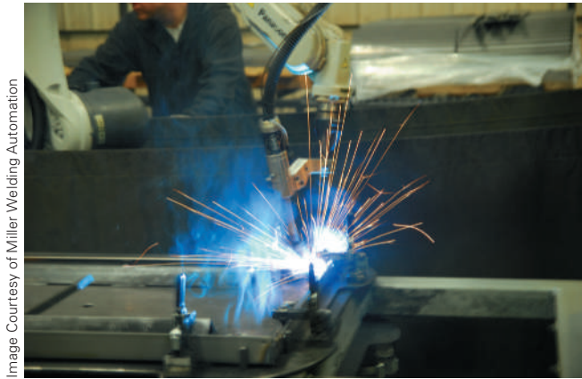
FIGURE 6-20 In these two pictures, you can see the types of movements that often require a rapid move in manual mode. Switching the orientation of the tooling in such a radical manner over a small distance usually requires a rapid movement with a break in the welding, which can be detrimental to weld quality.
