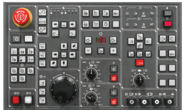
FIGURE 10-13 A close up of the various input buttons you may find on a CNC controller. The pictures on the buttons are intended to help the operator determine what the button influences.
