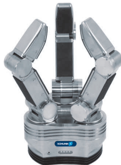
FIGURE 5-4 A set of angular grippers that have an extra joint on each finger to make them more like human fingers.
