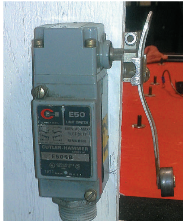
FIGURE 7-1 A Cutler-Hammer limit switch with the arm mounted for contact on the right side of the unit.
