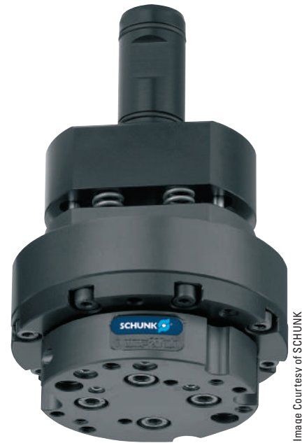
FIGURE 5-28 Notice the springs between the tooling base and where the base attaches into the tooling holder on the robot. This arrangement allows for some side-to-side motion of the tooling without incident.
