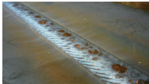
FIGURE 6-8 This example shows what a weave weld can do. Notice how wide the weld path is and the wavy patter it creates.
