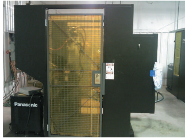
FIGURE 12-5 The Panasonic-Miller welding robot PA55 has an initial cost of approximately $55,000.
