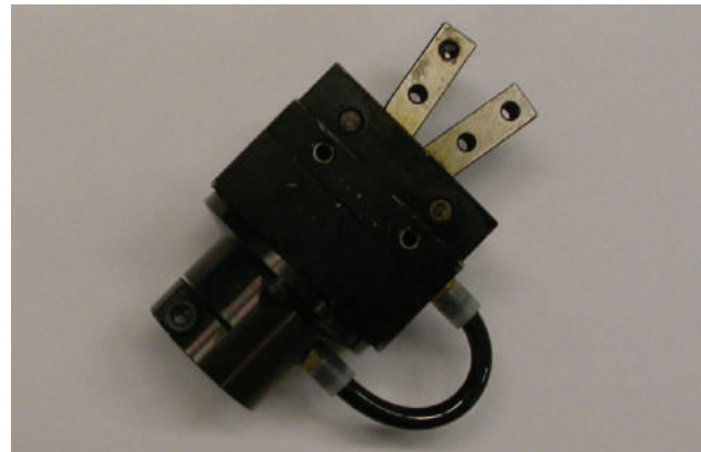
FIGURE 5-3 A simple angular set of grippers that create a scissors-type motion.
