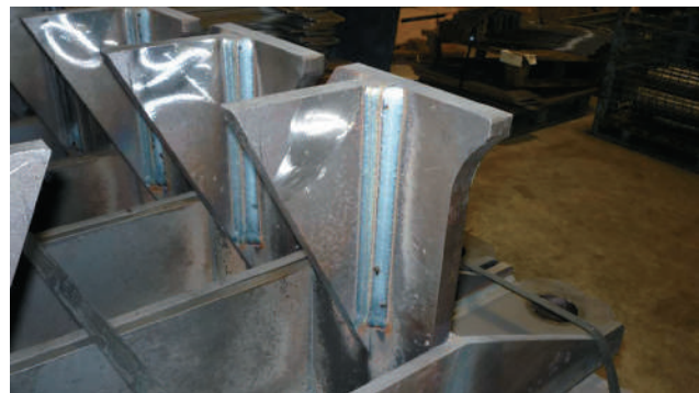
FIGURE 6-5 This part has multiple welds laid on top of one another to create the strength required. Without proper planning, these welds could look fine but actually have imperfections and other flaws that would reduce their structural strength.
