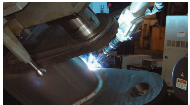
FIGURE 12-7 Welding thick metals (also called heavy plate) requires a great amount of skill and experience when done by hand. When we program a robot to perform welding, we give operators who are new to heavy plate the chance to make parts with quality welds while they learn all the specifics of this type of welding.
