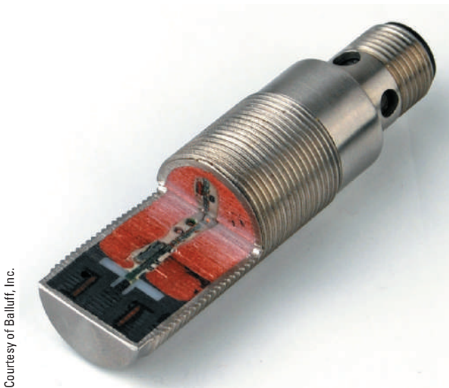
FIGURE 7-4 A cutaway of a prox switch, showing both the internal solid-state components (surrounded by the red resin) and the coil in the tip (surrounded by the black resin). The coil is the copper color in the black resin.
