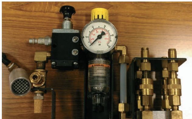
FIGURE 3-9 On the left side are two mufflers: The gold cone is the muffler for the pressure regulation unit pictured, and the silver cylinder is a muffler for use where needed. To control the air pressure to the system, the yellow knob on top of the pressure gauge (center) is used. The brass connections on the right are points where air is supplied to the system.
