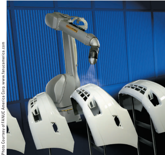
FIGURE 5-21 A paint-spraying robot working on bumpers.
