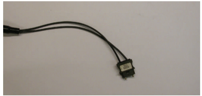
FIGURE 9-6 A fiber-optic cable. If you shine a light on one end, you can see the light through the pins on the other end if the cable is undamaged.
