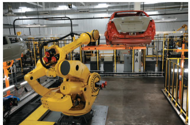
FIGURE 2-5 FANUC's larger robots can handle a car body with ease.
