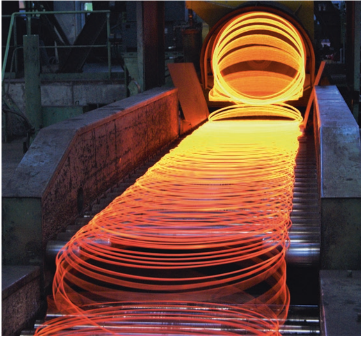
Fig. 5.34 Wire with a diameter of 5 mm directly at the outlet of a continuous rolling mill. (Photo: Schlegel, J., BGH Edelstahl Freital GmbH)
