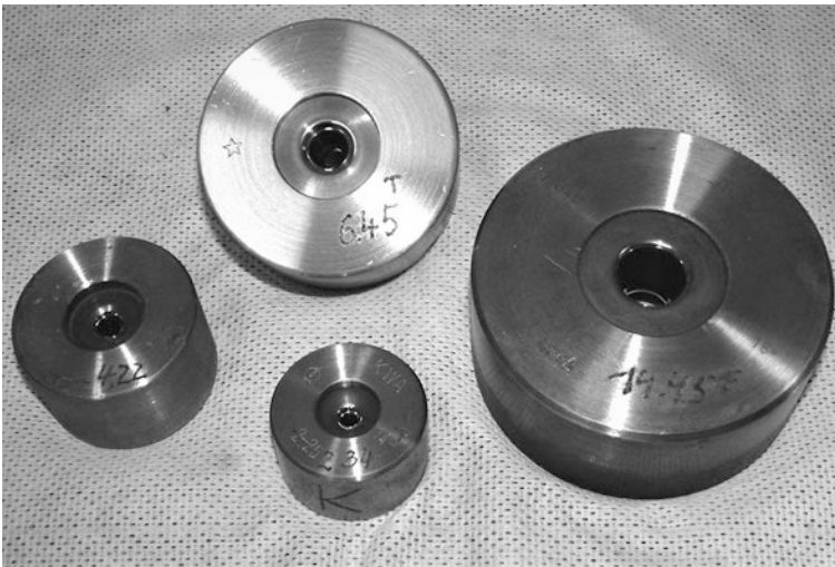
Fig. 5.62 Tungsten carbide drawing dies with different diameters for the dry drawing of steel wire. (Photo: Schlegel, J., BGH Edelstahl Lugau GmbH)
