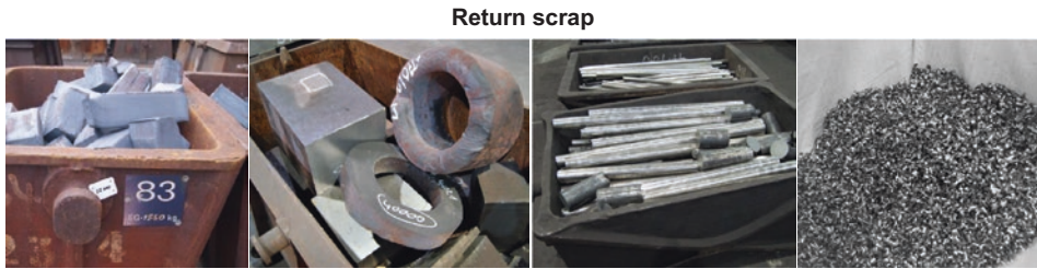
Fig. 10.5 Examples of return scrap, from left to right : hot-rolled ends of billets, sawed-off parts of forged square and hollow profiles, cut-to-length peeled bars, chips from turning. (Photos: Schlegel, J. BGH Edelstahl Freital GmbH)
