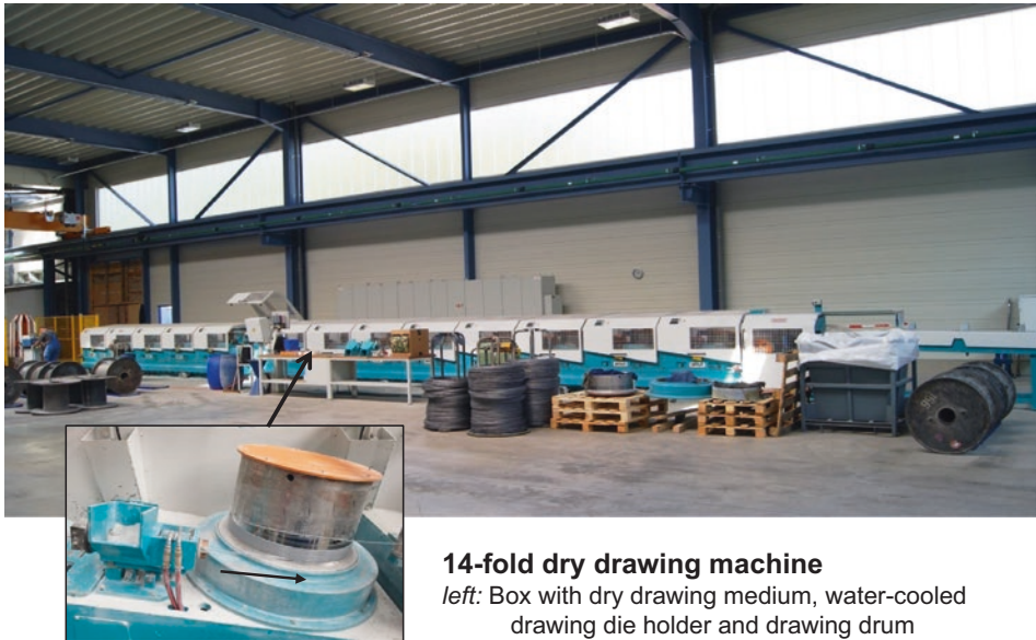
Fig. 5.72 Multi dry drawing machine with 14 draws and spooler. (Photo: Schlegel, J., BGH Edelstahl Lugau GmbH)
