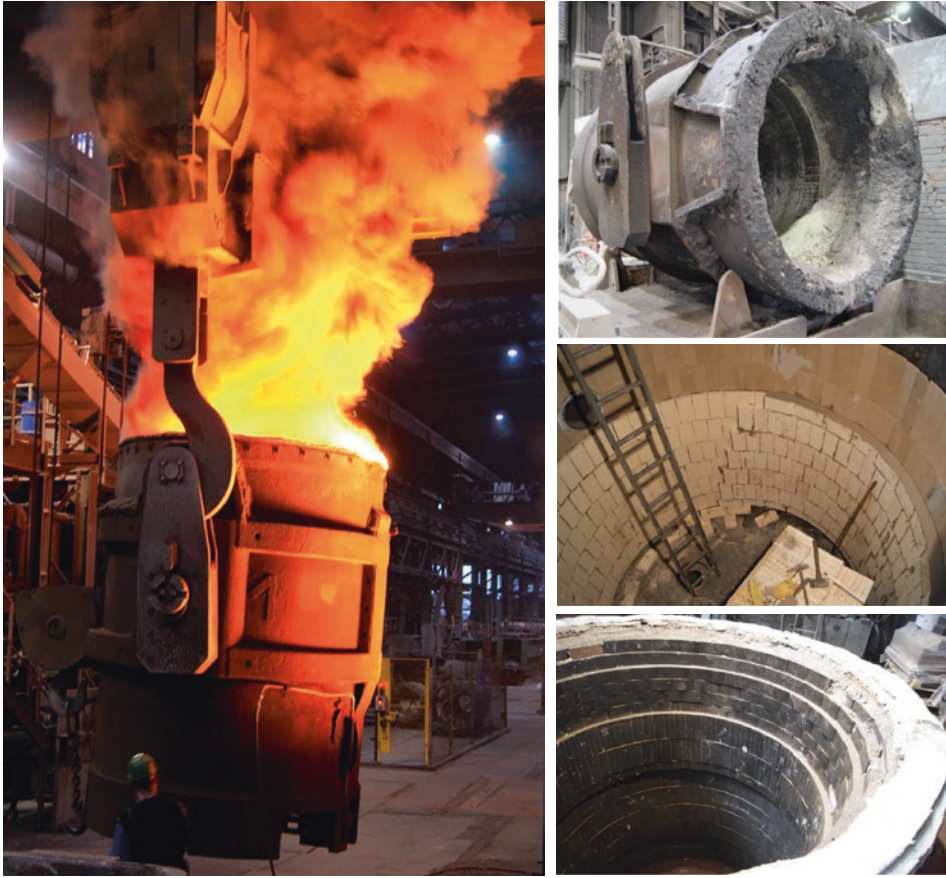
Fig. 10.12 Steel casting ladle, melt charge size approx. 42 t, left : in use for transporting raw steel to the ladle metallurgical (fine treatment) plant, right from top to bottom : lining worn out, new lining installation and finished ladle. (Photos: Schlegel, J., BGH Edelstahl Freital GmbH)
