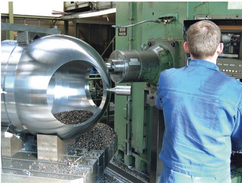
Fig. 8.30 Milling of a spherical piece on a CNC milling machine. (Photo: Schlegel, J., BGH Edelstahl Siegen GmbH)
