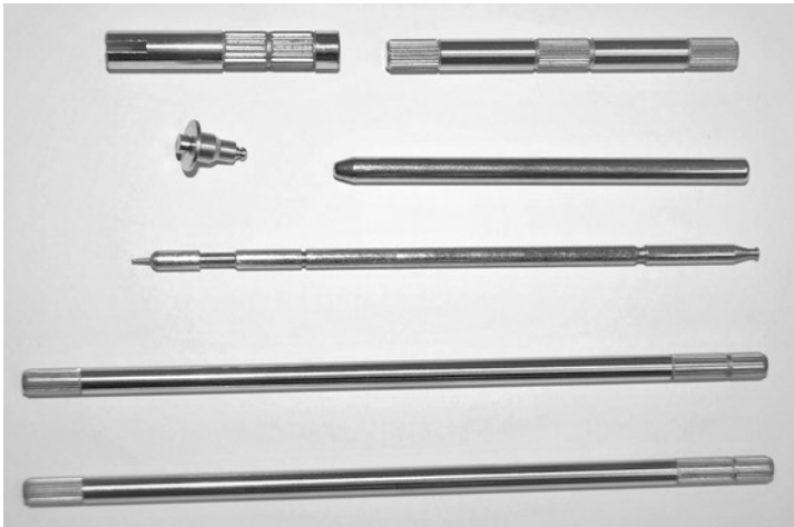
Fig. 2.40 Examples of precision turned parts made of automation steel. (Photo: Rödel, C., BGH Edelstahl Lugau GmbH)
