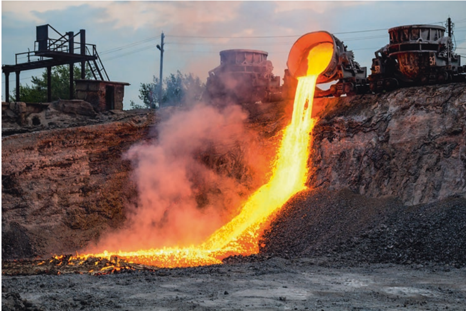
Fig. 10.8 Discharge of blast furnace slag into a slag pit for a slow cooling. (Photo from the Internet)
