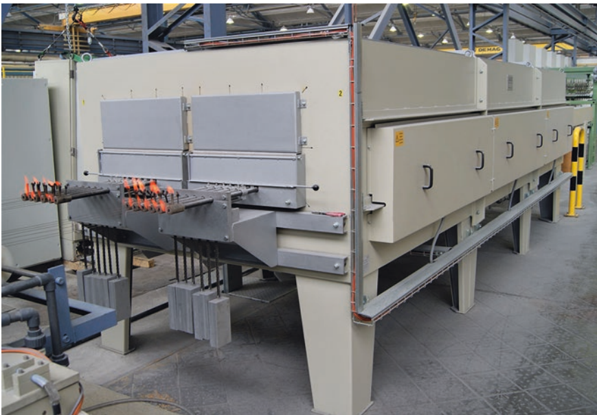
Fig. 6.17 Wire pull-through type furnace for the recrystallization and solution annealing of drawn wire. (Photo: Schlegel, J., BGH Edelstahl Lugau GmbH)
