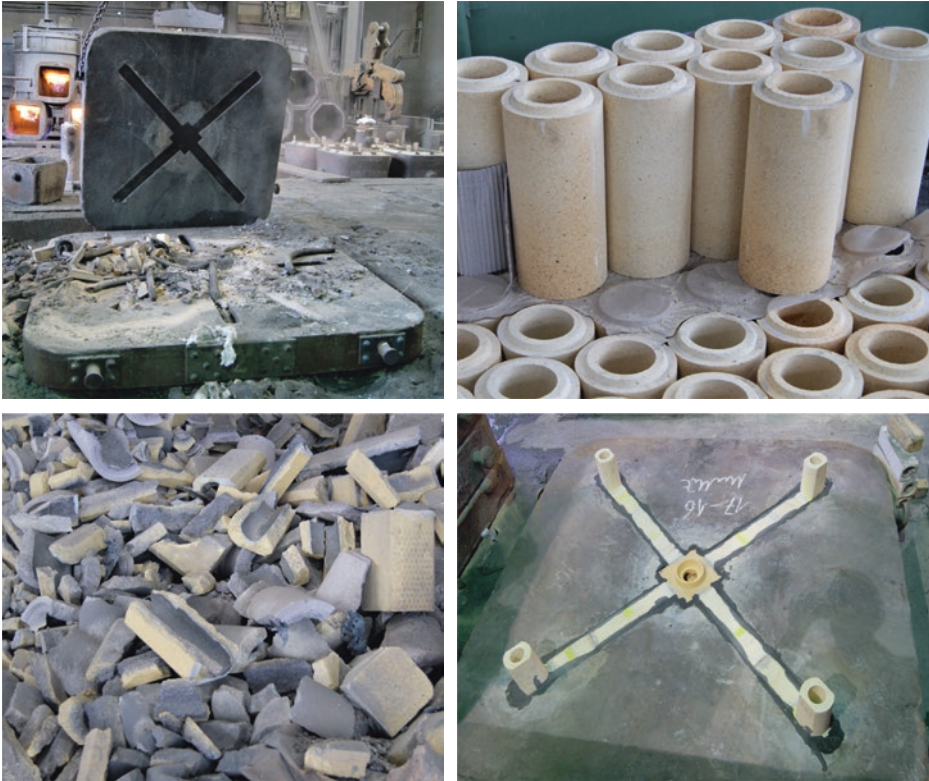
Fig. 10.11 Refractory material breakout after ingot casting and new lining of the mold frame with tubular refractory bricks. (Photos: Schlegel, J., BGH Edelstahl Siegen GmbH)
