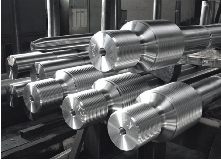
Fig. 2.32 Tie rods for automobile presses. (Photo: Schlegel, J., BGH Edelstahl Siegen GmbH)
