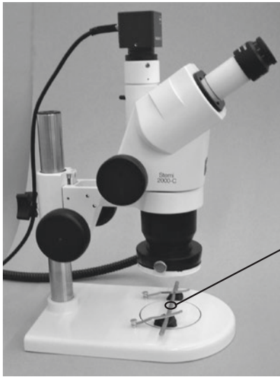
Fig. 7.24 Classic reflected light stereomicroscope with a recording of a surface section of a coated bar made of 1.4718 - X45CrSi9-3. (Photos: BGH Edelstahl Lugau GmbH)
