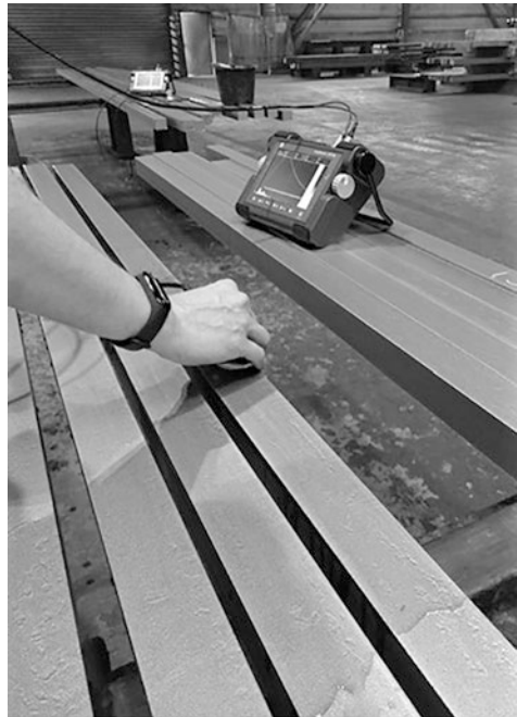
Fig. 7.27 Principle of the US testing according to the pulse-echo method. (Photos: Schlegel, J., BGH Edelstahl Lugau GmbH)
