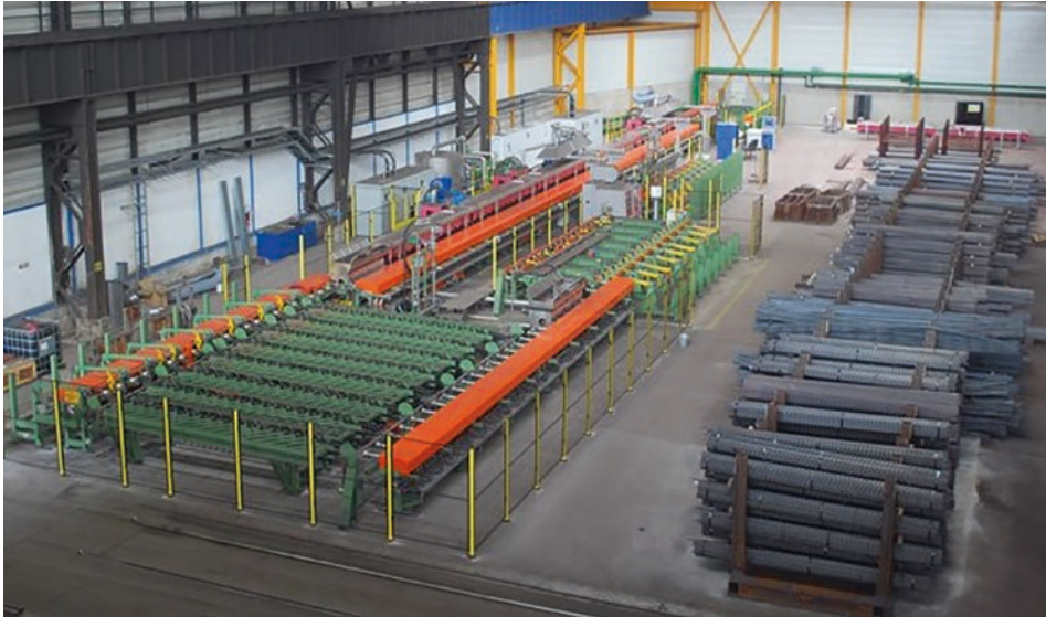
Fig. 6.18 Induction single-rod annealing plant for rolled bars. (Photo: Kopsch, St., BGH Edelstahl Freital GmbH)
