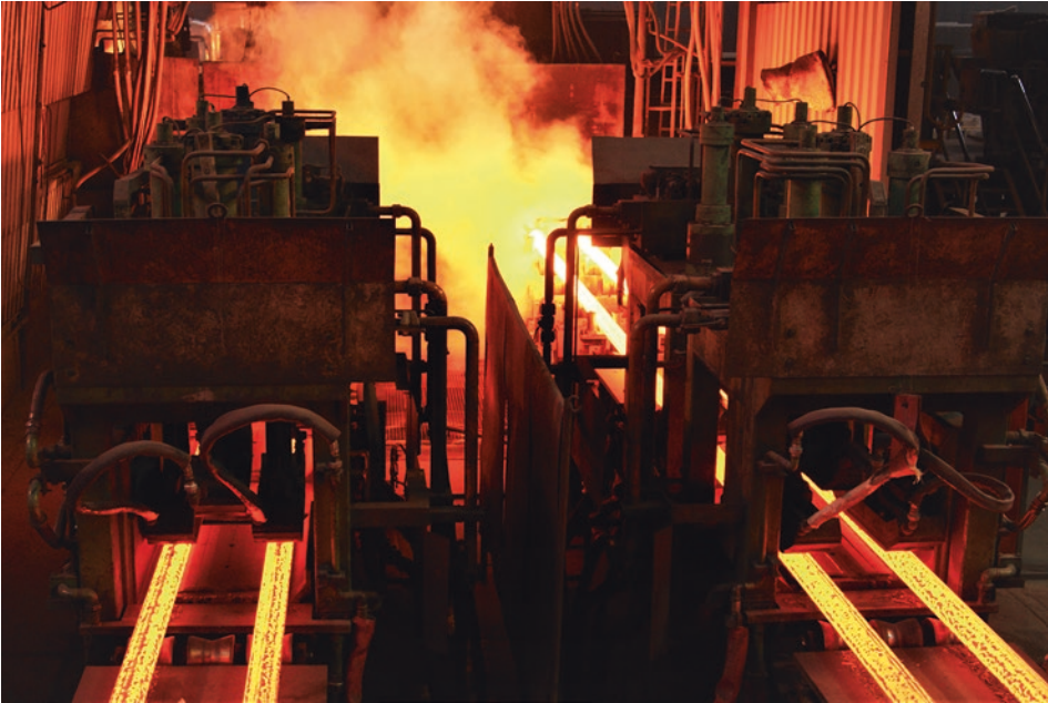
Fig. 4.35 View of a horizontal continuous casting plant, strand exit to the front. (Photo: Schlegel, J., BGH Edelstahl Freital GmbH)
