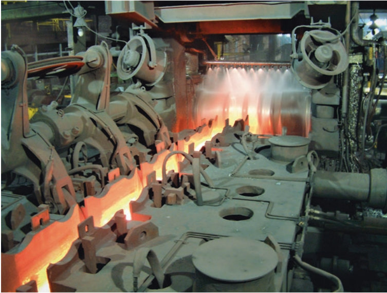
Fig. 5.30 Duo reversing blooming mill with box pass. (Photo: Schlegel, J., BGH Edelstahl Freital GmbH)
