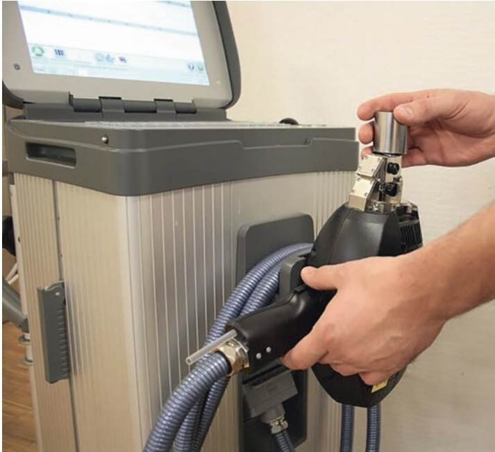
Fig. 7.20 Spark spectrometer for rapid analysis in a laboratory of a university. (Photo: Kurdewan, T., DHBW Stuttgart)
