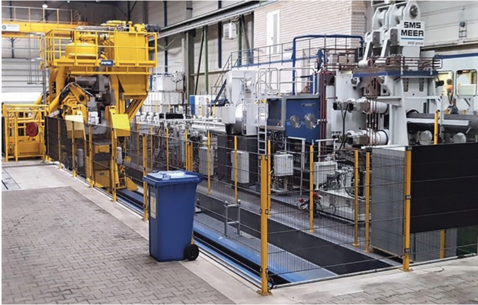
Fig. 8.33 Modern bar peeling machine for long-forged bars in the diameter range 160 to 610 mm. (Photo: BGH Edelstahl Siegen GmbH)
