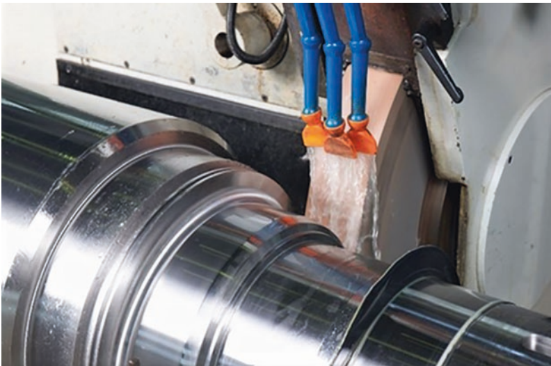
Fig. 8.39 Grinding a bearing journal of a cold rolling mill on a universal cylindrical grinding machine. (Photo: Jeibmann, J., Photographik, Dresden)
