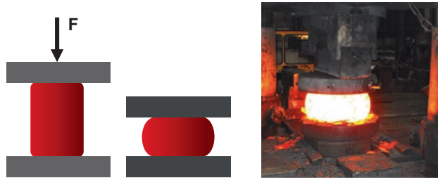
Fig. 5.7 Upsetting process in practice. (Photo: Schlegel, J., BGH Edelstahl Lippendorf GmbH)
