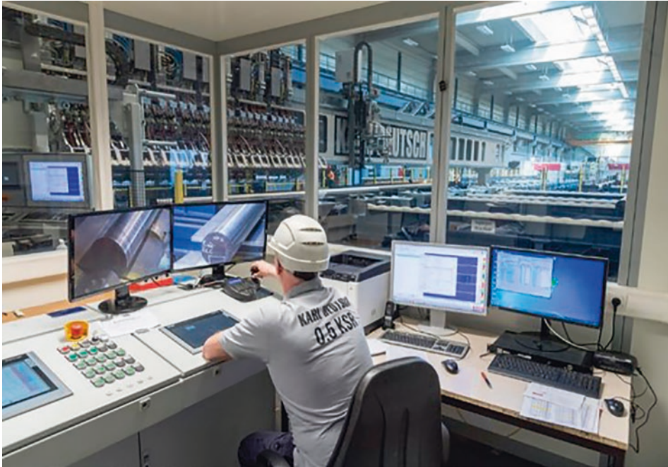
Fig. 7.30 Control panel of a fully-automatic US continuous passage testing facility for forged and peeled semi-finished products with a diameter of 100 to 400 mm. (Photo: BGH Edelmetall Siegen GmbH)
