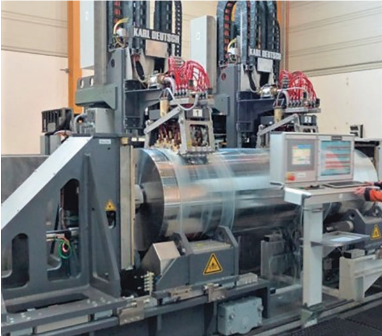
Fig. 7.29 Fully automated ultrasonic inspection system for round bars \varnothing 300 to 1000 mm. (Photo: BGH Edelstahl Siegen GmbH)
