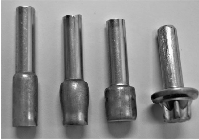
Fig. 5.19 4 stages of cold flow pressing of a screw blank. (Photos: Schlegel, J.)
