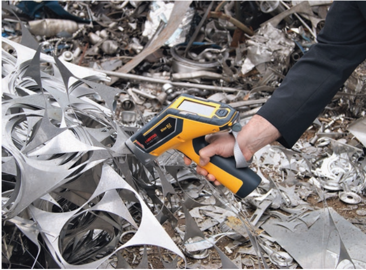
Fig. 10.4 Mobile XRF device in use for the quick detection of the chemical analysis of steel scrap. (Photo: Schlegel, J., BGH Edelstahl Siegen GmbH)
