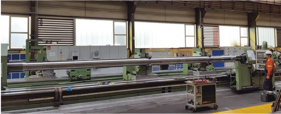
Fig. 8.26 CNC long-turning machine for parts up to 18 m in length and with diameters up to 1440 mm. (Photo: Schlegel, J., BGH Edelstahl Siegen GmbH)
