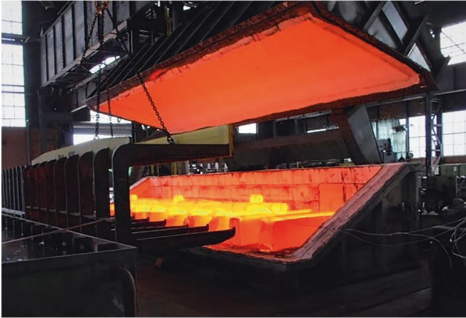
Fig. 6.15 Hood type annealing furnace for forged semi-products. (Photo: Kopsch, St., BGH Edelstahl Freital GmbH)
