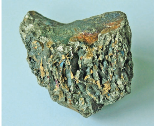
Fig. 3.34 Ferro-manganese. (Photo: Schlegel, J., BGH Edelstahl Freital GmbH)
