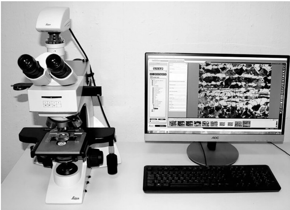
Fig. 7.25 Bright-field microscope with computer-aided image analysis in a research laboratory. (Photo: Kurdewan, T., DHBW Stuttgart)
