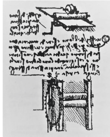
Fig. 5.29 Leonardo da Vinci and his designs for two hand-driven sheet metal rolling mills, drawing from 1495. (From the Internet: Feldhaus, 1913, p. 55)
