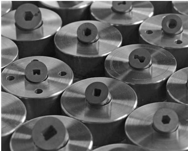
Fig. 5.75 Examples of drawing dies profiles for drawing bars from steel. (Photo: EZM Edelstahl-zieherei Mark GmbH, Wetter)
