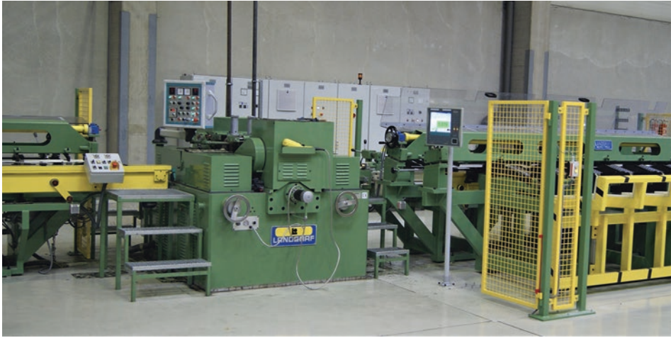
Fig. 8.38 Centerless continuous working through-feed grinding machine in a grinding line for bar diameters of 5 to 10 mm. (Photo: Schlegel, J., BGH Edelstahl Lugau GmbH)
