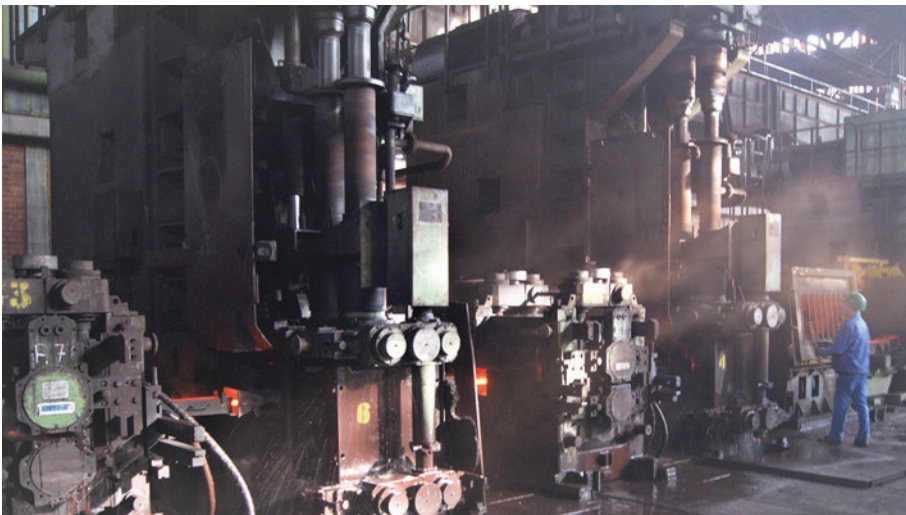
Fig. 5.32 Example of a continuous rolling mill (center section) for bars and wire. (Photo: Schlegel, J., BGH Edelstahl Freital GmbH)
