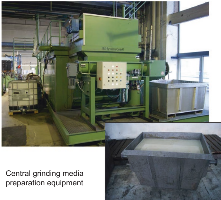
Fig. 10.14 Example of a central facility for filtering used grinding emulsion in a bright steel grinding plant. (Photos: Schlegel, J., BGH Edelstahl Lugau GmbH)
