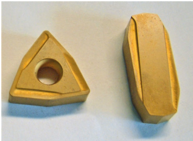
Fig. 8.20 Carbide indexable inserts for turning. (Photo: Schlegel, J.)
