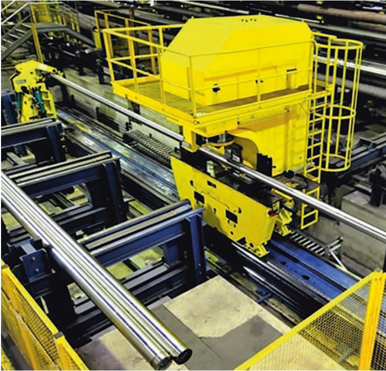
Fig. 9.5 Bending and straightening of forged round stock with an automatic 10 MN fine straightening press. (Photo: BGH Edelstahl Siegen GmbH)
