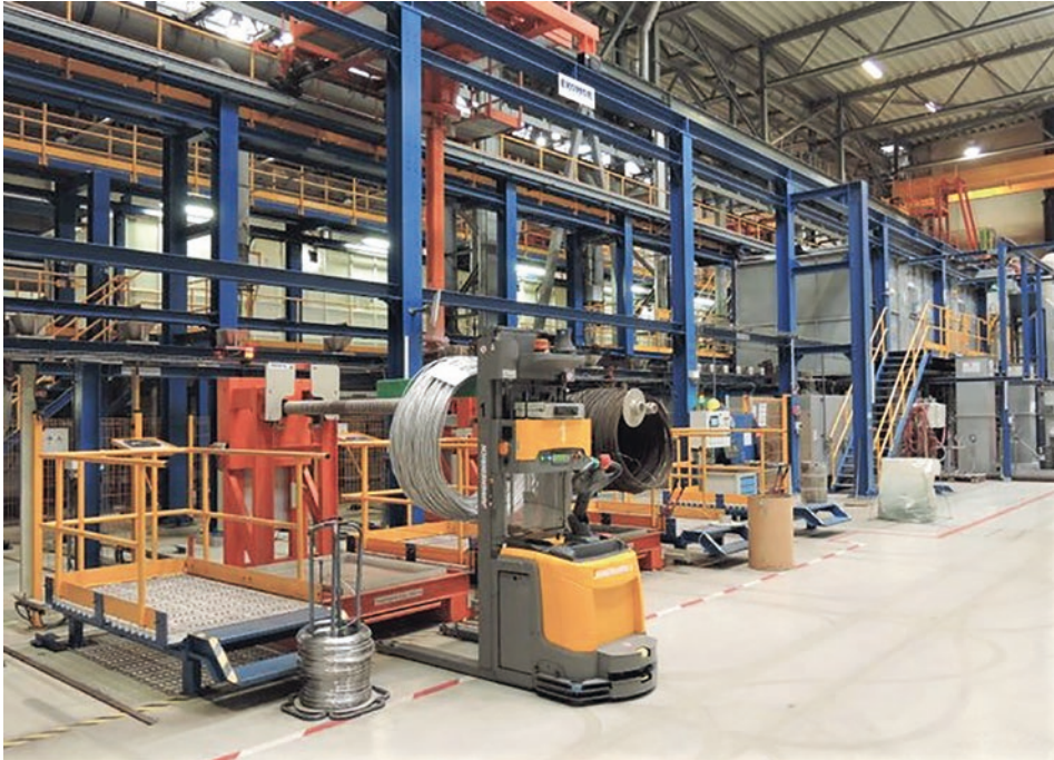
Fig. 5.66 Automated pickling line for rolled wire. (Photo: BGH Edelstahl Lugau GmbH)
