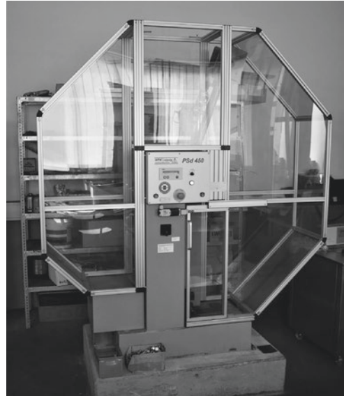
Fig. 7.13 Principle of the Charpy impact test and photo of a pendulum impact machine in a material testing laboratory. (Photo: Schlegel, J., BGH Edelstahlwerke GmbH)
