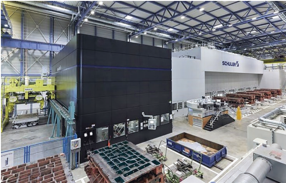
Fig. 5.56 Fully automatic servo press line with a press force of 10,000 t for the mass production of car body parts for automobiles. (Photo: Schuler AG, Göppingen)
