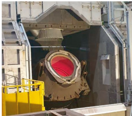
Fig. 4.20 Schematic of an AOD converter and view into an open AOD converter plant. (Photo: BGH Edelstahl Freital GmbH)
