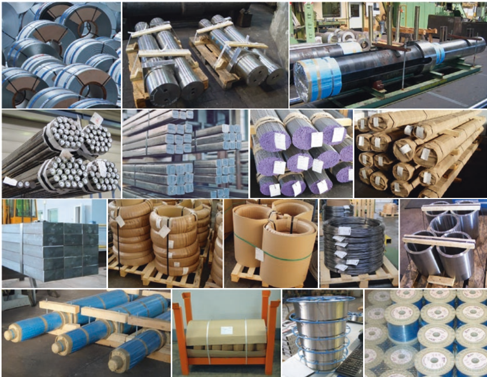
Fig. 9.8 Packaging types for various steel products. (Photos: Thyssenkrupp Steel Europe AG, Schlegel, J., BGH Edelstahlwerke GmbH)
