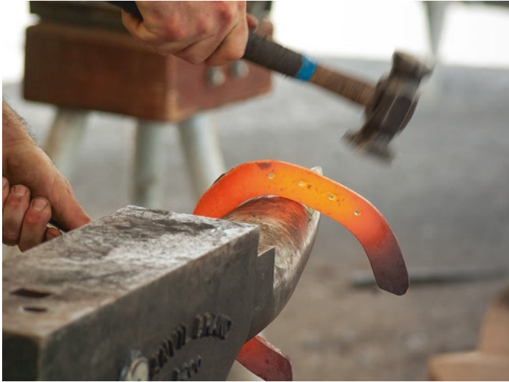
Fig. 5.3 Forging a horseshoe with the hand hammer on the anvil. (Photo from the Internet)
