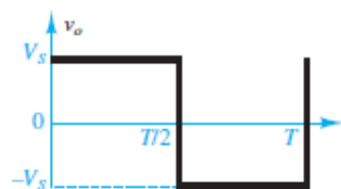
Figure 15.54 Half-bridge voltage source inverter output waveform
