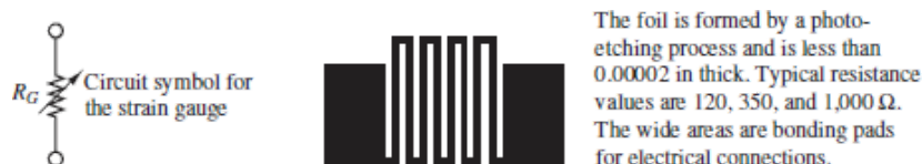
Figure 2.6 Metal-foil resistance strain gauge
