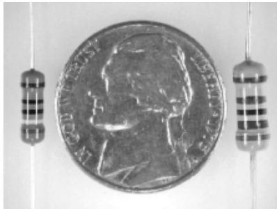
Figure 1.43 Typical \frac{1}{2} -W resistors ( Jim Kearns )
