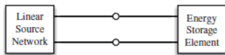
Figure 4.15 Generalized first-order circuit seen as a source network attached to an energy storage element as the load
