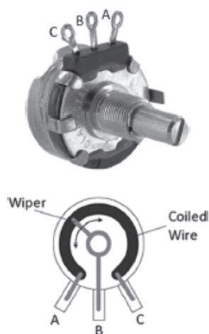
Figure 1.51 A typical \frac{1}{2} -watt potentiometer and its internal construction ( Jim Kearns )
