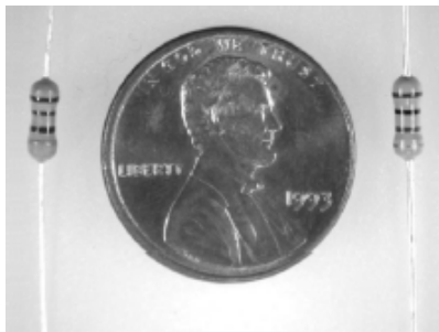
Figure 1.42 Typical \frac{1}{4} -W resistors ( Jim Kearns )
