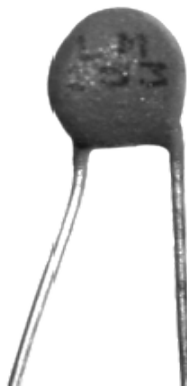
Figure 1.48 A typical negative temperature coefficient (NTC) thermistor ( Jim Kearns )
