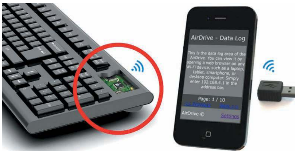
Figure 3-4 Wi-Fi USB keylogger, keylogger keyboard, and keylogger phone app
