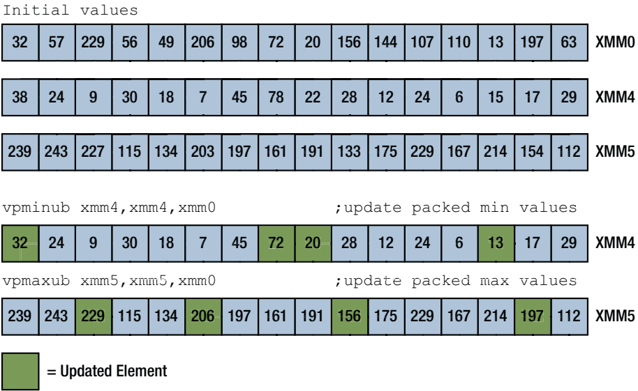
Figure 8-3. Pixel minimum and maximum compares using vpmminub and vpmmaxub
