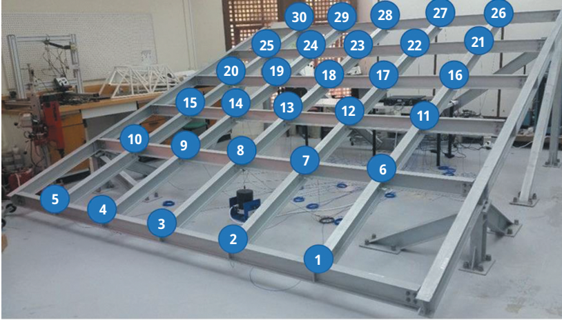
Figure 7.5: Qatar University Grandstand simulator structural steel frame [25].
