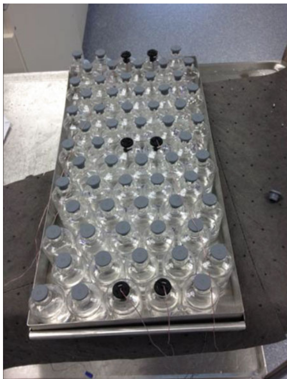
Fig. 1 Hexagonal packing of vials on lyophilizer tray
