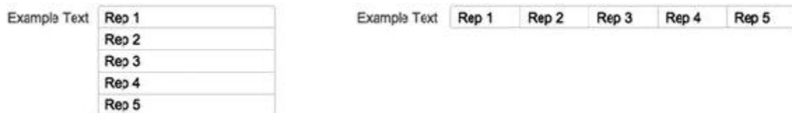
Figure 30-29. A text field defined with five repetitions displayed on a layout in both vertical and horizontal arrangement
