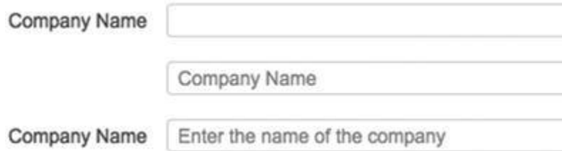
Figure 30-27. An example of three instances of the same Company Name field: one with no placeholder text, one with the field name as the placeholder, and one with a prompt message as the placeholder.
