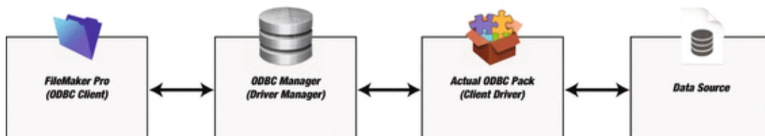
Figure 7-2. The connection between a FileMaker and an external data source through an ODBC connection
