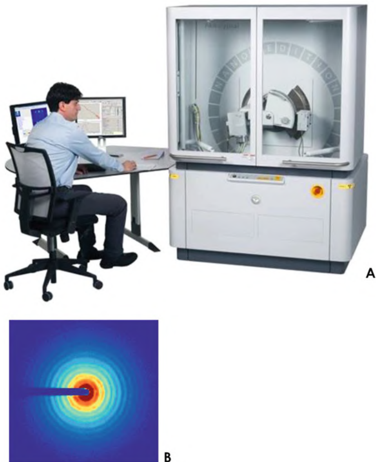
Fig. 6.22 An SAXS instrument based-on an X-ray diffraction platform (a), and a 2D image of a colloidal crystal generated by the instrument (b). Courtesy of Malvern Panalytical
