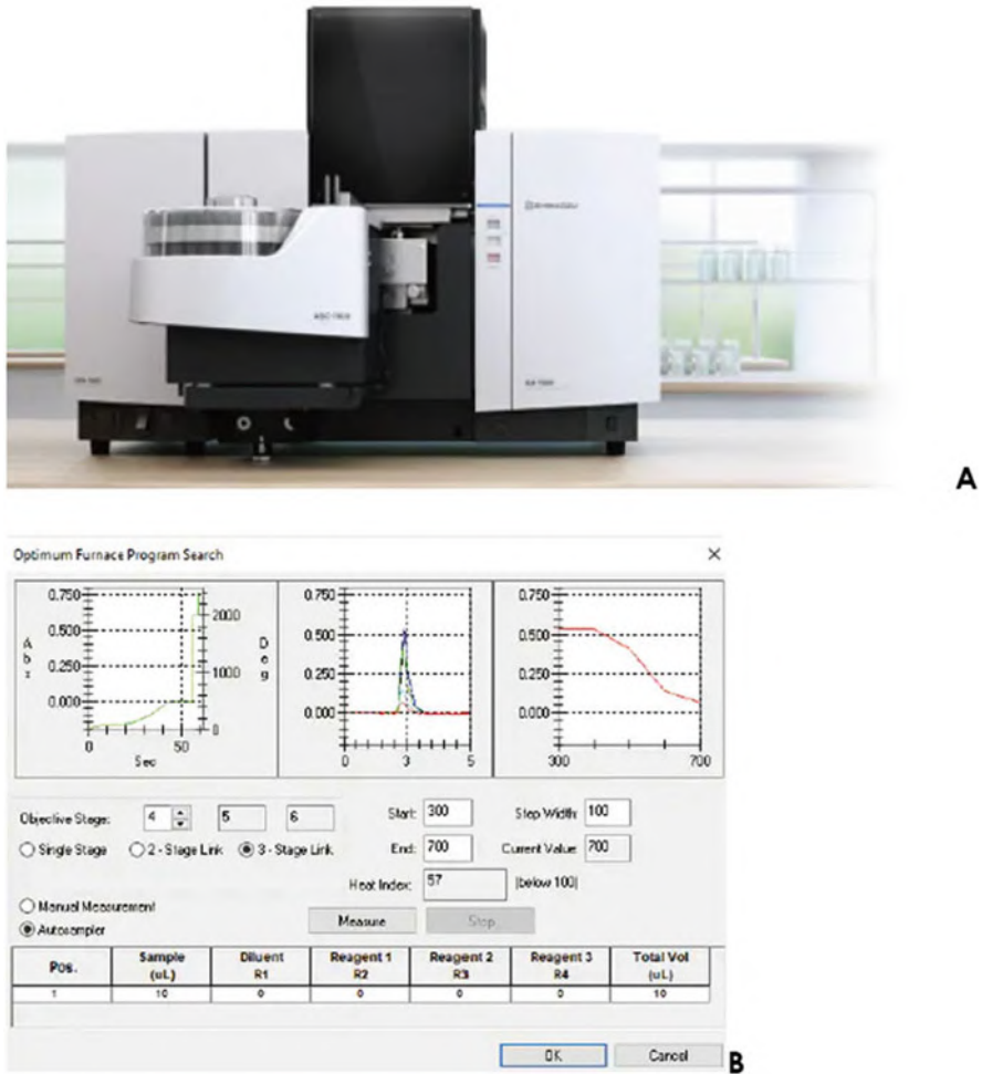
Fig. 5.3 An AAS spectrometer (a), and the obtained measurement (b). Courtesy of Shimadzu
