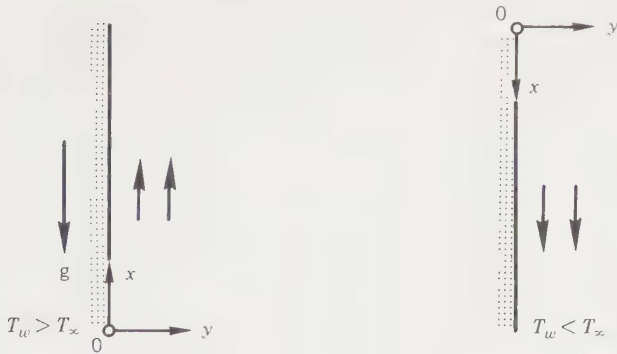
Figure 18.10. System coordinates for heating and cooling of a vertical plate.
