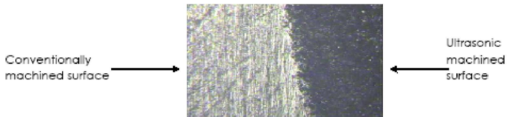
Figure 14. Photomicrograph of the machined surface showing comparison of the conventional machining and ultrasonic machining; Magnification; 100x [1].
