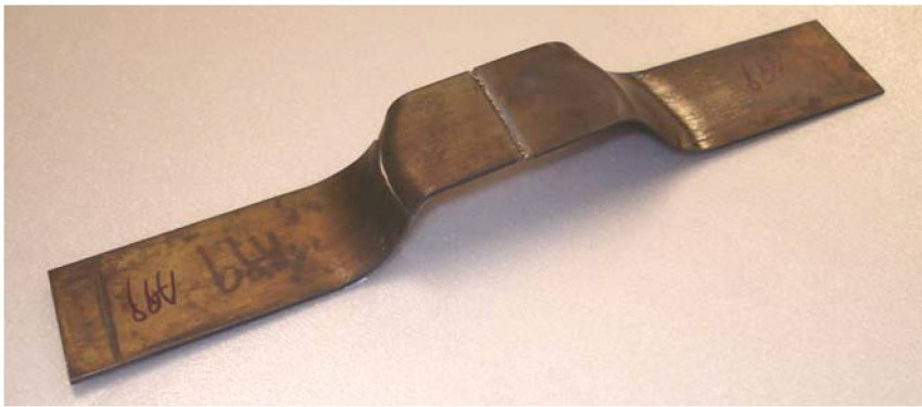
Figure 7. Specimen of 25mm width Ti-TWB after forming test at 550°C.
