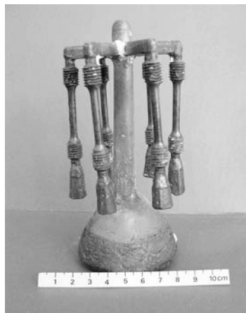
Figure 2. Assembly of precision cast samples for tensile tests.
