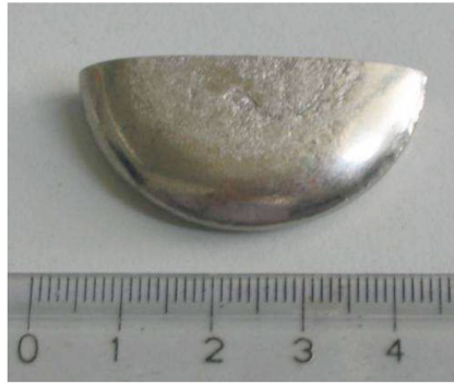
Figure 1. Outer shape of a Ti-Fe-Sn ingot solidified at a cooling rate of \sim 10 K/s.
