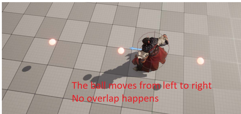
Figure 8.19 – A projectile moving fast may skip the player without firing overlap events
