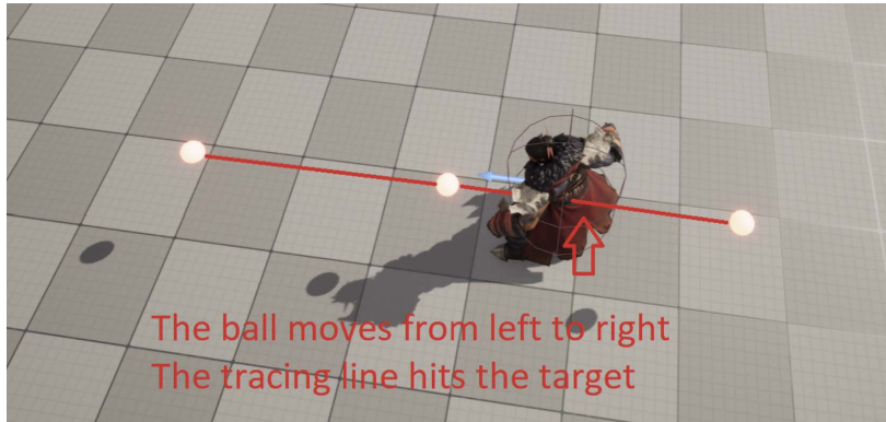
Figure 8.20 – A projectile moving fast with a tracing line can detect hitting the player
