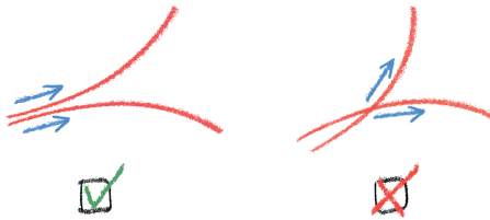
Figure 1.6: Two trajectories cannot intersect in the phase space.
