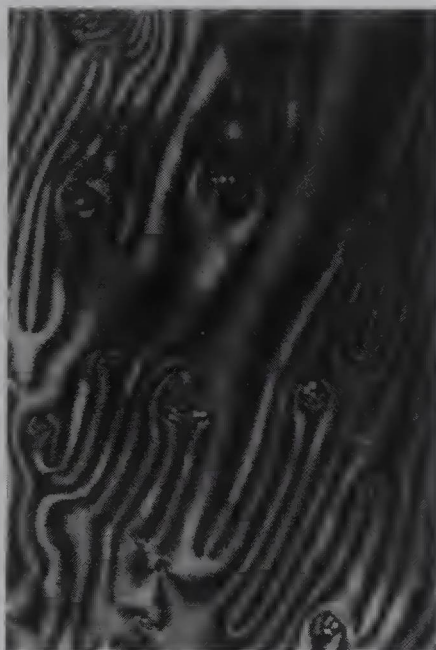
Fig. 4.8-6 Characteristic optical texture of the nematic phase (from J. Chem. Soc., Chem. Commun. , 1994, 729, by permission of the Royal Society of Chemistry).
