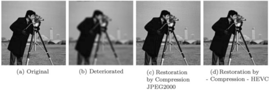
Fig. 3 The deblurring experiment (settings #2 in Dar et al. 2018c) for the Cameraman image ( 256 \times 256 pixels). (a) The underlying image. (b) Degraded image (20.76 dB). (c) Restored image using Algorithm 5 with JPEG2000 compression (28.10 dB). (d) Restored image using Algorithm 5 with HEVC compression (30.14 dB)
