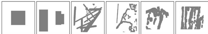
Fig. 8 Example for each kind of mask considered for evaluation. In gray are the hidden pixels. From left to right: center, random regular, random irregular, and irregular Pconv masks from Liao et al. (2018) with <20\% , [40\%, 60\%] and [40\%, 60\%] hidden pixels
