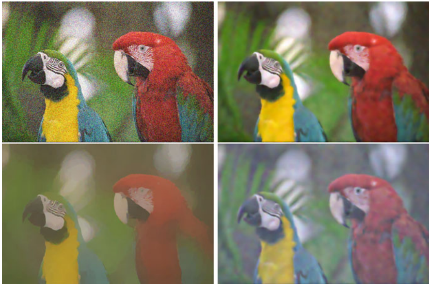
Fig. 13 Application of the Chambolle-Lions model to the denoising of the parrots image. Upper row, left: Noisy data. Upper row, right: Total result \hat{u}_1 + \hat{u}_2 using the balanced discrepancy principle. Lower row, left: Cartoon part \hat{u}_1 of the solution. Lower row, right: Texture part \hat{u}_2 of the solution
