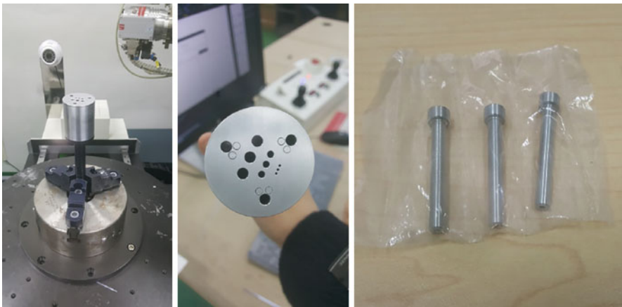
Fig. 16 Sample 2: Data acquisition setting (left), upper view of sample body (middle), and lead (Pb) poles. (Reprinted from Jeon et al. (2021) with permission from Taylor & Francis)
