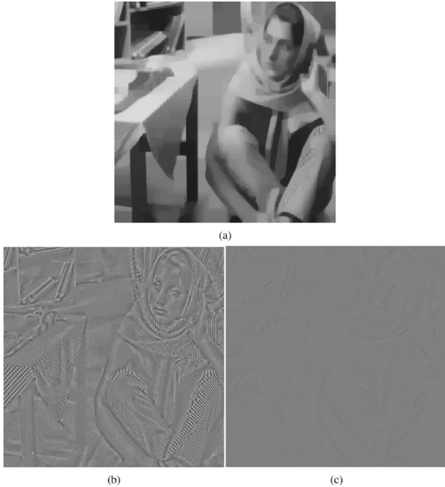
Fig. 2 The minimizer of the first problem in (24). The output images x - u_1 - u_2 , u_1 + 0.5 , and u_2 + 0.5 are shown in (a), (b), and (c), respectively
