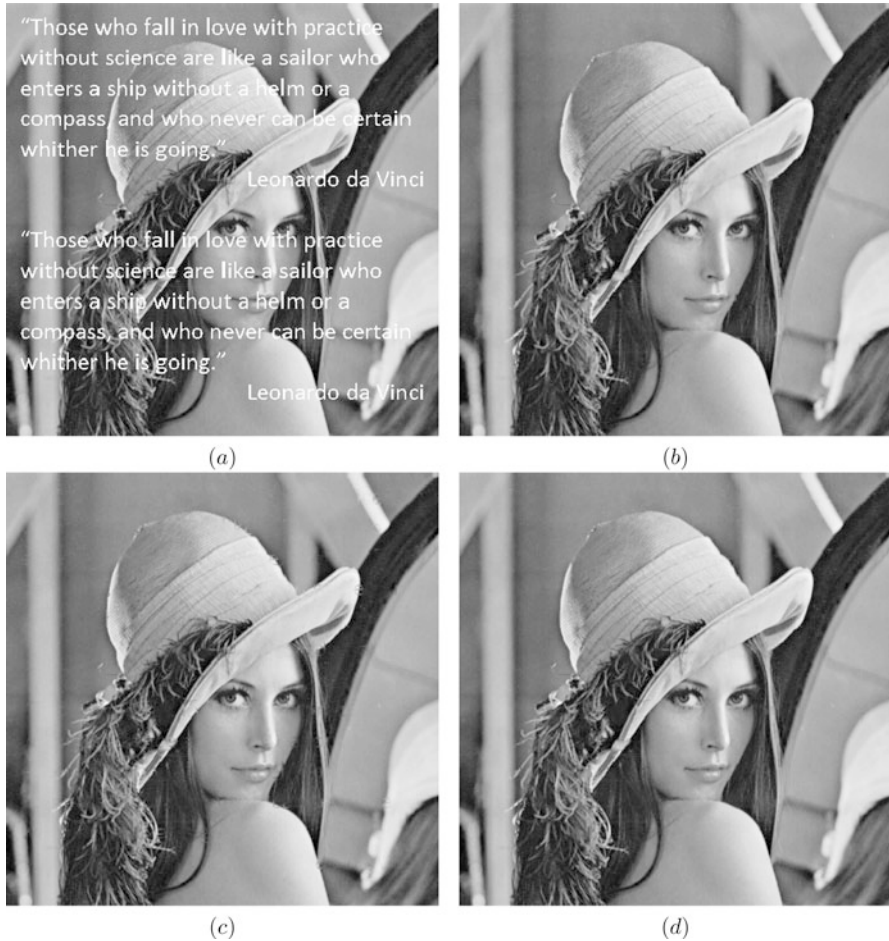
Fig. 28 Inpainting of a text overprinted on an image. (a) Input image; (b) restored image A_{\lambda}^M(f_K) using Algorithm 2. PSNR = 39.122 dB. Parameters: \lambda = 18 and M = 1 \cdot 10^5 . Total number of iterations: 19; (c) restored image by the AMLE method described in Schönlieb (2015) and Parisotto and Schönlieb (2016). PSNR = 36.406 dB. Total number of iterations: 5247; (d) restored image by the split Bregman inpainting method described in Getreuer (2012). PSNR = 39.0712 dB. Total number of iterations: 19
