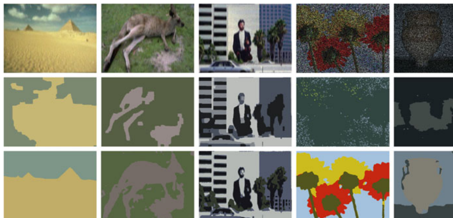
Fig. 6 Color image segmentation for degraded images. First row: degraded color images (the first three images are degraded by various noise and blur, and the last two images are degraded by 60% information loss and noise). Second row: Pock et al. (2009a). Third row: SLaT method (Cai et al. 2017)
