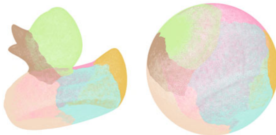
Fig. 7 The spherical conformal parameterization of a genus-0 duck surface mesh obtained using the parallelizable global conformal parameterization (PGCP) method. (Image adapted from Choi et al. 2020a). The colors indicate the correspondence between the subdomains in the original mesh and in the parameterization result
