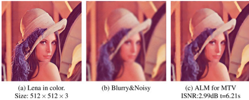
Fig. 7 Augmented Lagrangian method for multichannel TV (MTV) restoration (b) is a corruption of (a) with within-channel Gaussian blur f_{\text{special}}('gaussian', 21, 5) , and Gaussian noise with variation 1e - 3 ; (c) is the recovered result
