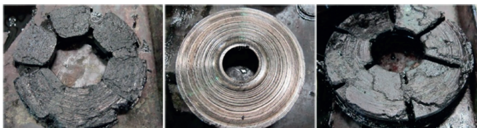
Figure 16. Examples of protector thrust bearing/runner damages.
