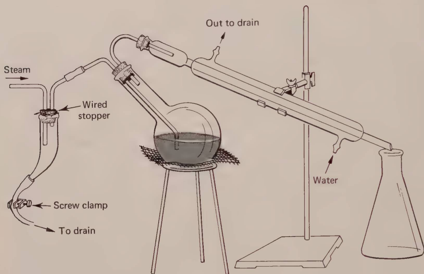
Figure 22. Assembly for Steam Distillation
