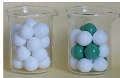
Figure 6.4 An illustration of Raoult's law: lowering of vapor pressure by addition of solute molecules. White units represent solvent molecules, and green units are solute molecules. Solute molecules present a barrier to escape of solvent molecules, thus decreasing the vapor pressure. Danaë R. Quirk, Ph.D.
