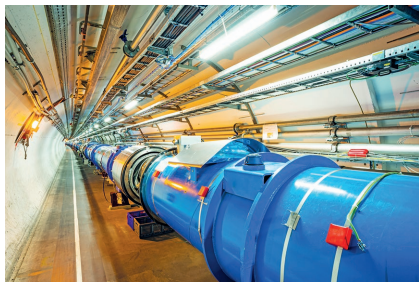
Figure 9.7 A portion of the Large Hadron Collider beneath the France-Switzerland border. Particles can be accelerated at velocities close to the speed of light and accurately strike small “target” nuclei. At such facilities, rare isotopes can be synthesized and their properties studied. Xenotar/Getty Images
