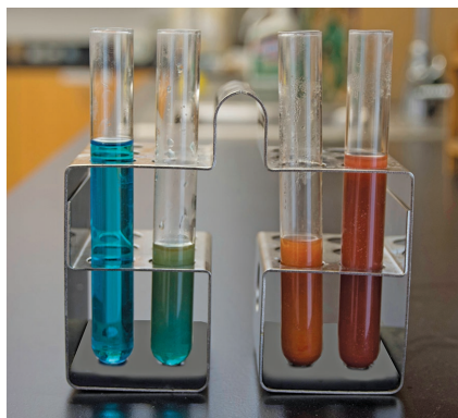
Figure 13.5 The amount of precipitate formed and thus the color change observed in the Benedict's test are directly proportional to the amount of reducing sugar in the sample.
