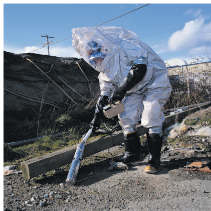
Figure 9.11 A worker in a protective suit is measuring soil radioactivity using a Geiger counter. Arthur S. Aubry/Getty Images
