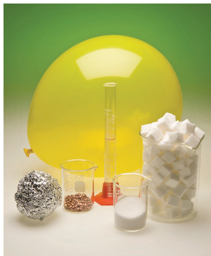
Figure 4.1 The comparison of approximately 1 mol each of aluminum, copper, water, nitrogen (in the balloon), salt, and sugar shows the considerable difference in mass of equivalent mol of various substances.
