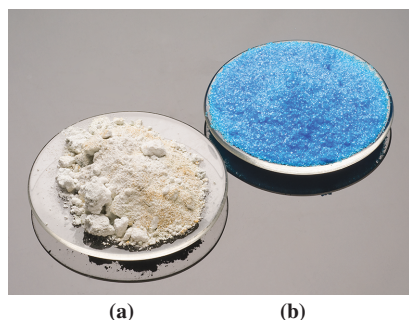
Figure 4.3 The marked difference in color of (a) anhydrous and (b) hydrated copper sulfate is clear evidence that they are, in fact, different compounds. Charles D. Winters/Timeframe Photography/McGraw Hill
