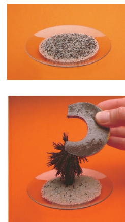
Figure 1.7 An example of separation based on differences in physical properties. Magnetic iron is separated from nonmagnetic substances. A large-scale version of this process is important in the recycling industry.
