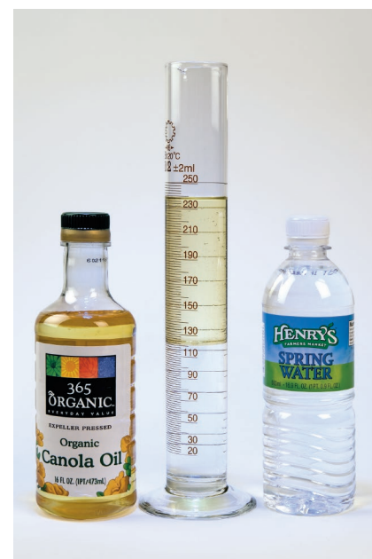
Figure 3.14 The interaction of polar water molecules and nonpolar oil molecules. The familiar salad dressing—oil and vinegar—forms two layers. The oil does not dissolve in vinegar, an aqueous solution of acetic acid.
