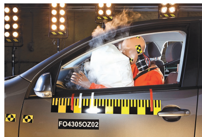
Air bag deployment is frequently evaluated in crash tests. fStop Images GmbH/Alamy Stock Photo
