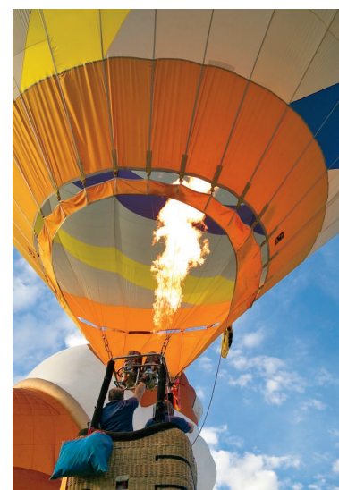
Figure 5.5 Charles's law predicts that the volume of air in the balloon will increase when heated. Open Door/Alamy Stock Photo
