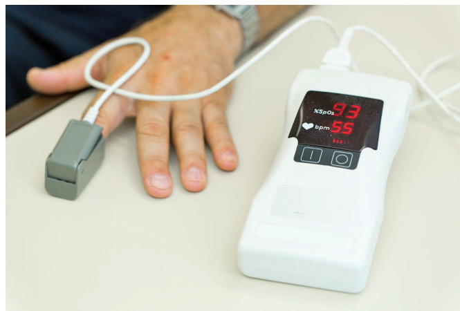
A pulse oximeter measures oxygen saturation which can be used to determine how well oxygen is being distributed to tissues. Choja/Getty Images
