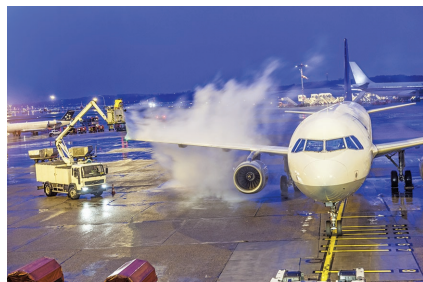
The solute ethylene glycol, “antifreeze,” is commonly used in aircraft deicing/anti-icing solutions to prevent the buildup of ice by lowering the freezing point of the coolant. Meinzahn/iStock/Getty Images
