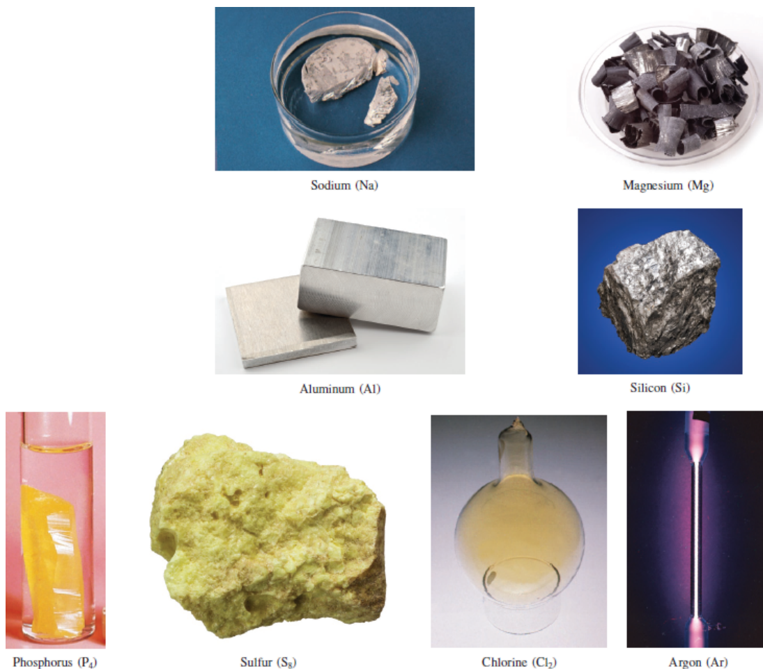
Figure 8.10 The third-period elements. The photograph of argon, which is a colorless, odorless gas, shows the color emitted by the gas from a discharge tube.
