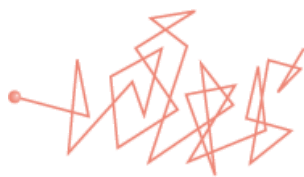
Figure 5.19 The path traveled by a single gas molecule. Each change in direction represents a collision with another molecule.
