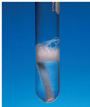
Figure 4.6 A piece of blackboard chalk, which is mostly \text{CaCO}_3 , reacts with hydrochloric acid.
