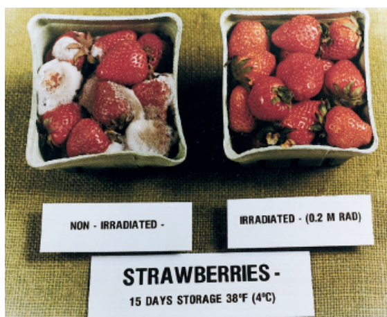
Strawberries irradiated at 200 kilorads (right) are still fresh after 15 days storage at 4°C; those not irradiated are moldy.
