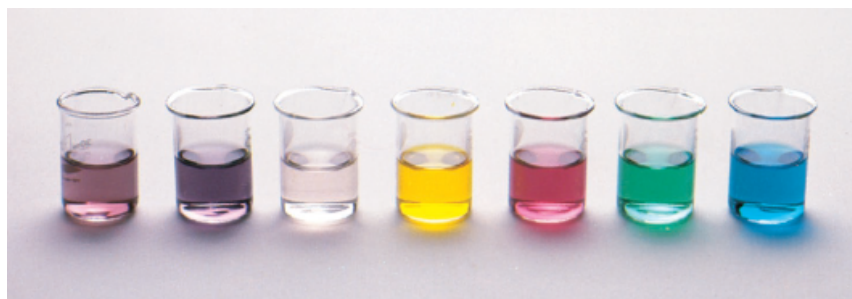
Figure 23.17 Colors of some of the first-row transition metal ions in solution. From left to right: \text{Ti}^{3+} , \text{Cr}^{3+} , \text{Mn}^{2+} , \text{Fe}^{3+} , \text{Co}^{2+} , \text{Ni}^{2+} , \text{Cu}^{2+} . The \text{Sc}^{3+} and \text{V}^{5+} ions are colorless.
