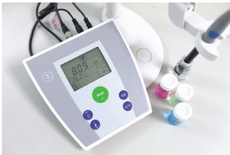
Figure 15.2 A pH meter is commonly used in the laboratory to determine the pH of a solution. Although many pH meters have scales marked with values from 1 to 14, pH values can, in fact, be less than 1 and greater than 14.
