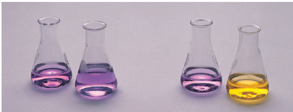
Figure 16.1 The acid-base indicator bromophenol blue (added to all solutions shown) is used to illustrate buffer action. The indicator's color is blue-purple above pH 4.6 and yellow below pH 3.0. (Left to right) (a) A buffer solution made up of 50 mL of 0.1 M \text{CH}_3\text{COOH} and 50 mL of 0.1 M \text{CH}_3\text{COONa} . The solution has a pH of 4.7 and turns the indicator blue-purple. (b) After the addition of 40 mL of 0.1 M \text{HCl} solution to the solution in (a), the color remains blue-purple. (c) A 100-mL \text{CH}_3\text{COOH} solution whose pH is 4.7. (d) After the addition of 6 drops (about 0.3 mL) of 0.1 M \text{HCl} solution, the color turns yellow. Without buffer action, the pH of the solution decreases rapidly to less than 3.0 upon the addition of 0.1 M \text{HCl} .
