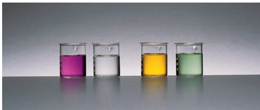
Figure 4.22 Left to right: Solutions containing the \text{MnO}_4^- , \text{Mn}^{2+} , \text{Cr}_2\text{O}_7^{2-} , and \text{Cr}^{3+} ions.
