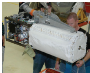
Figure 18.12 A hydrogen- oxygen fuel cell once used in the space program. The pure water produced by the cell was consumed by the astronauts.
