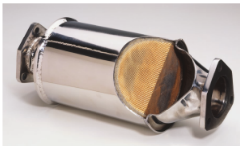
Figure 13.29 A cross-sectional view of a catalytic converter. The beads contain platinum, palladium, and rhodium, which catalyze the conversion of CO and hydrocarbons to carbon dioxide and water.
