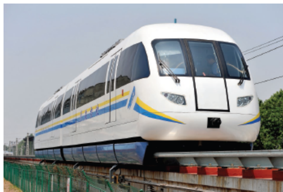
An experimental levitation train that operates on superconducting material at the temperature of liquid helium.
