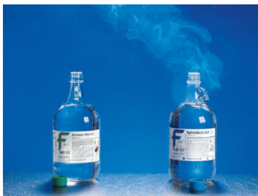
Figure 5.20 A demonstration of gas diffusion. \text{NH}_3 gas (from a bottle containing aqueous ammonia) combines with \text{HCl} gas (from a bottle containing hydrochloric acid) to form solid \text{NH}_4\text{Cl} . Because \text{NH}_3 is lighter and therefore diffuses faster, solid \text{NH}_4\text{Cl} first appears nearer the \text{HCl} bottle (on the right).
