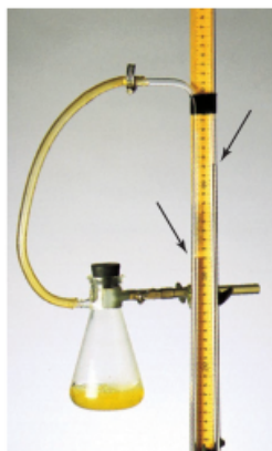
Figure 13.7 The rate of hydrogen peroxide decomposition can be measured with a manometer, which shows the increase in the oxygen gas pressure with time. The arrows show the mercury levels in the U tube.
