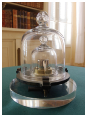
Figure 1.5 The prototype kilogram is made of a platinum-iridium alloy. It is kept in a vault at the International Bureau of Weights and Measures in Sèvres, France. In 2007 it was discovered that the alloy has mysteriously lost about 50 \mu\text{g} !
