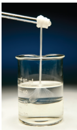
Figure 25.7 The nylon rope trick. Adding a solution of adipoyl chloride (an adipic acid derivative in which the OH groups have been replaced by Cl groups) in cyclohexane to an aqueous solution of hexamethylenediamine causes nylon to
