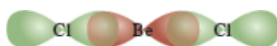
Figure 10.13 The linear geometry of \text{BeCl}_2 can be explained by assuming that Be is sp -hybridized. The two sp hybrid orbitals overlap with the two chlorine 3p orbitals to form two covalent bonds.
