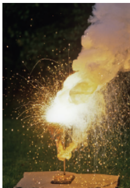
Figure 21.19 The temperature of a thermite reaction can reach 3000°C.
