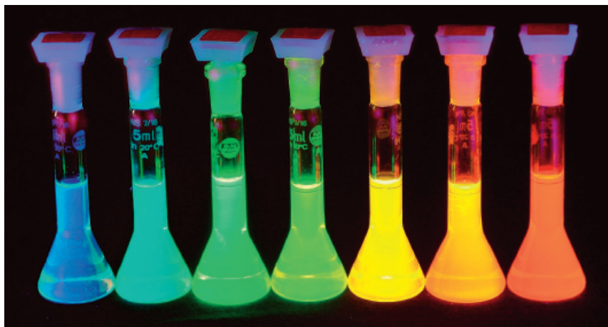
Emission from dispersed solutions of CdSe quantum dots arranged from left to right in order of increasing diameter (2 nm to 7 nm).
