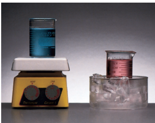
Figure 14.11 (Left) Heating favors the formation of the blue \text{CoCl}_4^{2-} ion. (Right) Cooling favors the formation of the pink \text{Co}(\text{H}_2\text{O})_6^{2+} ion.
