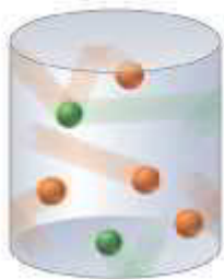
FIGURE 8.1 Gas particles moving in straight lines within a container exert pressure when they collide with the walls of the container.
