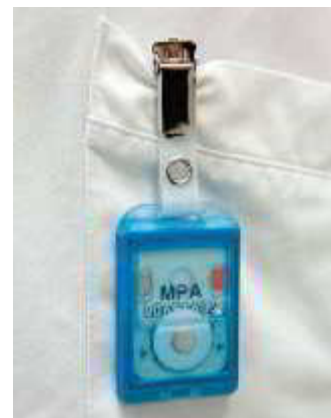
A dosimeter measures radiation exposure.
