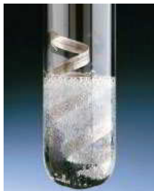
Magnesium reacts rapidly with acid and forms \text{H}_2 gas and a salt of magnesium.
