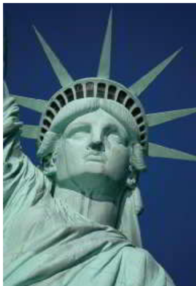
The green patina on copper is due to oxidation.
