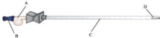
Fig. 12.20 Magseed—A—Safety bung made of rubber—prevents accidental deployment of seed, B—Plunger, C—Hollow needle containing plunger and Magseed, D—Needle tip for release of seed
