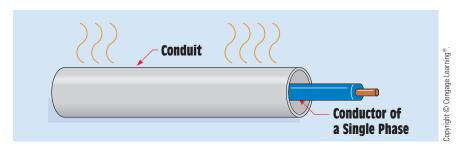
FIGURE 11-22 A single-phase conductor causes heat to be produced in the conduit.
