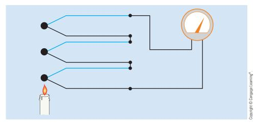
FIGURE 13-36 A thermopile is a series connection of thermocouples.
