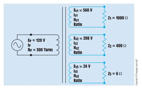
FIGURE 28–15 Calculating values for a transformer with multiple secondary windings.
