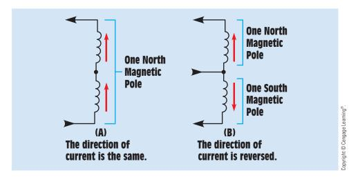
**FIGURE 33–45** The number of poles can be changed by reversing the current flow through alternate poles.
