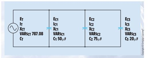
FIGURE 21–14 Capacitors connected in parallel.
