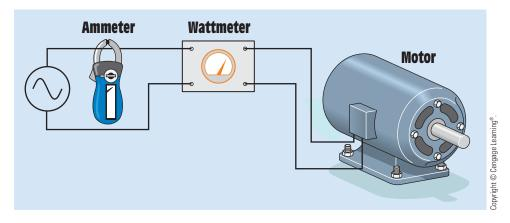
FIGURE 25–15 Determining motor power factor.
