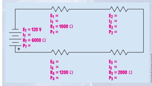
FIGURE 6–12 Series circuit, Example 2.
