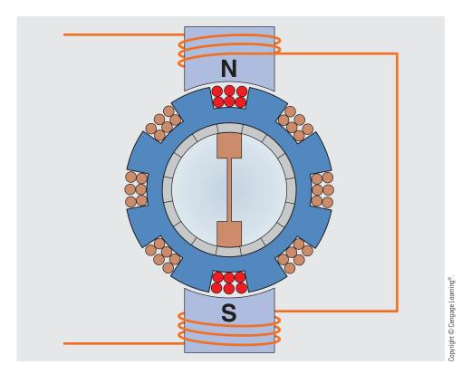
FIGURE 34-40 The brushes are set at a 0° angle to the pole pieces.
