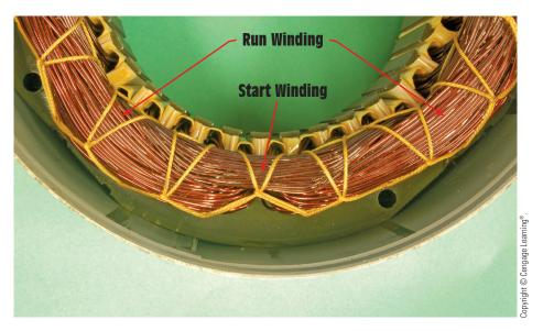
**FIGURE 34–2A** Stator winding of a resistance-start induction-run motor. The start winding contains much smaller wire than the run winding.
