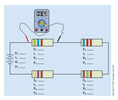
FIGURE 6-27 Determine resistor values using the color code, and determine all missing electrical values.
