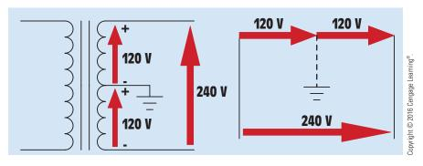
**FIGURE 27–9** The voltages of a residential system are in phase with each other.
