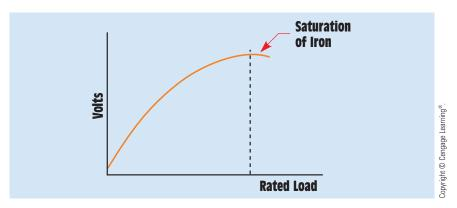
FIGURE 30–31 Characteristic curve of a series generator.
