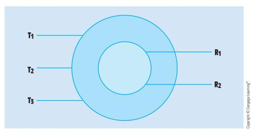
FIGURE 33-57 Schematic symbol for a synchronous motor.
