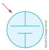
FIGURE 13–32 Schematic symbol for a solar cell.
