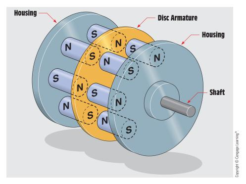
FIGURE 31–34 The permanent magnets are arranged to produce alternate magnetic polarities.
