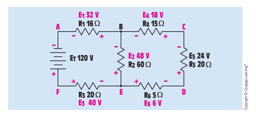
FIGURE 9-3 Marking resistor elements.
