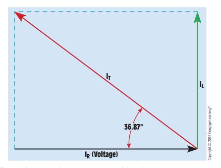
FIGURE 19-10 Relationship of voltage and current in an R-L parallel circuit.
