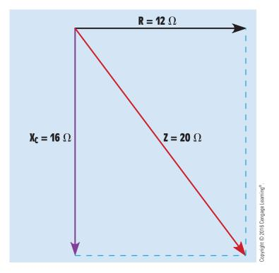
FIGURE 22–3 Impedance vector for example circuit 1.
