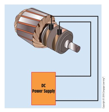
FIGURE 33-52 DC excitation current supplied through sliprings.
