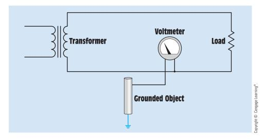
FIGURE 10-44 High-impedance ground paths can produce misleading voltage readings.
