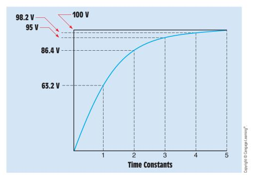
FIGURE 20–14 Capacitors charge at an exponential rate.
