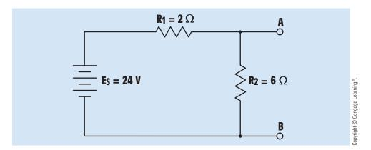
FIGURE 9-15 Determining the Norton equivalent circuit.
