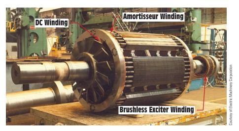
FIGURE 33-51 Synchronous-motor rotor with amortisseur winding.
