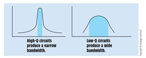
FIGURE 25–12 The Q of the circuit determines the bandwidth.
