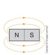
**FIGURE 4–8** Magnetic lines of force are called lines of flux.
