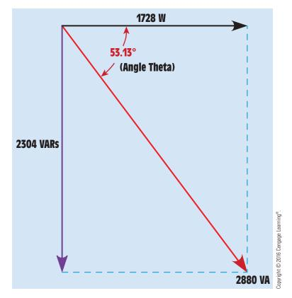
FIGURE 22–6 Apparent power vector for example circuit.
