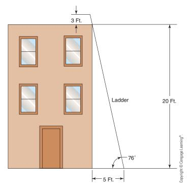
FIGURE S-15 A ladder should be placed at an angle of approximately 76°.
