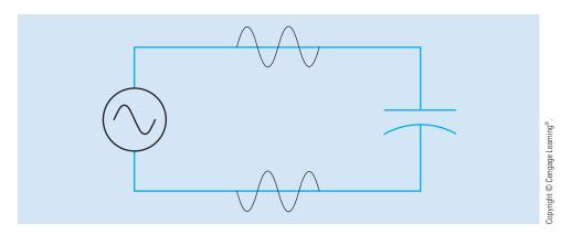
FIGURE 21–3 A capacitor connected to an AC circuit.
