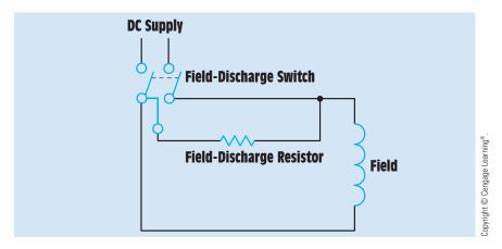
FIGURE 32-18 Switch in open position.
