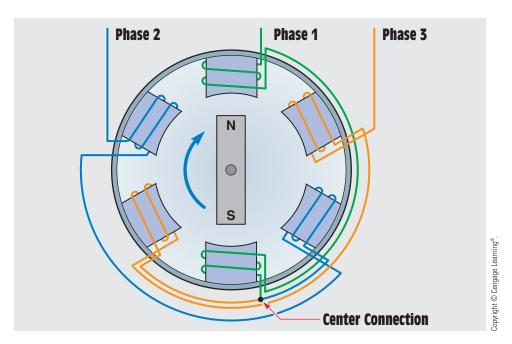
FIGURE 32–3 Basic design of a three-phase alternator.
