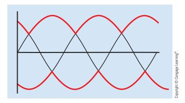
**FIGURE 27–2** Three-phase power never falls to zero.
