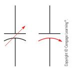
FIGURE 20–29 Variable capacitor symbols.
