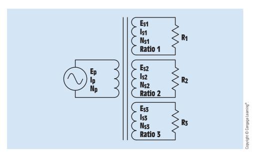
FIGURE 28–70 Single-phase transformer with multiple secondaries.
