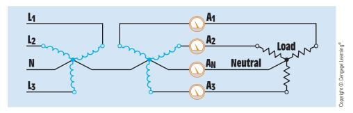
FIGURE 29–25 Neutral conductor is supplied by the incoming power.
