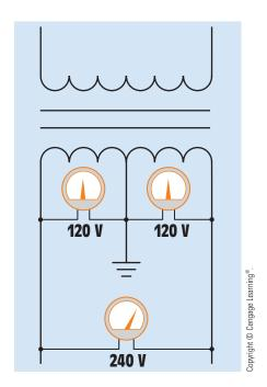
**FIGURE 28–18** The voltage from either line to neutral is 120 volts. The voltage across the entire secondary winding is 240 volts.
