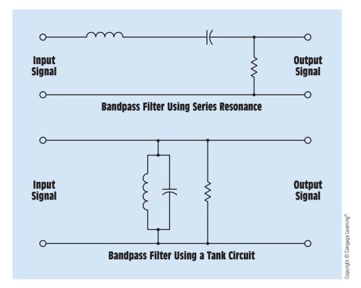
FIGURE 26-14 Basic bandpass filters.
