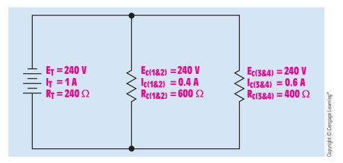
FIGURE 8-3 Simplifying the combination circuit.
