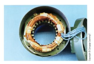
FIGURE 33-11 Stator of a three-phase motor.
