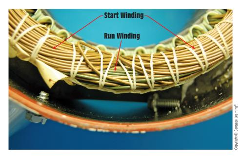
**FIGURE 34–2B** Stator winding of a capacitor-start capacitor-run motor. The wire size is the same for both start and run windings.
