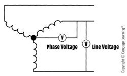
In a wye connection, the line current and phase current are the same:
