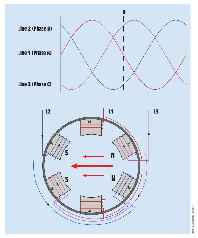
FIGURE 33–5 The magnetic field is concentrated between phases B and C.
