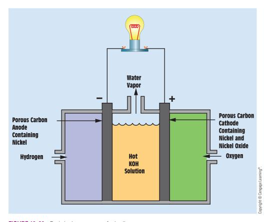
**FIGURE 13–39** Basic hydrogen-oxygen fuel cell.
