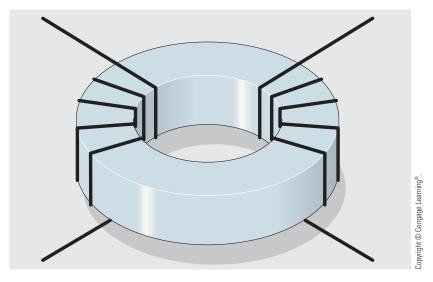
FIGURE 28–32 A toroid transformer.
