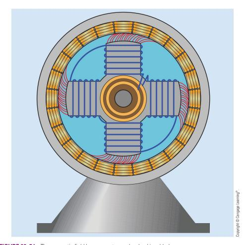
FIGURE 33–54 The magnetic field becomes stressed as load is added.
