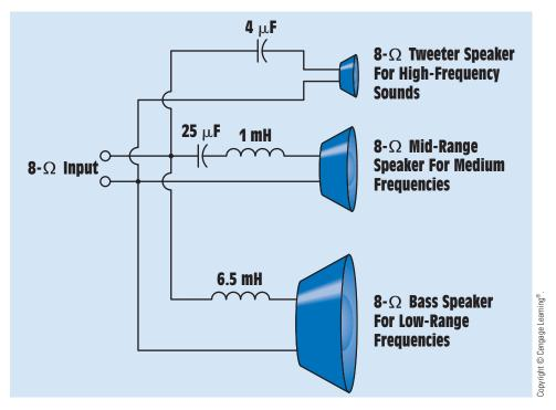
FIGURE 26-19 Speaker crossover network using low-pass, high-pass, and bandpass filters.
