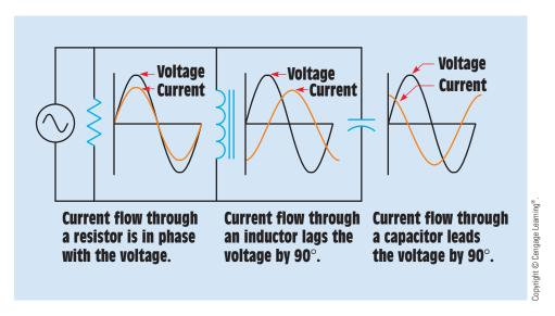
**FIGURE 25–1** Voltage and current relationship in an RLC parallel circuit. The voltage is the same across each branch, but the currents are out of phase.
