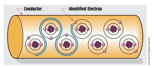
FIGURE 2-5 Electrons moving from atom to atom.
