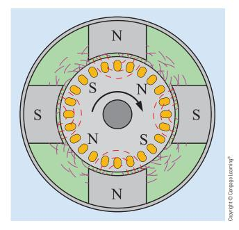
**FIGURE 34–15** A rotating magnetic field is produced by the stator and rotor flux.
