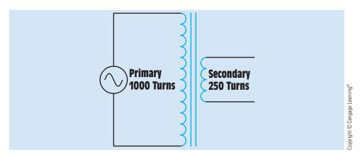
FIGURE 28–1 All values of a transformer are proportional to its turns ratio.
