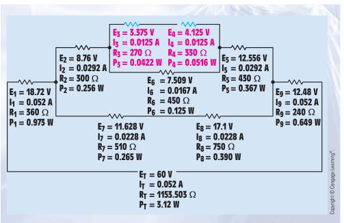
FIGURE 8-20 The values for R<sub>3</sub> and R<sub>4</sub>.
