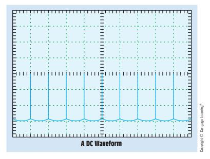
FIGURE 10-58 A DC waveform.
