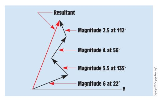
FIGURE 15–18 Adding vectors with different magnitudes and directions.
