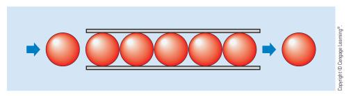
**FIGURE 2–6** When a ball is pushed into one end, another ball is forced out the other end. This basic principle causes the instantaneous effect of electric impulses.
