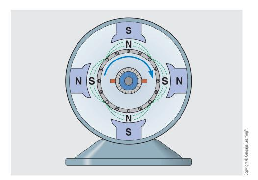
FIGURE 30–47 A magnetic field is produced around the armature.
