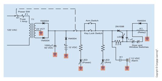
FIGURE 6-24 Burglar alarm with battery backup.
