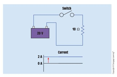
FIGURE 14-13 The current rises instantly in a resistive circuit.
