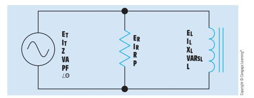
FIGURE 19–1 A resistive-inductive parallel circuit.
