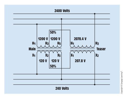
**FIGURE 29–27** T-connected transformers with same voltage rating.
