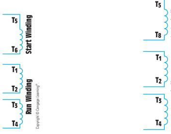
**FIGURE 34–22** Dual-voltage motor with one start winding labeled  $T_5$  and  $T_6$ .
