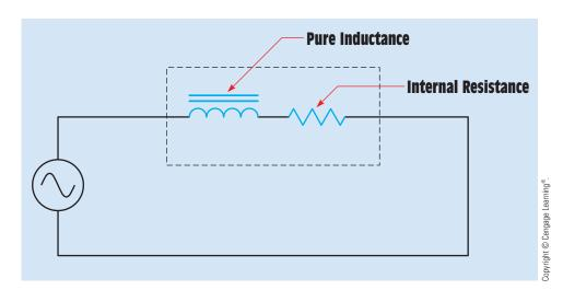
FIGURE 17–16 Inductors contain internal resistance.
