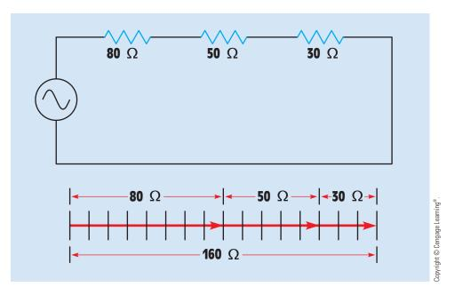
FIGURE 15–15 Addition of series resistors.
