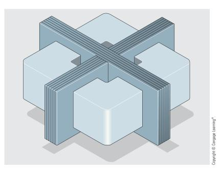
**FIGURE 28–31** A transformer with an H-type core.
