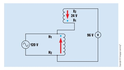
FIGURE 28–52 The arrows help indicate subtractive polarity.
