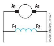
**FIGURE 30–33** Schematic drawing of a shunt generator.
