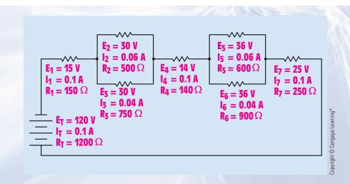
FIGURE 8-8 All values solved for the combination circuit.
