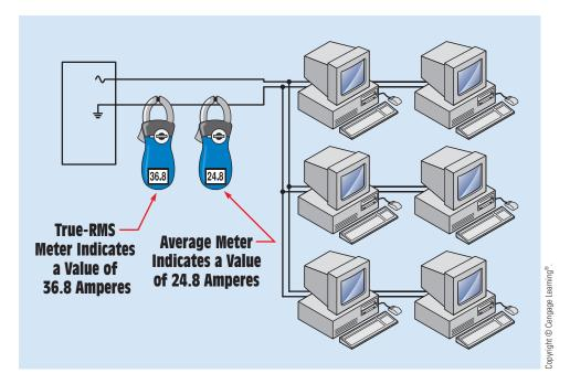
FIGURE 35–8 Determining harmonic problems using two ammeters.
