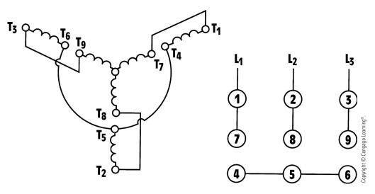
FIGURE A-2 Low-voltage connection.
