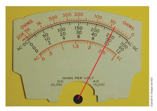
FIGURE 10-11 The meter indicates a value of 250.
