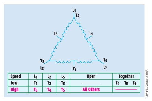
FIGURE 33–46 High-speed series-delta connection.
