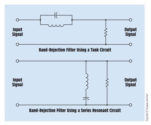
FIGURE 26–16 Basic band-rejection filters.
