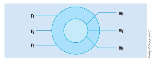
FIGURE 33-50 Schematic symbol for a wound-rotor induction motor.
