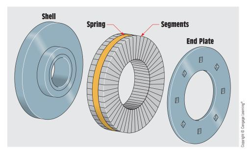
FIGURE 34–44 Short-circuiting ring for brush-riding-type repulsion-start induction-run motor.
