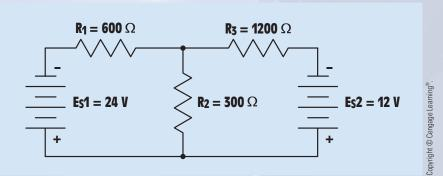
FIGURE 9-20 A circuit with two power sources.
