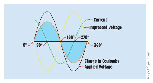
FIGURE 21–7 Voltage, current, and charge relationships for a capacitive circuit.
