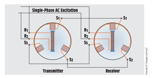
FIGURE 33-60 Connection of two selsyn motors.
