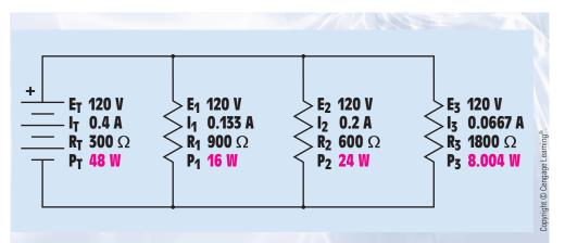
FIGURE 7–18 The values of power for the circuit in Example 2.
