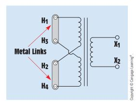
**FIGURE 28–26** Metal links connect transformer for 240-volt operation.
