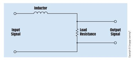
**FIGURE 26–5** A low-pass filter can be constructed by connecting an inductor in series with the load resistance.
