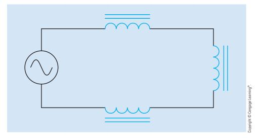
FIGURE 17–10 Inductors connected in series.
