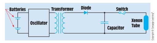
FIGURE 20–10 Energy is stored in a capacitor.
