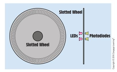
**FIGURE 34–69** Basic operating principle of an encoder.
