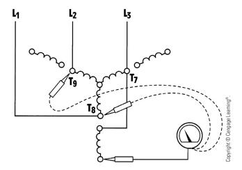
FIGURE A-5 Measure voltage from unconnected paired leads to T<sub>8</sub> and T<sub>9</sub>.
