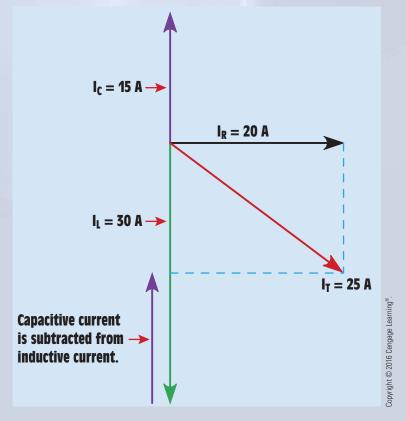
FIGURE 25-3 Vector diagram of resistive, inductive, and capacitive currents in example circuit.
