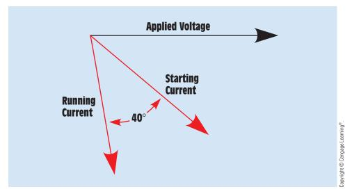
FIGURE 34-4 Running current and starting current are 35° to 40° out of phase with each other.
