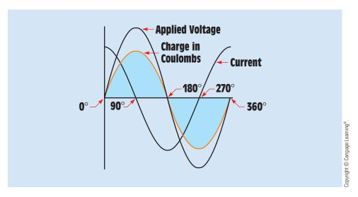
FIGURE 21-5 Capacitive current leads the applied voltage by 90°.
