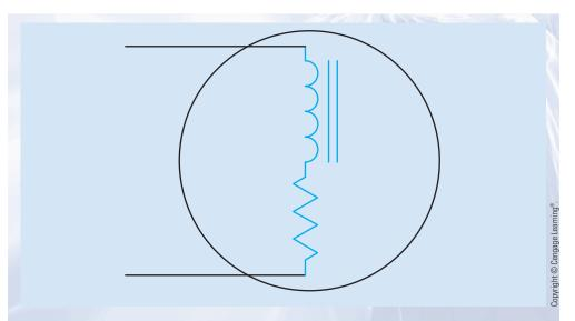
FIGURE 18-26 A motor winding appears to be an R-L series circuit.
