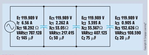
FIGURE 21–15 Parallel circuit with completed values.
