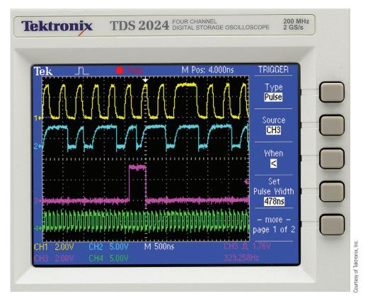
FIGURE 10-52 A four-trace oscilloscope.
