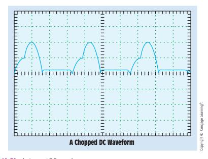
**FIGURE 10–59** A chopped DC waveform.
