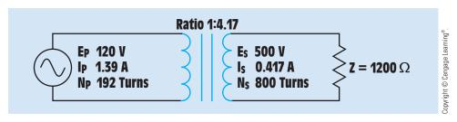
FIGURE 28–11 Transformer with calculated values.
