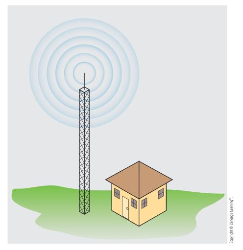
FIGURE 16–17 High-frequency AC causes a magnetic field to radiate at the speed of light.
