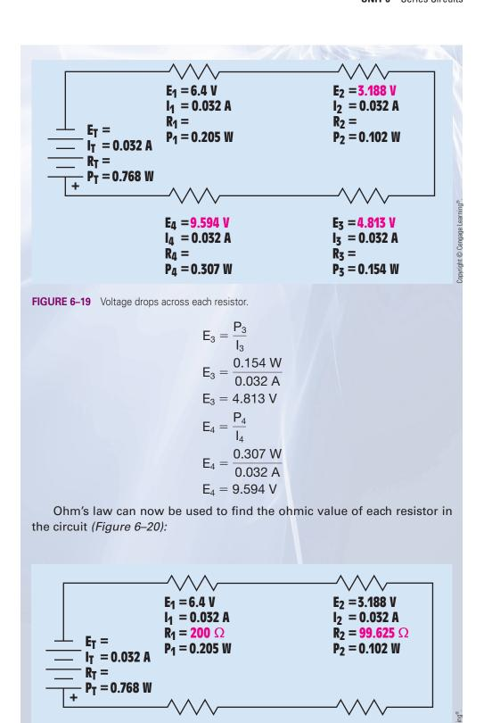
FIGURE 6–20 The ohmic value of each resistor.
