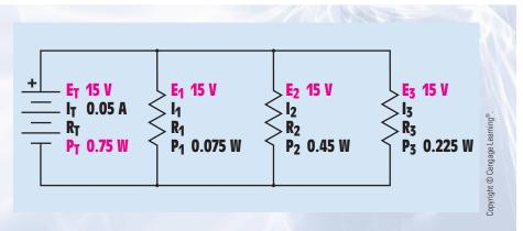
FIGURE 7–20 The applied voltage for the circuit.
