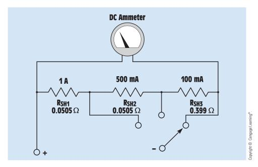
FIGURE 10-24 The Ayrton shunt with resistor values.
