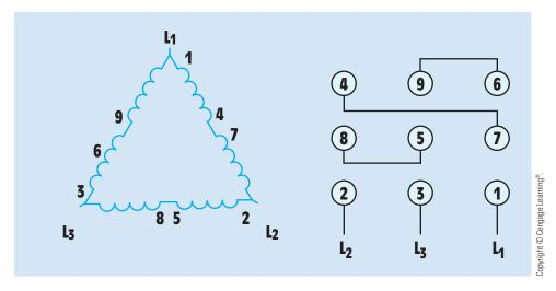
FIGURE 33–17 High-voltage delta connection.
