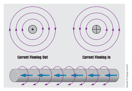
FIGURE 14-1 Current flowing through a conductor produces a magnetic field around the conductor.
