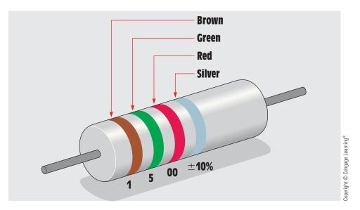
**FIGURE 5–10** Determining resistor values using the color code.
