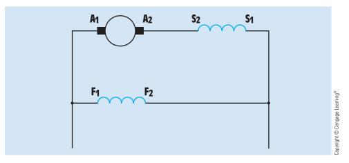
FIGURE 30-41 Schematic drawing of a long shunt compound generator.
