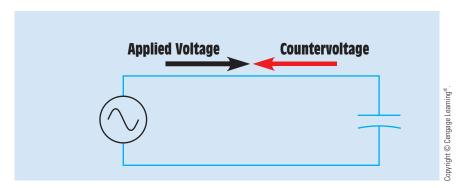
FIGURE 21-4 Countervoltage limits the flow of current.
