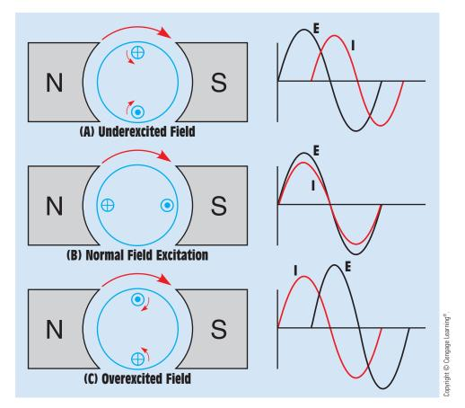
FIGURE 33-55 Field excitation in a synchronous motor.
