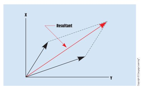
FIGURE 15–20 The parallelogram method of vector addition.
