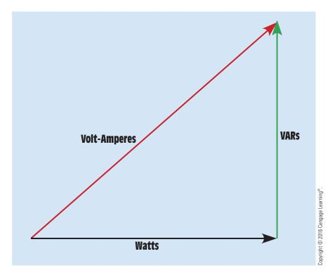
**FIGURE 19–7** Relationship of apparent power (volt-amperes), true power (watts), and reactive power (VARs) in an R-L parallel circuit.
