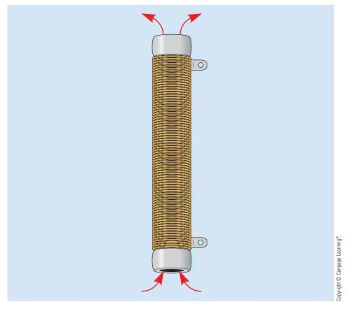
FIGURE 5-8 Airflow helps cool the resistor.
