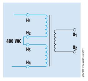
**FIGURE 28–24** Control transformer connected for 480-volt operation.
