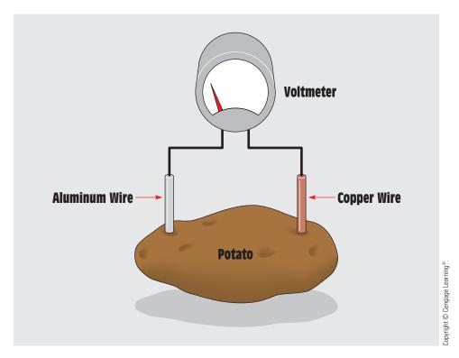
FIGURE 13–3 Simple voltaic cell constructed from a potato and two different metals.
