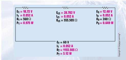
FIGURE 8–15 Missing values are found for the first part of the circuit.
