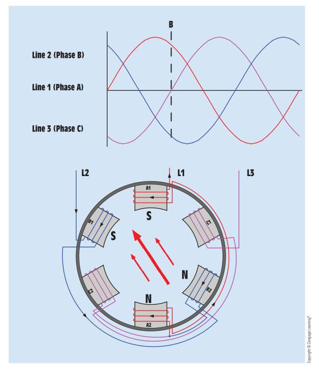
FIGURE 33-3 The magnetic field is concentrated between phases A and B.
