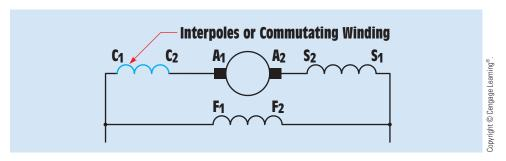
**FIGURE 30–50** Interpoles are connected in series with the armature.
