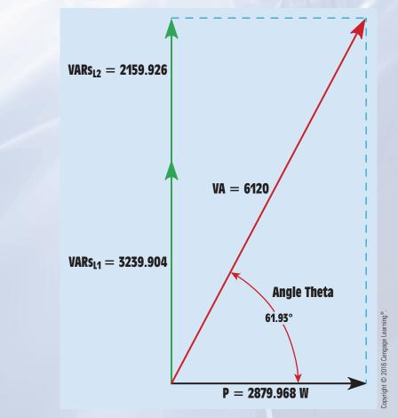
FIGURE 19–13 Angle theta determined by power vectors.
