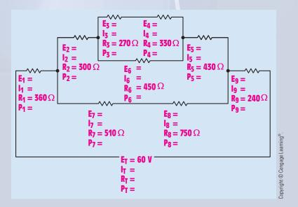
FIGURE 8–9 A complex combination circuit.
