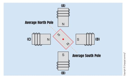
FIGURE 34–53 The magnet aligns with the average magnetic pole.
