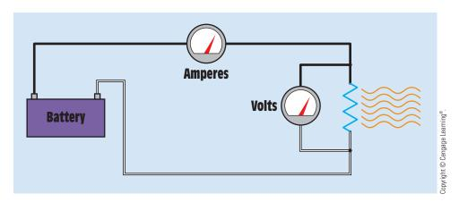
FIGURE 2-16 Amperes times volts equals watts.
