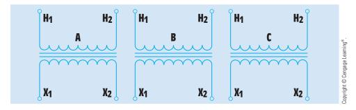
**FIGURE 29–9** Three single-phase transformers.
