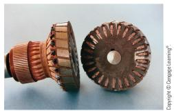
FIGURE 30–16B Cutaway view of an armature.
