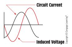
**FIGURE 17–12** Induced voltage is proportional to the rate of change of current.
