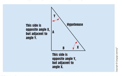
FIGURE 15-6 Determining opposite and adjacent sides.
