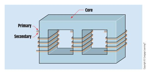
**FIGURE 29–1** Basic construction of a three-phase transformer.
