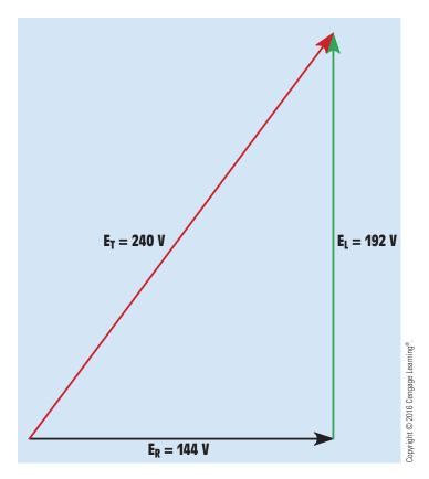
FIGURE 18-8 Relationship of resistive and inductive voltage drops in an R-L series circuit.
