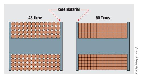
FIGURE 30-22 Square wire permits more turns than round wire in the same area.
