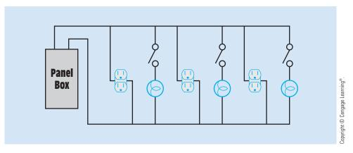
FIGURE 7-3 Lights and receptacles are connected in parallel.
