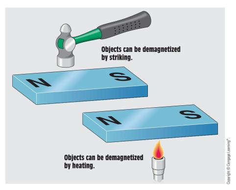
FIGURE 4–19 Other methods for demagnetizing objects.
