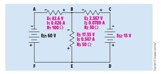
FIGURE 9-6 All circuit values have been calculated.
