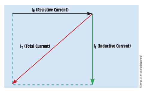
**Helpful Hint**: It should be noted that in an R-L parallel circuit, vectors cannot be used to plot the impedance because the values of resistance and inductive reactance do not add as they do in a series circuit.
