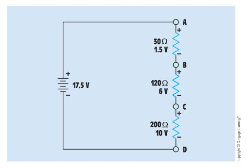
FIGURE 5–2 Resistors used as a voltage divider.
