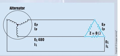
**FIGURE 27–19** Calculating three-phase values using a wye-connected power source and a delta-connected load (example circuit).
