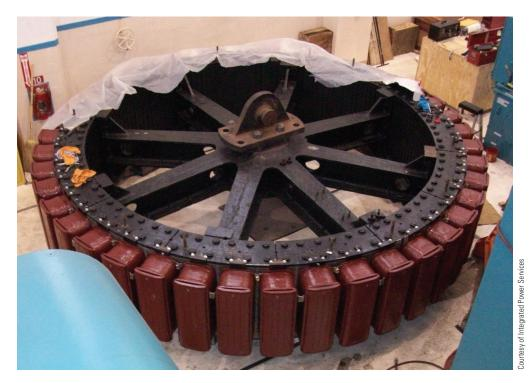
FIGURE 32–7 Rotor of the salient pole type.
