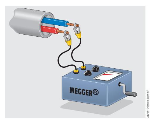
FIGURE 11–29 Testing for shorts with a MEGGER.
