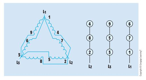
FIGURE 33–21 Low-voltage delta connection.
