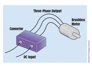
FIGURE 31-25 A converter changes DC into three-phase AC.
