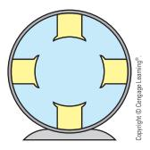
FIGURE 30-21 Pole pieces are constructed of soft iron and placed on the inside of the housing
