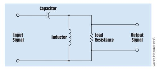
FIGURE 26–11 High-pass filters combining the effects of an inductor and a capacitor.
