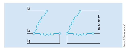
FIGURE 29-18 Open-delta connection.
