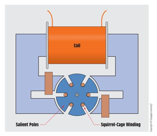
FIGURE 34-50 A Holtz motor.
