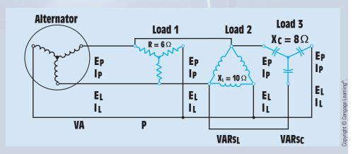
**FIGURE 27–22** Calculating three-phase values with a wye-connected source supplying power to a resistive, inductive, and capacitive load (example circuit).
