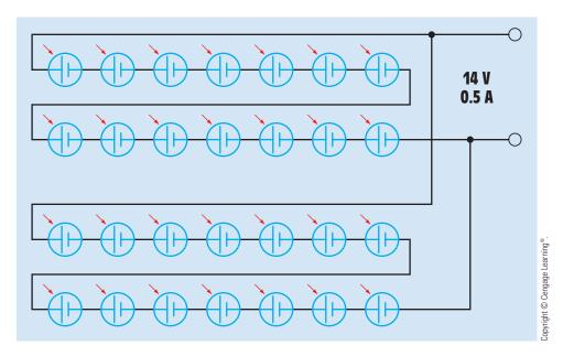
FIGURE 13–33 Series-parallel connection of solar cells.
