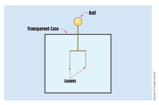
FIGURE 3-5 An electroscope.
