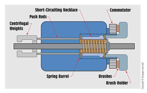
FIGURE 34–46 Brush-lifting-type repulsion-start induction-run motor.
