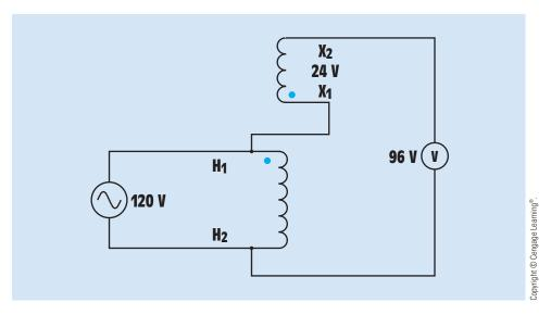
FIGURE 28-49 Polarity dots indicate subtractive polarity.
