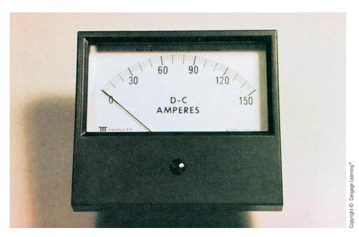
FIGURE 10-14 In-line ammeter.
