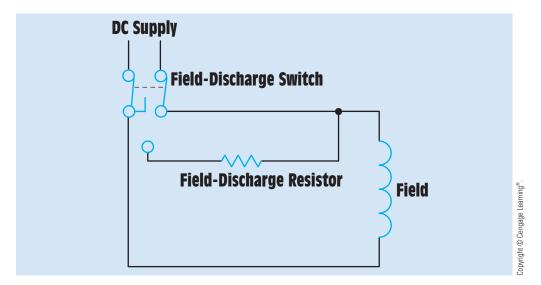
FIGURE 32-17 Switch in closed position.
