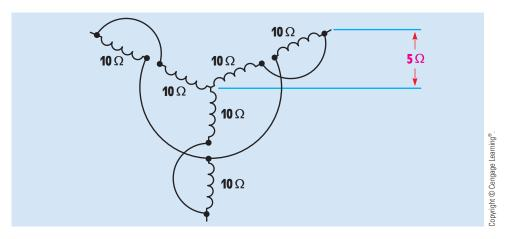
FIGURE 33-24 Impedance is less in parallel.
