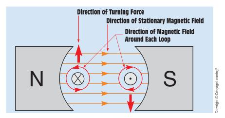
**FIGURE 31–2** Flux lines in the same direction repel each other, and flux lines in the opposite direction attract each other.
