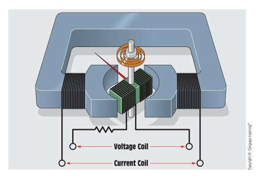
FIGURE 10-60 The wattmeter contains two coils—one for voltage and the other for current.
