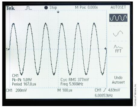
FIGURE 10-49 Display of a digital oscilloscope.
