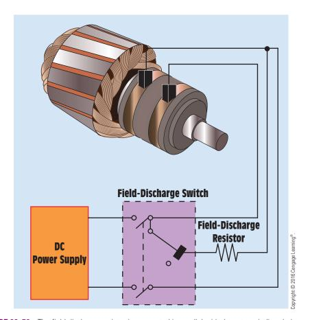
**FIGURE 33–53** The field-discharge resistor is connected in parallel with the rotor winding during starting.
