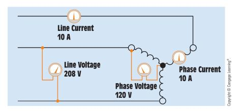
FIGURE 27-7 Line current and phase current are the same in a wye connection.
