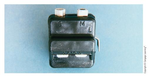
FIGURE 34-12 Solid-state starting relay.
