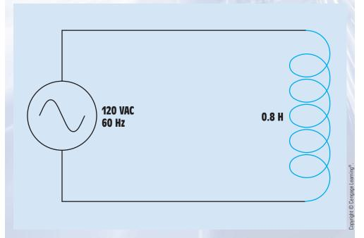
FIGURE 17–8 Circuit current is limited by inductive reactance.
