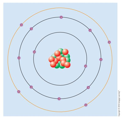
FIGURE 1–25 Semiconductors contain four valence electrons.
