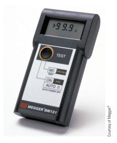
FIGURE 11–28 Battery-operated MEGGER.
