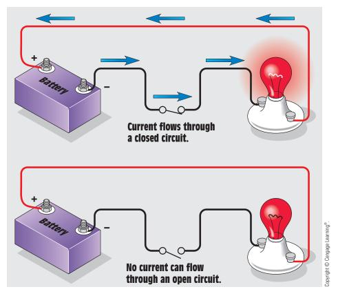
FIGURE 2-8 Current flows only through a closed circuit.
