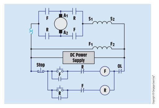
FIGURE 31–18 Forward-reverse control for a compound motor.
