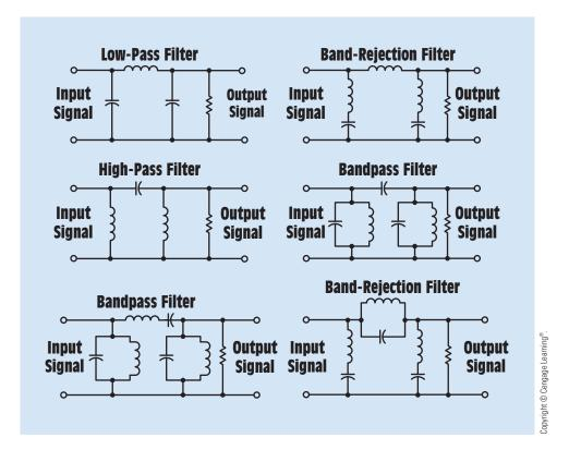
FIGURE 26–18 Basic Pl-type filters.
