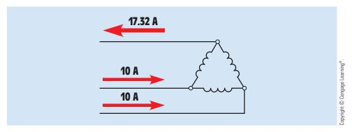
FIGURE 27-16 Division of currents in a delta connection.
