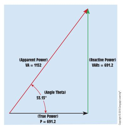
**FIGURE 18–14** The angle theta is the relationship of true power to apparent power.
