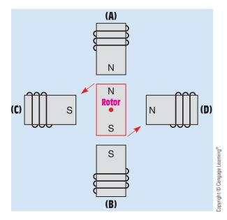
**FIGURE 34–51** The rotor could turn in either direction.
