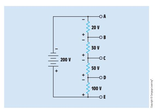
FIGURE 6-22 Series circuit used as a voltage divider.
