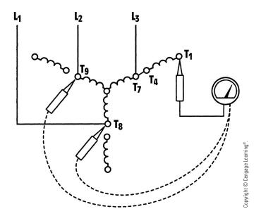
**FIGURE A–7**  $T_4$  connected to  $T_7$ .
