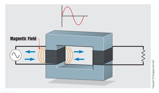
**FIGURE 28–7** Magnetic field produced by AC.
