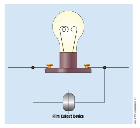
FIGURE 28-61 A film cutout device shorts and maintains the circuit if the lamp should fail.
