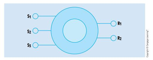
FIGURE 33-59 Schematic symbol for a selsyn motor.
