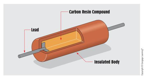
FIGURE 5–3 Composition carbon resistor.
