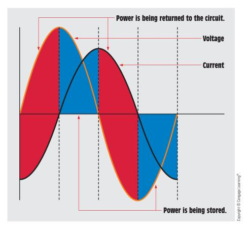
FIGURE 18–10 Power is stored and then returned to the circuit.
