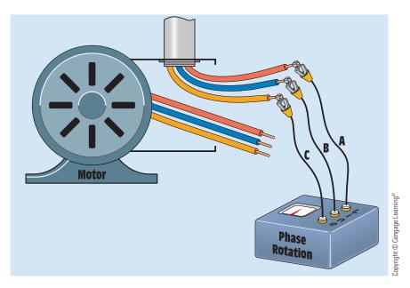
FIGURE 33-14 Connecting the phase rotation meter to the line.
