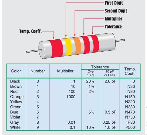
FIGURE 20–31 Color codes for ceramic capacitors.
