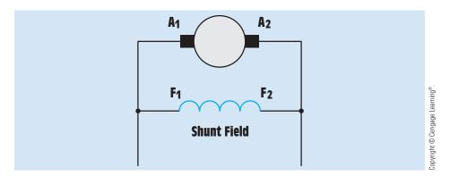
FIGURE 31–5 The shunt motor has the shunt field connected in parallel with the armature.
