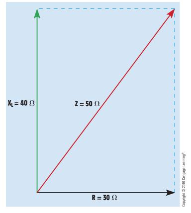
**FIGURE 18–5** Finding the impedance of the circuit using the parallelogram method of vector addition.
