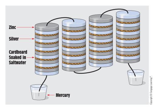
FIGURE 13-1 A voltaic pile.
