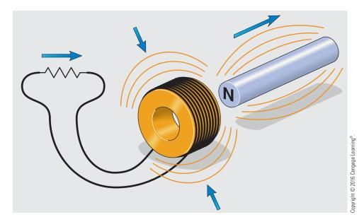
FIGURE 14–12 The induced voltage forces current to flow in the opposite direction.
