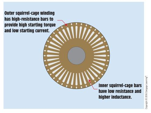
FIGURE 33–37 Double-squirrel-cage rotor used in NEMA design code C motors.
