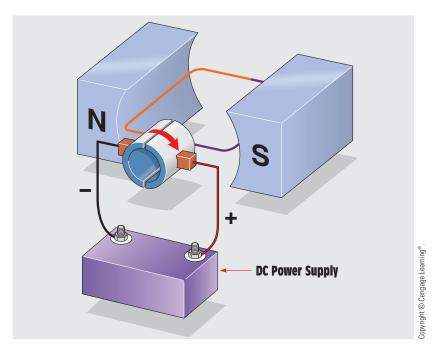
FIGURE 31-1 DC is supplied to the loop.
