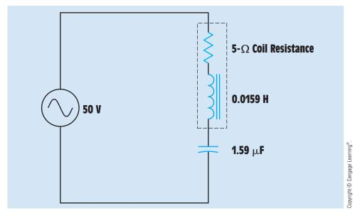
FIGURE 24-9 LC series circuit.
