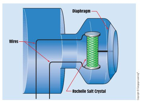
FIGURE 1–28 Producing sound with electricity.
