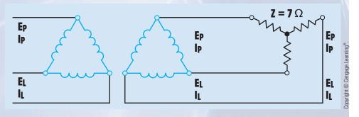
**FIGURE 29–16** Example circuit 2 three-phase transformer calculation.
