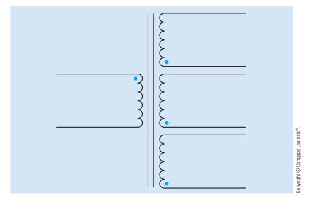
FIGURE 28-45 Polarity marks for multiple secondaries.
