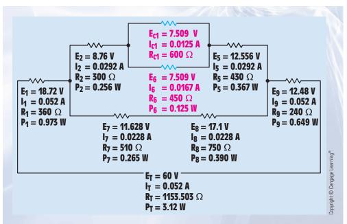
**FIGURE 8–19** The values of  $R_{c1}$  and  $R_{6}$ .
