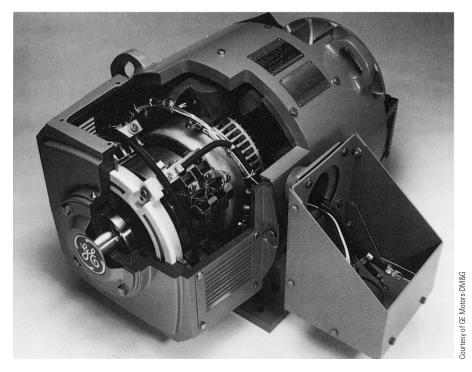
FIGURE 30-53 Exposed view of a DC machine.
