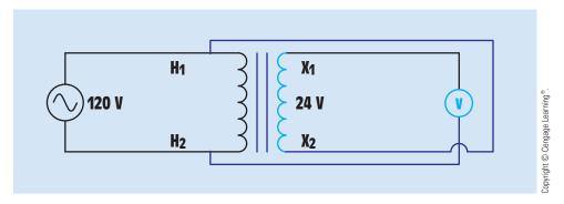
FIGURE 28–46 Connecting the secondary and primary windings forms an autotransformer.
