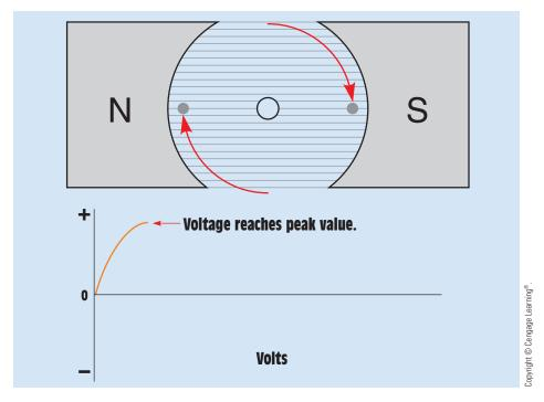
FIGURE 30-3 Induced voltage after 90° of rotation.
