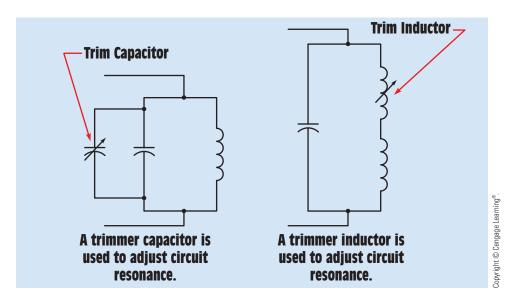
**FIGURE 26–1** Trimmer capacitors and trimmer inductors are used to overcome tolerance differences in capacitors and inductors.
