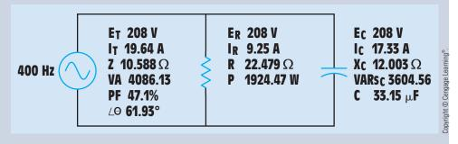
FIGURE 23–11 Example Circuit 2 with completed values.
