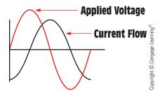
FIGURE 17-14 The current lags the applied voltage by 90°.
