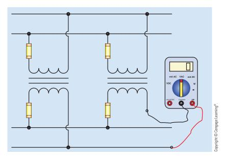
FIGURE 28-66 Checking the polarity of a parallel transformer connection.
