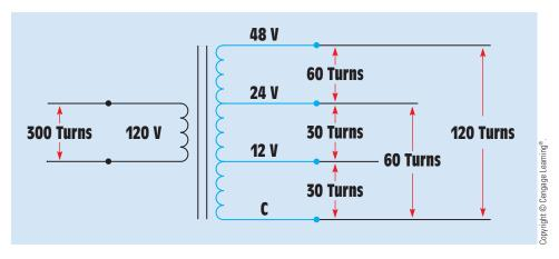
FIGURE 28–13 Transformer secondary with multiple taps.
