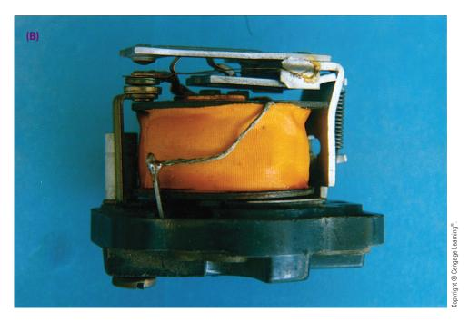
FIGURE 34–29A AND B Potential starting relays.
