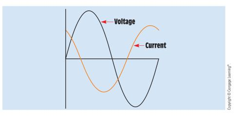
FIGURE 22-7 The current leads the voltage by 53.13°.
