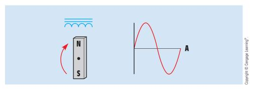
FIGURE 27–3 Producing a single-phase voltage.
