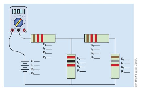
FIGURE 8-24 Combination circuit.
