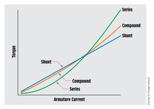
FIGURE 31-9 Torque curves of DC motors.
