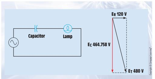
FIGURE 22–12 Determining voltage drop across the capacitor.
