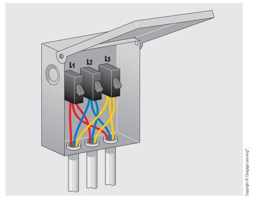
**FIGURE 11–26** Each conduit contains a conductor from each phase. This permits the magnetic fields to cancel each other.
