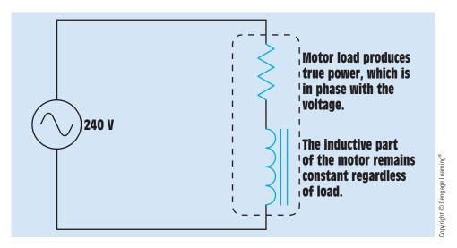
FIGURE 25-16 Equivalent motor circuit.
