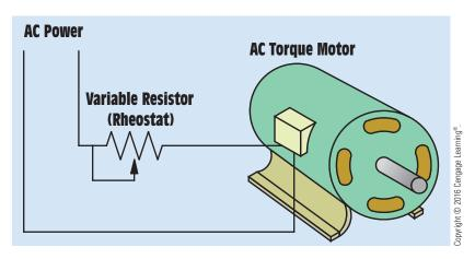
FIGURE 34-76 A high-wattage variable resistor is connected in series with the torque motor.
