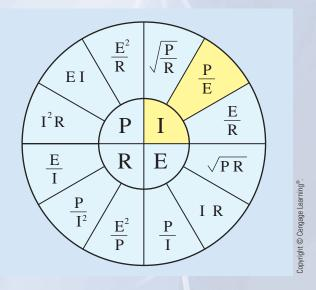
FIGURE 2–22 Finding current when power and voltage are known.
