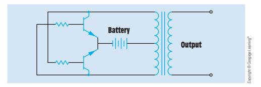
FIGURE 16-4 Square wave oscillator.
