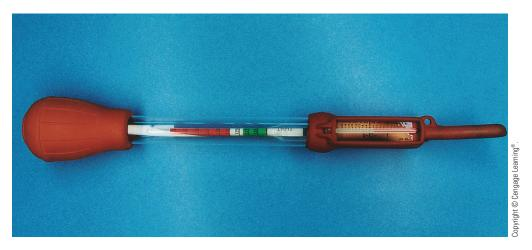
FIGURE 13–19 Hydrometer.
