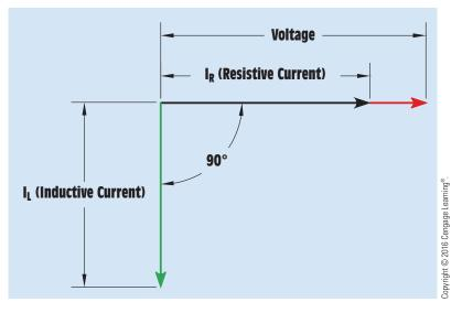
**FIGURE 19–3** Resistive and inductive currents are  $90^{\circ}$  out of phase with each other in an R-L parallel circuit.
