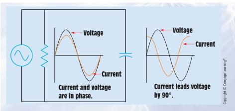
FIGURE 23–3 Phase relationship of current and voltage in an RC parallel circuit.
