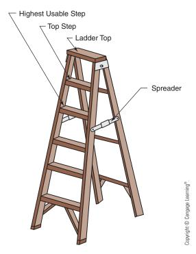
FIGURE S-16 Typical step ladder.
