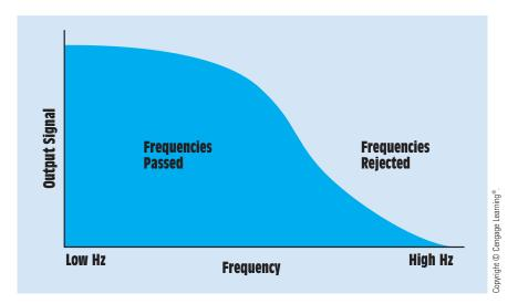
FIGURE 26-4 Low-pass filters pass low frequencies and reject high frequencies.
