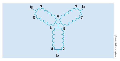
FIGURE 33–18 Stator windings connected in parallel.
