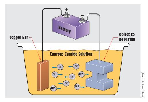
**FIGURE 12–5** The electroplating process.
