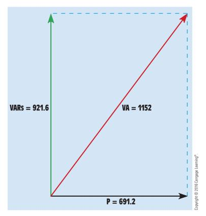
**FIGURE 18–13** Using the parallelogram method to plot the relationship of volt-amperes, watts, and VARs.
