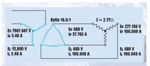
FIGURE 29–15 Example circuit 1 with all missing values.
