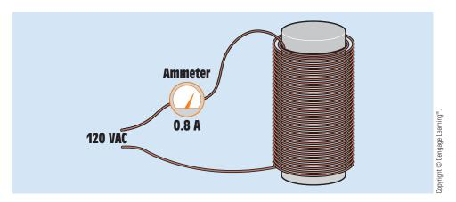
FIGURE 17–6 Measuring circuit current with an ammeter.
