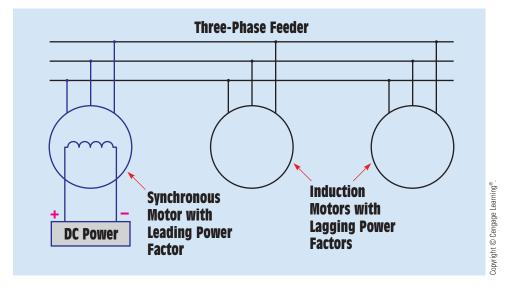
FIGURE 33–56 Synchronous motor used to correct the power factor of other motors.
