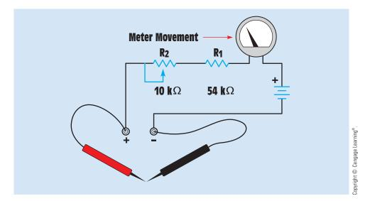
FIGURE 10-36 Basic series ohmmeter.
