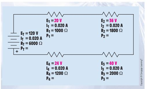
FIGURE 6-15 Voltage drops across each resistor.
