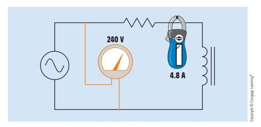
**FIGURE 18–11** Apparent power is the product of measured values (240 V  $\times$  4.8 A = 1152 VA).
