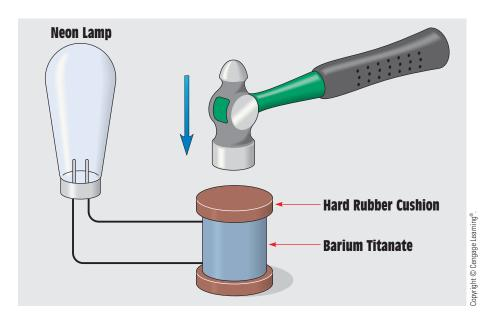
FIGURE 13–38 Voltage produced by piezoelectric effect.
