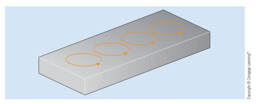
FIGURE 11–24 Eddy currents are currents induced in metals.
