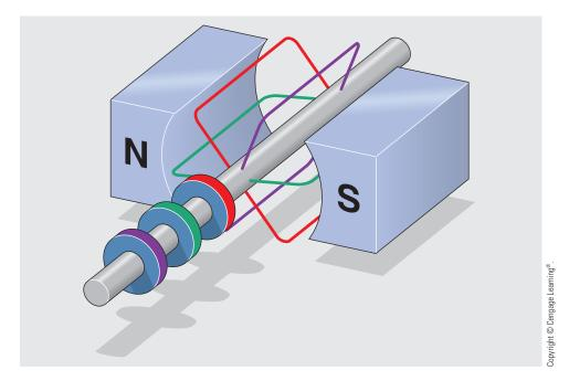
FIGURE 32–2 The armature conductors rotate inside a magnetic field.
