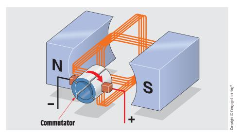
FIGURE 31–3 Increasing the number of loops and turns increases the torque.
