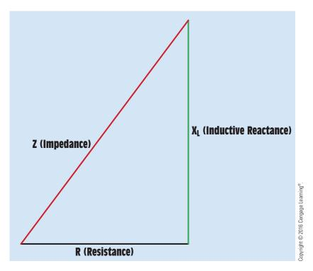
**FIGURE 18–3** Impedance is the combination of resistance and inductive reactance.
