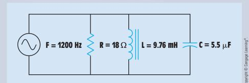
FIGURE 25-7 Example circuit.
