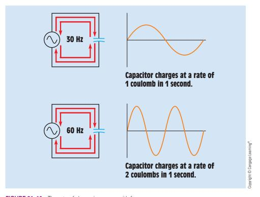
FIGURE 21–10 The rate of charge increases with frequency.
