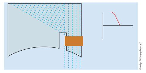
FIGURE 34–34 The shading coil opposes a change of flux when the current decreases.
