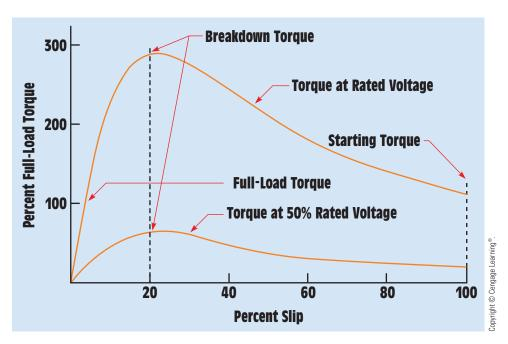
FIGURE 33–33 Typical torque curves for a squirrel-cage motor.
