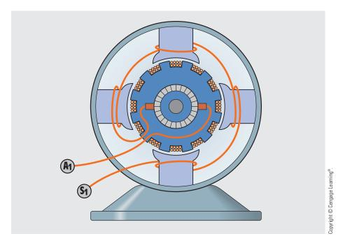
FIGURE 30–27 The series field is connected in series with the armature.
