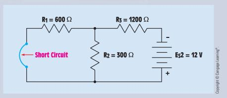
**FIGURE 9–24** Voltage source E<sub>s</sub>2 is shorted.
