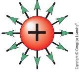
**FIGURE 1–7** The lines of force extend outward.
