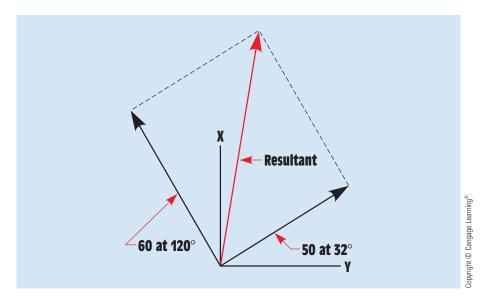
FIGURE 15–21 The parallelogram method of vector addition, second example.
