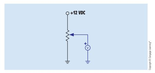
FIGURE 5–18 Variable resistor used as a potentiometer.
