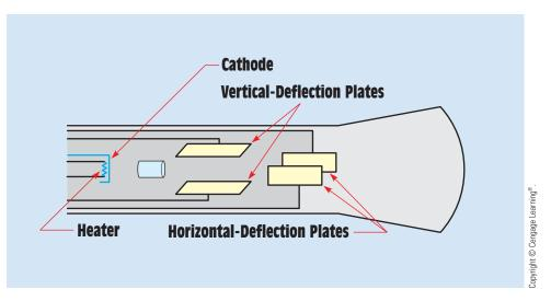
FIGURE 12-12 Cathode ray tube.
