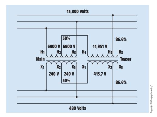
FIGURE 29–26 T-connected transformers.
