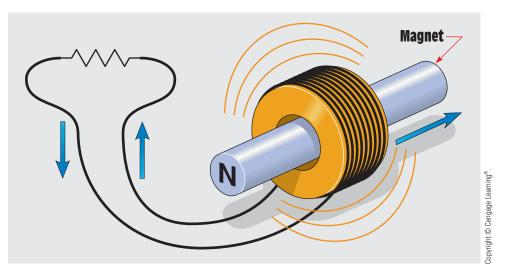
FIGURE 14-9 An induced current produces a magnetic field around the coil.
