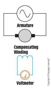
**FIGURE 34–67** Using the compensating winding to set the brushes to the neutral plane position.
