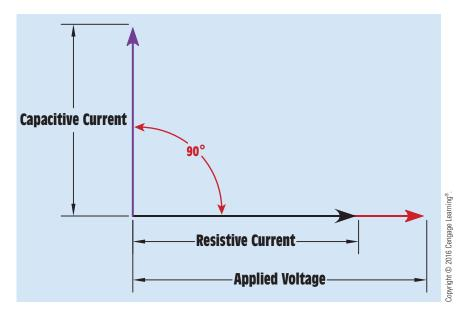
**FIGURE 23–1** Current flow through the capacitor is 90° out of phase with both the current flow through the resistor and the applied voltage.
