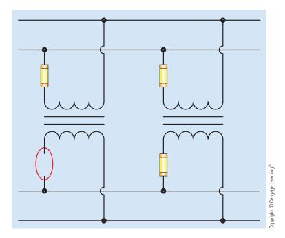
**FIGURE 28–67** The secondary winding should be disconnected before disconnecting the primary winding.
