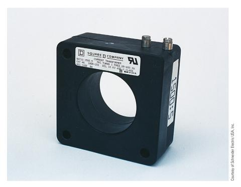
FIGURE 10–26 A toroid current transformer.
