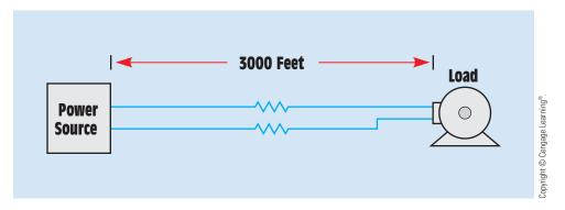
FIGURE 11–13 Long wire runs have the effect of adding resistance in series with the load.
