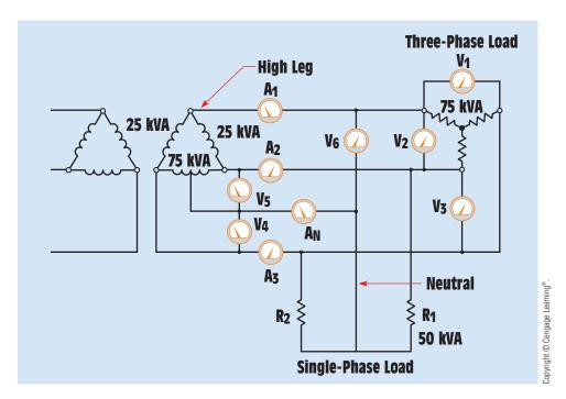
FIGURE 29–22 Closed-delta connection with high leg.
