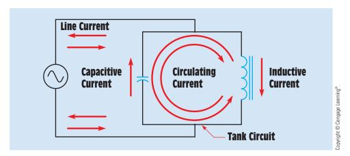
**FIGURE 25–9** The amount of current circulating inside the tank is equal to the product of the line current and the Q of the circuit.
