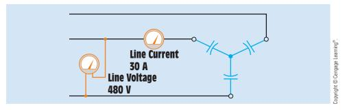
FIGURE 27–18 Pure capacitive three-phase load.
