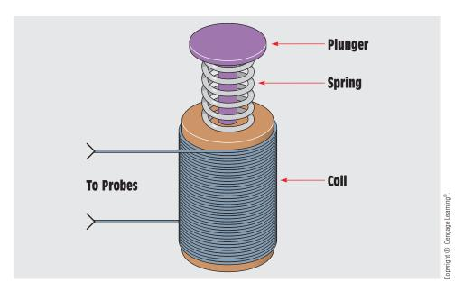
FIGURE 10-43 Low-impedance voltage tester.
