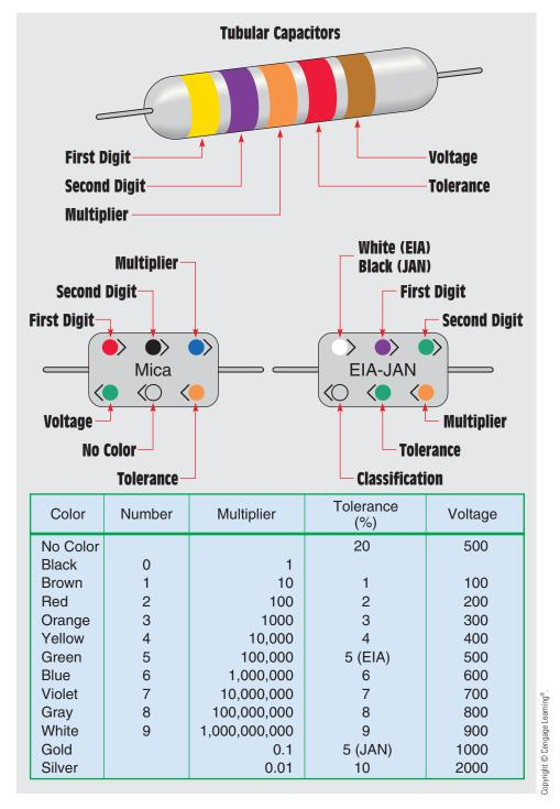
FIGURE 20–30 Identification of mica and tubular capacitors.
