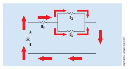
FIGURE 8-1 A simple combination circuit.
