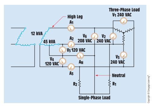
FIGURE 29-20 Three-phase open-delta transformer supplying both three-phase and single-phase loads.
