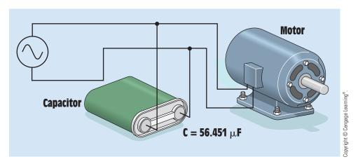
**FIGURE 25–19** The capacitor corrects the power factor to 95%.
