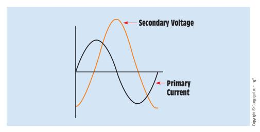
**FIGURE 28–55** The secondary voltage lags the primary current by 90°.
