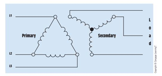
FIGURE 29–6 Delta–wye connected three-phase transformer.
