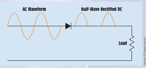
FIGURE 16–15 A half-wave rectifier converts only one half of the AC waveform into DC.
