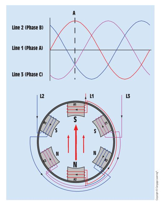
FIGURE 33-2 The magnetic field is concentrated between poles A1 and A2.
