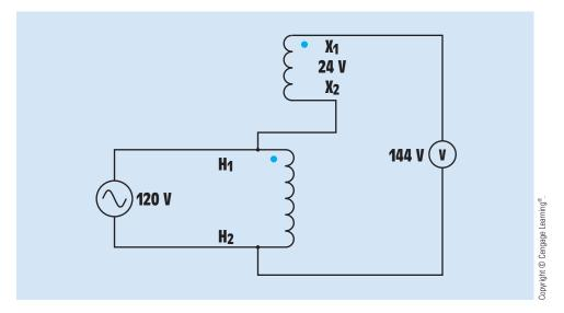
FIGURE 28-48 Placing polarity dots to indicate additive polarity.
