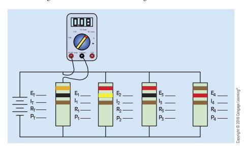
FIGURE 7-26 Parallel circuit.
