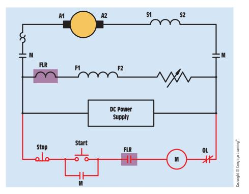
FIGURE 31–22 The field loss relay disconnects power to the armature if shunt field current stops.
