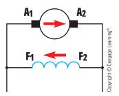
**FIGURE 30–34** Residual magnetism in the pole pieces produces an initial voltage, which causes current to flow through the shunt field and the field flux to increase.
