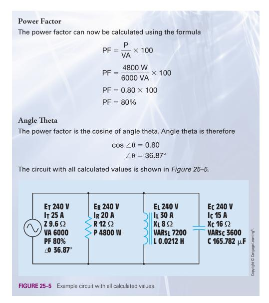
The phase angle relationship of voltage and current is shown in *Figure 25–6*. Because the circuit has more inductive VARs than capacitive VARs, the current lags the voltage by 36.87°.
