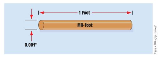
**FIGURE 11–15** A mil-foot is equal to a piece of wire one foot long and one thousandth of an inch in diameter.
