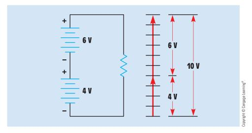
FIGURE 15–14 Adding scalars in the same direction.
