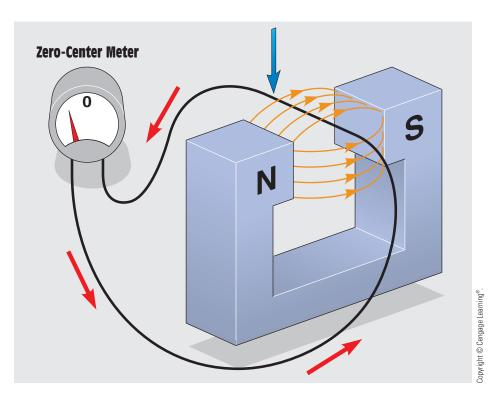
FIGURE 14-2 Voltage is induced when a conductor cuts magnetic lines of flux.
