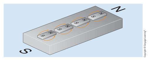
FIGURE 11–25 The molecules reverse direction each time the magnetic field changes direction.
