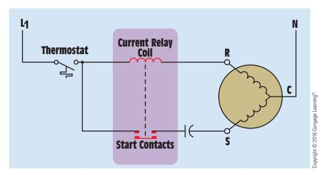
FIGURE 34-11 Current relay connection.
