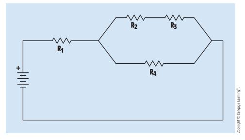
FIGURE 8-21 Series-parallel circuit.
