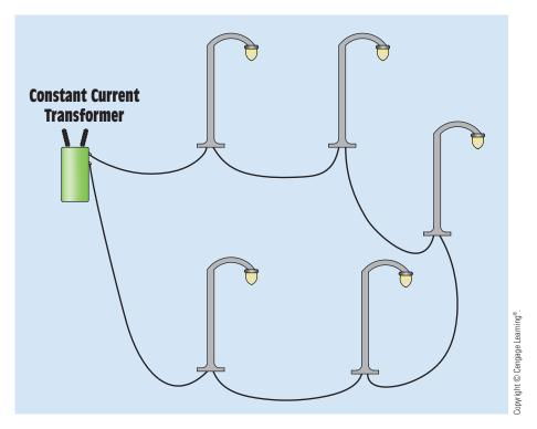
FIGURE 28-59 Street lamps are often connected in series.
