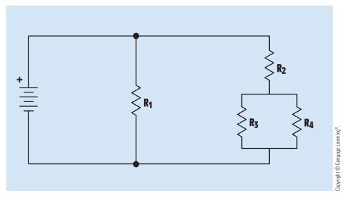
FIGURE 8-22 A parallel-series circuit.
