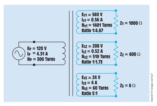
FIGURE 28–16 The transformer with all calculated values.
