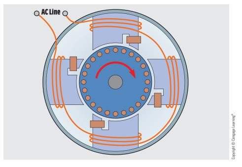
FIGURE 34-36 Four-pole shaded-pole induction motor.
