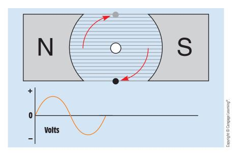
FIGURE 30-6 Voltage produced after 360° of rotation.
