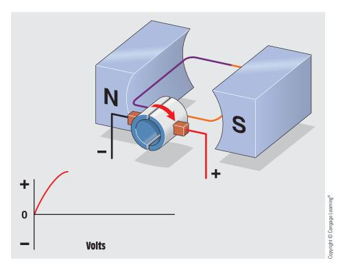
FIGURE 30-9 The loop has rotated 90°.
