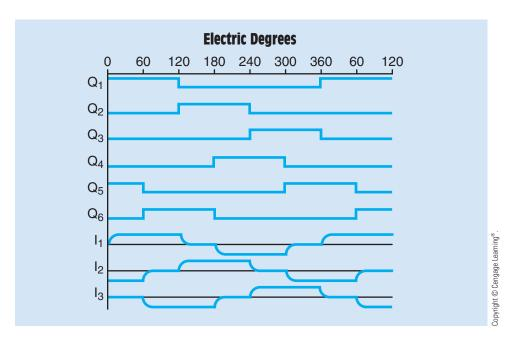
FIGURE 31–29 Converter commutation sequence.
