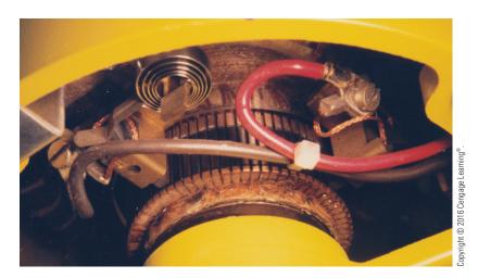
FIGURE 30-20 Brushes make contact with segments of the commutator.
