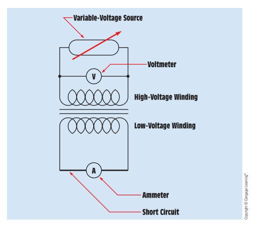
FIGURE 28–58 Determining transformer impedance.
