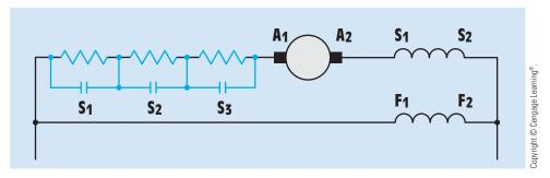
FIGURE 31-19 Resistors limit armature current.
