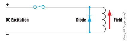
FIGURE 32-19 Normal current flow.
