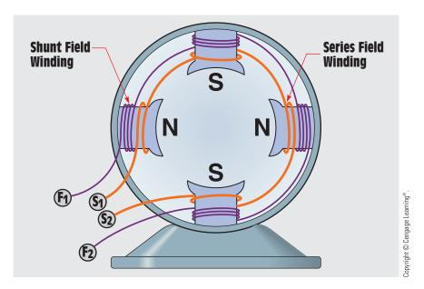
FIGURE 30-25 Both series and shunt field windings are contained on each pole piece.
