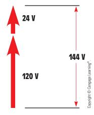
FIGURE 28–51 The values of the arrows add to indicate additive polarity (boost connection).
