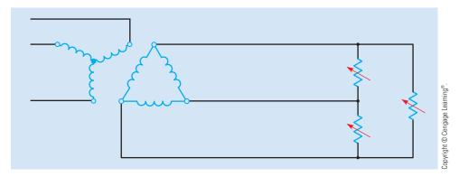
FIGURE 29–23 Single-phase loads supplied by a wye-delta transformer connection.
