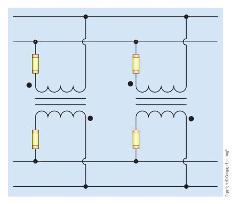
**FIGURE 28–65** Transformers are sometimes connected in parallel to increase the current capacity of the circuit.
