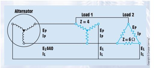
**FIGURE 27–21** Calculating three-phase values using a wye-connected source and two three-phase loads (example circuit).
