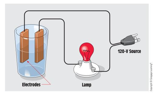
FIGURE 12-3 Conduction in a liquid.
