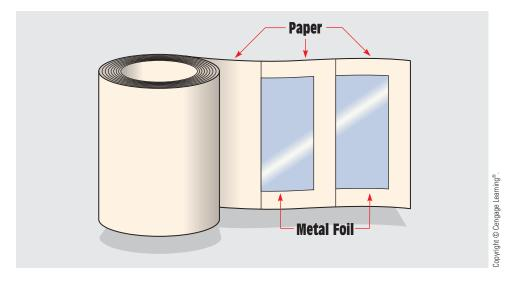
FIGURE 20-19 Oil-filled paper capacitor.
