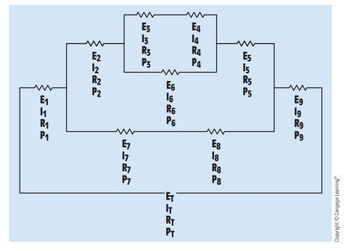
FIGURE 8-23 A combination circuit.
