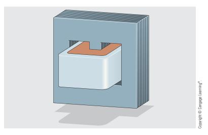
FIGURE 28–30 A shell-type transformer.
