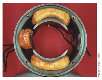
FIGURE 30-26 A two-pole DC machine with one interpole.
