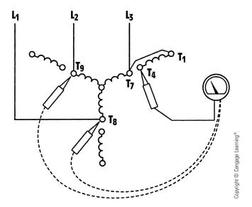
**FIGURE A–6**  $T_1$  connected to  $T_7$ .
