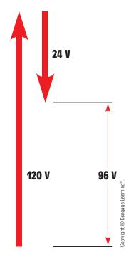
FIGURE 28-53 The values of the arrows subtract (buck connection).
