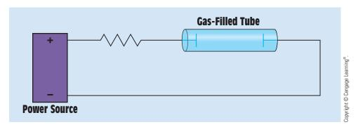
FIGURE 12-8 Conduction in a gas.
