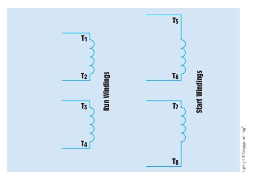
FIGURE 34–19 Dual-voltage windings for a split-phase motor.
