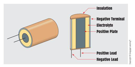
FIGURE 20-24 Wet-type electrolytic capacitor.
