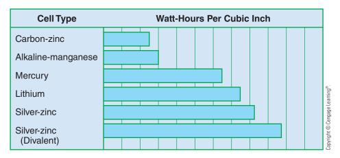
FIGURE 13-15 Watt-hours per cubic inch for different types of cells.
