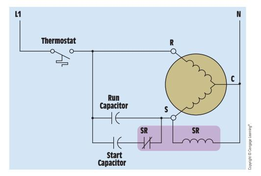
FIGURE 34–30 Potential relay connection.
