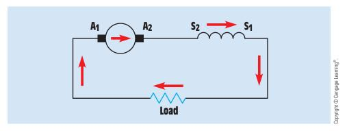
**FIGURE 30–29** Residual magnetism produces an initial voltage used to provide a current flow through the load.
