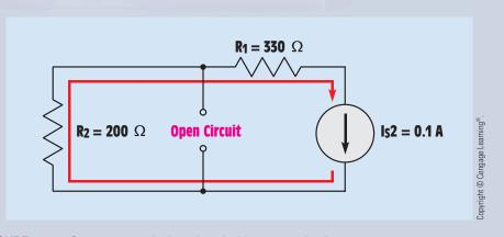
**FIGURE 9–31** Current source  $I_S1$  is replaced with an open circuit.
