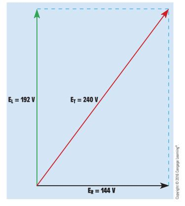
**FIGURE 18–9** Graphic representation of voltage drops using the parallelogram method of vector addition.
