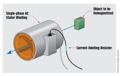
FIGURE 4-18 Demagnetizing an object.
