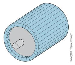
FIGURE 34-43 Axial commutator.
