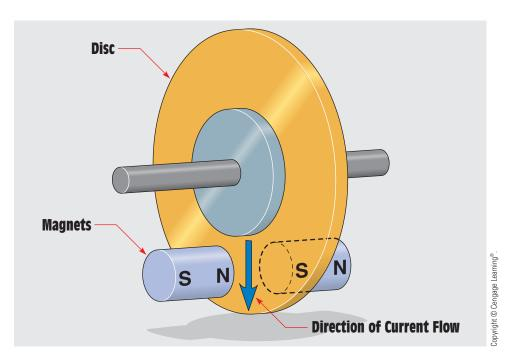
FIGURE 31-33 Basic construction of a ServoDisc motor.
