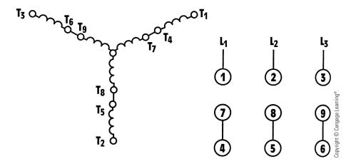
FIGURE A-3 High-voltage connection.
