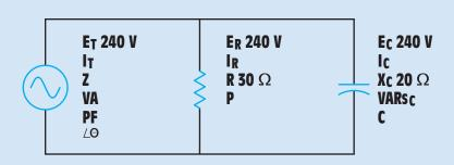
FIGURE 23–2 Resistive-capacitive parallel circuit.
