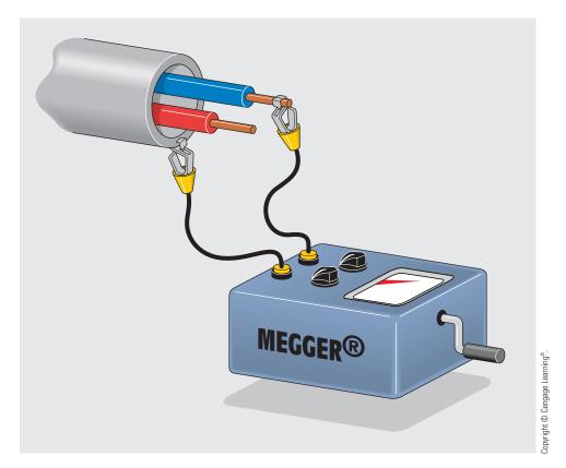
FIGURE 11–30 Testing for grounds with a MEGGER.
