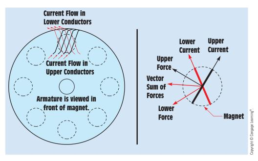
FIGURE 31–35 A force tangent to the magnet is produced.
