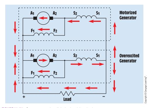
FIGURE 30–56 One generator takes all the load, and the other becomes a motor.
