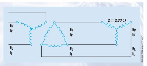
FIGURE 29-14 Example Circuit 1 three-phase transformer calculation.
