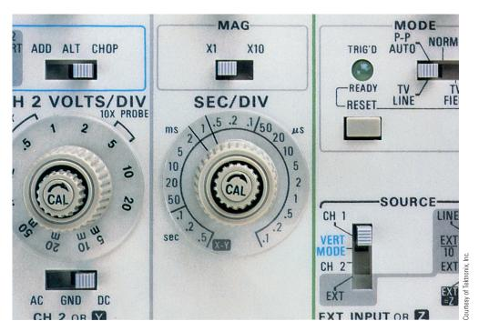
**FIGURE 10–53** Time base of an analog oscilloscope.
