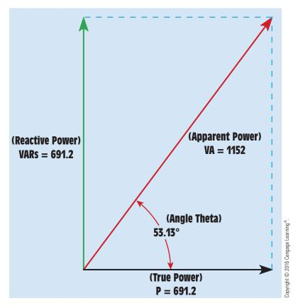
FIGURE 18-15 The angle theta can be found using vectors provided by the parallelogram method.
