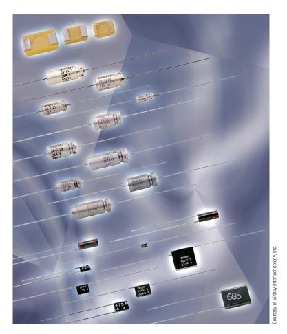
FIGURE 20–23 Polarized capacitors.
