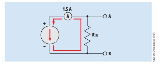
**FIGURE 9–14** The current source supplies a continuous 1.5 amperes.
