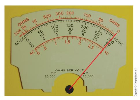
FIGURE 10–37 Adjusting the ohmmeter to zero.
