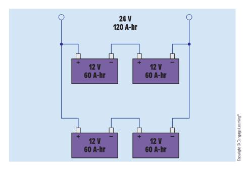
FIGURE 13–30 Series-parallel connection.
