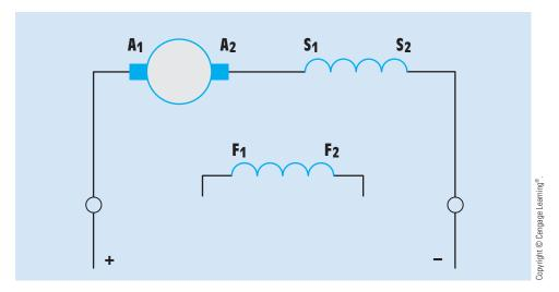
FIGURE 31-11 The motor is first connected as a series motor.
