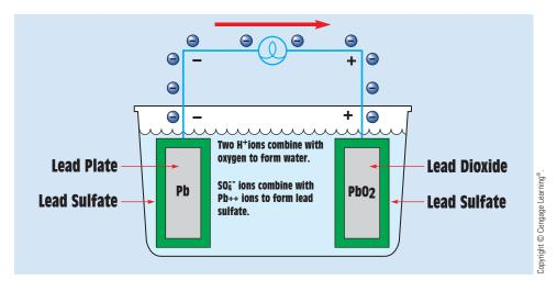
FIGURE 13–20 Discharge cycle of a lead-acid cell.
