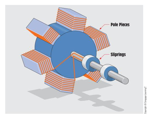
FIGURE 32–6 The rotor contains pole pieces that become electromagnets.
