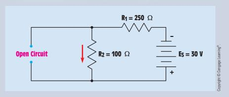
FIGURE 9–27 The current source is replaced with an open circuit.
