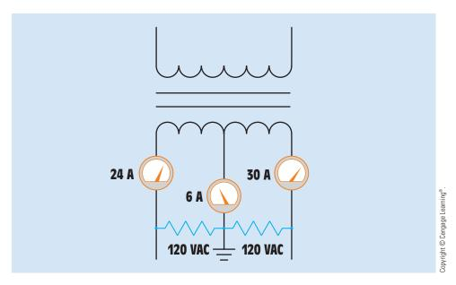
FIGURE 28-21 The neutral carries the sum of the unbalanced load.
