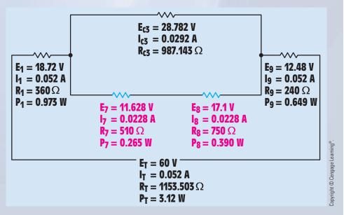
**FIGURE 8–17** The values for  $R_7$  and  $R_8$ .
