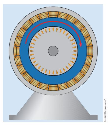
FIGURE 33–27 Voltage is induced into the rotor by the rotating magnetic field.
