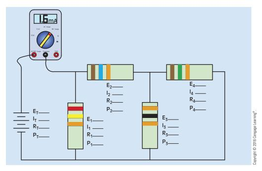
FIGURE 8-25 Combination circuit.
