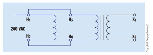
FIGURE 28–23 Control transformer connected for 240-volt operation.
