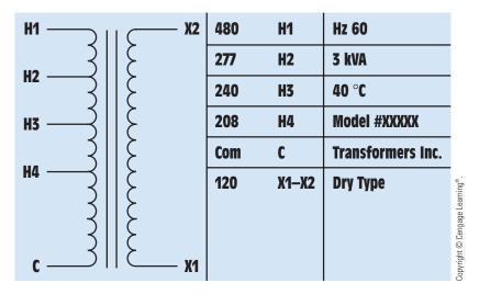
FIGURE 28-68 Transformer nameplate.
