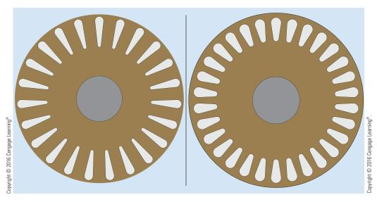
**FIGURE 33–35** Type B–E rotor used in NEMA code B motors.
