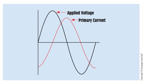
FIGURE 28-54 At no load, the primary current lags the voltage by 90°.
