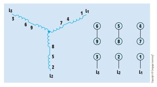
FIGURE 33–16 High-voltage wye connection.
