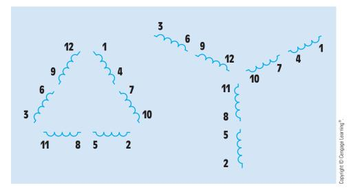
FIGURE 33–22 A 12-lead motor.
