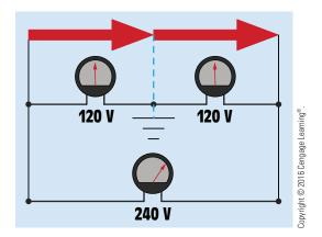
FIGURE 28–19 The voltages across the secondary are in phase with each other.
