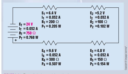
FIGURE 6–21 The applied voltage and the total resistance.
