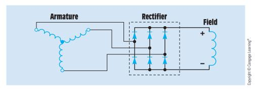
FIGURE 32-9 Basic brushless exciter circuit.
