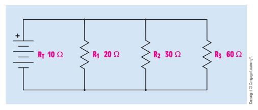
**FIGURE 7-7** Finding the total resistance of a parallel circuit by dividing the product of two resistors by their sum.
