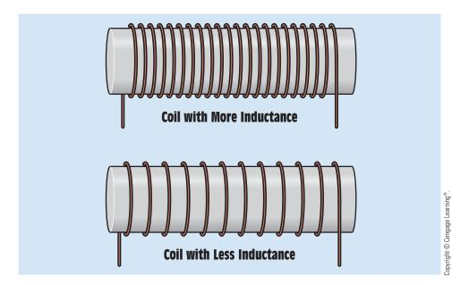
FIGURE 17-7 Coils with turns closer together produce more inductance than coils with turns farther apart.
