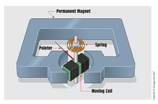
FIGURE 10-2 Basic d'Arsonval meter movement.
