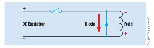
FIGURE 32-20 Induced current flow.
