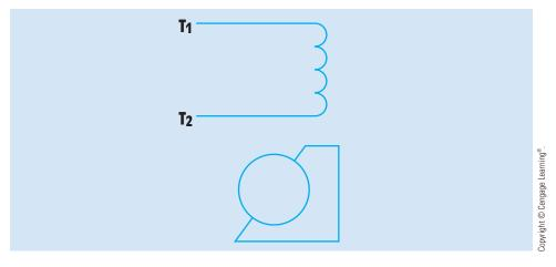
FIGURE 34-48 Schematic symbol for a repulsion motor.
