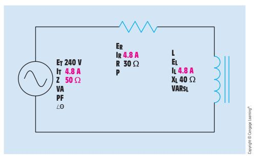
FIGURE 18-6 Total voltage divided by impedance equals total current.
