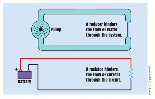
FIGURE 2–13 A resistor in an electric circuit can be compared to a reducer in a water system.
