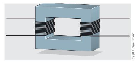
FIGURE 28-38 Isolation transformer.
