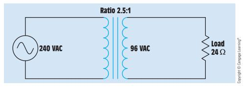
FIGURE 28–9 Calculating transformer values using the turns ratio.
