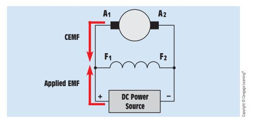
FIGURE 31–7 CEMF limits the flow of current through the armature.
