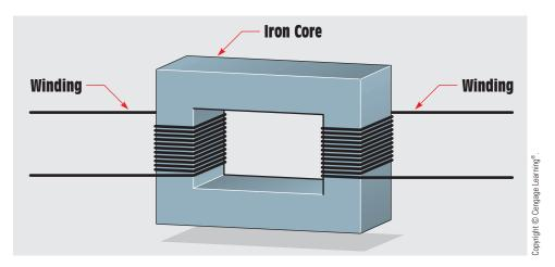
FIGURE 28-6 Basic construction of an isolation transformer.
