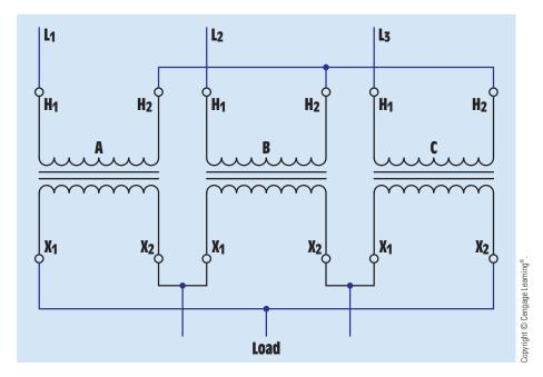
FIGURE 29–10 Connecting three single-phase transformers to form a wye-delta three-phase bank.
