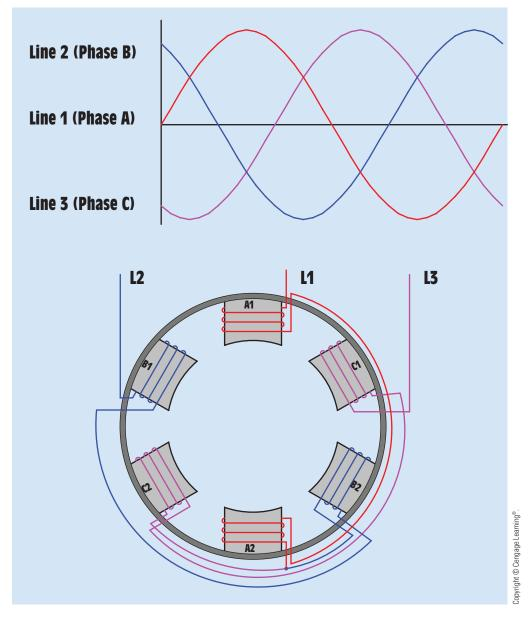
FIGURE 33–1 Three-phase stator and three sine wave voltages.
