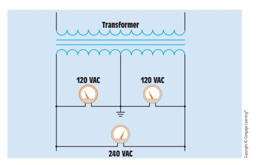
FIGURE 27–8 Single-phase transformer with grounded center tap.
