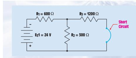
**FIGURE 9–21** Voltage source E<sub>s</sub>2 is replaced with a short circuit.
