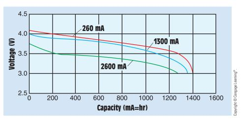
FIGURE 13–27 Typical discharge curves for lithium-ion cells.
