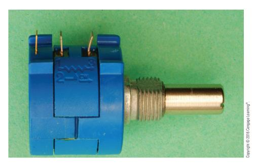
FIGURE 5-17 Multiturn variable resistor.
