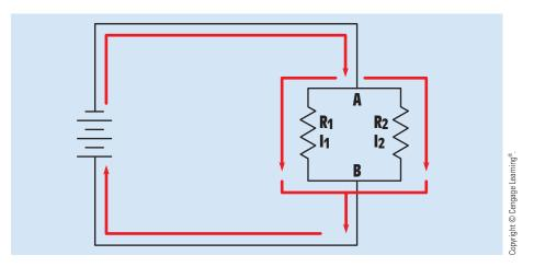
FIGURE 7–23 Parallel circuits are current dividers.
