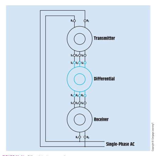
FIGURE 33–61 Differential selsyn connection.
