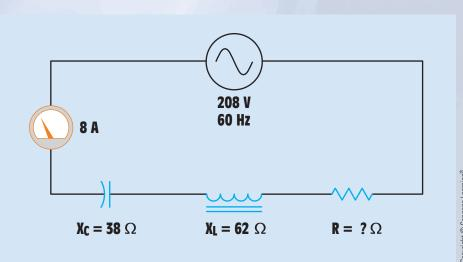
FIGURE 24-8 Example circuit.
