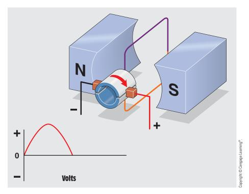
FIGURE 30–10 The loop has rotated 180°.
