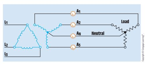
FIGURE 29–24 Three-phase four-wire connection.
