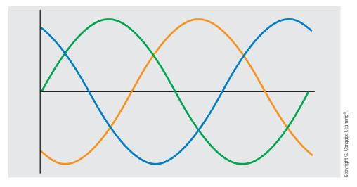
FIGURE 32-4 The alternator produces three sine wave voltages 120° out of phase with each other.
