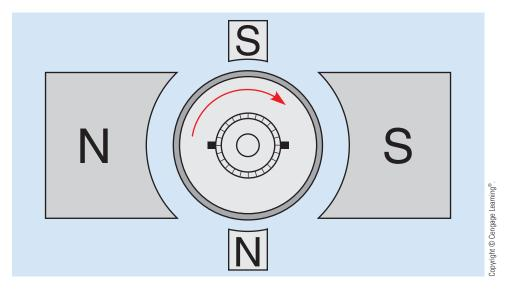
FIGURE 30-51 Interpoles must have the same polarity as the pole piece directly ahead of them.
