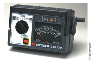
FIGURE 11-27 A hand-crank MEGGER.
