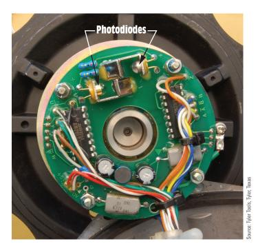
FIGURE 34-71 An encoder on the shaft of a servo motor.
