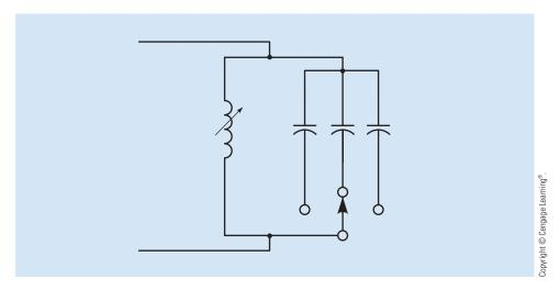
FIGURE 26–3 Broadband filter using multiple capacitors and a trimmer inductor.
