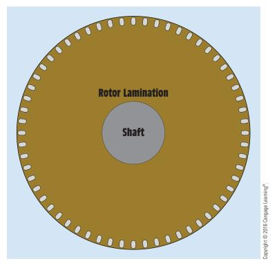
FIGURE 33-34 Type A rotor used in NEMA code D motors.
