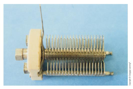
FIGURE 20–27 A variable capacitor.
