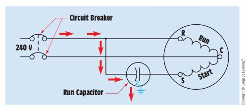
FIGURE 20–22 Identified terminal connected to the line (correct connections).
