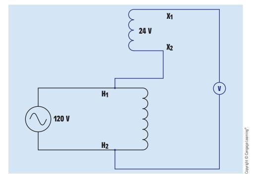
FIGURE 28-47 Redrawing the connection.
