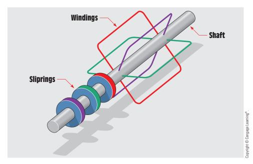
FIGURE 32–1 Basic design of a three-phase armature.
