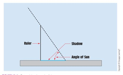
**FIGURE 15–9** Determining the angle of the sun.
