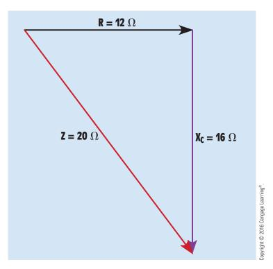
FIGURE 22–2 Resistance and capacitive reactance are 90° out of phase with each other.
