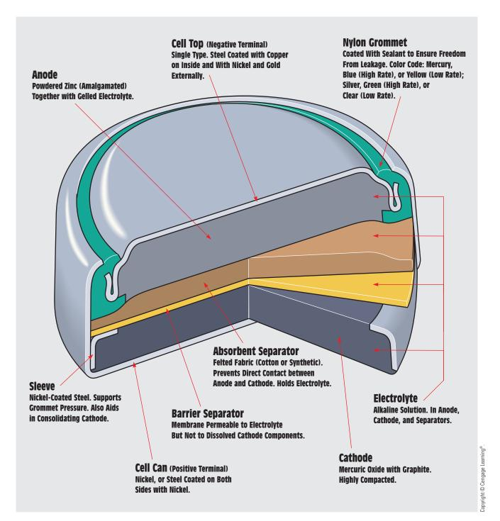
FIGURE 13-13 Mercury button cell.
