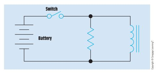
FIGURE 14–21 The resistor helps prevent voltage spikes caused by the inductor.
