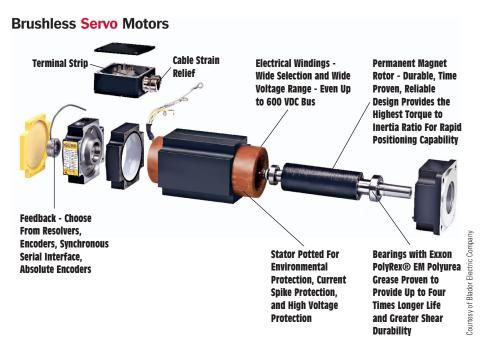
FIGURE 34–73 Exploded diagram of an AC servo motor.
