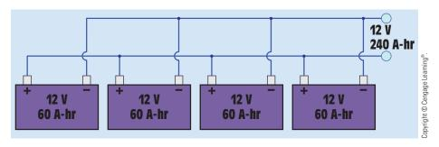
**FIGURE 13–29** When batteries are connected in parallel, their voltages remain the same and their ampere-hour capacities add.
