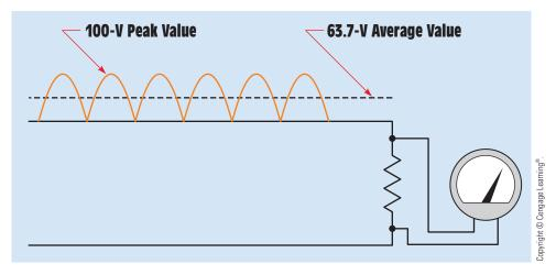
FIGURE 16–13 A DC voltmeter indicates the average value.
