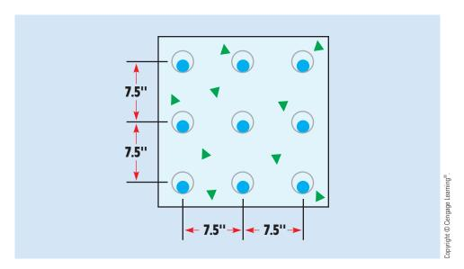
FIGURE 11-12 Electric duct banks.
