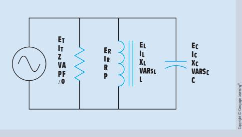
FIGURE 25-2 RLC parallel circuit.
