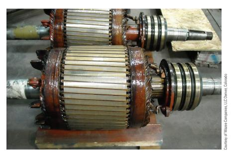
FIGURE 33–48 Rotors of wound-rotor induction motors.
