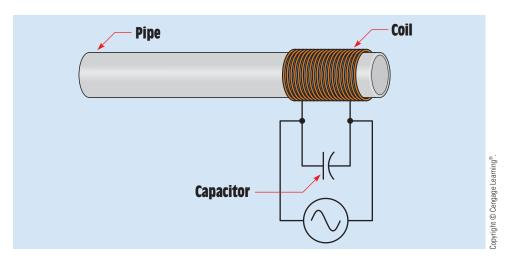
FIGURE 25–13 Induction heating system.
