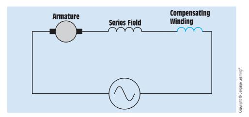
FIGURE 34-64 Conductive compensation.
