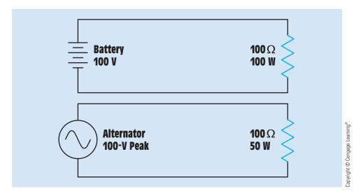
FIGURE 16-10 DC compared with a sine wave AC.
