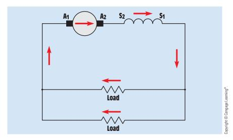
FIGURE 30–30 If more load is added, current flow and output voltage increase.
