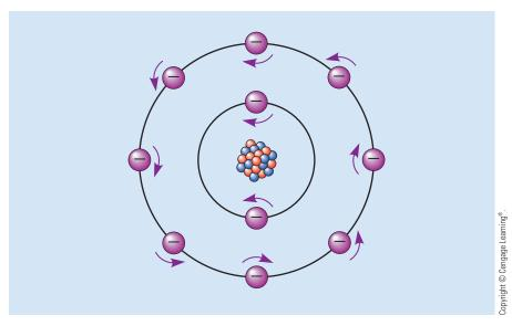
FIGURE 4–3 Electron pairs generally spin in opposite directions.
