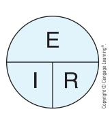
**FIGURE 2–18** Chart for finding values of voltage, current, and resistance.
