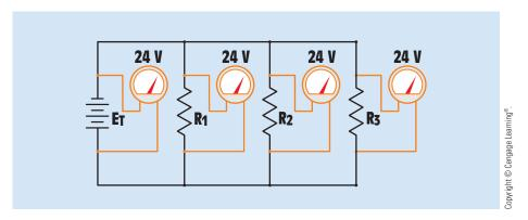
FIGURE 7-24 The voltage is the same across all branches of a parallel circuit.
