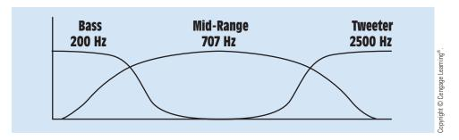
FIGURE 26–20 Filters direct the proper frequency to each speaker.
