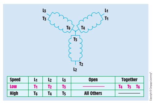
FIGURE 33–47 Low-speed parallel-wye connection.
