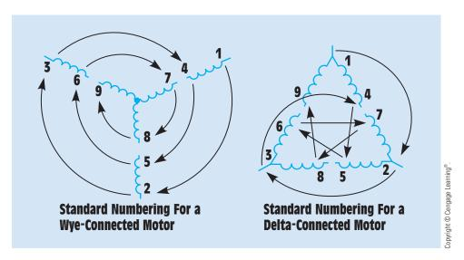
FIGURE 33–15 Standard numbering for three-phase motors.
