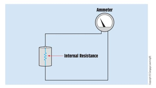
FIGURE 13–16 Short-circuit current is limited by internal resistance.
