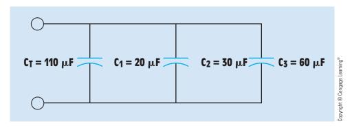
FIGURE 20-12 Capacitors connected in parallel.
