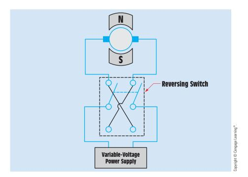
**FIGURE 31–31** PM motors can be reversed by reversing the polarity to the armature, and the speed can be controlled by variable voltage.
