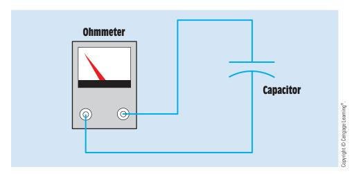
FIGURE 20–35 Testing the capacitor with an ohmmeter.
