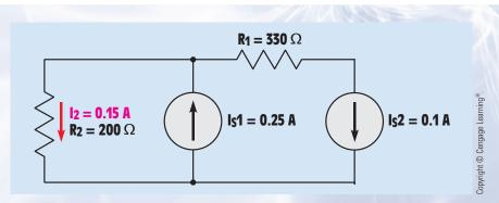
**FIGURE 9-32** The amount and the direction of current flow through  $R_2$  have been determined.
