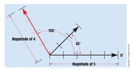
FIGURE 15–13 A third vector with a magnitude of 4 and a direction of 120° is added.
