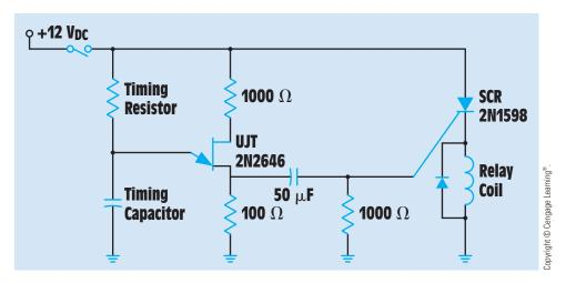
FIGURE 2-4 On-delay timer.
