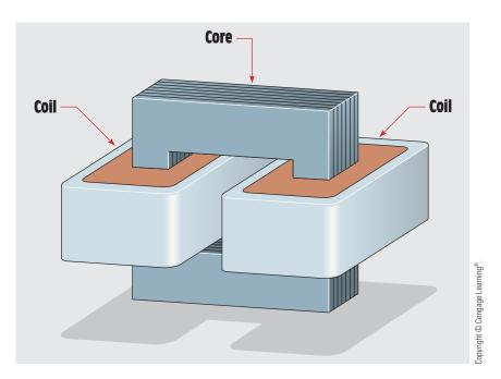
FIGURE 28–29 A core-type transformer.
