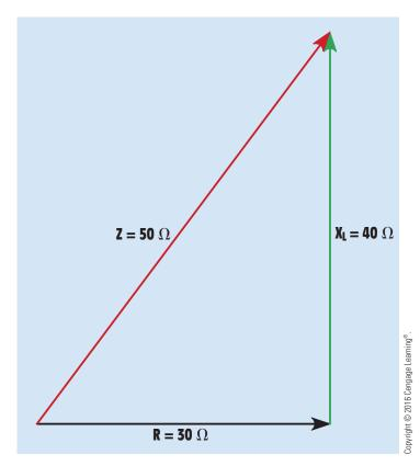
FIGURE 18-4 Determining impedance using vector addition.
