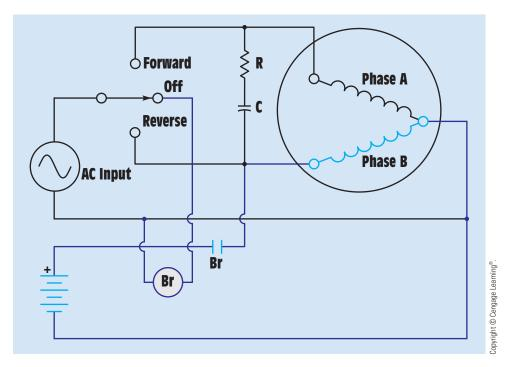
FIGURE 34-61 Applying DC voltage to increase holding torque.
