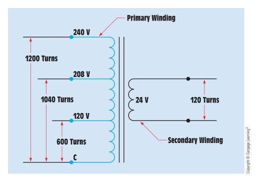
FIGURE 28–12 Transformer with multiple-tapped primary winding.
