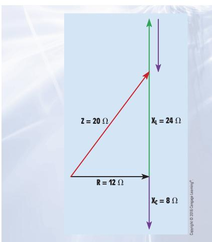
FIGURE 24-4 Right triangle formed by circuit impedance.
