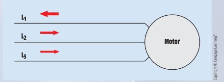
FIGURE 11-20 Current flows from lines 2 and 3 to line 1.
