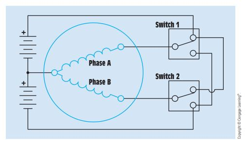
FIGURE 34–55 A standard three-lead motor.
