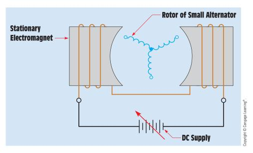
FIGURE 32–8 The brushless exciter uses stationary electromagnets.
