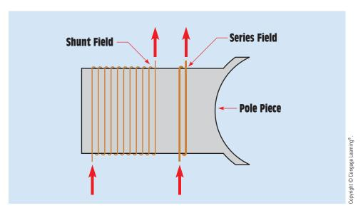
**FIGURE 30–45** In a cumulative-compound machine, the current flows in the same direction through both the series and the shunt field.
