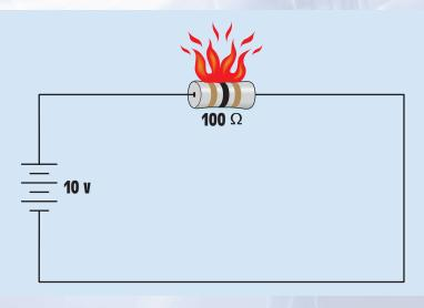
**FIGURE 5–13** Exceeding the power rating causes damage to the resistor.
