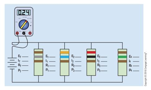
FIGURE 7-27 Parallel circuit.
