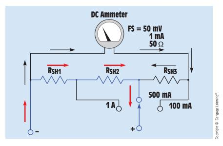
FIGURE 10-22 Current path through the meter and shunt for a full-scale value of 0.5 ampere.
