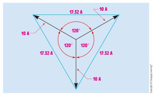
FIGURE 27-17 Vector addition is used to calculate the sum of the currents in a delta connection.
