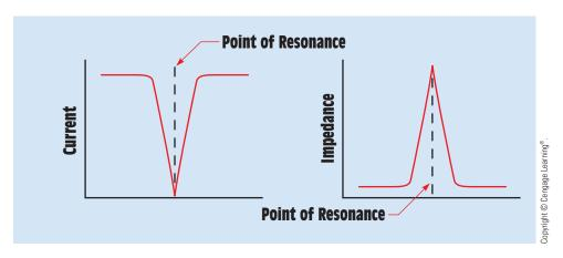
FIGURE 25–11 Characteristic curves of an LC parallel circuit at resonance.
