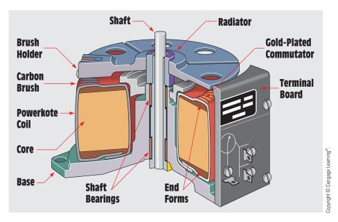
FIGURE 28-42 Cutaway view of a Powerstat.
