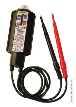
FIGURE 10-45 Low-impedance voltage tester.
