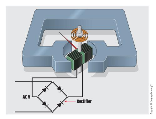
FIGURE 10-3 Rectifier changes AC voltage into DC voltage.
