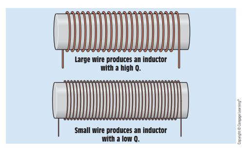
**FIGURE 17–17** The  $\Omega$  of an inductor is a ratio of inductive reactance as compared to resistance. The letter  $\Omega$  stands for quality.
