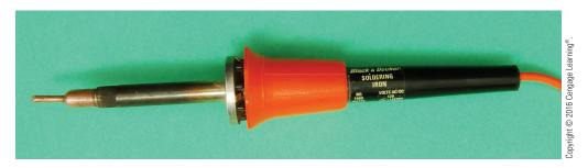
FIGURE S-17 Typical soldering iron used to connect electronic components.
