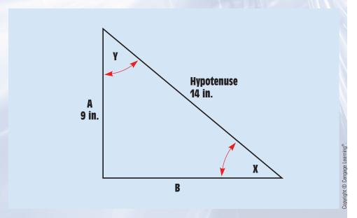
FIGURE 15–7 Finding the angles using trigonometric functions.
