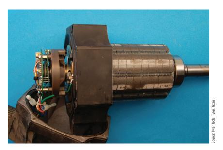
FIGURE 34–72 Permanent magnet rotor with an encoder mounted on the shaft.
