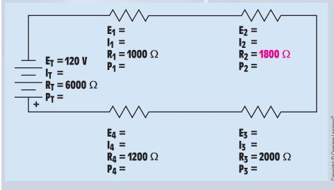
FIGURE 6–13 The missing resistor value.
