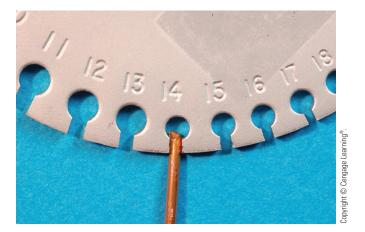
FIGURE 11–5 The slot, not the hole, determines the wire size.
