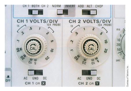
FIGURE 10-47 Voltage control of an analog oscilloscope.
