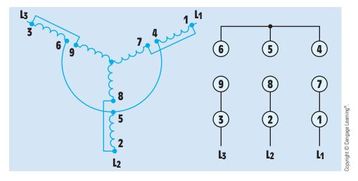
FIGURE 33-19 Low-voltage wye connection.
