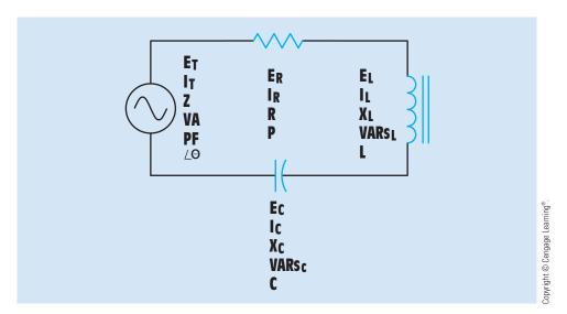
FIGURE 24-2 Resistive-inductive-capacitive series circuit.
