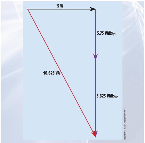
FIGURE 22-9 Power triangle for example circuit.
