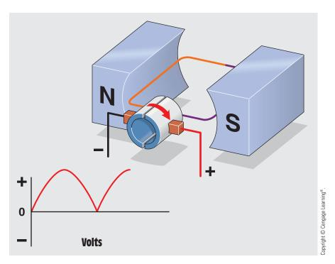
FIGURE 30–11 The commutator maintains the proper polarity.
