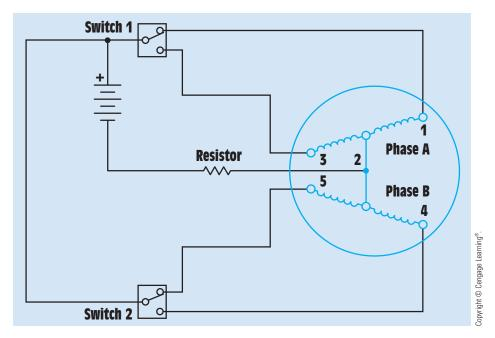
FIGURE 34–56 Bifilar-wound stepping motor.
