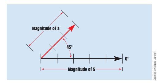
**FIGURE 15–11** A vector with a magnitude of 5 and an angle of 0°.
