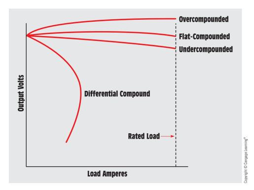
FIGURE 30-43 Characteristic curves of compound generators.
