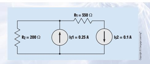
FIGURE 9-29 The circuit contains two current sources.
