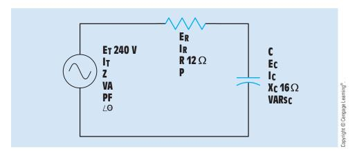
FIGURE 22-1 Resistive-capacitive series circuit.
