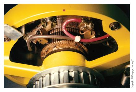
FIGURE 34-62 Armature and brushes of a universal motor.
