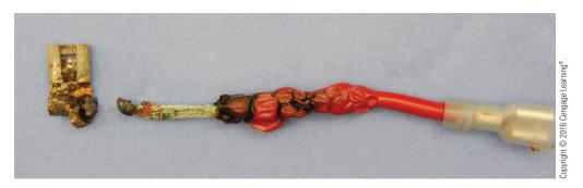
FIGURE S-19 Burned wire caused by a poor connection.
