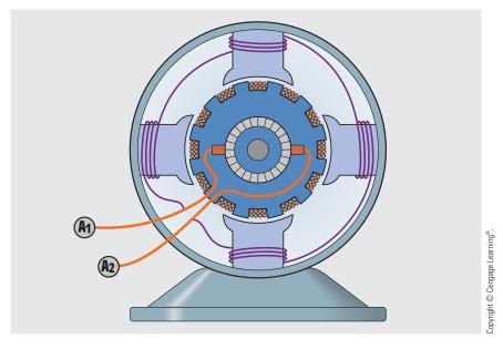
**FIGURE 30–32** Shunt field windings are connected in parallel with the armature.
