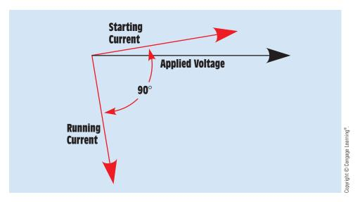
FIGURE 34-17 Run-winding current and start-winding current are 90° out of phase with each other.
