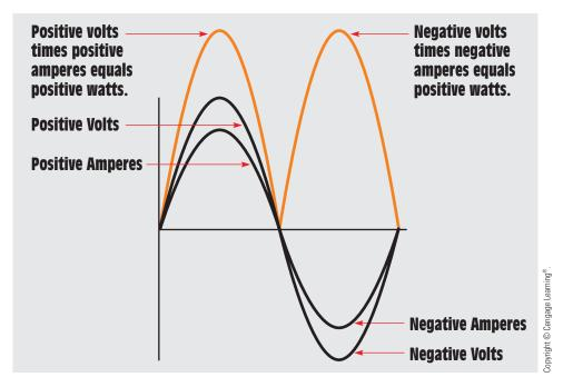
FIGURE 16–20 Power in a pure resistive AC circuit.
