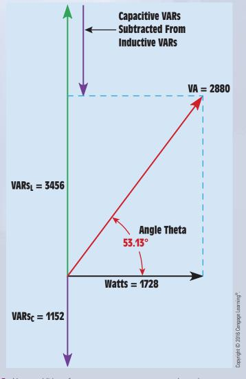
**FIGURE 24–5** Vector addition of apparent power, true power, and reactive power.
