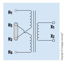
**FIGURE 28–27** Control transformer connected for 480-volt operation.
