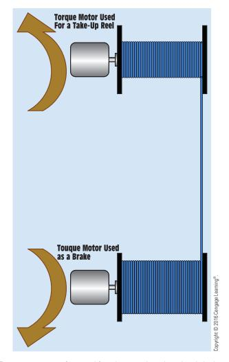
**FIGURE 34–74** Torque motors are often used for take-up reels and as electric brakes.
