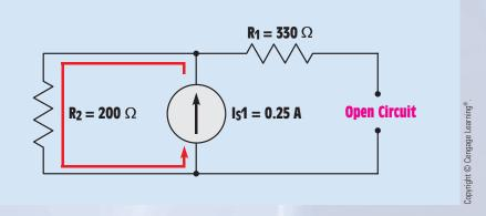
FIGURE 9-30 Current source I<sub>S</sub>2 is replaced with an open circuit.
