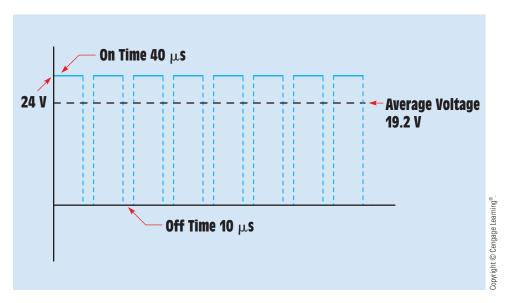
**FIGURE 31–37** The amount of average voltage is determined by the peak voltage and the amount of time it is turned on or off.
