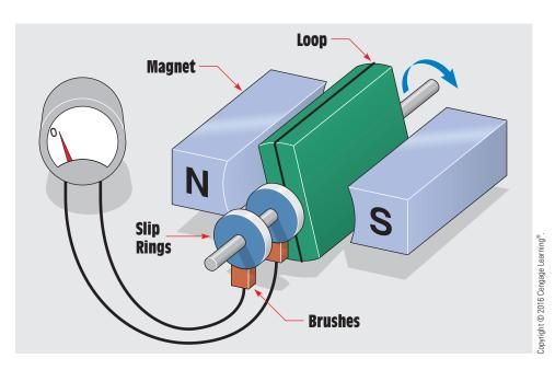
FIGURE 14-7 A single-loop generator.
