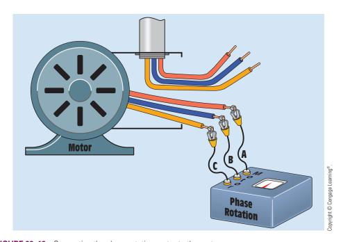
**FIGURE 33–13** Connecting the phase rotation meter to the motor.
