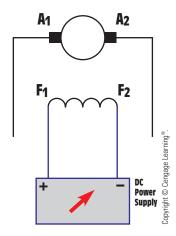
**FIGURE 30–35** Separately excited shunt generators must have an external power source to provide excitation current for the shunt field.
