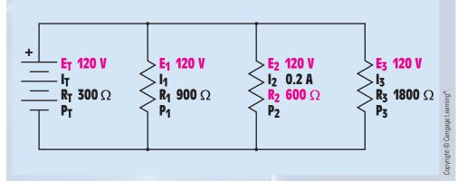
**FIGURE 7–16** The missing resistor and voltage values.
