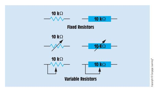
FIGURE 5-19 Schematic symbols used to represent resistors.
