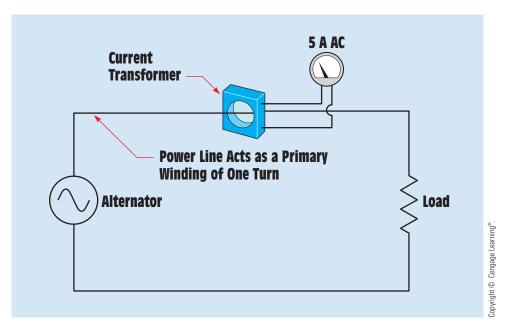
**FIGURE 10–27** Toroid transformer used to change the scale factor of an AC ammeter.
