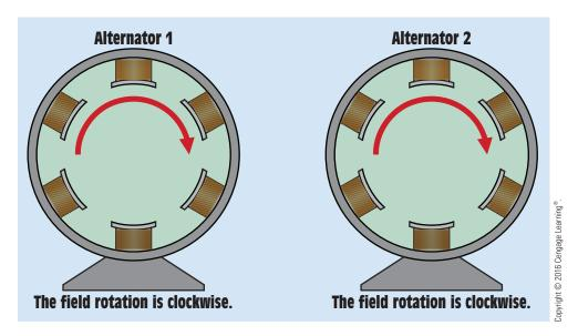
**FIGURE 32–13** The field rotation must be the same for both alternators.
