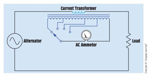
**FIGURE 10–25** A current transformer is used to change the range of an AC ammeter.
