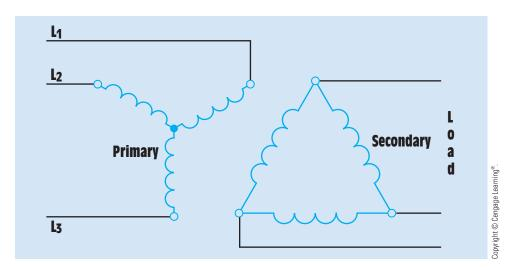
FIGURE 29-5 Wye-delta connected three-phase transformer.
