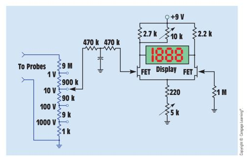
FIGURE 10-42 Digital voltmeter.
