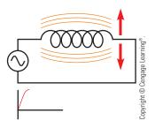
**FIGURE 17–2** As current flows through a coil, a magnetic field is created around the coil.
