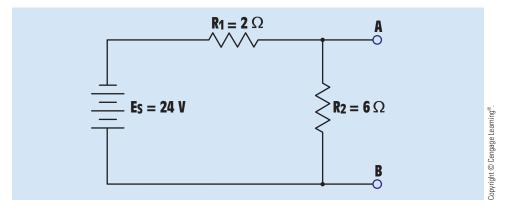
FIGURE 9-9 Determining the Thevenin equivalent circuit.
