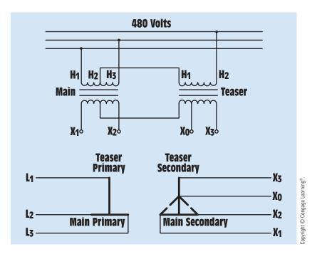
**FIGURE 29–29** T-connected transformers provide a three-phase four-wire connection.  $X_0$  is used as a center tap to the other phases.
