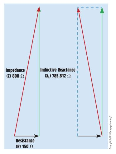
**FIGURE 17–19** The inductive reactance forms one leg of a right triangle.
