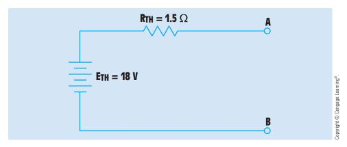
FIGURE 9-11 The Thevenin equivalent circuit.
