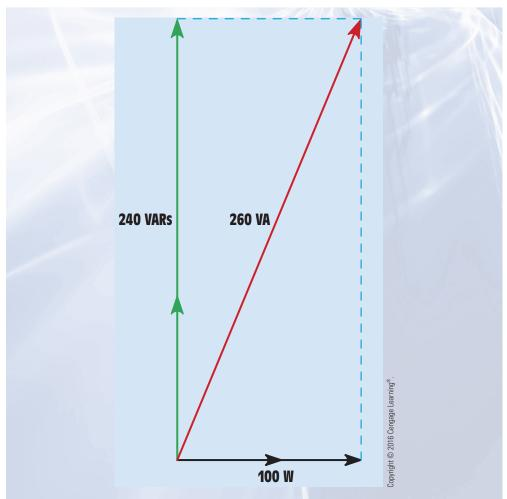
FIGURE 18–21 Power vector for the circuit.
