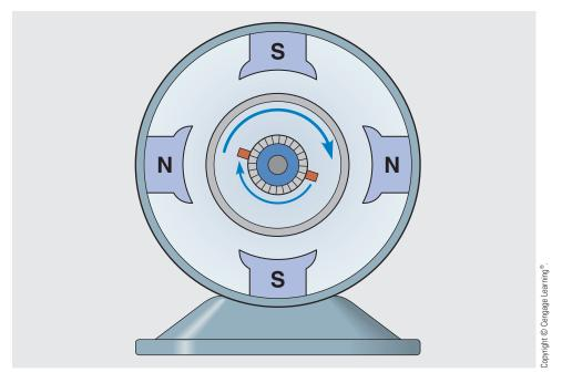
**FIGURE 30–49** In a generator, the brushes are rotated in the direction of armature rotation to correct armature reaction.
