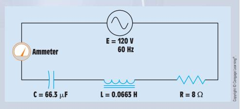
FIGURE 24-7 Example circuit.
