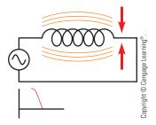
**FIGURE 17–3** As current flow decreases, the magnetic field collapses.
