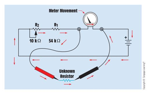
FIGURE 10-39 Shunt-type ohmmeter.
