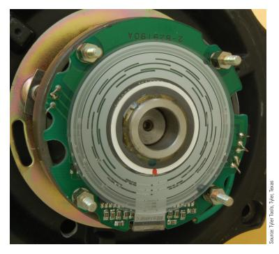
FIGURE 34–70 The slotted wheel of an encoder.
