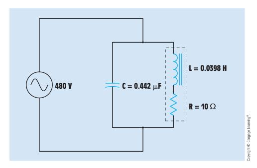
FIGURE 25-8 Parallel resonant circuit.
