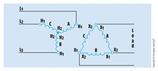
FIGURE 29-8 Identifying the windings.
