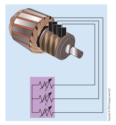
**FIGURE 33–49** The rotor of a wound-rotor motor is connected to external resistors.
