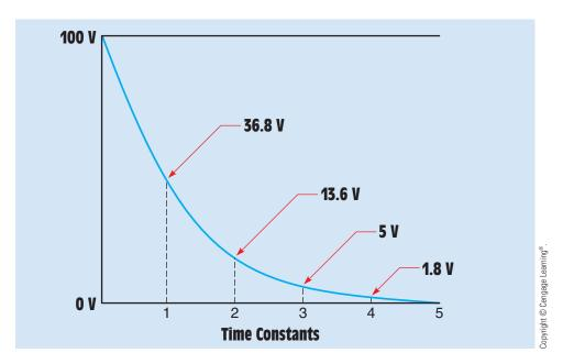
FIGURE 20–15 Capacitor discharge curve.
