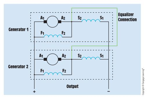
FIGURE 30-55 The equalizer connection is used to connect the series fields in parallel with each other.
