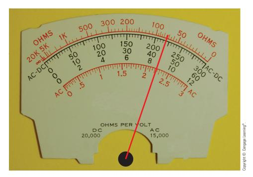
FIGURE 10-12 The meter indicates a value of 440.
