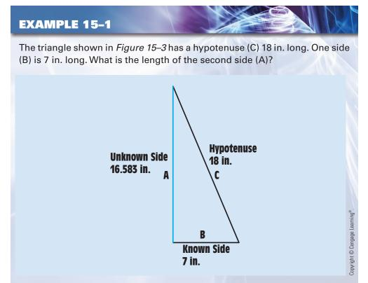
FIGURE 15-3 Using the Pythagorean theorem to find the length of one side.
