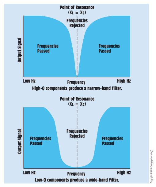
FIGURE 26–15 Band-rejection filters pass most frequencies and reject only a certain range.
