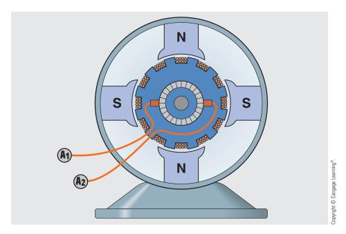
FIGURE 31–30 Permanent magnet motor.
