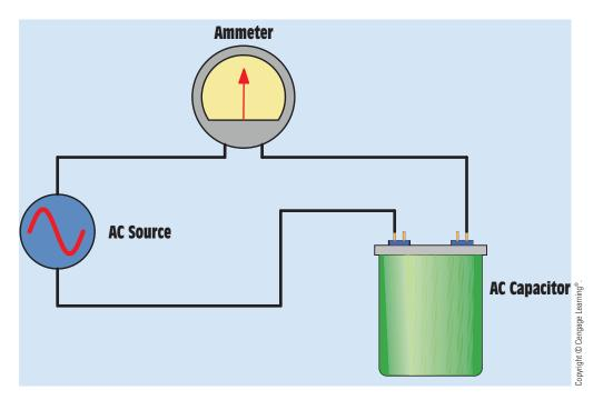
FIGURE 20-37 Determining the capacitance value.
