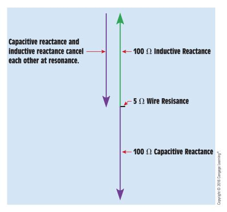
FIGURE 24–10 Inductive reactance and capacitive reactance become equal at resonance.
