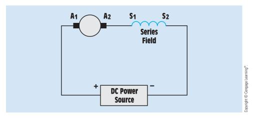
FIGURE 31-8 Series motor connection.
