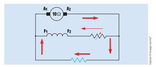
FIGURE 30–39 Armature resistance causes a drop in output voltage.
