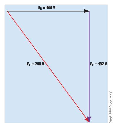
**FIGURE 22–4** The voltage drops across the resistor and capacitor are 90° out of phase with each other.
