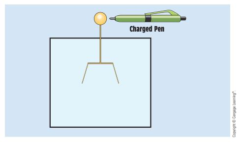
FIGURE 3–8 The leaves move closer together, indicating that the object has a positive charge.
