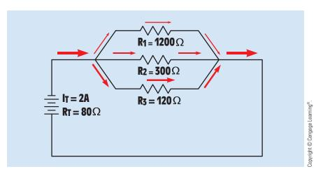
FIGURE 7–25 The current divides through each branch of a parallel circuit.
