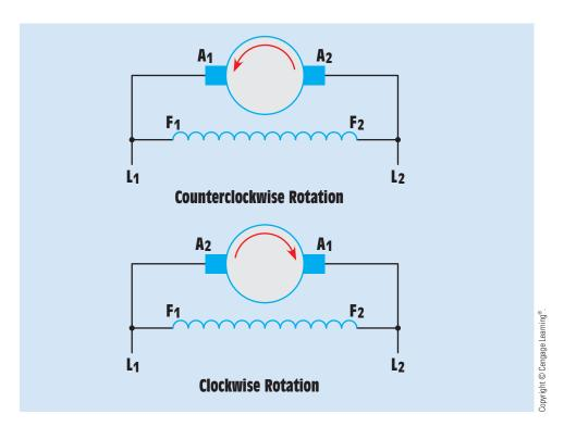
FIGURE 31-15 Shunt motors.
