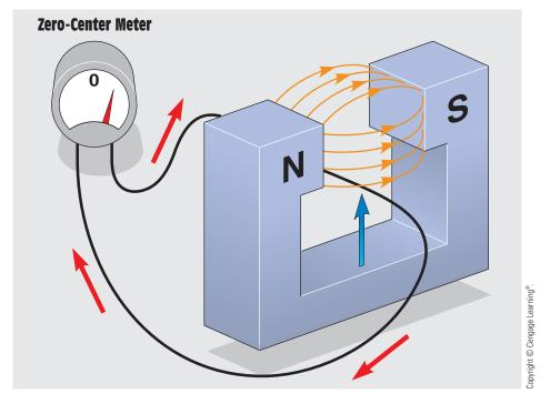
FIGURE 14–3 Reversing the direction of movement reverses the polarity of the voltage.
