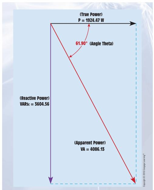
FIGURE 23–10 Vector diagram of apparent power, true power, reactive power, and angle theta.
