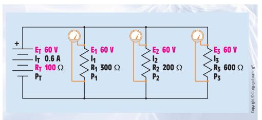
FIGURE 7–12 The voltage is the same across all branches of a parallel circuit.
