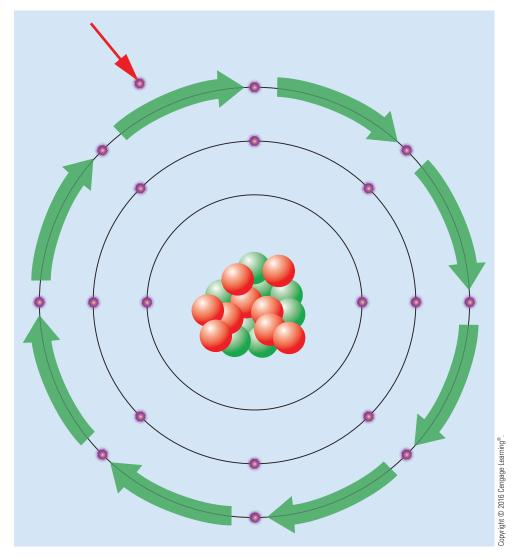
FIGURE 1–24 The energy of the striking electron is divided among the eight electrons.
