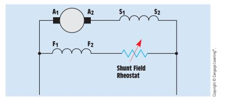
FIGURE 31–21 The shunt field rheostat can be used to overspeed the motor.
