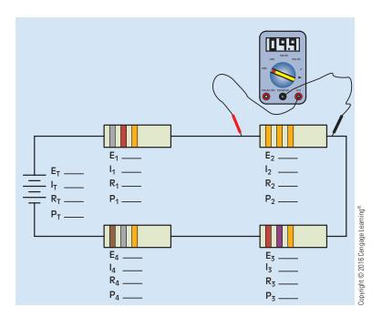
FIGURE 6-28 Determine resistor values using the color code, and determine all missing electrical values.
