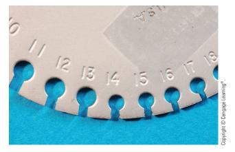
**FIGURE 11–3** One side of the wire gauge is marked with the AWG size.
