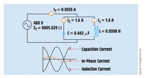
FIGURE 25-10 Total current is equal to the in-phase current.
