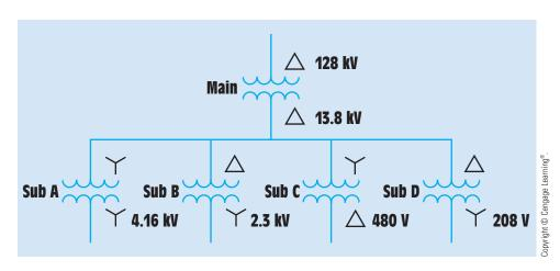
FIGURE 29–12 One line diagrams are generally used to show the main power distribution of a plant.
