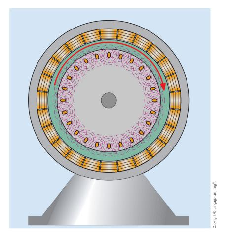
FIGURE 33–28 A magnetic field is produced around each rotor bar.
