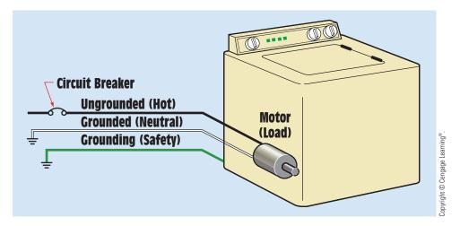
FIGURE 2-10 120-V appliance circuit.
