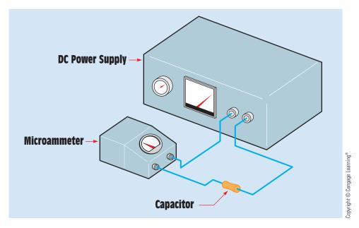
FIGURE 20–34 Testing a capacitor for leakage.
