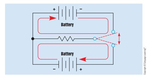
FIGURE 16-3 Square wave AC produced with a switch and two batteries.
