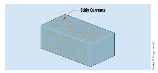
FIGURE 30-40 Eddy currents heat the metal and cause power loss.
