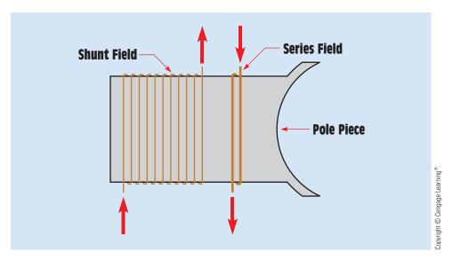
**FIGURE 30–46** In a differential-compound machine, the current flows through the shunt field in a direction opposite that of the current flow through the series field.
