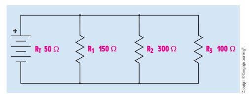
**FIGURE 7–10** Finding the total resistance using the reciprocal method.
