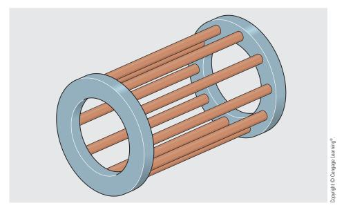
FIGURE 33–25 Basic squirrel-cage rotor without laminations.
