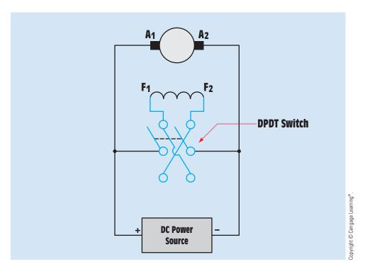
FIGURE 31–17 Reversing the rotation of a shunt motor by changing the shunt field leads.
