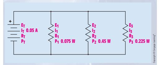
FIGURE 7–19 Parallel circuit, Example 3.
