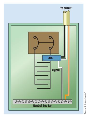
**FIGURE S-30** The arc-fault interrupter connects in the same manner as a ground-fault interrupter.
