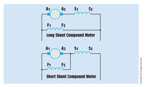
FIGURE 31-10 Compound motor connections.
