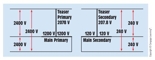
FIGURE 29–28 Voltage vector relationships of a T connection.
