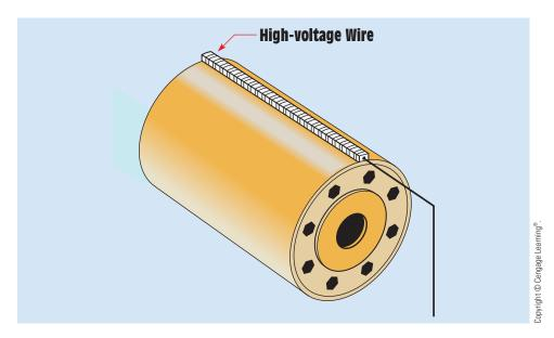
FIGURE 3–14 The drum receives a positive charge.
