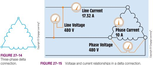
FIGURE 27–15 Voltage and current relationships in a delta connection.
