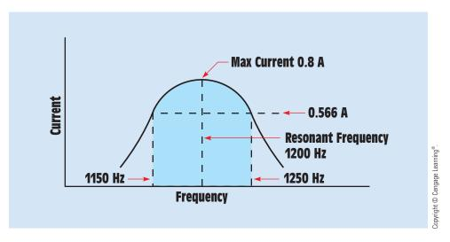
FIGURE 24–14 A wide-band resonant circuit is produced by low-Q inductors and capacitors.
