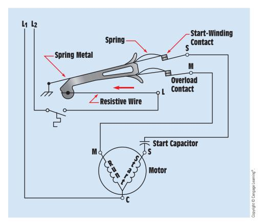
FIGURE 34-8 Hot-wire relay connection.
