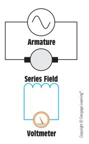
**FIGURE 34–66** Using the series field to set the brushes at the neutral plane position.
