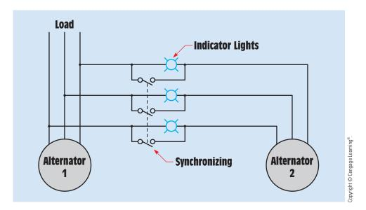
FIGURE 32–14 Determining phase rotation using indicator lights.
