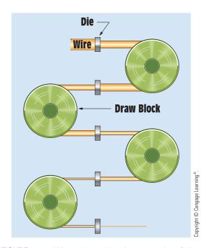
**FIGURE 11–1** Wire is drawn through a succession of dies to produce the desired diameter.
