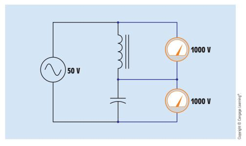
FIGURE 24–12 The voltage drops across the inductor and capacitor increase at resonance.
