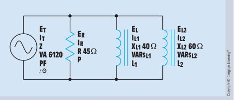
FIGURE 19–12 Example Circuit 2.
