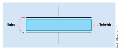
FIGURE 21-1 A basic capacitor.
