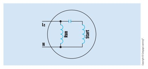
FIGURE 34–27 A capacitor-start capacitor-run motor.
