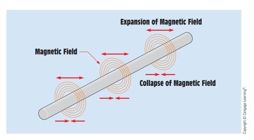
FIGURE 17-1 A continually changing magnetic field induces a voltage into any conductor.
