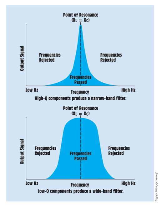
FIGURE 26–13 The bandwidth is controlled by the Q of the components.
