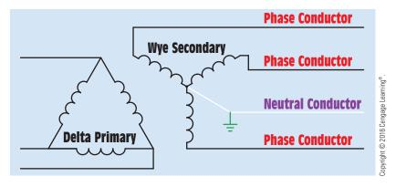
**FIGURE 35–4** In a three-phase four-wire wye-connected system, the center of the wye-connected secondary is tapped to form a neutral conductor.
