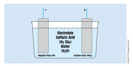
FIGURE 13-18 Basic lead-acid cell.
