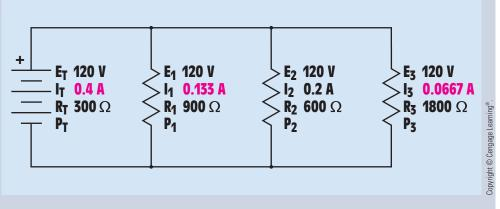
FIGURE 7-17 Determining the current using Ohm's law.
