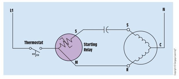
**FIGURE 34–13** Solid-state starting relay connection.
