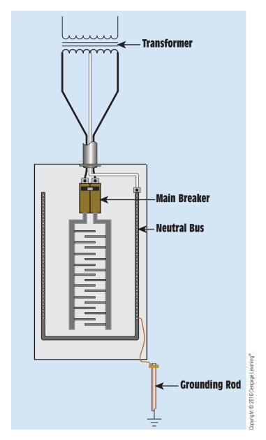
FIGURE 27–10 Grounding circuit for a single-phase power panel.
