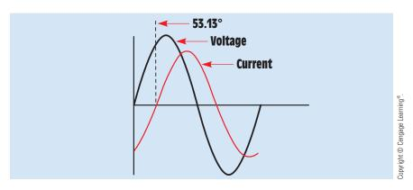
FIGURE 18–16 Current and voltage are 53.13° out of phase with each other.
