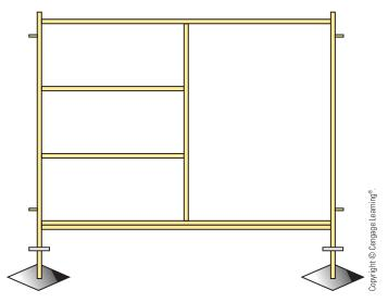
FIGURE S-12 Typical section of scaffolding.
