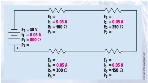
FIGURE 6-9 The current is the same at any point in a series circuit.
