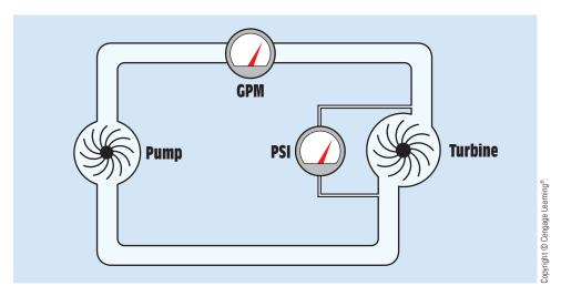
FIGURE 2–15 Force equals flow rate times pressure.
