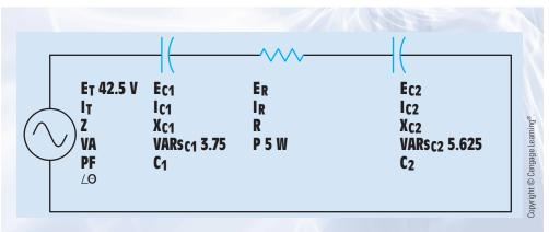
FIGURE 22-8 Example circuit.
