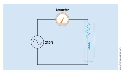
**FIGURE 25–18** At full load, the motor appears to be an R-L series circuit with a large amount of resistance and a smaller amount of inductance.
