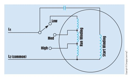
FIGURE 34-38 A three-speed motor.
