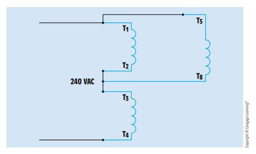
FIGURE 34–24 High-voltage connection with one start winding.
