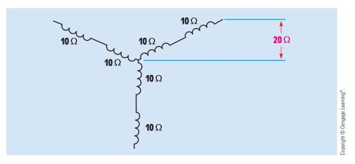
FIGURE 33-23 Impedance adds in series.
