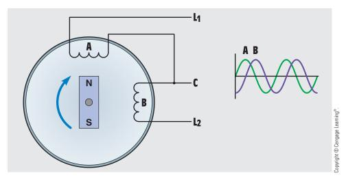
FIGURE 34-1 A two-phase alternator produces voltages that are 90° out of phase with each other.
