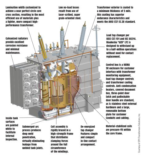
FIGURE 29–2 Three-phase transformer.
