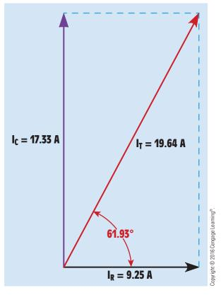
FIGURE 23-12 The total circuit current leads the resistive current and voltage by 61.93°.
