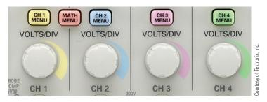
FIGURE 10-48 Voltage control knobs of a four-channel digital oscilloscope.
