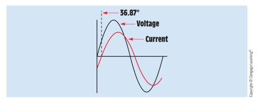
FIGURE 19-9 The current is 36.87° out of phase with the voltage.
