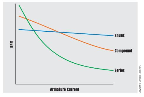
FIGURE 31-6 Characteristic speed curves for different DC motors.
