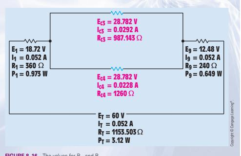
FIGURE 8-16 The values for R<sub>c3</sub> and R<sub>c4</sub>.
