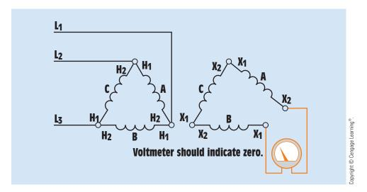
FIGURE 29–13 Testing for proper transformer polarity before closing the delta.
