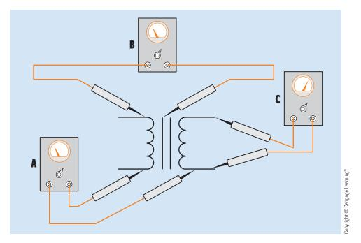
FIGURE 28–57 Testing a transformer with an ohmmeter.
