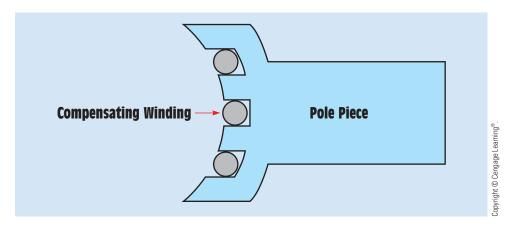
FIGURE 30–52 Compensating winding helps correct armature reaction.
