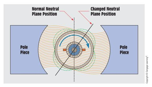
FIGURE 30-48 Armature reaction changes the position of the neutral plane.
