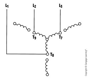
FIGURE A-4 T<sub>7</sub>, T<sub>8</sub>, and T<sub>9</sub> connected to a three-phase, 240-volt line.
