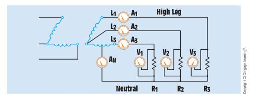
FIGURE 29-21 High leg supplies a single-phase load.
