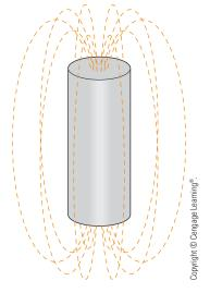
**FIGURE 4–9** Magnetic lines of flux surround the entire magnet.
