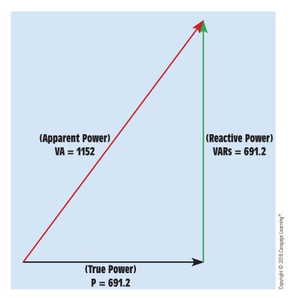
**FIGURE 18–12** Relationship of true power (watts), reactive power (VARs), and apparent power (volt-amperes) in an R-L series circuit.
