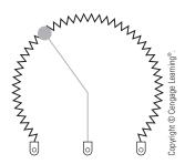
FIGURE 5-14 Variable resistor.
