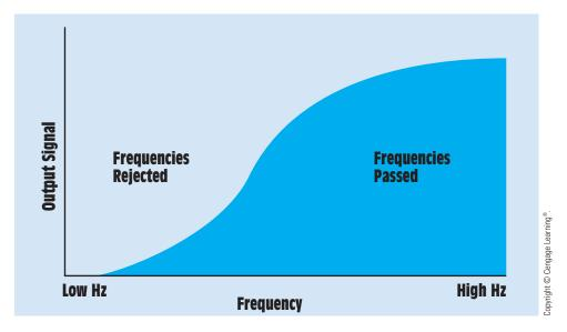
FIGURE 26-9 High-pass filters reject low frequencies and pass high frequencies.
