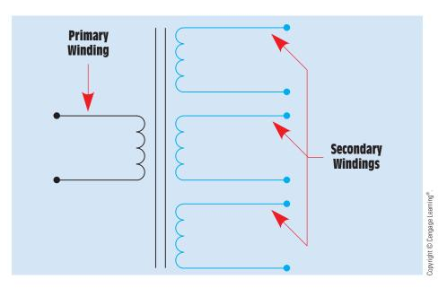
FIGURE 28–14 Transformer with multiple secondary windings.
