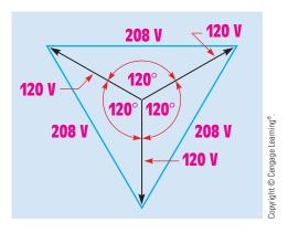
FIGURE 27–11 Vector sum of the voltages in a three-phase wye connection.
