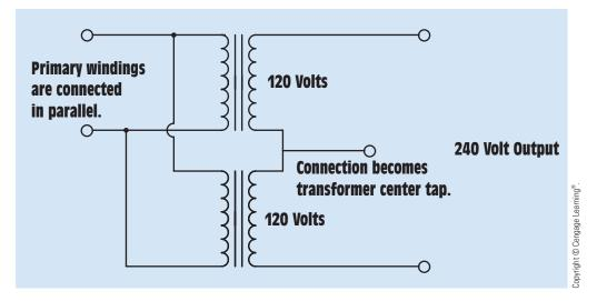
FIGURE 28–64 Transformer secondary windings connected in series.
