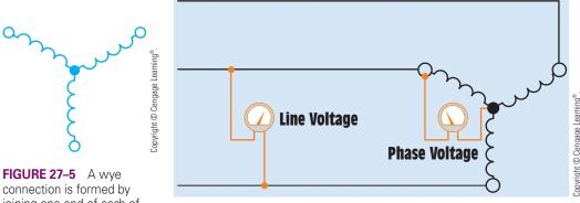
connection is formed by joining one end of each of the windings together.
