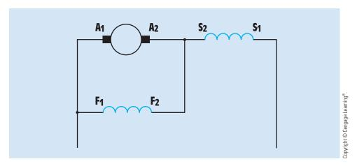
FIGURE 30-42 Schematic drawing of a short shunt compound generator.
