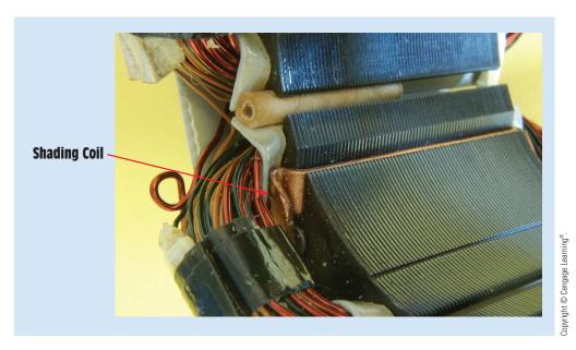
FIGURE 34-35 The shading coil is a large copper conductor wound around one side of the pole piece.
