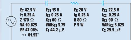
FIGURE 22-11 Example circuit with completed values.
