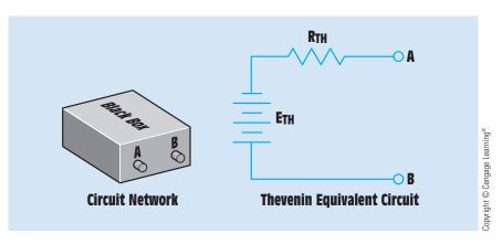
**FIGURE 9-7** Thevenin's theorem reduces a circuit network to a single power source and a single series resistor.
