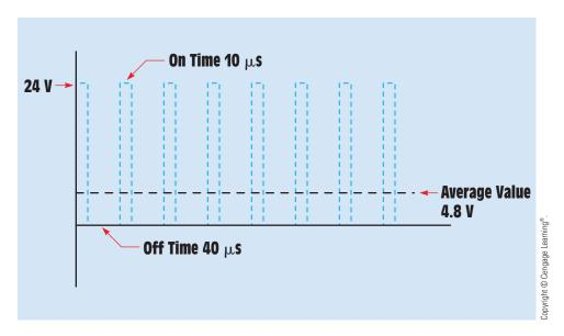
FIGURE 31–38 Reducing the on time reduces the average voltage.
