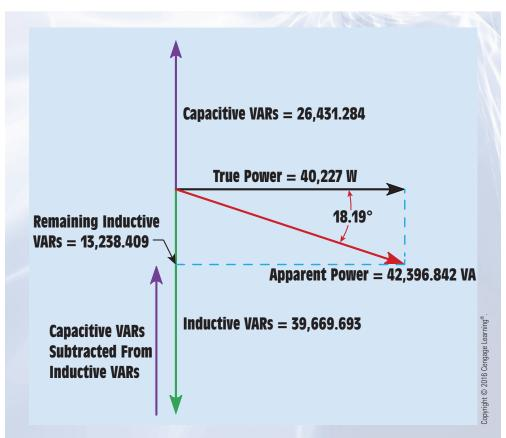
**FIGURE 27–25** Vector relationship of powers to correct motor power factor.
