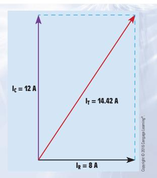
FIGURE 23-5 Vector addition can be used to find total current.
