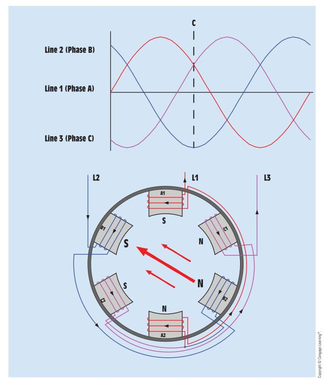
FIGURE 33-4 The magnetic field is concentrated between poles B1 and B2.
