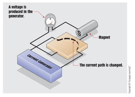
FIGURE 10-34 The presence of a magnetic field causes the Hall generator to produce a voltage.
