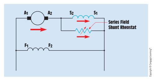
FIGURE 30-44 The series field shunt rheostat controls the amount of compounding.
