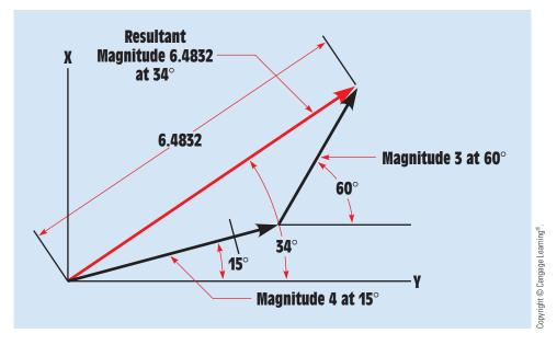
FIGURE 15–17 Adding two vectors with different directions.
