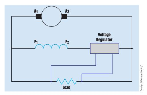
FIGURE 30-38 The voltage regulator controls the amount of shunt field current.
