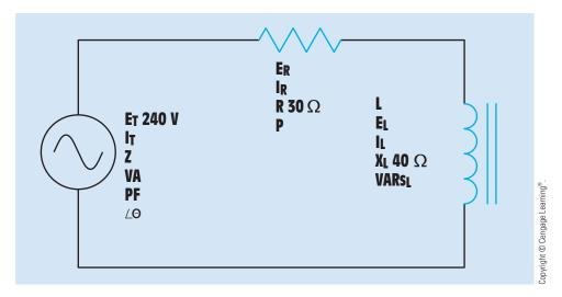
FIGURE 18-2 R-L series circuit.
