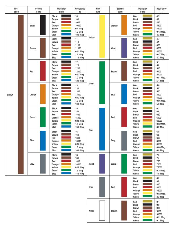
**FIGURE 5–9** Resistor color code chart.
