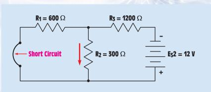
FIGURE 9-25 Current flows in the same direction.
