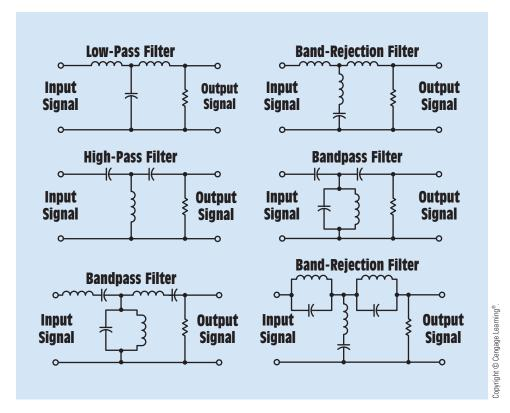
FIGURE 26–17 Basic T-type filters.
