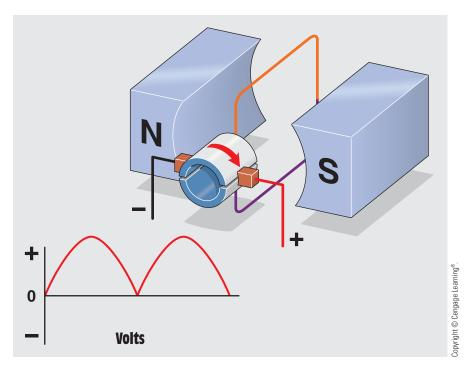
**FIGURE 30–12** The loop completes one complete rotation.
