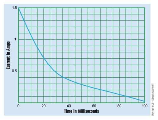
FIGURE 14–20 Current flow through an inductor decreases at an exponential rate.
