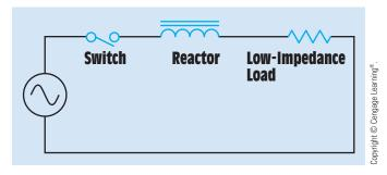
**FIGURE 28–33** Reactors are used to help prevent inrush current from becoming excessive when power is first turned on.
