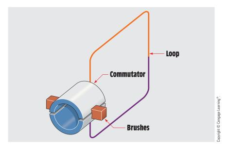
**FIGURE 30–7** The commutator is used to convert the AC voltage produced in the armature into DC voltage.
