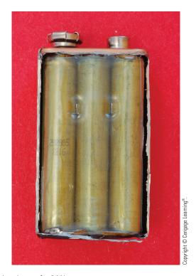
FIGURE 13–12 Internal makeup of a 9-V battery.
