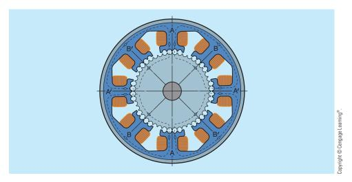
FIGURE 34-54 Construction of a stepping motor.
