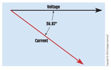
**FIGURE 25–6** The current lags the voltage by 36.87°.
