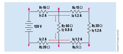
FIGURE 9–2 The current splits to separate branches.
