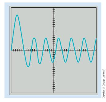
FIGURE S-27 Current spike produced by turning a light on or off.
