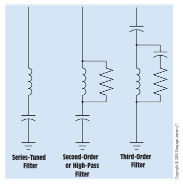
**FIGURE 35–10** The construction of a harmonic filter is dictated by the frequency of the harmonic to be eliminated.
