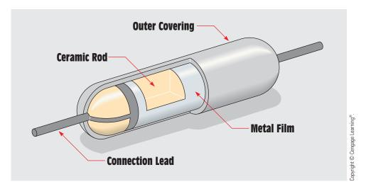
FIGURE 5-5 Metal film resistor.
