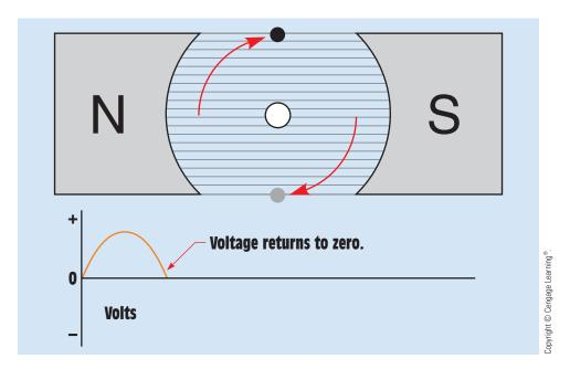
FIGURE 30-4 Induced voltage after 180° of rotation.
