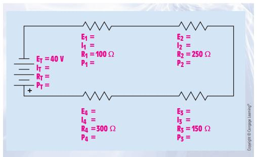
FIGURE 6-8 Series circuit, Example 1.
