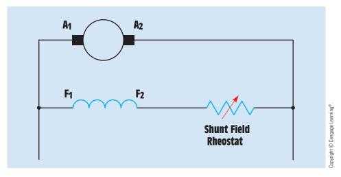
FIGURE 30–37 The shunt field rheostat is used to control the output voltage.
