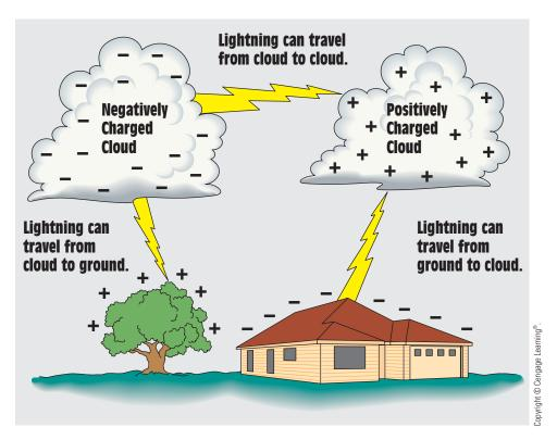
FIGURE 3–10 Lightning travels from negative to positive.
