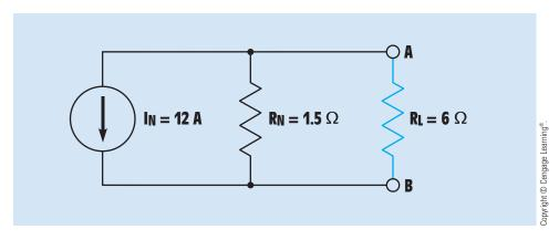
FIGURE 9–19 A 6-ohm load resistor is connected to the equivalent Norton circuit.
