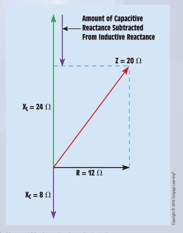
**FIGURE 24–3** Vector addition is used to determine impedance.
