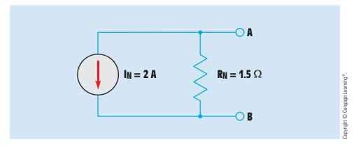
FIGURE 9–18 Equivalent Norton circuit.
