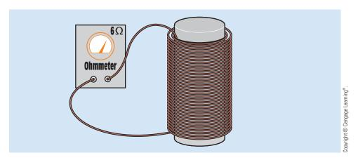
**FIGURE 17–5** Measuring the resistance of a coil.
