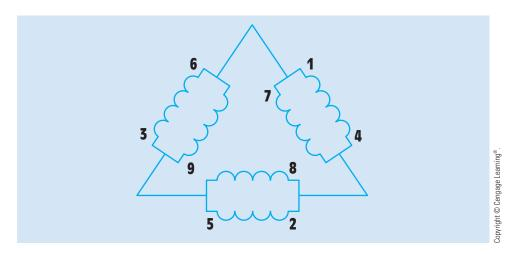
FIGURE 33–20 Parallel delta connection.
