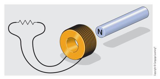
FIGURE 14-10 No current flows through the coil.
