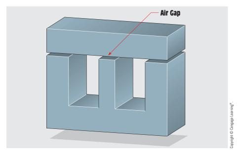
FIGURE 28-37 The core of an inductor contains an air gap.
