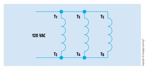
FIGURE 34–25 Low-voltage connection for a split-phase motor with one start winding.
