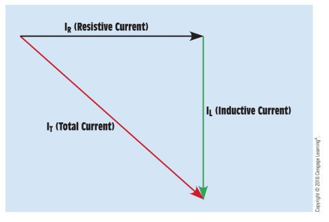
FIGURE 19–5 Relationship of resistive, inductive, and total current in an R-L parallel circuit.
