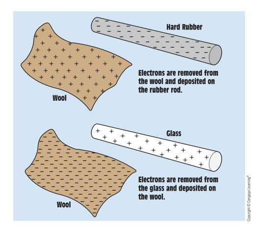
**FIGURE 3–4** Producing a static charge.
