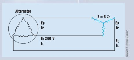
**FIGURE 27–20** Calculating three-phase values using a delta-connected source and a wye-connected load (example circuit).
