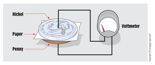
FIGURE 13-4 A voltaic cell constructed from two coins and a piece of paper.
