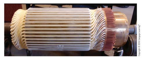
FIGURE 30–24 Armature wound with rectangular wire.
