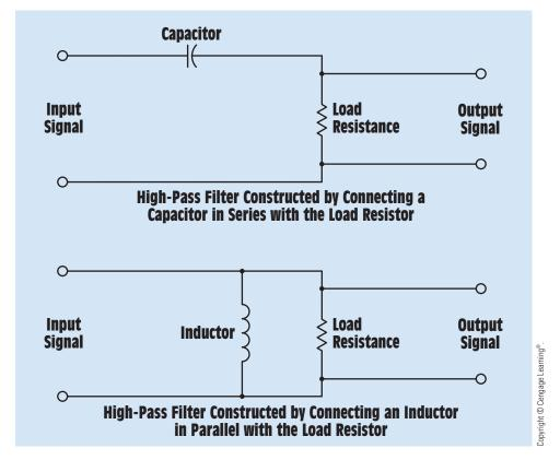
FIGURE 26-10 Construction of high-pass filters using capacitors and inductors.
