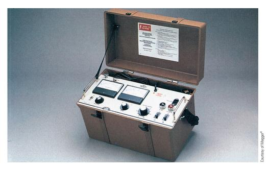
FIGURE 20-36 A dielectric test set.
