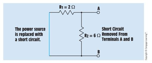
FIGURE 9–17 Determining the Norton equivalent resistance.
