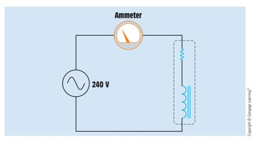
FIGURE 25–17 At no load, the motor appears to be an R-L series circuit with a large amount of inductance and a small amount of resistance.
