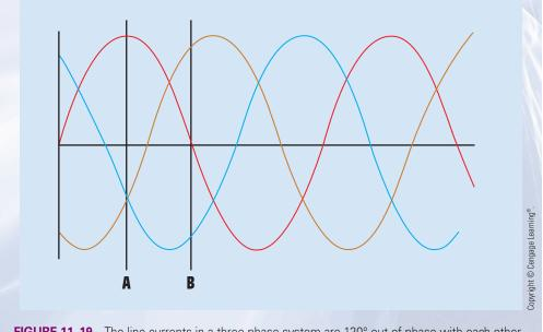
FIGURE 11–19 The line currents in a three-phase system are 120° out of phase with each other.
