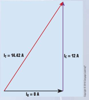
**FIGURE 23–4** Resistance current and capacitive current are 90° out of phase with each other.
