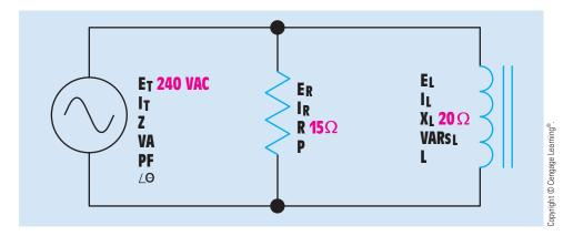
FIGURE 19-4 Typical R-L parallel circuit.
