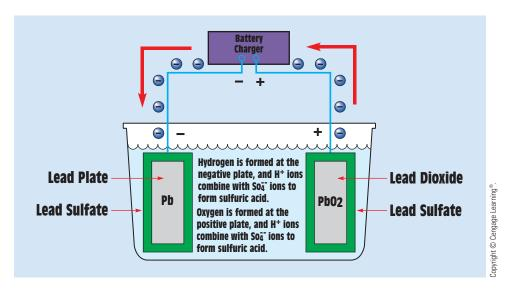
FIGURE 13-21 A lead-acid cell during the charging cycle.
