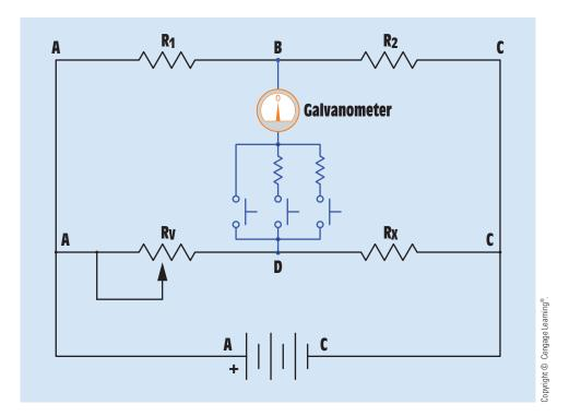
**FIGURE 10–64** The Wheatstone bridge circuit is used to make accurate measurements of resistance and operates on the principle that the sum of the voltage drops in a series circuit must equal the applied voltage.
