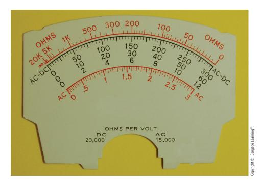
**FIGURE 10–10** Typical multimeter scale.
