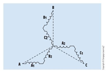
FIGURE 29–32 Schematic diagram of a zig-zag connection.
