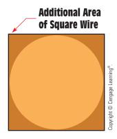
FIGURE 30-23 A square wire of equal size contains more surface area than round wire.
