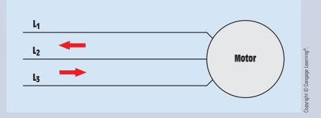
FIGURE 11-21 Current flows from line 3 to line 2.
