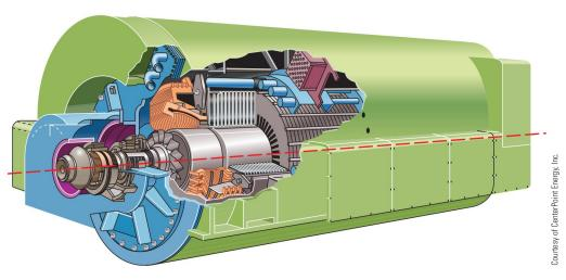
FIGURE 32–12 Two-pole, turbine-driven, hydrogen-cooled alternator.
