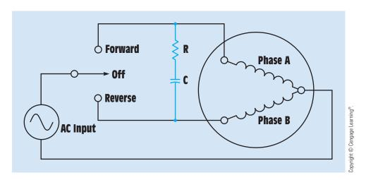
FIGURE 34-60 Phase-shift circuit converts single-phase into two-phase.
