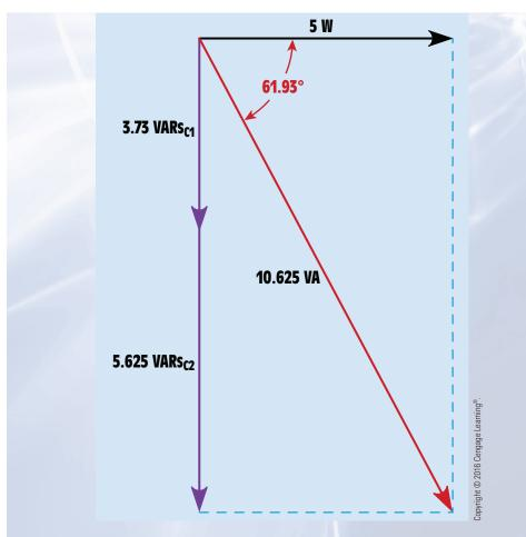
FIGURE 22–10 Vector relationship of reactive, true, and apparent power.
