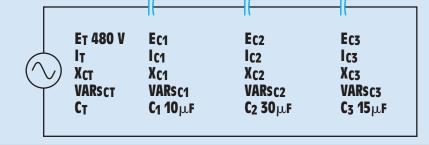
FIGURE 21-11 Capacitors connected in series.
