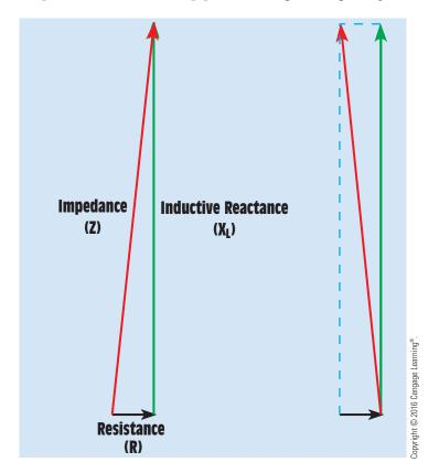
FIGURE 17–18 Coil impedance is a combination of wire resistance and inductive reactance.
