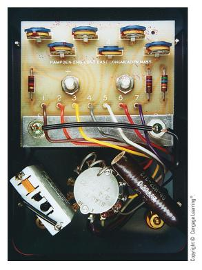
FIGURE 10-23 DC ammeter with an Ayrton shunt.
