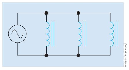
FIGURE 17-11 Inductors connected in parallel.
