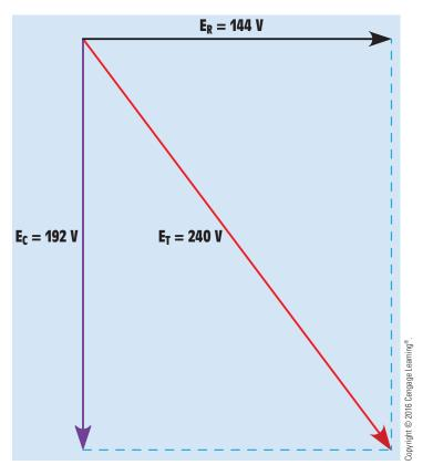
FIGURE 22–5 Voltage vector for example circuit.
