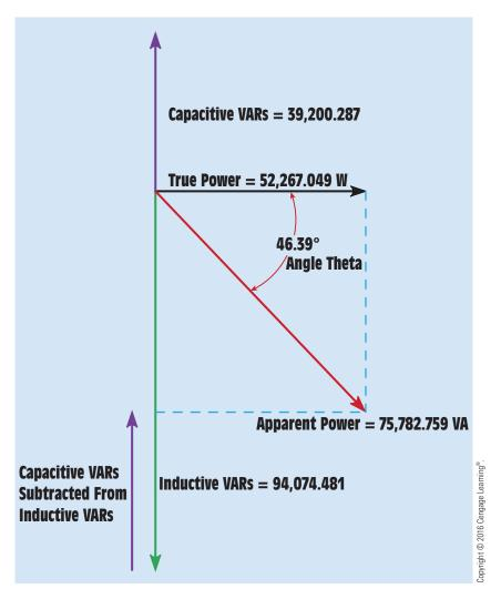
**FIGURE 27–23** The current lags the voltage by 46.39°.
