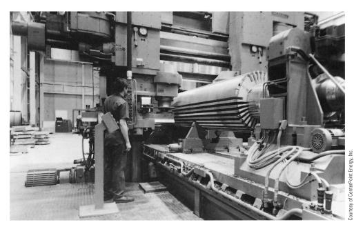
FIGURE 32–11 Two-pole rotor slotting.
