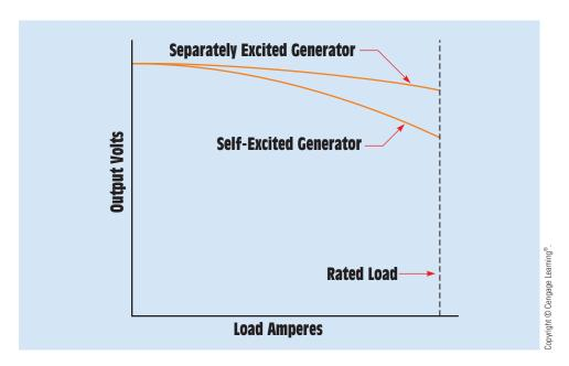
FIGURE 30-36 Characteristic curves of self- and separately excited shunt generators.
