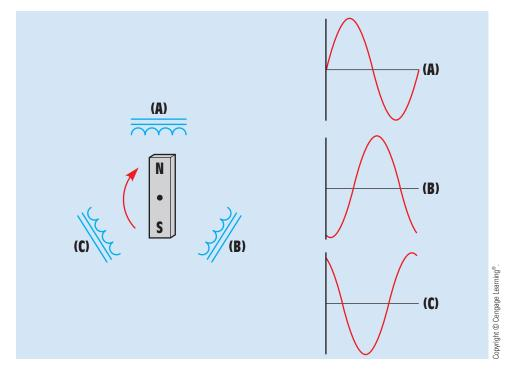
FIGURE 27-4 The voltages of a three-phase system are 120° out of phase with each other.
