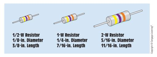
FIGURE 5-4 Power rating is indicated by size.
