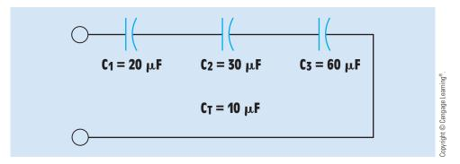
FIGURE 20-13 Capacitors connected in series.
