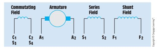
FIGURE 31–13 Terminal identification for DC machines.
