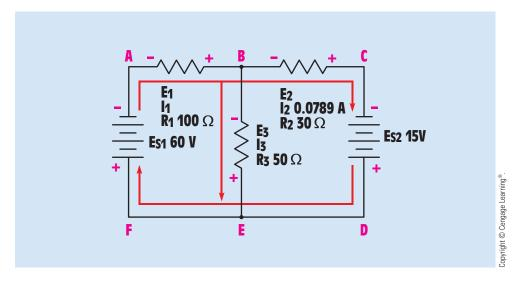
FIGURE 9-5 Actual direction of current flow.
