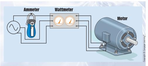
FIGURE 27–24 Determining apparent and true power for a three-phase motor.
