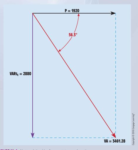
**FIGURE 23–6** Vector relationship of apparent, true, and reactive power.
