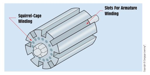
FIGURE 34–47 Repulsion-induction motors contain both armature and squirrel-cage windings.
