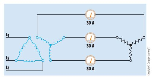
FIGURE 29–19 Three-phase transformer connected to a balanced three-phase load.
