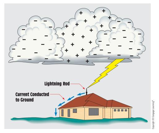
FIGURE 3–11 A lightning rod provides an easy path to ground.
