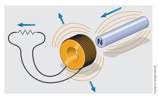
FIGURE 14–11 Induced current produces a magnetic field around the coil.
