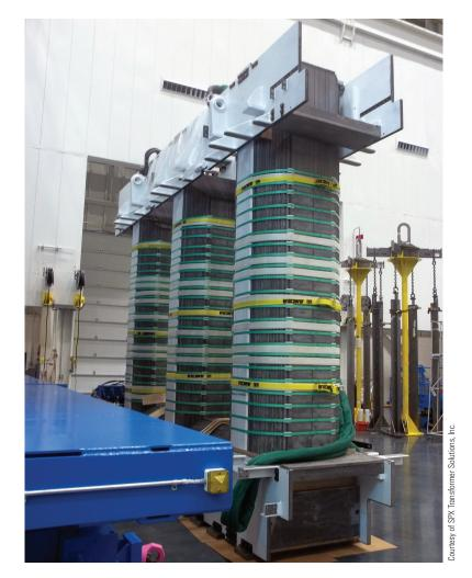
FIGURE 28–28 Core of a 630-MVA three-phase transformer.
