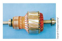
**FIGURE 30–16A** DC machine armature.
