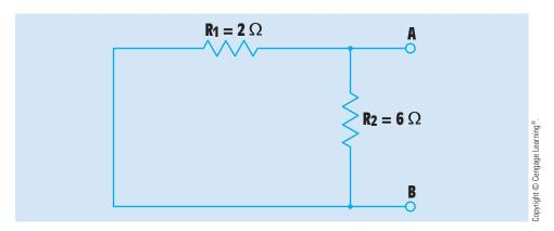
FIGURE 9-10 Determining the Thevenin equivalent resistance.
