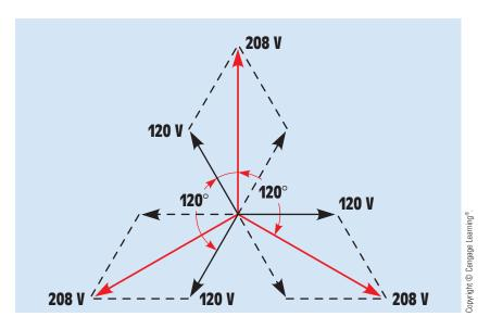
**FIGURE 27–13** The parallelogram method of adding three-phase vectors.
