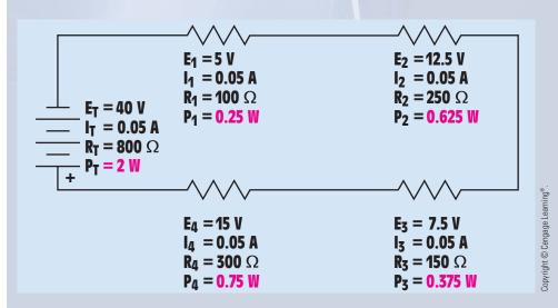
FIGURE 6–11 The final values for the circuit in Example 1.
