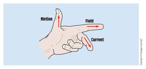
FIGURE 14–5 Left-hand generator rule.
