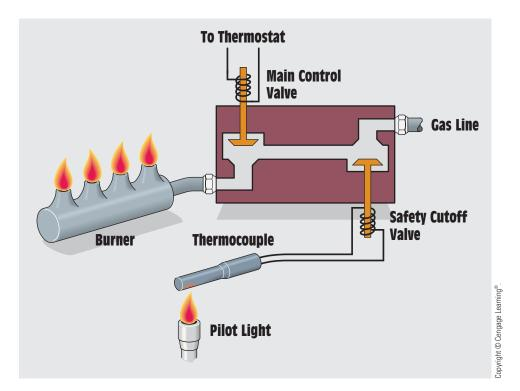
FIGURE 13-37 A thermocouple provides power to the safety cutoff valve.
