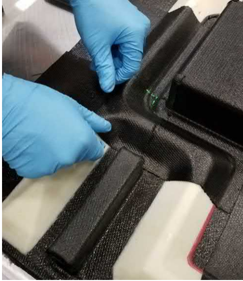
FIGURE 1.5 Part with complex shape being laminated requiring additional skill to prevent defects.
