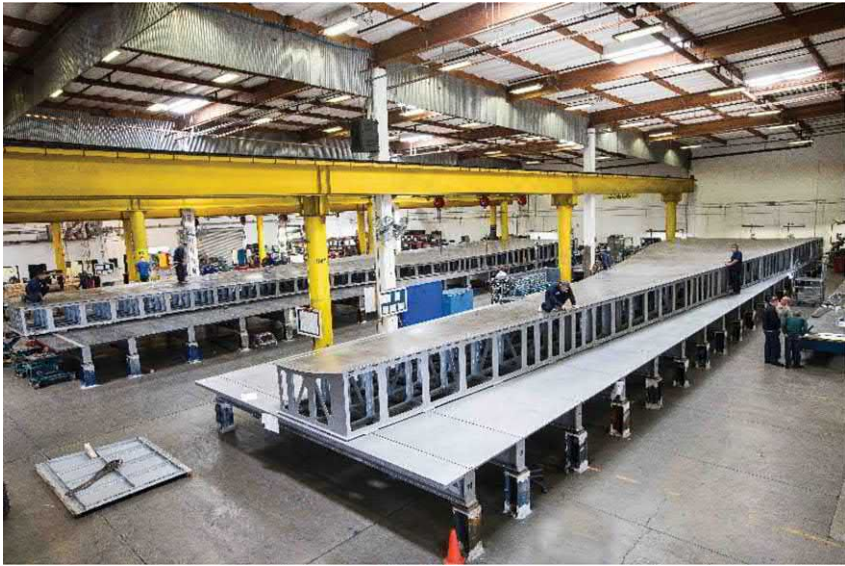
FIGURE 4.16 Large invar tool for wing skin [17].
