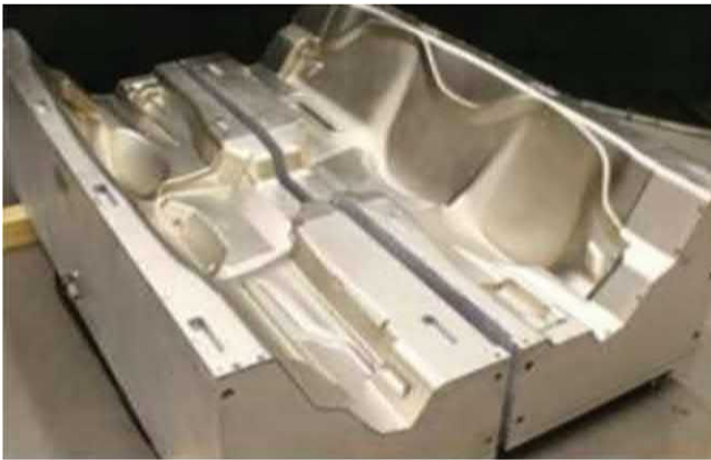
FIGURE 1.14 Nickel Vapor Deposition (NVD) shell tooling.
