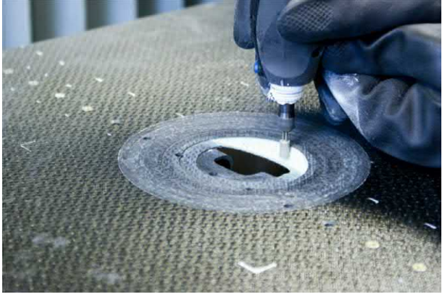
FIGURE 3.3 Example of tool modification to support late part design change [9].
