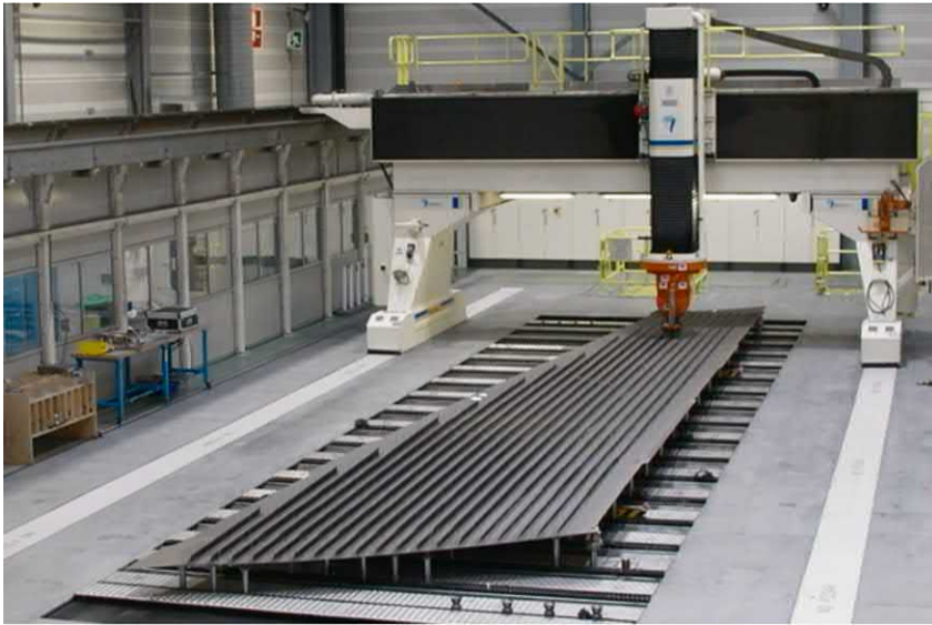
FIGURE 6.36 Standard universal holding fixture example [23].
