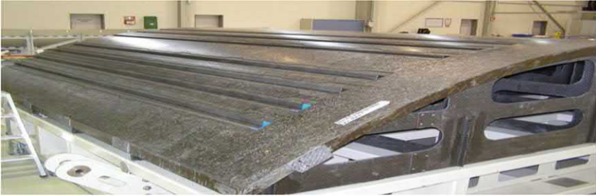
FIGURE 1.13 HexTool® M61 tooling fabricated from Hexcel's BMI resin.
