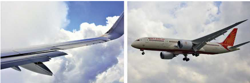
FIGURE 5.3 Control surfaces and fairing made from composite materials [4-5].
