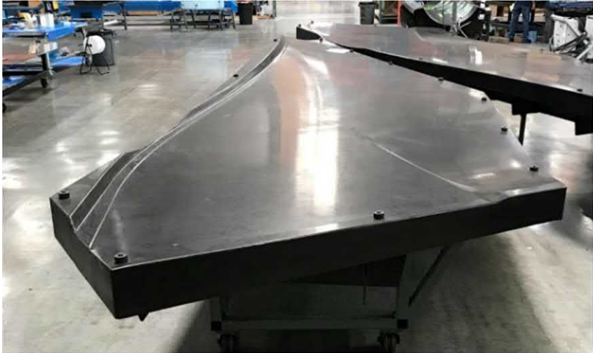
FIGURE 1.7 Example of a tool used for composite lamination.
