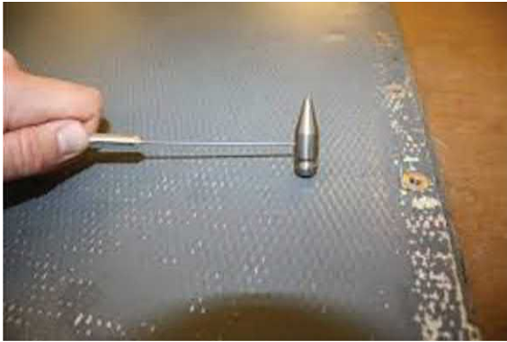
FIGURE 6.41 Tap test occurring on a composite part [29].
