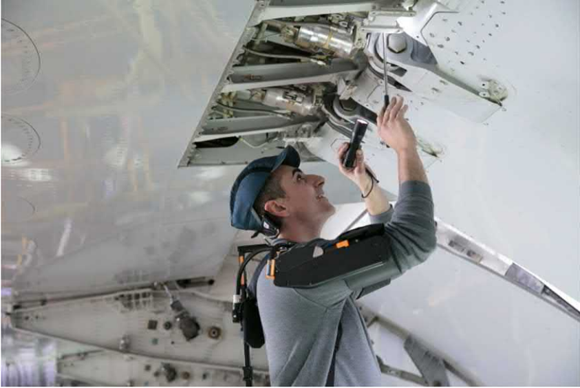
FIGURE 6.39 Visual inspection example that occurs typically during operation [27].
