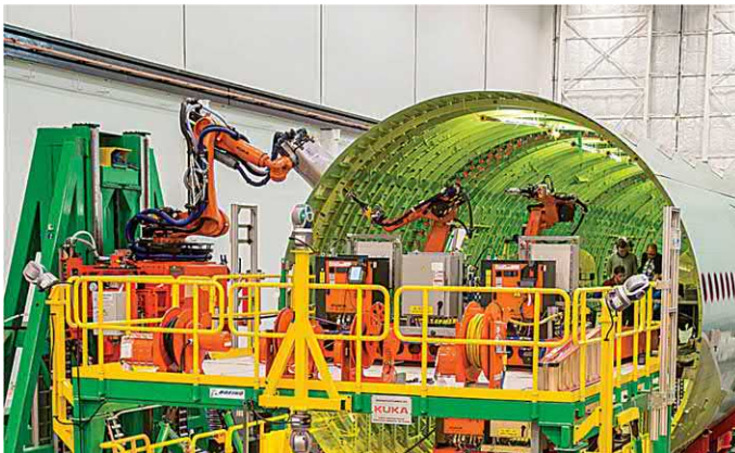
FIGURE 6.16 Automation drilling process [14].
