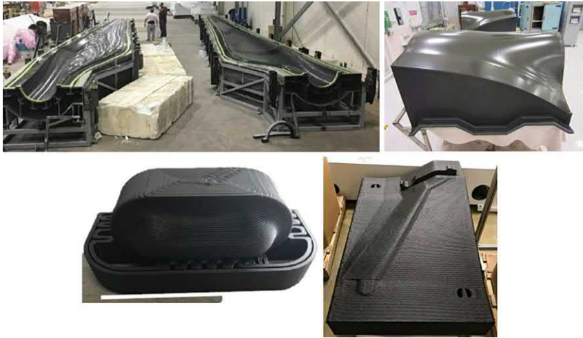
FIGURE 8.1 Tooling used for composite fabrication built from additive manufacturing [4–7].
