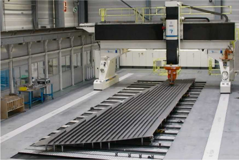
FIGURE 6.36 Standard universal holding fixture example [23].
