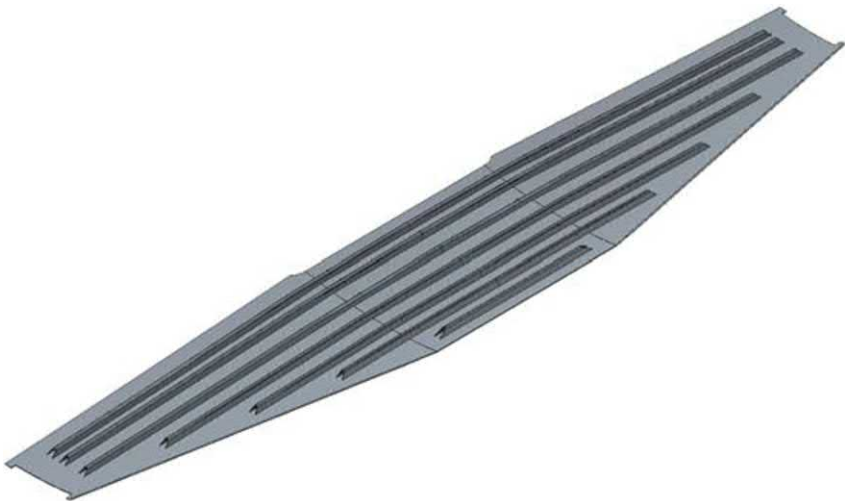
FIGURE 5.7 Wing skin with stiffeners [21].
