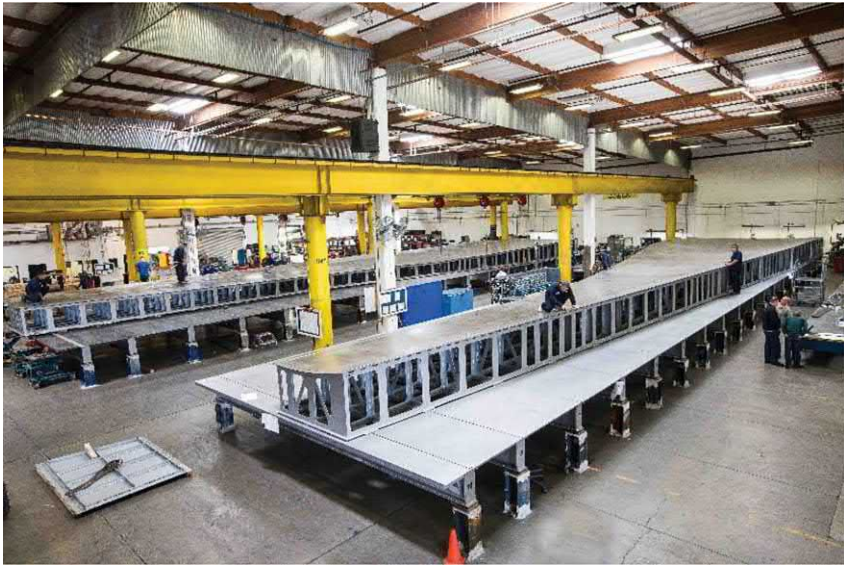
FIGURE 4.16 Large invar tool for wing skin [17].
