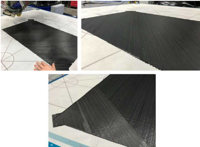
FIGURE 5.60 Flat panel fabrication using AFP.
