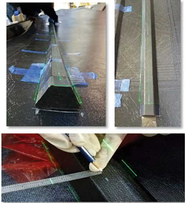
FIGURE 5.19 Mandrel placement during the wing skin demo fabrication utilizing laser projection.
