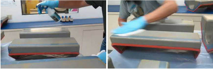
FIGURE 3.19 Tool being prepared using FreKote release agent [16].
