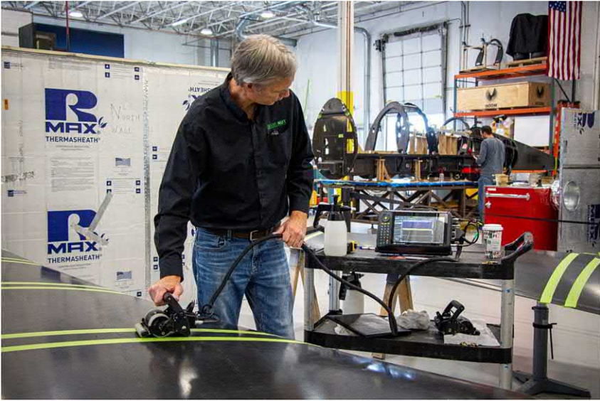
FIGURE 6.44 Example of a bond tester on composite wing structure [31].
