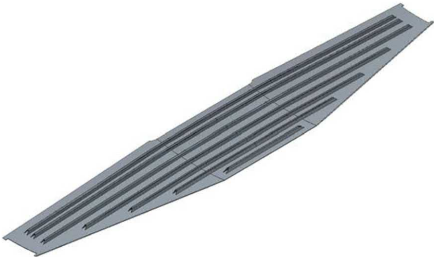
FIGURE 5.7 Wing skin with stiffeners [21].
