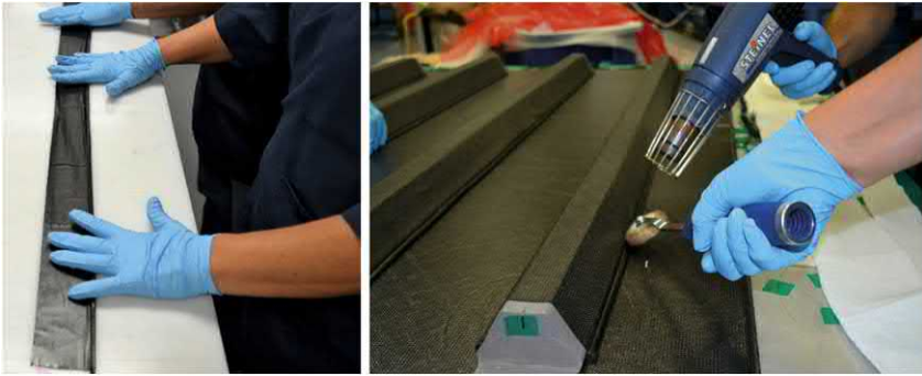
FIGURE 7.20 Rolled tow filler fabrication approach.
