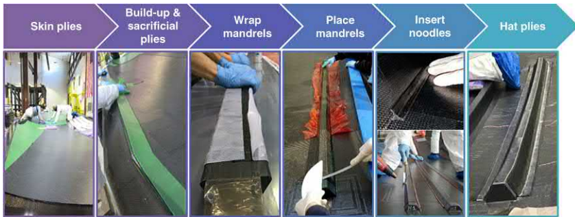
FIGURE 5.15 Overview of the lamination process used for the wing skin demo.
