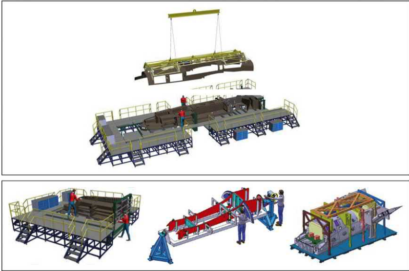
FIGURE 4.28 Full assembly process versus sub-assembly.
