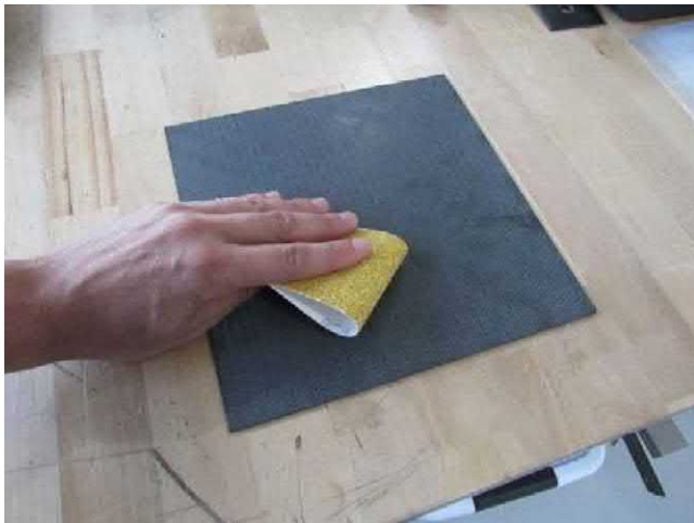
FIGURE 3.9 Example of hand sanding process of composite.
