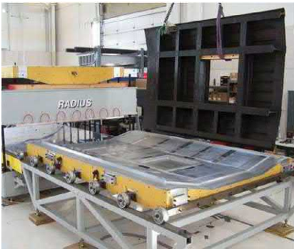
FIGURE 5.44 Part getting demolded out of the tool post cure [37].
