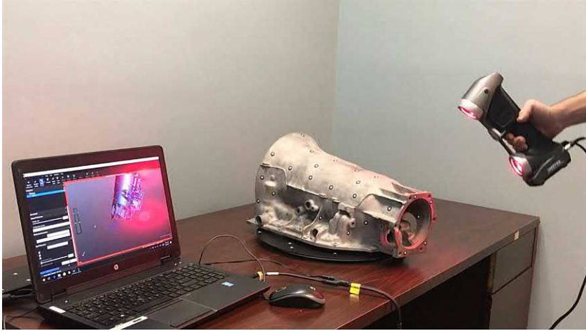
FIGURE 6.29 Laser scanning example [19].
