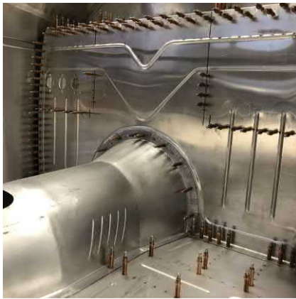
FIGURE 4.24 Cleco's used to hold different parts together prior to final installation [20].
