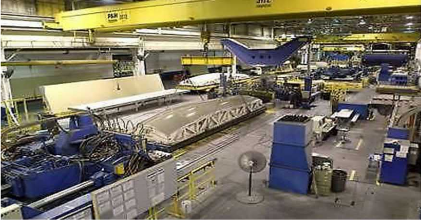
FIGURE 6.3 Example of a large tool that requires a crane for movement [3].
