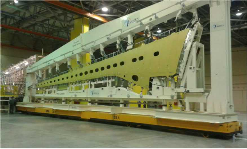
FIGURE 6.14 Assembly tools used for airplane wing [13].
