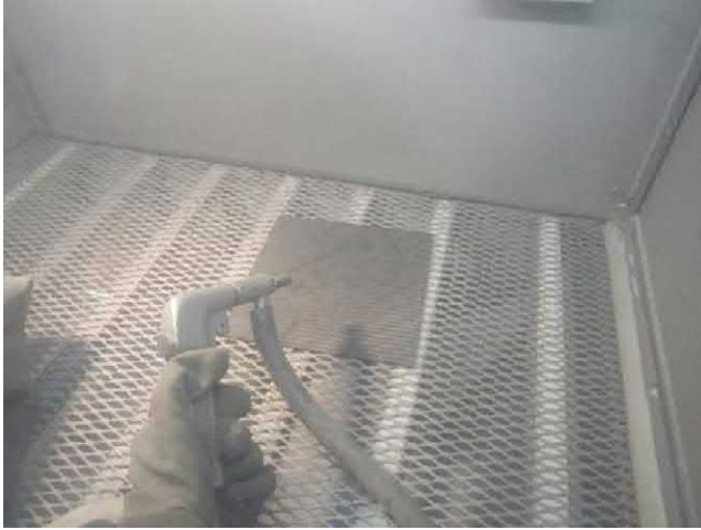
FIGURE 3.10 Example of grit blasting of composite surface.
