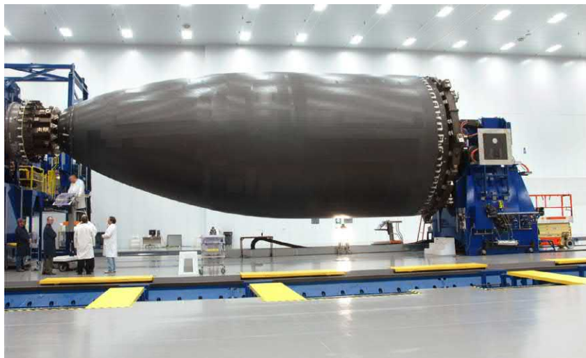
FIGURE 3.6 BMI tool used to fabricate the 787 fuselage sections [10].
