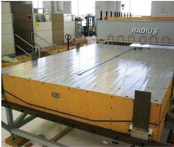
FIGURE 5.43 Mold closed and resin being injected [37].
