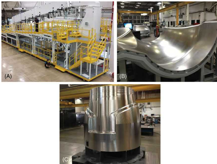
FIGURE 4.10 Different types of tools used in production (A) assembly tools (B), (C) lamination tools [4–5].
