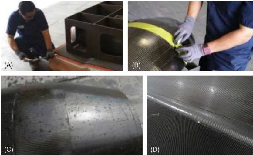
FIGURE 3.4 Examples of manufacturing techniques (A) Demolding with metal wedges. (B) Cutting on tool surface. (C) Tool exposed to moisture and UV (D) dent on composite tool.
