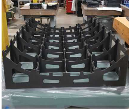
FIGURE 4.17 Tool backing structure example made from composite material with aluminum core [18].
