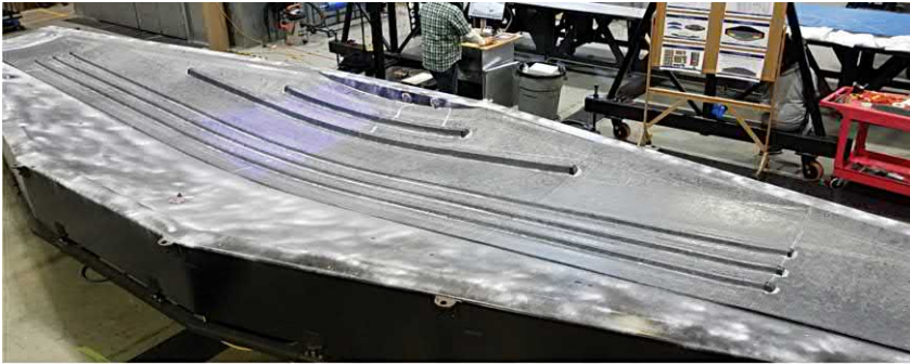
FIGURE 5.28 Blue light used to measure the part deformation precure and postcure.
