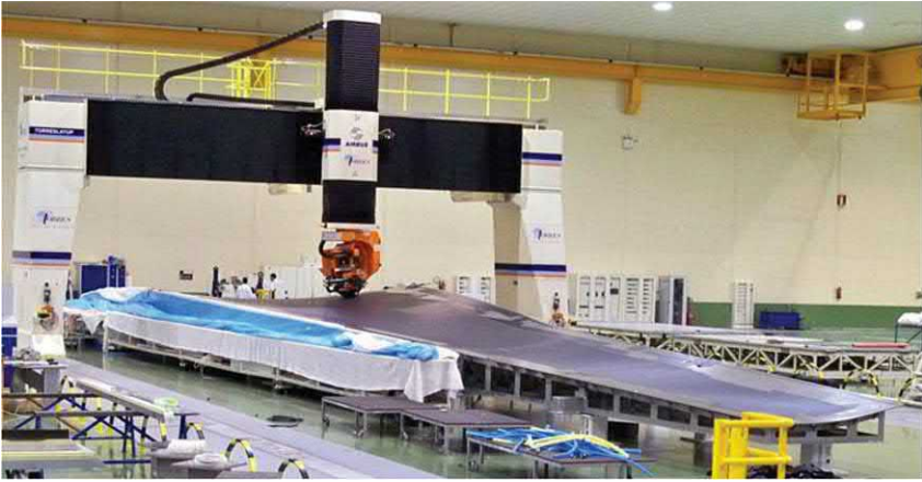
FIGURE 5.53 Aerospace part lamination example using AFP [43].
