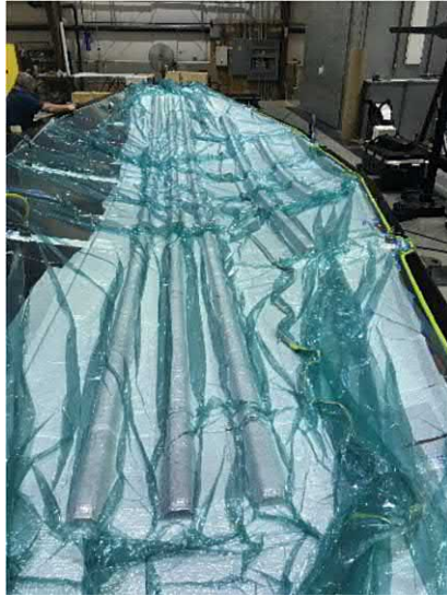
FIGURE 5.25 Bagging pleats used around the part.
