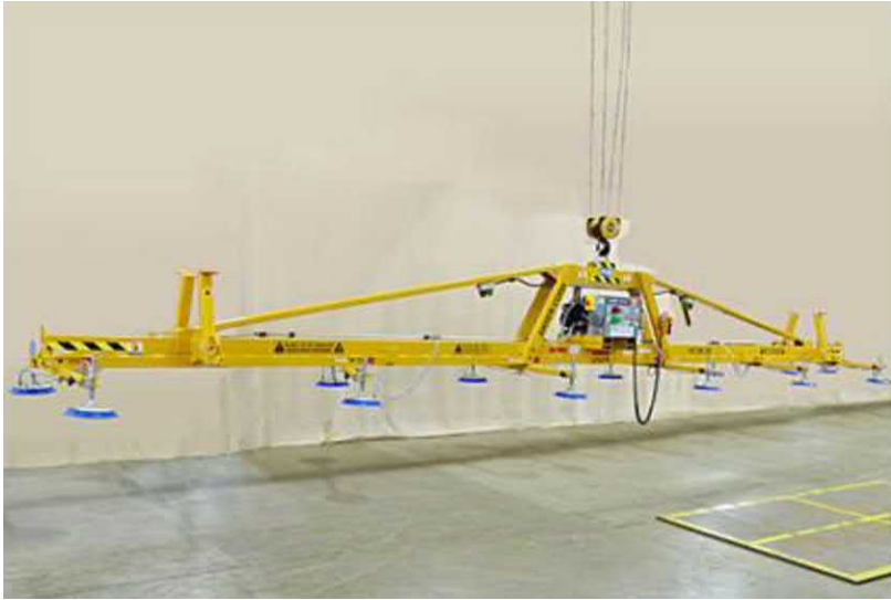
FIGURE 4.23 Assembly fixture tool with integrated vacuum suction cups.
