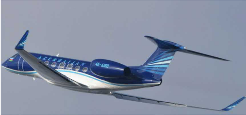
FIGURE 2.13 The Gulfstream G650's tail rudder and elevators are made of carbon fiber/polyphenylene sulfide (PPS) thermoplastic composite [20].
