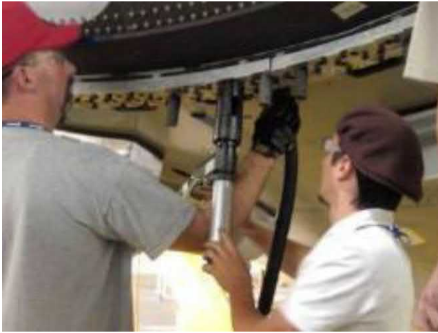
FIGURE 1.19 Match drilling process in aerospace components.
