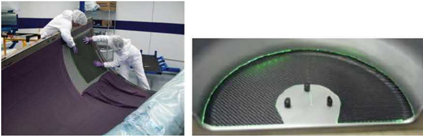
FIGURE 4.8 Laser projection used to simplify the lamination processes during manufacturing [3].
