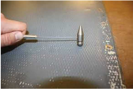
FIGURE 6.41 Tap test occurring on a composite part [29].
