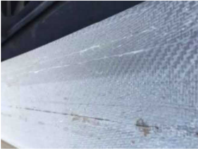
FIGURE 3.5 Scratches from knife cuts on a lamination tool.
