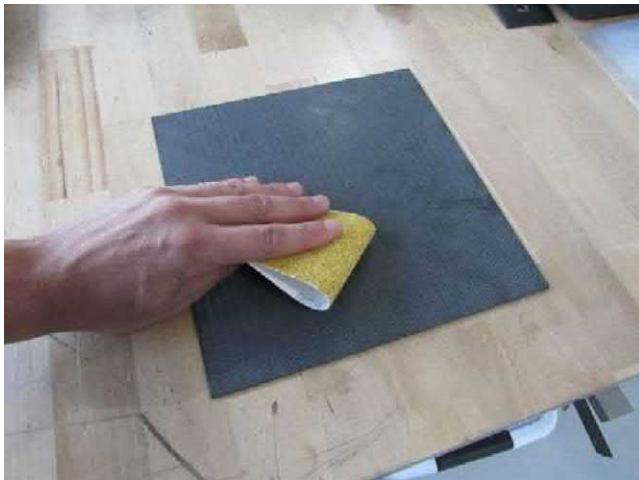
FIGURE 3.9 Example of hand sanding process of composite.
