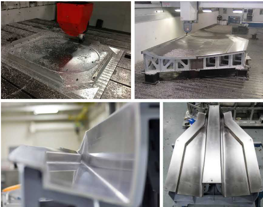
FIGURE 3.1 Metallic lamination tooling examples [1–3].
