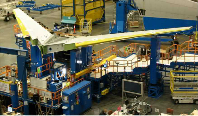
FIGURE 6.12 Combination of assembly platform and ground support equipment [11].
