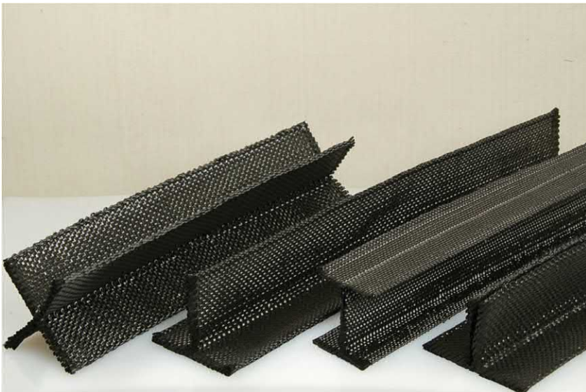
FIGURE 5.39 Example of composite preform used in RTM [33].
