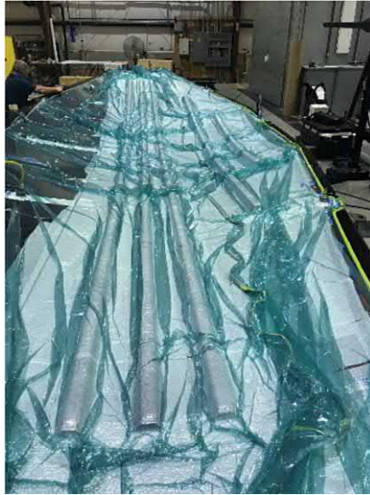
FIGURE 5.25 Bagging pleats used around the part.
