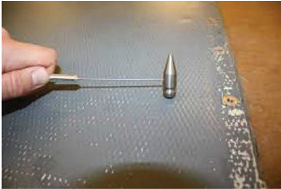
FIGURE 6.41 Tap test occurring on a composite part [29].
