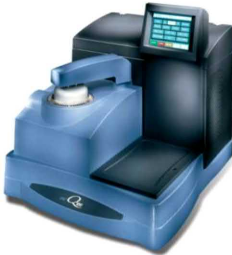
FIGURE 2.18 Modulated differential scanning calorimeter [24].
