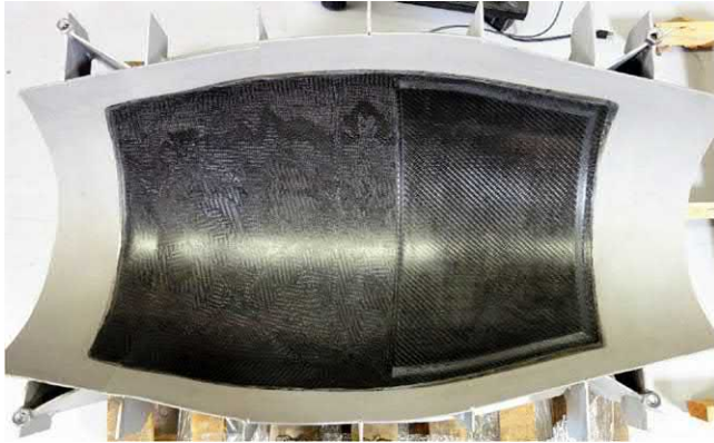
FIGURE 1.12 HyVarC tooling with invar base and composite face sheet.
