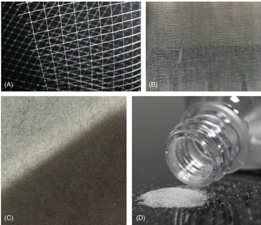
FIGURE 3.13 Bondline control techniques (A) Woven scrim cloth, (B) Knit carrier, (C) Non-woven (mat), (D) glass beads.
