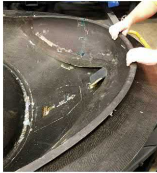
FIGURE 4.18 Example of a removable draft lock feature on a composite lamination tool.
