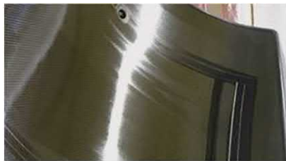
FIGURE 6.1 Illustration of the wetting of Marbocote W1151B release agent onto a carbon/epoxy tool [2].
