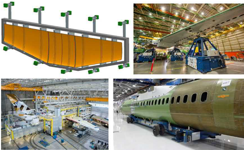
FIGURE 1.17 Assembly tooling used for airplane production.
