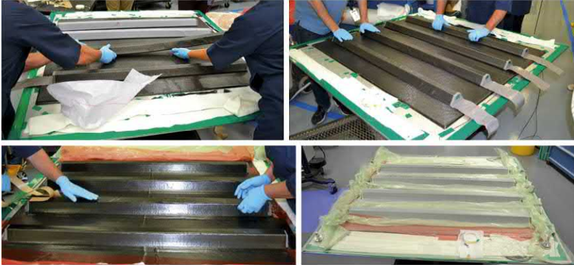
FIGURE 7.24 Fabrication steps of the hat stiffened panel.
