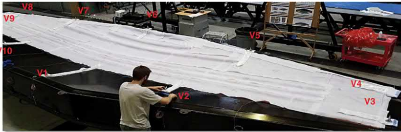
FIGURE 5.24 Thermocouple location across the part.
