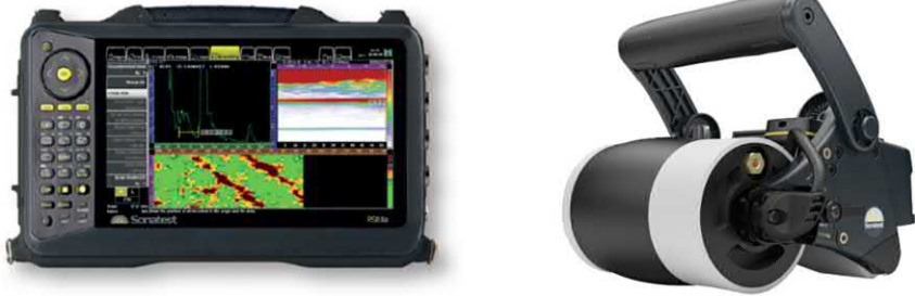
FIGURE 6.43 Pulse echo ultrasonic inspection equipment typically used for composite structures [30].
