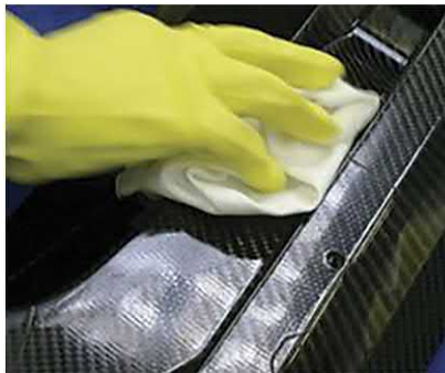
FIGURE 6.2 Release agent being wipe-applied to a carbon/epoxy composite mold [2].
