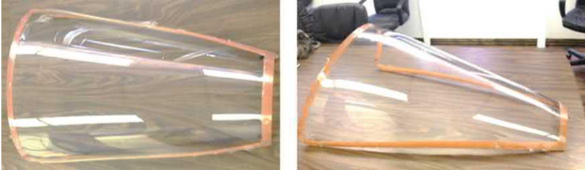
FIGURE 2.12 Example use of PC material in aircraft canopies.
