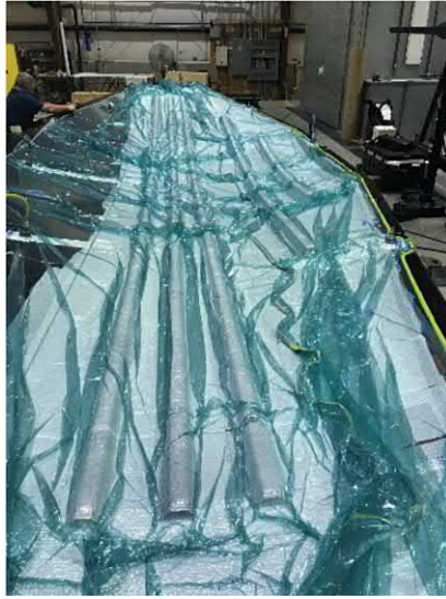
FIGURE 5.25 Bagging pleats used around the part.
