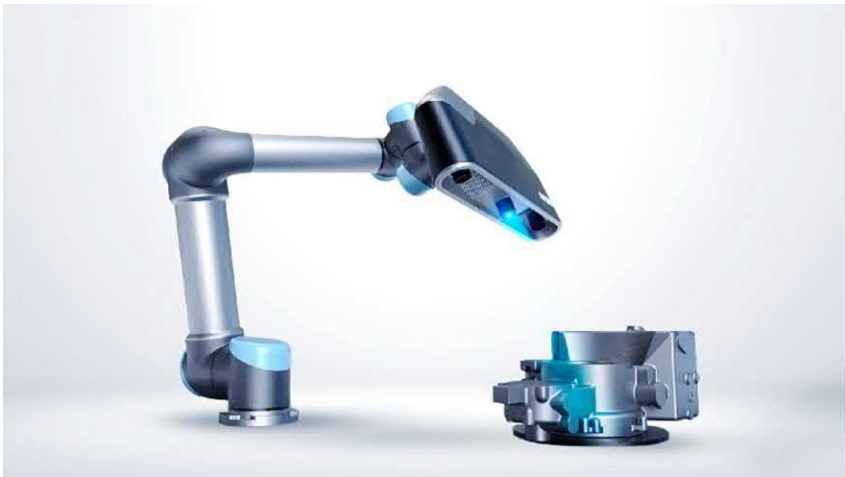
FIGURE 6.30 Blue light technology scanning process [20].
