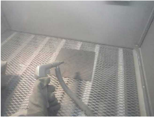
FIGURE 3.10 Example of grit blasting of composite surface.
