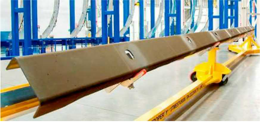
FIGURE A1 Example of a composite spar part used on aircraft structures.
