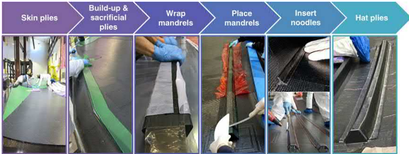
FIGURE 5.15 Overview of the lamination process used for the wing skin demo.
