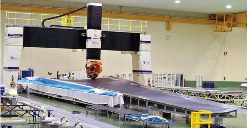
FIGURE 5.53 Aerospace part lamination example using AFP [43].
