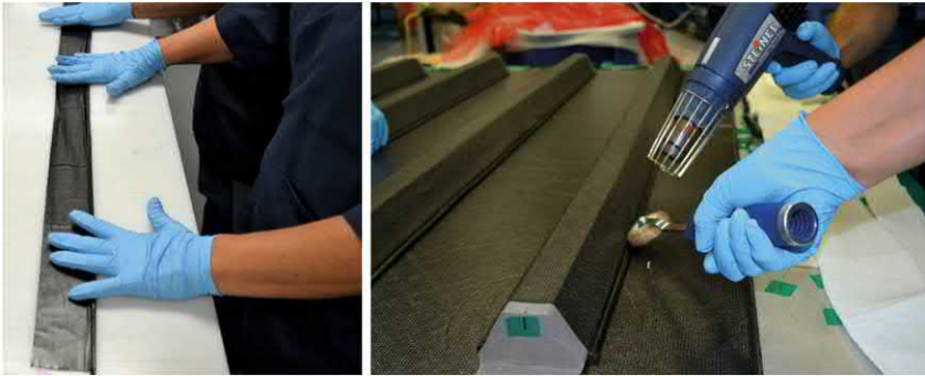
FIGURE 7.20 Rolled tow filler fabrication approach.
