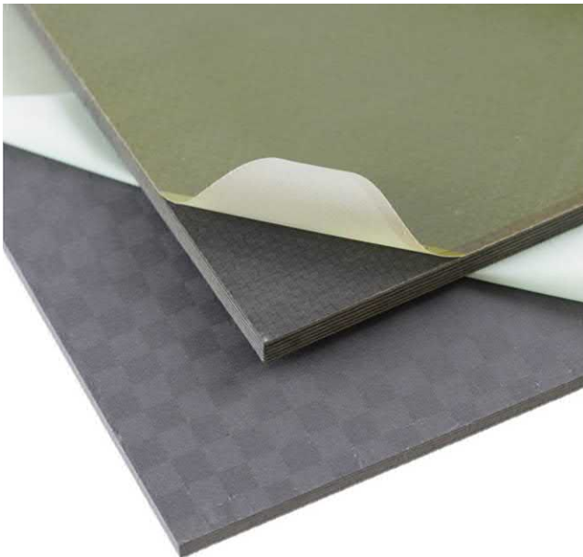
FIGURE 3.8 Peel ply example used on composite panel.
