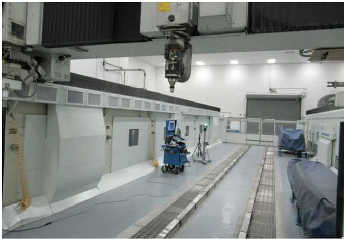
FIGURE 6.35 5-axis machine typically used for composite machining [22].
