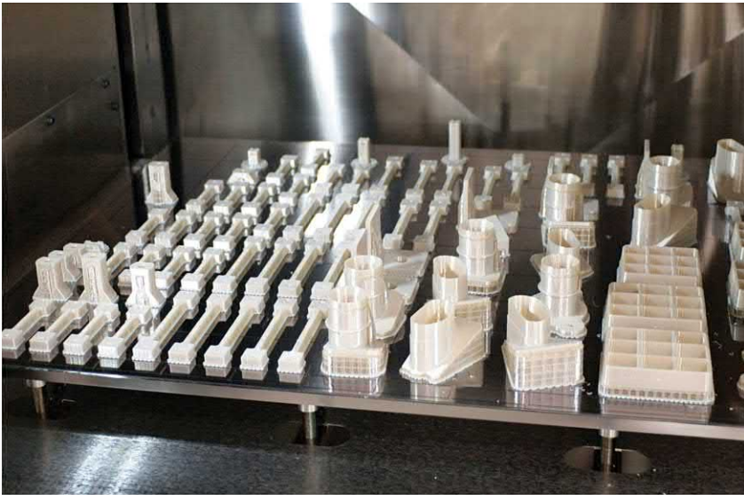
FIGURE 2.14 Aircraft part made from Ultem material [21].
