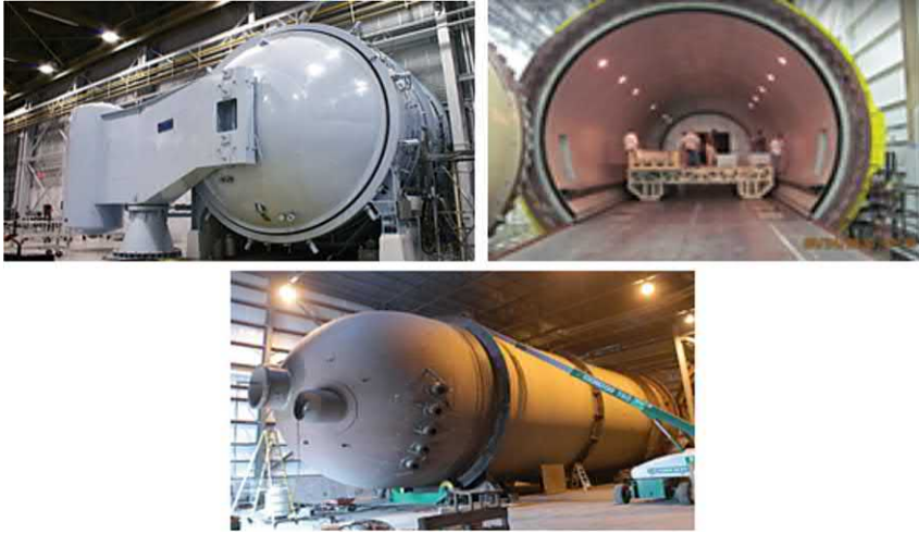
FIGURE 8.4 Large scale autoclaves used to fabricate composite parts [11].
