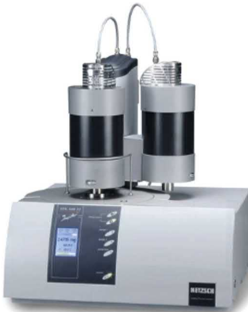
FIGURE 2.17 Thermal gravimetric analyzer used during thermal stability analysis [23].
