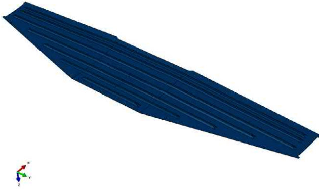
FIGURE 5.61 Wing skin example that was used to demonstrate AFP/ATL process restrictions.
