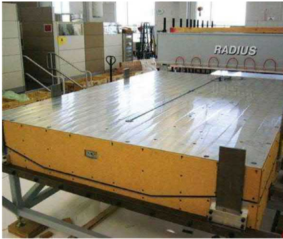
FIGURE 5.43 Mold closed and resin being injected [37].
