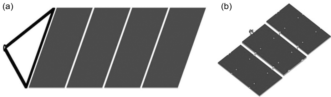
FIGURE 7.14 Solar wing deployment configuration (a: series type, b: parallel type).
