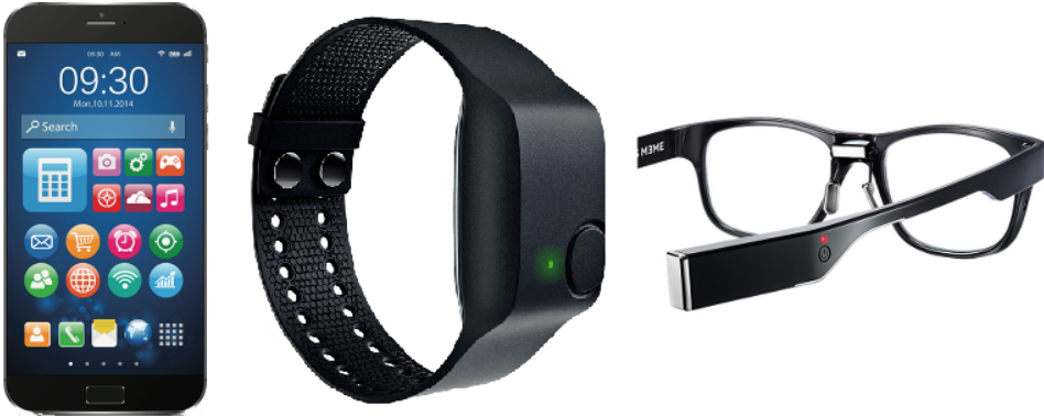
Figure 5.1: Wearable devices become more important for activity recognition since new sensor modalities are integrated into them. A smartphone is typically equipped with an accelerometer, gyroscope and magnetometer. Smartwatches have pulse-sensors and sensors for electrodermal activity [3] and some smartglasses offer electrooculography [1].
