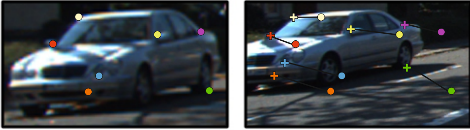
Figure 4.6: An illustration of object observation computation based on point matching.
