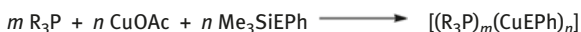
Figure 10.8: Synthesis of phosphine-stabilized copper(I) chalcogenolate clusters with varying ratios of phosphine and trimethylsilylchalcogenide reagents [83].
