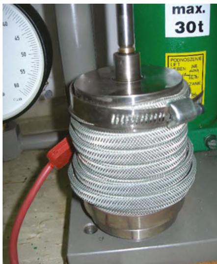
**Figure 1.5:** External heating of HP reactor chamber.
