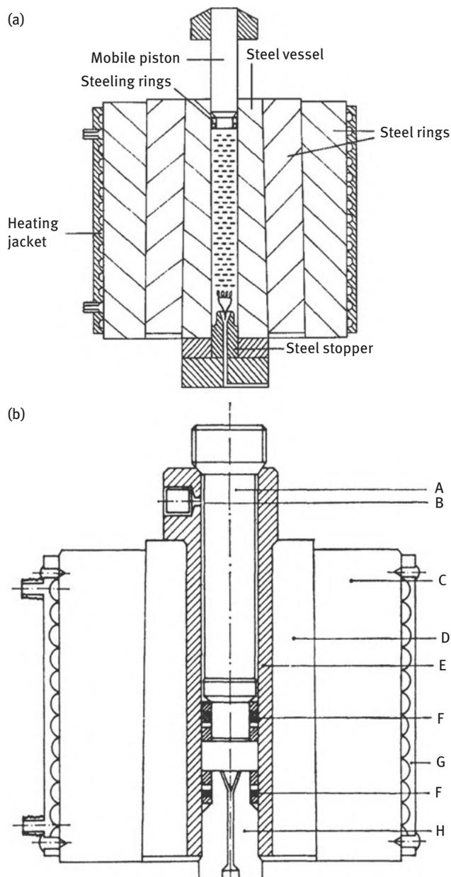
**Figure 1.4:** (a) Reaction chamber of piston-cylinder HP apparatus. Reproduced with permission from Jurczak J, Chmielewski M, Filipek S. *Synthesis*, 1979, 41–42. Copyright Georg Thieme Verlag KG; (b) Apparatus with gas inlet. Reproduced with permission from Jurczak J. *Bull Chem Soc Jpn* 1979, 52, 3438–42. Copyright Japan Chemical Society.
