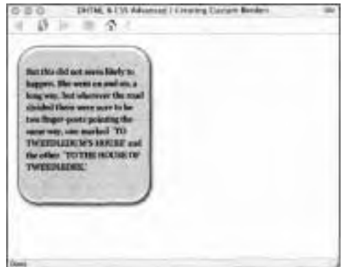
Figure 5.25 The final layout with all of the pieces in place. This technique can stretch vertically indefinitely and horizontally 750 pixels.
