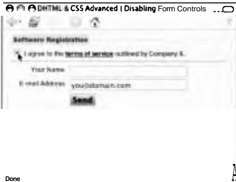
Figure 8.27 After the visitor checks to accept the terms, the form fields become active and look as if they can be typed in.
