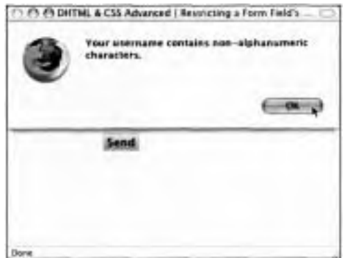
Figure 8.25 If the visitor enters something other than letters, numbers, or an underscore, an alert appears.
