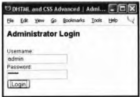
Figure 10.10 This is the login. php page. Any page that includes the securePage. php file will forward the visitor here if the user name is not in the session.
