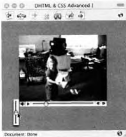
Figure 7.18 QuickTime controls for volume, play, and scrub are built into the player.
