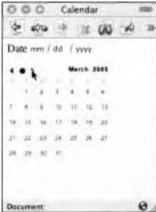
Figure 7.15 Clicking the controls allows you to move forward or backward in the calendar. Clicking the circle flips you back to the current month from wherever you are.
