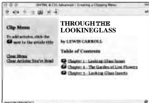
Figure 6.31 When the page first loads, the clipping menu is empty, ready to be filled by clicking the icon next to an article title.
