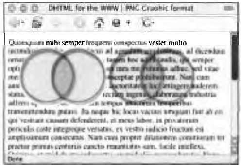
Figure 9.23 Both images are the same, but the left graphic was saved as a GIF and the right as a PNG. Notice that the GIF image covers the text even in transparent areas, while the text shows through the PNG.
