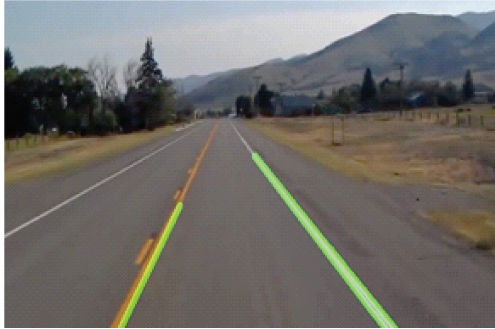
Figure 3.1 Example of lane marking detection.
