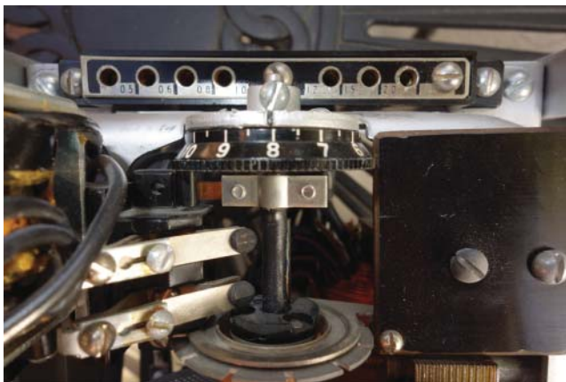
Figure 4.9 Close-up showing pickup taps and time dial. Source: Courtesy of GE.
